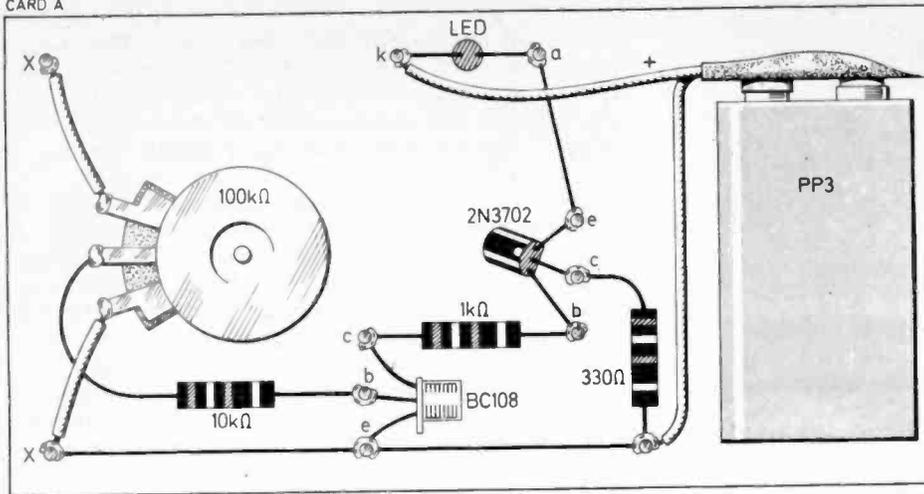
Fig. 3.10. The card required to go inside the box, glued to the inside of the lid. Nails or pins are mounted in all positions as shown. Be careful when inserting the pins that they do not come all the way through the other side. The two nails marked X are the only two to be inserted from the outside of the box. They then form the terminals.
