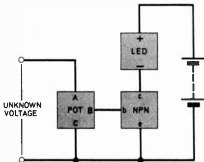
Fig. 3.6. In this experiment we are using an amplifier, driven by a voltage from the POT to light the LED
