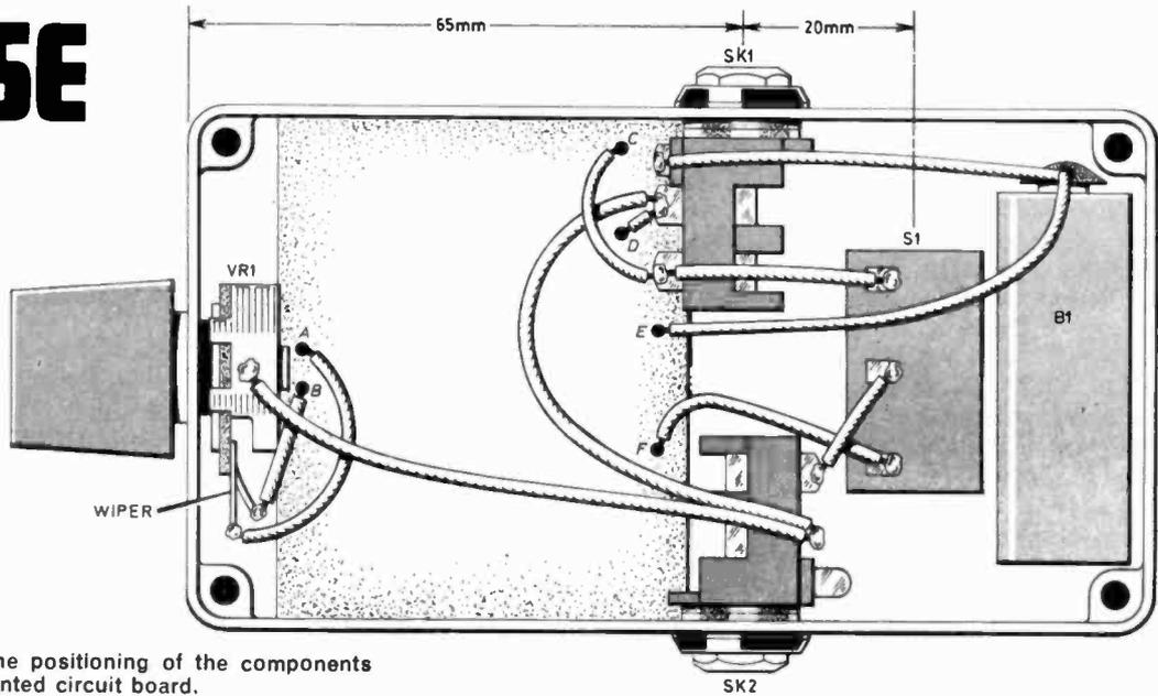
Fig. 2 (below). Shows the positioning of the components on the topside of the printed circuit board.
