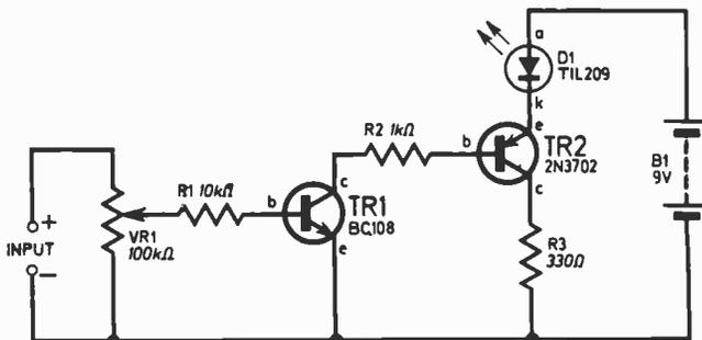
Fig. 3.9. A more compact version of the previous figure. This is the circuit diagram of our VOLTAGE INDICATOR.
