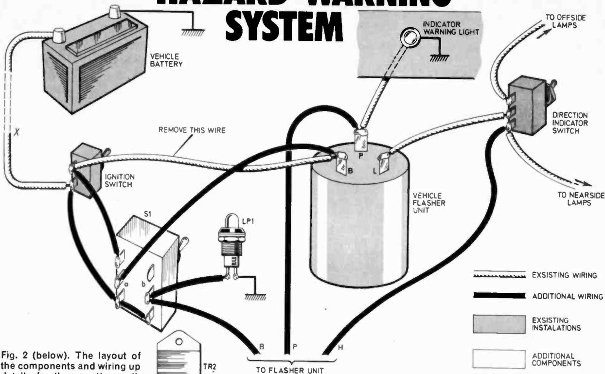
Fig. 2 (below). The layout of the components and wiring up details for the *negative earth* system.
