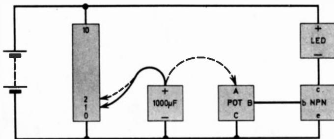
Fig. 3.7. Using a capacitor module to test the idea that the RESISTOR CHAIN really does divide the battery voltage by ten.
