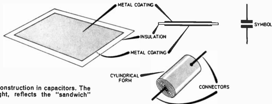
Fig. 3.2. A typical form of construction in capacitors. The symbol shown to the right, reflects the "sandwich" construction of a capacitor.
