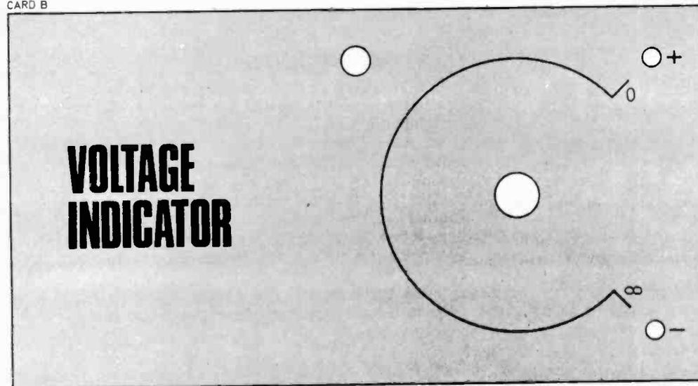
Fig. 3.11. The covercard required, shown full size, to be affixed to the top. No intermediate markings have been given, as the position of each depends on the individual tolerances of the components used to construct the module.
