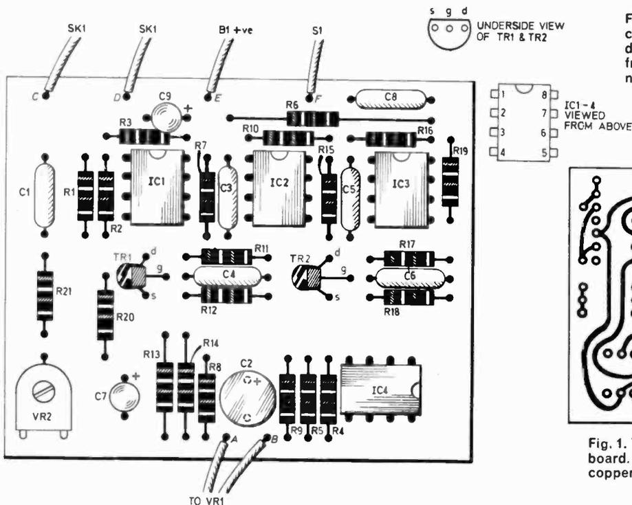
Fig. 3. The layout of the components in the case showing position and wiring up details. Note that VR1 is spaced away from the inside of the case with an extra nut to allow the lid to fit in place.
