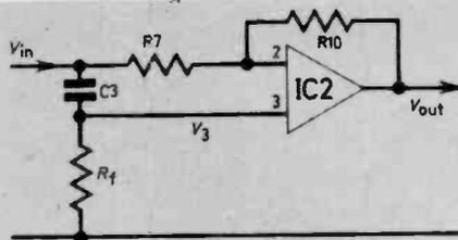
Fig. 4. A simplified phase delay segment.
