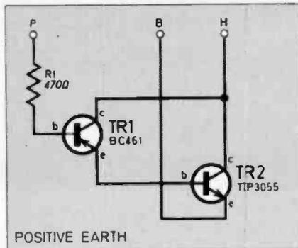
Fig. 6. The complete circuit diagram of the Hazard Warning System for both negative and positive earthing systems.
