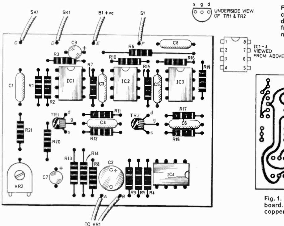
Fig. 3. The layout of the components in the case showing position and wiring up details. Note that VR1 is spaced away from the inside of the case with an extra nut to allow the lid to fit in place.
