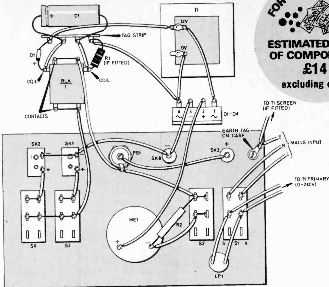
Fig. 2. Layout and wiring of the Emergency Lighting Unit.
