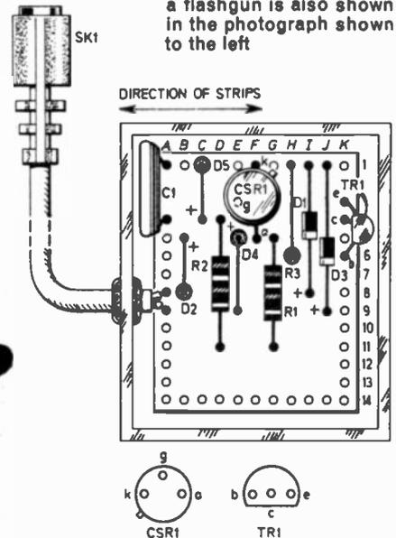
Three extra rows of holes are provided on the component panel so that there is space for mounting holes to be drilled, should it be necessary to bolt the panel to the case. It was not in the case of the prototype because the panel was found to be a firm fit into the housing.
