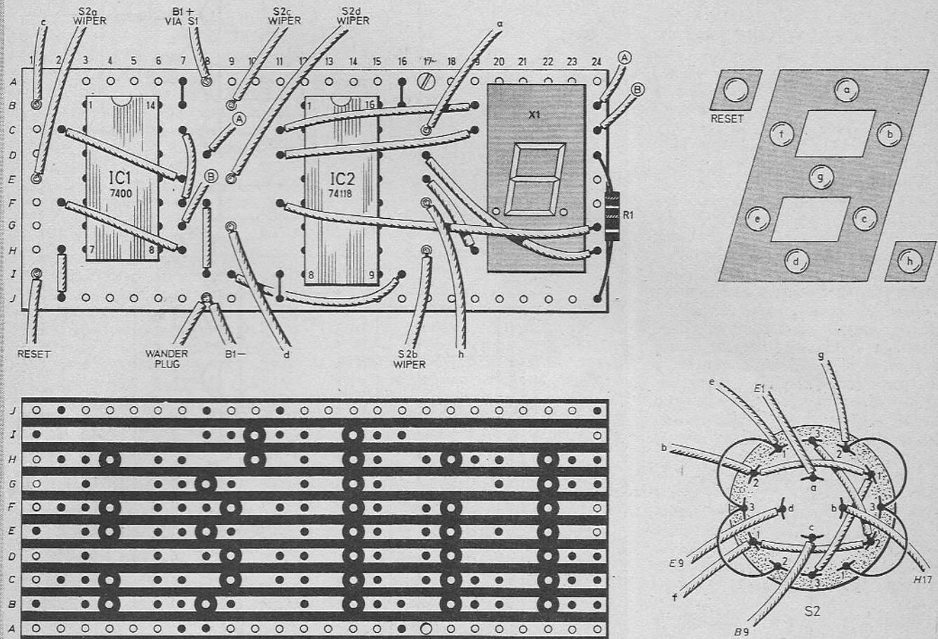
Fig. 6. Component layout and wiring of the stripboard. The breaks in the copper strips are shown above and the wiring for the switch S2 is given on the right.
