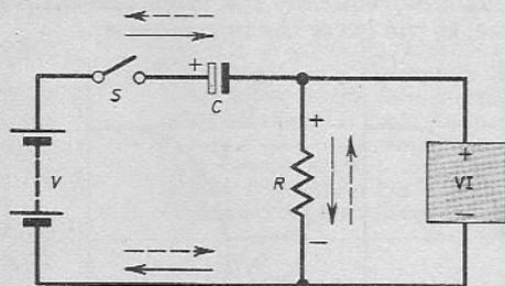
Fig. 4.11. The value of time constants may be demonstrated easily by using the voltage indicator and few additional components.
