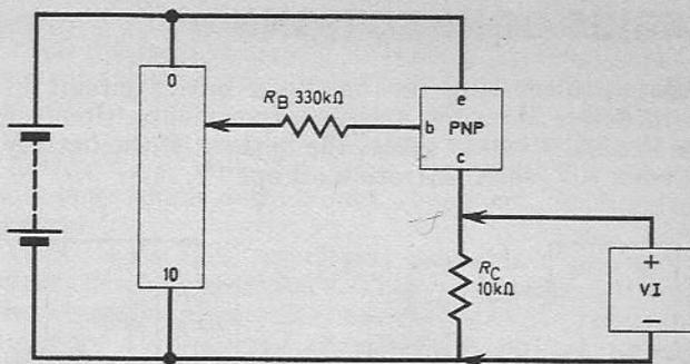
Fig. 4.4. The circuit here is to measure the current gain of the PNP module.
