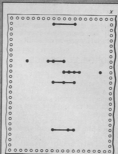
Fig. 3. Underside view of the board. The wire links are shown by the solid lines, the position where the component leads pass through the board as solid dots.
