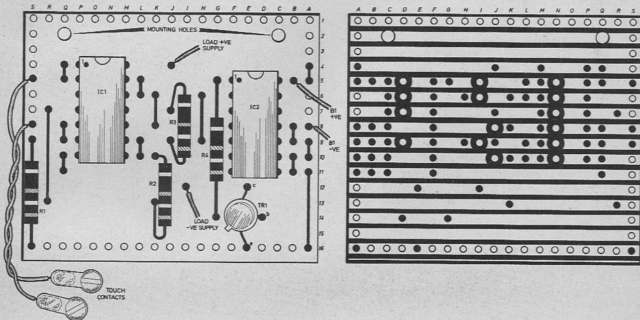
Fig. 1. Component layout and wiring of the touch switch circuit board. The breaks required on the copper side of the stripboard are shown on the right.
