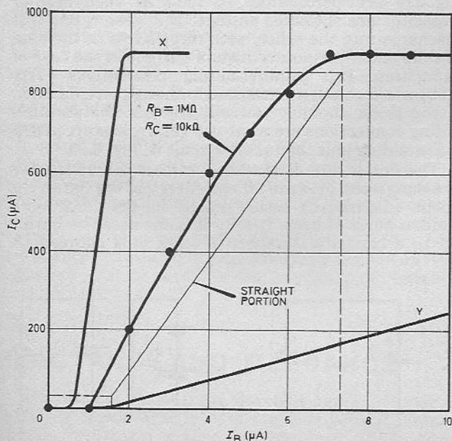
Fig. 4.3. Graph of collector current versus base current. The current gain is given by  $I_C/I_B$ .
