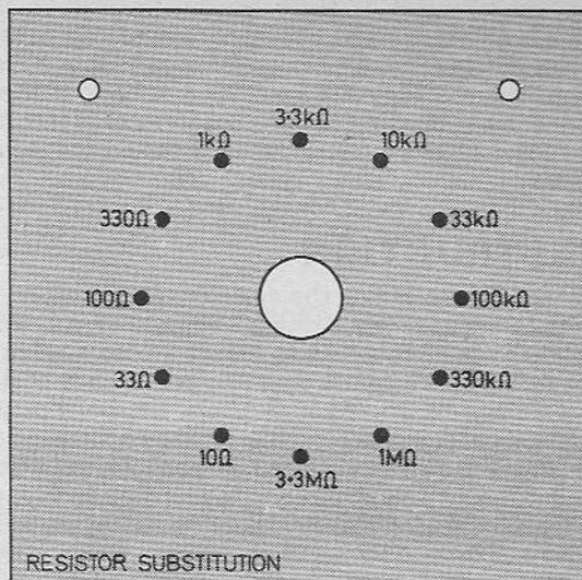
Fig. 4.14. Covercard, shown full size required for the RESISTOR BOX.
