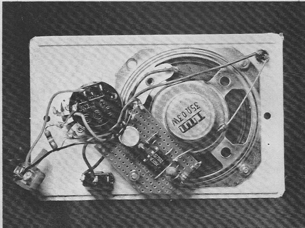
The completed metronome with all the components mounted on the lid of the case.
