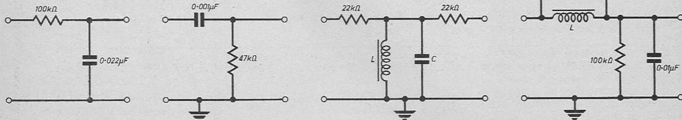
Four examples of voicing circuits. From left to right; Fig. 3. A simple RC filter; Fig. 4. A CR filter; A band-pass filter is shown in Fig. 5 and uses an inductor; Lastly, the filter of Fig. 6 is a band-elimination filter.
