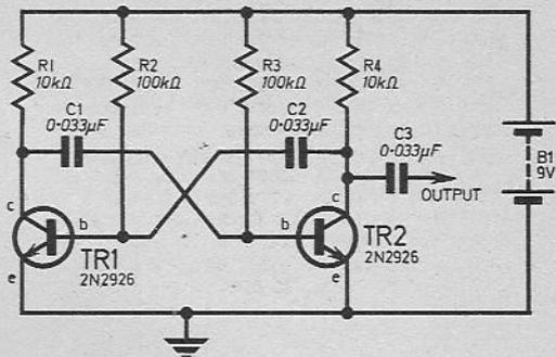
Fig. 1. Basic circuit for a simple organ which may be used with voicing circuits.
