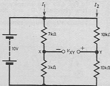
Fig. 4.5. A traditional circuit to illustrate Potential Difference.
