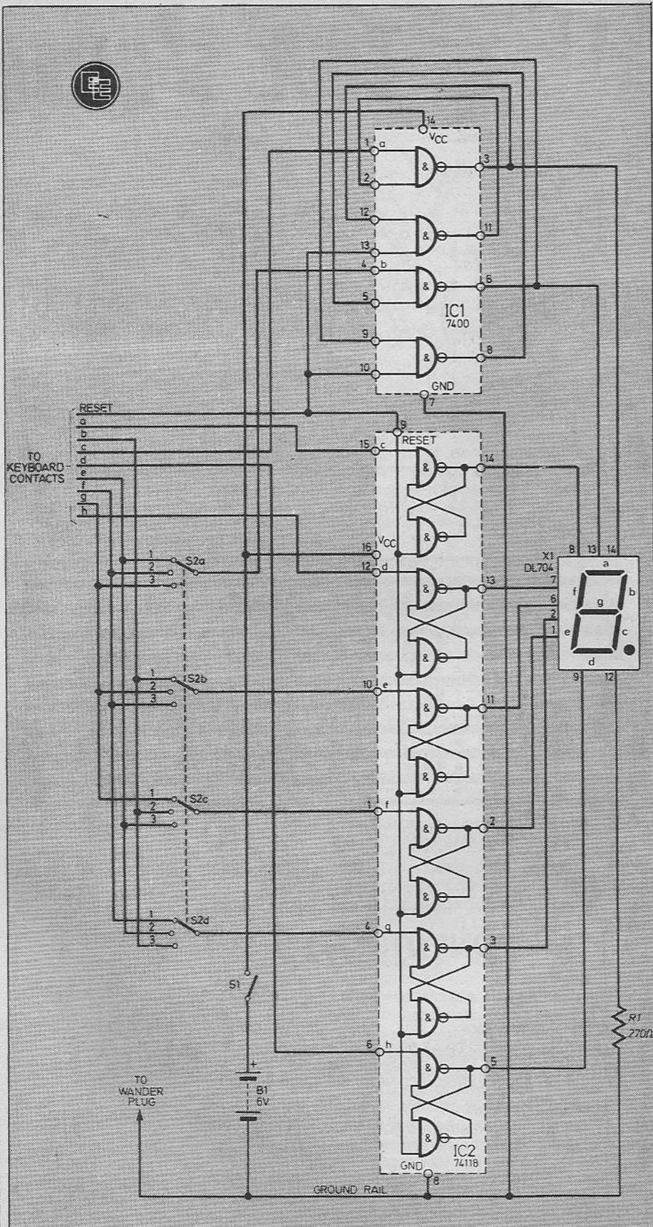
Fig. 5. Complete circuit diagram for the Code Scrambler.
