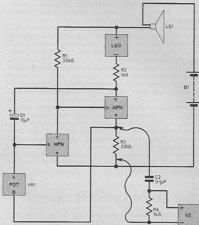
Fig. 4.12. Using the modules as shown construct this simple oscillator. By using the VOLTAGE INDICATOR, the impedance of  $C2$  can be checked.
