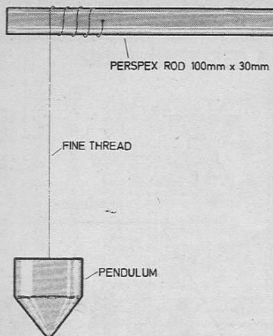
Fig. 1. Constructional details for the pendulum. Perspex is used throughout.
