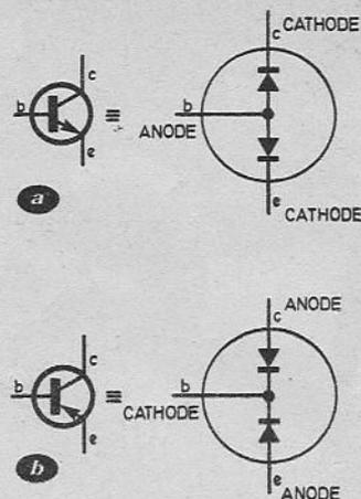
Fig. 3. Representation of transistors in terms of diodes. (a) npn type of transistor (b) pnp type.
