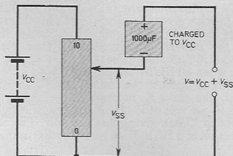
Fig. 4.7. By charging a capacitor to  $V_{cc}$  the net voltage  $V$  may be doubled. Twenty volts from 10V not a bad trick! Using this method the VOLTAGE INDICATOR may be calibrated in steps of 10V.
