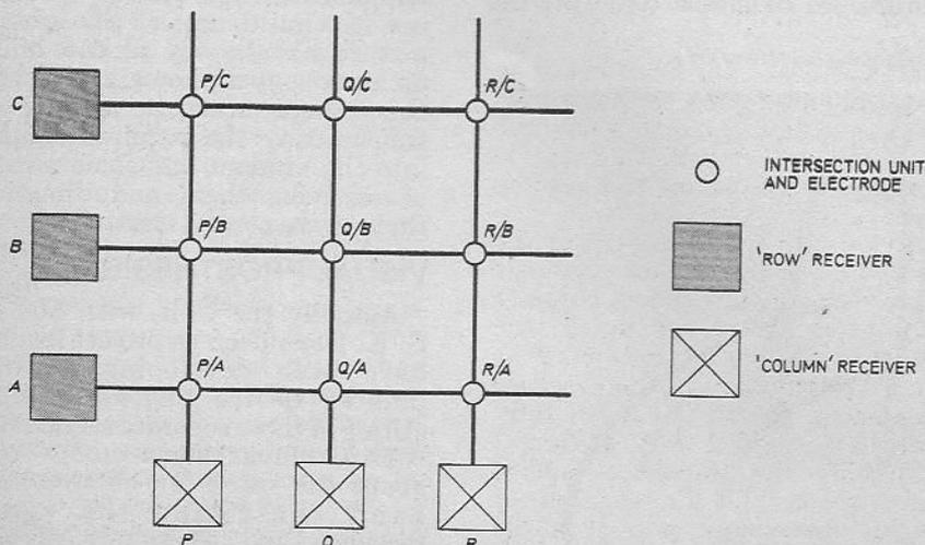
Fig. 2. An implanted "array" system used for present prostheses.
