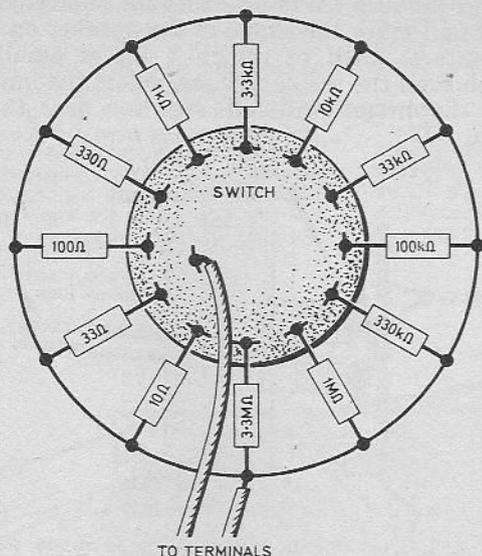
Fig. 4.13. The switch for the RESISTOR BOX is wired according to the method as shown.
