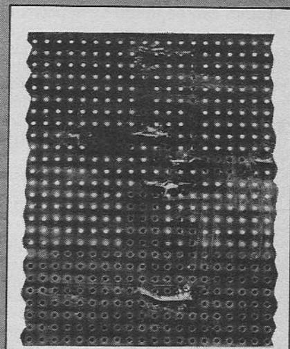
The underside view of the board is shown in this photograph. Note particularly how the leads of the components form the links.
