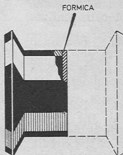
The knob can be attached to the control spindle by means of glue and packing (since the hole is slightly oversize for standard spindles). The more ambitious constructor may wish to install some type of grub screw, so that the knob can be removed when required.
