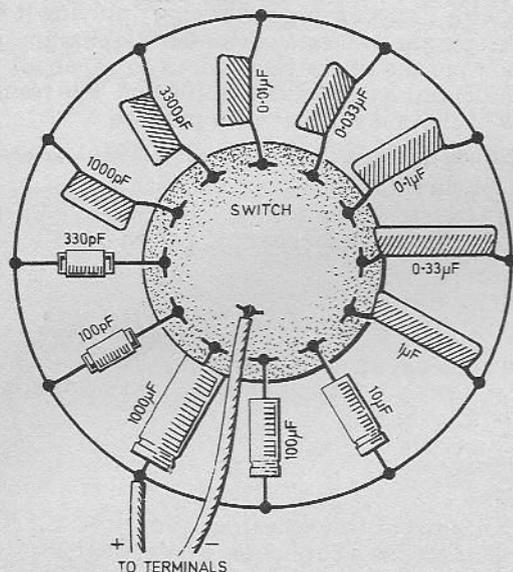
Fig. 4.15. The wiring for the CAPACITOR BOX. Observe the polarity of the electrolytic capacitors.
