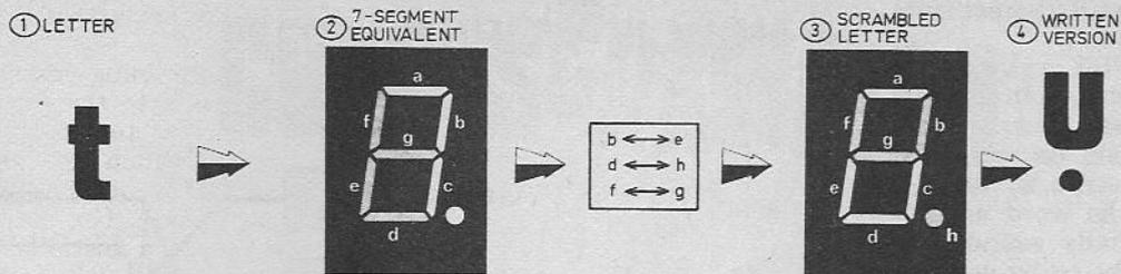
Fig. 1. The principle of the Code Scrambler.
