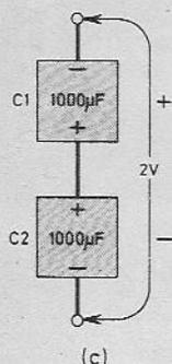
Fig. 4.6a. Connect the modules as shown to the RESISTOR CHAIN. Leave them charging for about 20 seconds. Now disconnect them and apply them to the VOLTAGE INDICATOR as in Fig. 4.6b. The voltage should be 10V. Now disconnect C1 and connect it up upside down as in Fig. 4.6c. What is the voltage across the two capacitors now?
