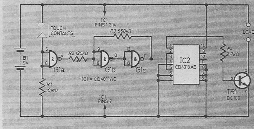
Fig. 2. The complete circuit diagram of the Electronic Touch Switch.
