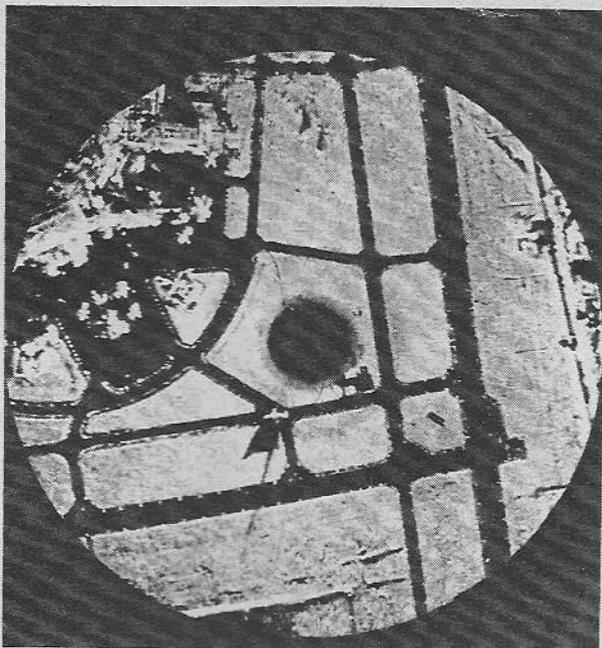
High-definition surface movement radar at Rome Airport built by Decca Radar. An aircraft can be clearly seen moving along the taxi-way.
