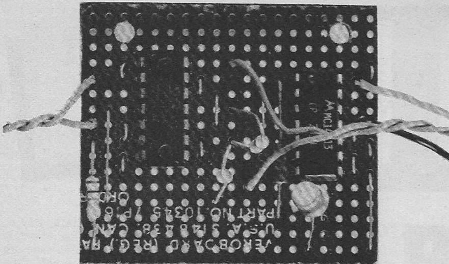
The completed circuit board. Extreme care should be taken when soldering the i.c.s to the board and it may be wise to unplug the soldering iron when doing so.
