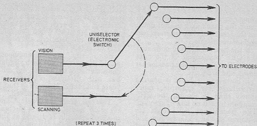
Fig. 3. Proposed future uniselector system for visual prosthesis implant (highly schematic).
