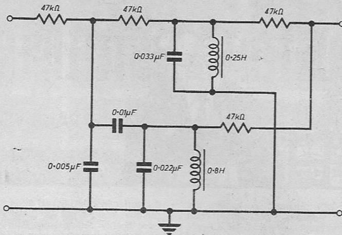
Fig. 7. An example of a commercially made filter; The Baldwin Vox Humana.
