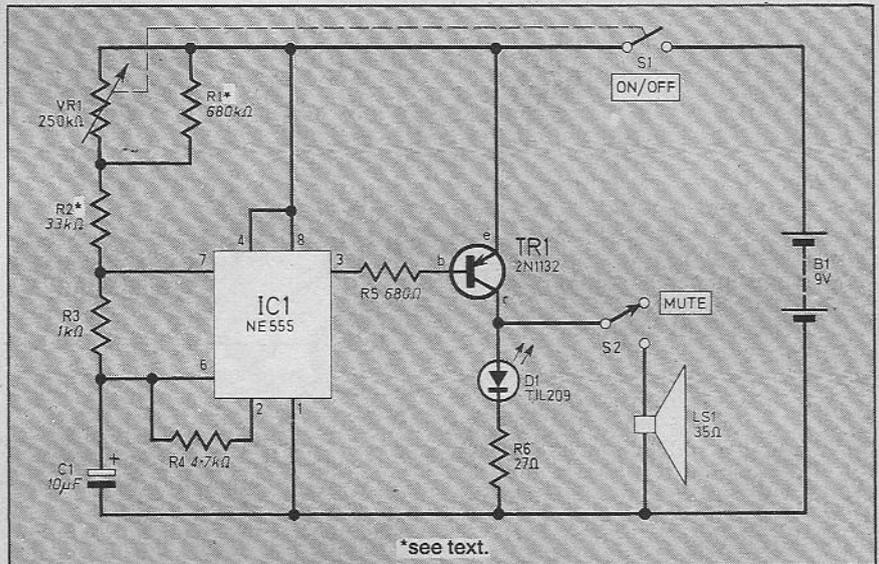
Fig. 1. Circuit diagram for the Audible Visual Metronome. For values of R1, R2 see text.
