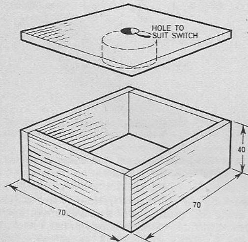
Fig. 4.17. Dimensions of the two boxes. Plywood can be used to construct them.
