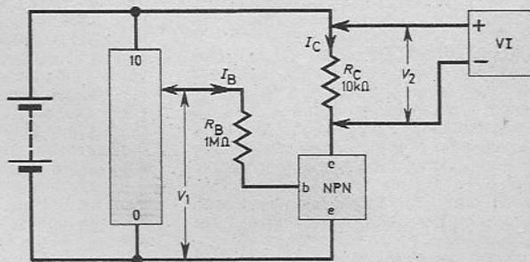
Fig. 4.2. Using the modules as shown, the current gain of the NPN module may be measured.
