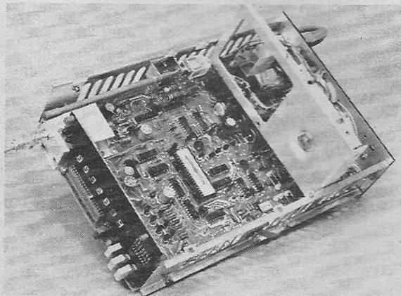
A modern counter/timer instrument manufactured by Marconi Instruments Ltd. Note the l.s.i. circuit (Large Scale Integrated circuit - centre) and the 14 i.c.s, as well as numerous transistors.
