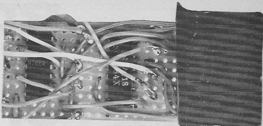
The completed circuit board showing the cardboard mask.
