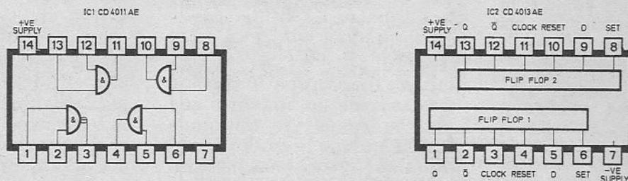
Fig. 3. The leadout details for the 4011 and 4013 integrated circuits.
