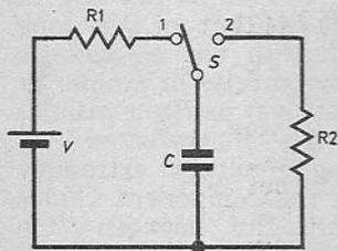
Fig. 4.9. Steadily charging and discharging a capacitor, some idea of the rate of charge is obtained.
