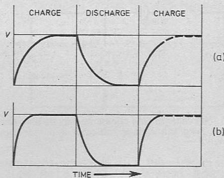
Fig. 4.10. Typical graphs obtained by varying the value of capacitors in Fig. 4.9.
