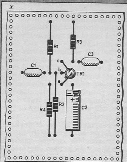
Fig. 2. The physical layout of the circuit in Fig. 1. Shown here is the top with the locations of the components. Note the correct orientation of the polarized components.
