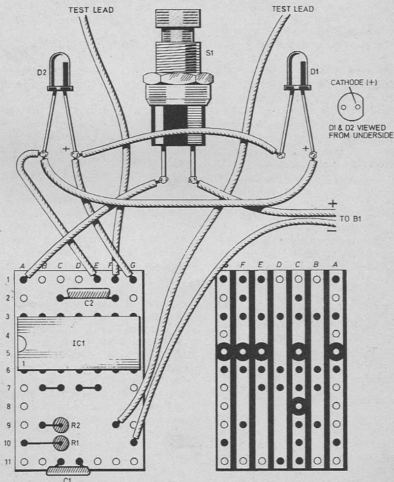
Fig. 2. Component layout and interwiring details for the Rapid Diode Check. The breaks to be made along the copper strips on the underside of the stripboard are shown on the right.
