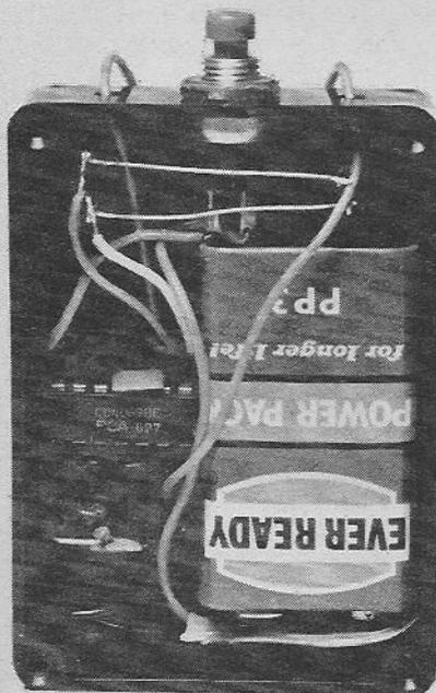
Interior of tester showing positioning of the board, battery and test switch S1.
