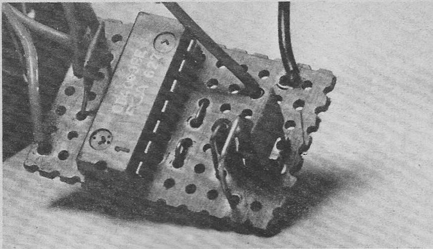
The prototype component board. It would be wise to purchase an integrated circuit holder to save any possible damage to IC1 through soldering.
