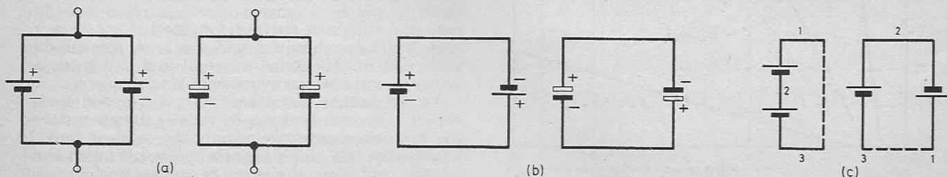
Fig. 4.8a. Parallel opposing connections as shown here are permissible only if the two voltages are the same. Fig. 4.8b & c. Parallel aiding connections as these are forbidden because you are effectively short-circuiting the two components.
