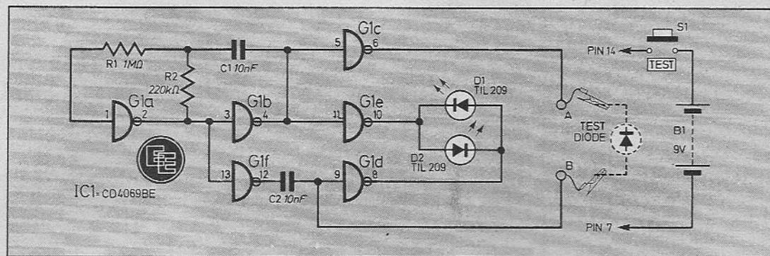
Fig. 1. The complete circuit diagram of the Rapid Diode Check.
