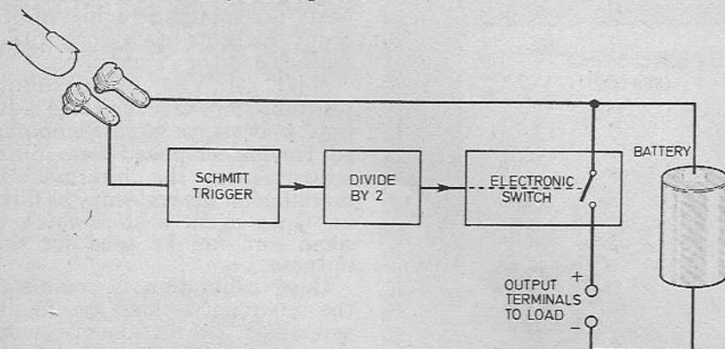
Normally the output of the Schmitt trigger is high (at positive supply level). Consider the load switched off. When the touch contacts are bridged by a finger for example, the output of the Schmitt trigger rapidly drops to a low state (zero volts). This rapid fall in level causes the output of the divide-by-two circuit to change from low to high. This causes the electronic switch to close and power is supplied to the load.
