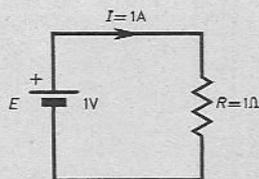
Fig. 4.1. Basic circuit to illustrate Ohm's Law.
