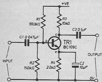
Fig. 1. Circuit diagram of the first stage in a complex amplifier.
