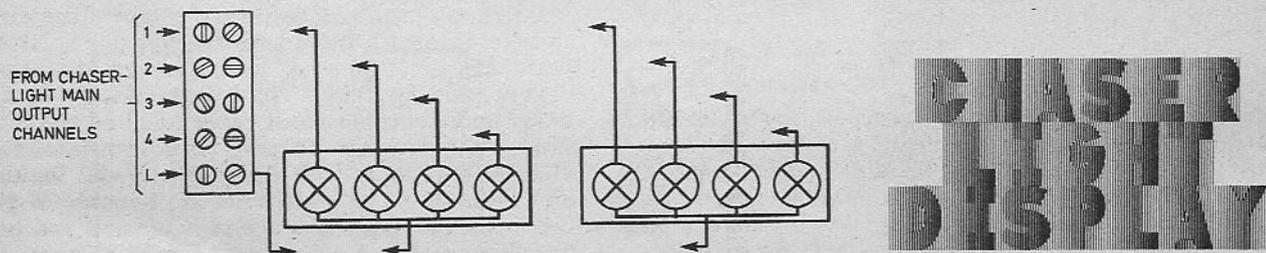
Fig. 5 Light box wiring details to the main unit.
