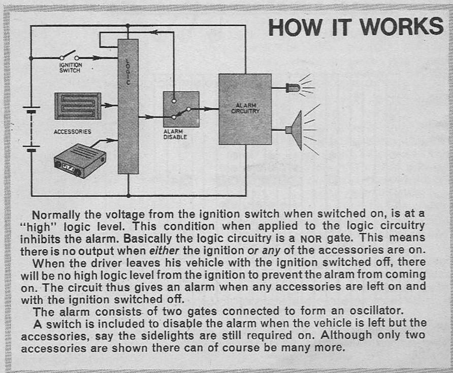
Normally the voltage from the ignition switch when switched on, is at a "high" logic level. This condition when applied to the logic circuitry inhibits the alarm. Basically the logic circuitry is a NOR gate. This means there is no output when *either* the ignition *or* any of the accessories are on.
