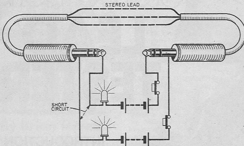
The Stereo/Mono Lead Tester is basically a three-position continuity checker. When a lead is plugged in and one of the switches is pressed the l.e.d. corresponding to that switch should light. If it does not then it would indicate that the lead is open circuit.
