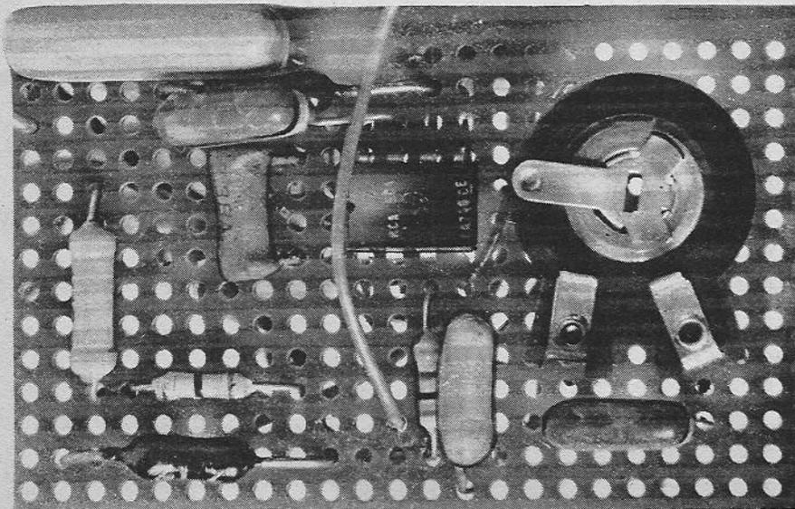
Position the completed component panel between S1 and SK2 so that it has its component side facing SK2 with C5 immediately below SK2. Then wire the panel up to the rest of the unit using ordinary insulated connecting wire. The two connections to SK2 are taken to the component side of the panel and all others are made to the underside.
