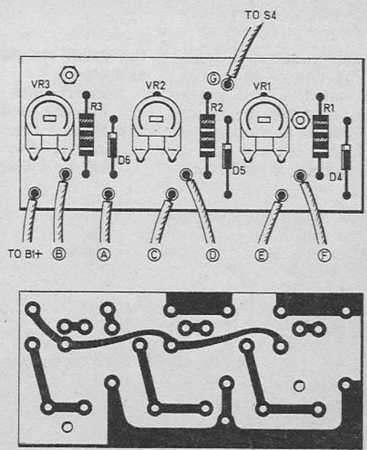
Fig. 2b. Printed circuit board component layout and the underside of the board showing copper tracks after etching (full size).
