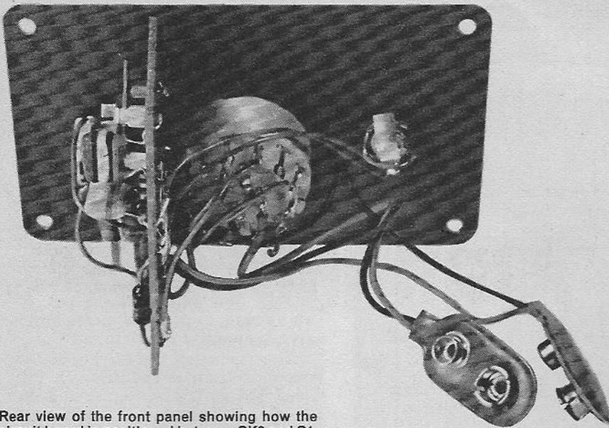
Rear view of the front panel showing how the circuit board is positioned between SK2 and S1.
