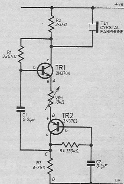
Fig. 1. A simple circuit to illustrate the effect of negative resistance.
