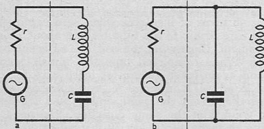
Fig. 5.4. Two ways of connecting an inductor and a capacitor. The first is in series, the second in parallel.
