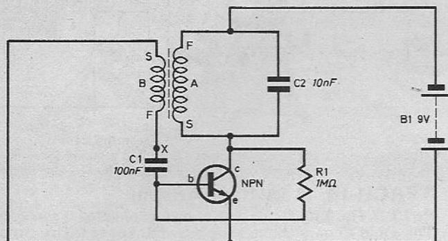
Fig. 5.8. The final circuit we use. This is constructed using the NPN module and the homewound coil. Note the connections to the coil. To check that it is working the **VOLTAGE INDICATOR** may be used.
