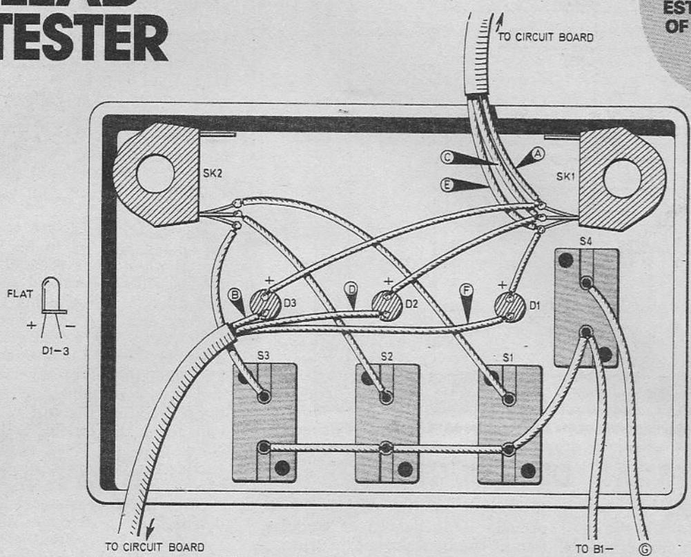
Fig. 2a. Interwiring details for the switches, light emitting diodes (l.e.d.s) and stereo jack sockets.
