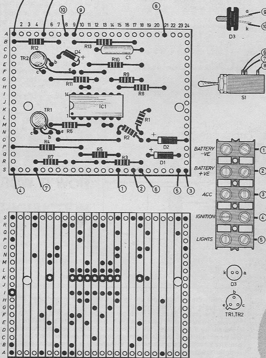
Fig. 3. Interwiring details, circuit board component layout and underside of the stripboard showing breaks in the copper tracks.
