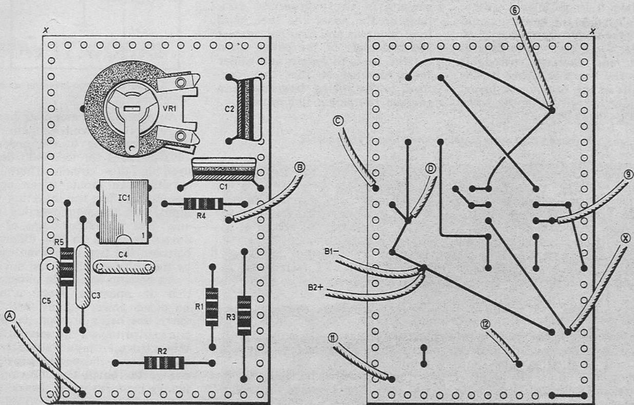
Fig. 3. Component layout and wiring for the plain perforated board. The wiring for the front panel components S1, SK1 and SK2 are also shown.
