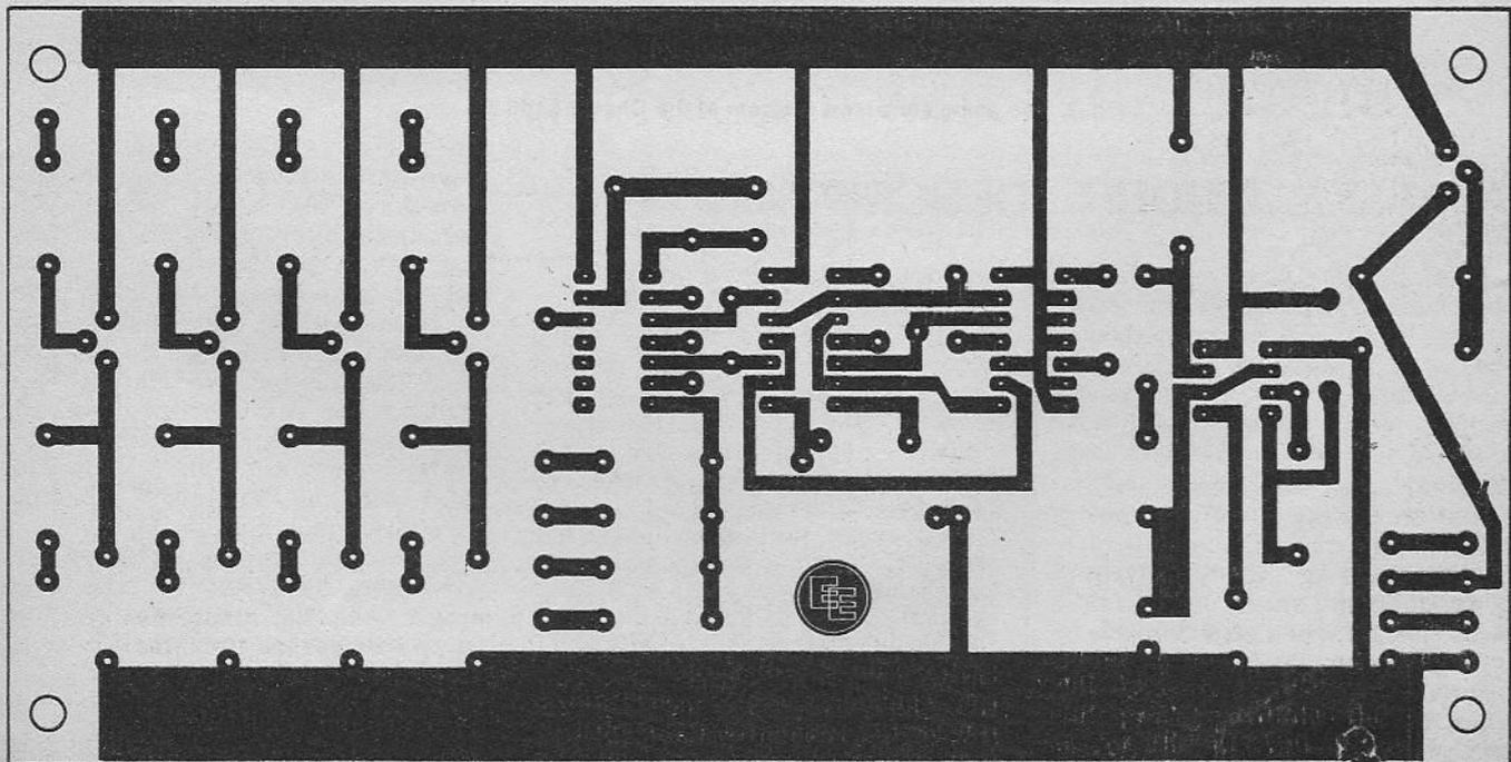
Fig. 1. The copper pattern to be etched on the Chaser Light Display component board, shown full size from copper side.
