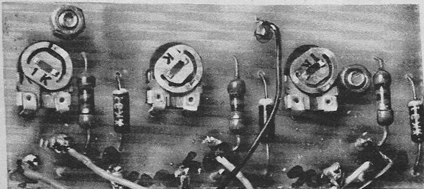
Close-up view of the printed circuit board showing the small preset potentiometers.
