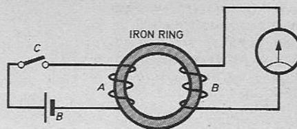
Fig. 5.1. Probably the best known of Faraday's experiments. Here the two coils A and B are coupled by the iron ring.
