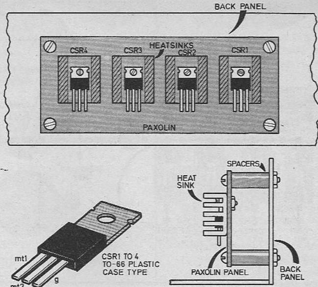
Fig. 3. Details of the triac mounting arrangement and heatsink fittings. Also shows pin configuration for the specified triacs.
