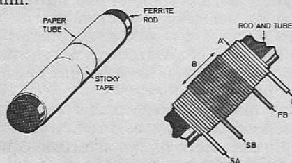
Fig. 5.6. Constructional details for our coil. Insure that the ends of the wires are clearly identified as shown.
