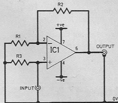
Fig. 1. The basic non-inverting amplifier circuit.
