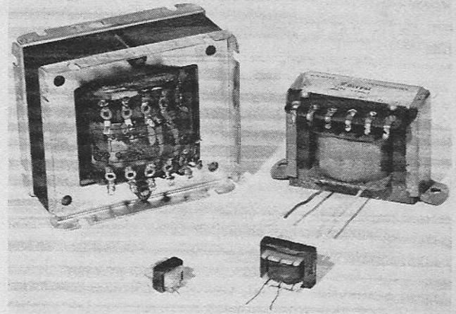
A few examples of transformers using laminated iron cores.
