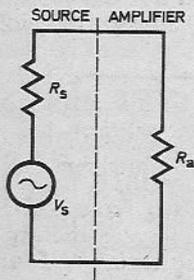
Fig. 5.11. Input impedance of amplifiers can pose quite a problem to a signal source. To obtain maximum output from the amplifier the impedance  $R_a$  should be as large as possible.
