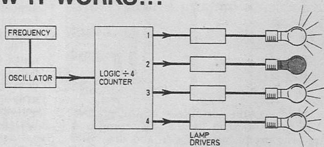
The variable frequency oscillator produces a train of square wave pulses suitable for inputting to a TTL logic section which acts as a divide by 4 counter with four independent outputs. The state of each output (high or low, logic 1 or 0) is dependant on the number of pulses received from the oscillator.
