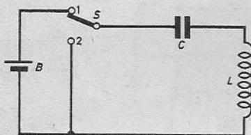
Fig. 5.2. The circuit shown here is helpful in understanding how an inductor behaves when connected to a source of energy.
