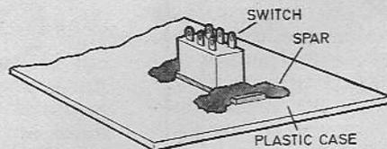
A short length is cut and used as a batten to affix the metal frame to the plastic lid. The diagram shows this more clearly.
