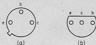
Fig. 2. Pin arrangements for (a) BC184L (b) BC184
