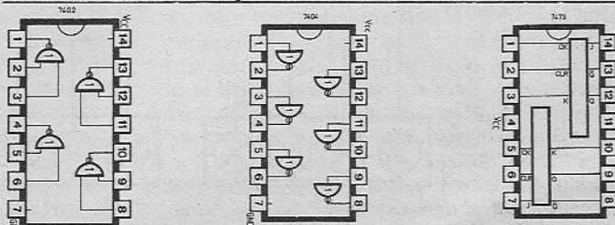
Pin and internal details of the three logic i.c.s employed in the Chaser Light Display.
