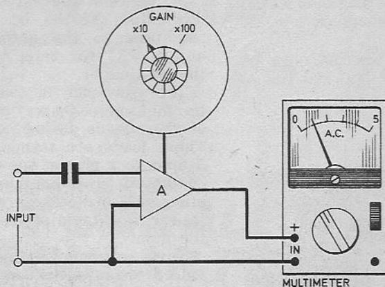
The A.C. Meter Converter is basically an a.c. amplifier with a switched gain of either 10 or 100. The gain being selected by varying the ratio of two resistors. Thus the set-up can be used to measure low level voltages which would be imperceptible using a standard multimeter alone.
