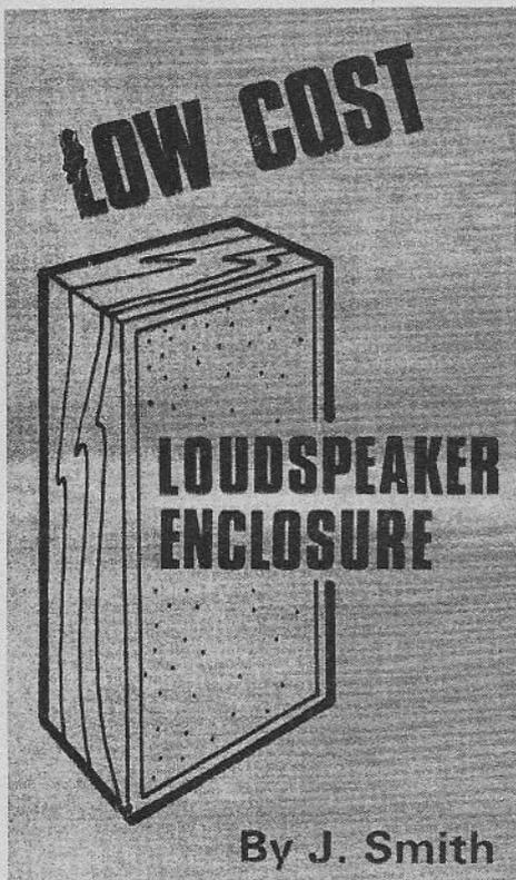
**T**HERE are a large number of old 3 ohm loudspeaker drivers available from out-of-date radio and television receivers. It is possible to use these drivers with modern transistor amplifiers. The trick necessary is to use three in series.
