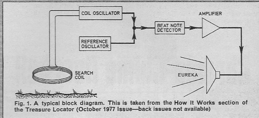
Fig. 1. A typical block diagram. This is taken from the *How It Works* section of the *Treasure Locator* (October 1977 Issue—back issues not available)
