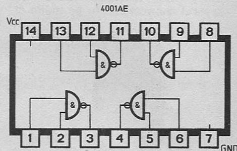
Pin configurations for the CD4001AE.
