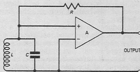
Fig. 5.5. A simple oscillator circuit. The circuit is tuned by the combination LC circuit.
