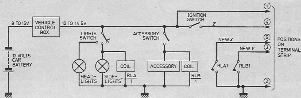
Fig. 4. Circuit diagram for use on Positive Earth vehicles.
