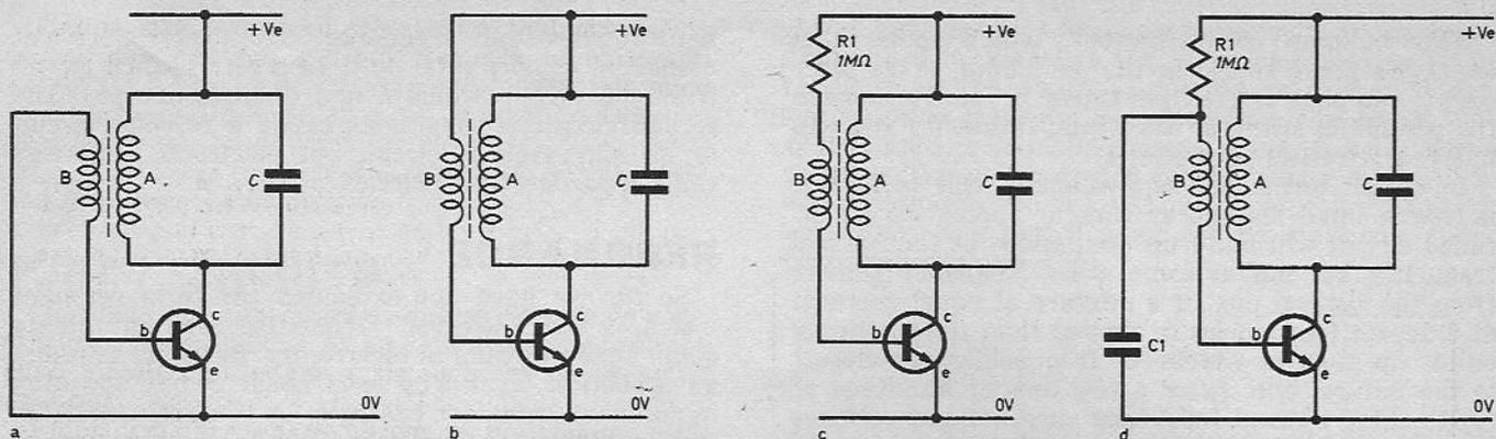
Fig. 5.7. Four ways of connecting our coil into a transistor circuit. The first (a) will not work as there is nothing to turn the transistor on. In (b) the transistor is turned on too much, whereas although (c) is satisfactory, the a.c. current is impeded. By adding a capacitor as in (d) this problem is solved.
