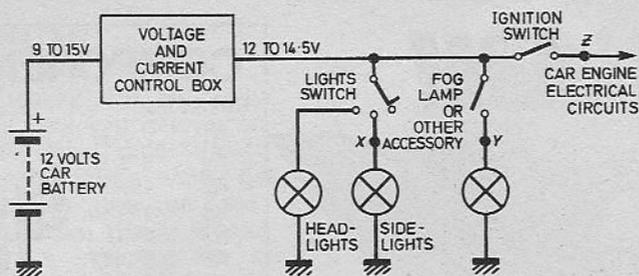
Fig. 1. A typical car electrical system.
