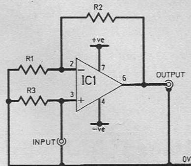
Fig. 1. The basic non-inverting amplifier circuit.
