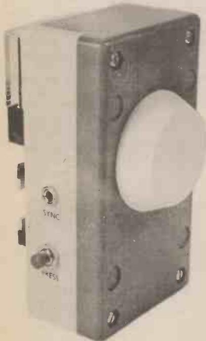
Rear of the finished unit showing the light diffuser.
