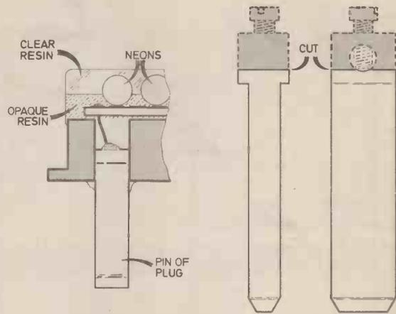
Fig. 3. Method of modifying the 13A plug pins.
