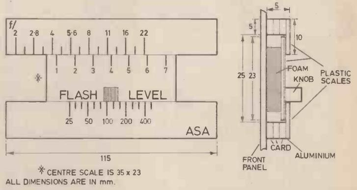
Fig. 4. Constructional details for the calculator. Note that the scale is in three sections. The middle section being slightly deeper than shown so as to fit under the two outer scales. All three are drawn full size and may be used as templates. The general arrangement can be seen in the photographs.
