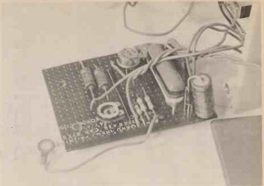
The Flashmeter circuit board removed from the case showing the layout of components.
