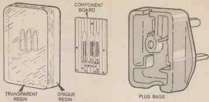
Fig. 1. Exploded view of the Mains Tester showing the two layers of resin and the component board.
