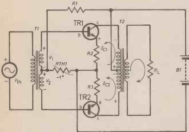
Fig. 8.6. Although this circuit seems complicated, the operation is quite easy to understand providing note is taken of the direction of currents.
