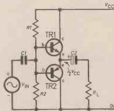
Fig. 8.7. A basic complementary output stage. Although both transistors should be identical with respect to their ratings, one should be npn and the other pnp.
