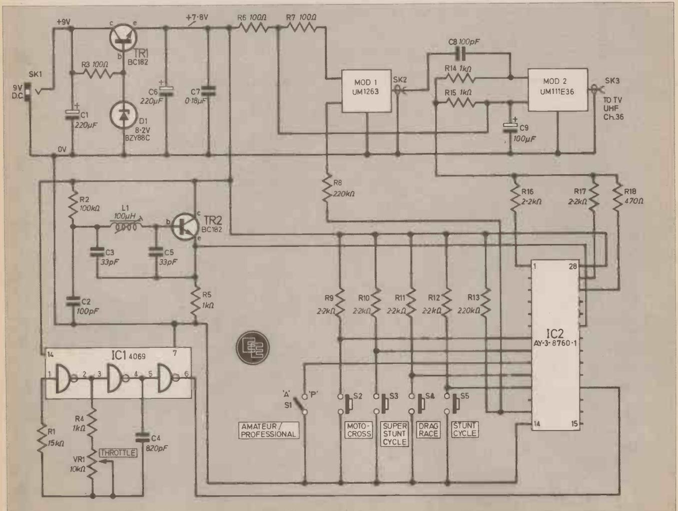
R1, R4, VR1 and C4 to form a square wave oscillator. This is tunable over the range 50-250kHz by VR1, the Throttle Control. The third inverter is a buffer stage and the oscillator output is fed to IC2, pin 18. (The remaining three inverter stages of the 4069 chip are not used).
