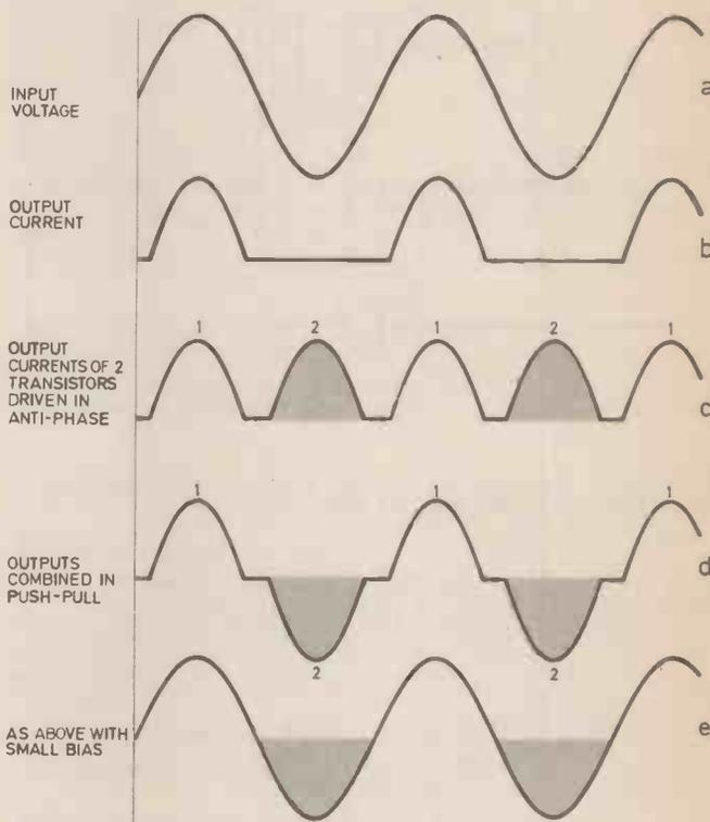
Fig. 8.5. A simple class B amplifier with an input waveform as shown will only produce the positive half cycles as in (b). If two similar transistors are used and their outputs added the waveform in (c) is produced. If however one of the outputs is inverted and added, the waveform shown in (d) will be the result. With a small bias a satisfactory output as in the last curve will be produced.
