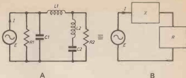
Fig. 8.1a. In this circuit which contains a mixture of resistance, inductance and capacitance, an equivalent circuit can be drawn which will simplify to just one reactance and one resistance as in (b). The cosine of a right angled triangle is represented as in (c).
