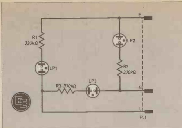
Fig. 4. The complete circuit diagram for the Mains Tester.
