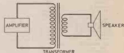
Fig. 2. If a speaker of incorrect impedance is to be used, then a matching transformer is required.
