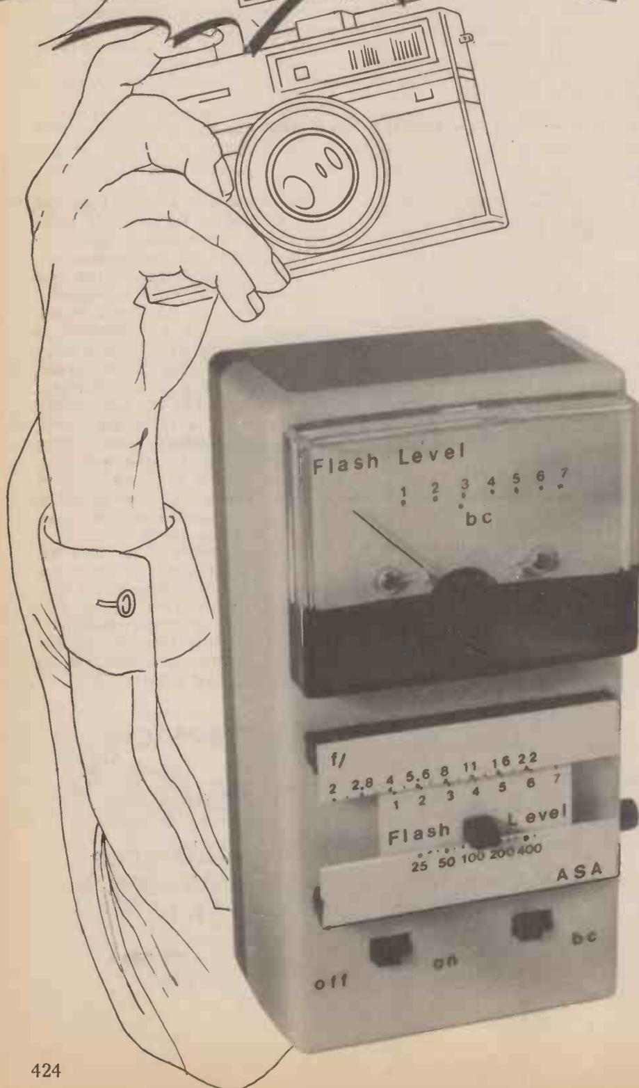
when the photocell receives the light from a flashgun a voltage spike will be produced.
