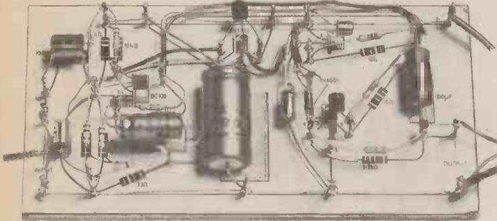
Photograph of the completed POWER AMPLIFIER. Note the screened lead used for the input connection.
