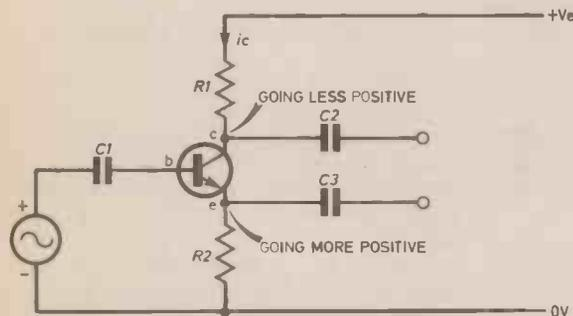
Fig. 8.3. A simple circuit for a phase splitter. If the values of  $R_1$  and  $R_2$  are equal then equal voltages but 180° out of phase will appear at the respective outputs.
