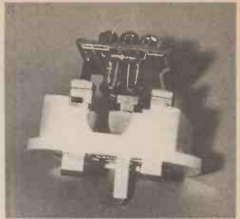
Attaching the circuit board to the plug pins.
