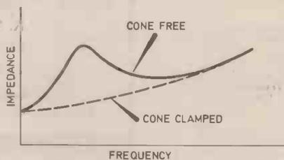
Fig. 1. Illustrating how the impedance can vary with different positions of the speaker cone.
