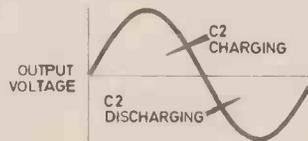
Forgetting for the moment about biasing, the basic circuit Fig. 8.7, has two transistors in series across the power supply. The transistors should be identical in current gain and ratings, but one is npn and the other pnp. The load is connected via a large capacitance C2 which allows free passage to a.c. to the speaker and also charges up to half the supply voltage as shown.
