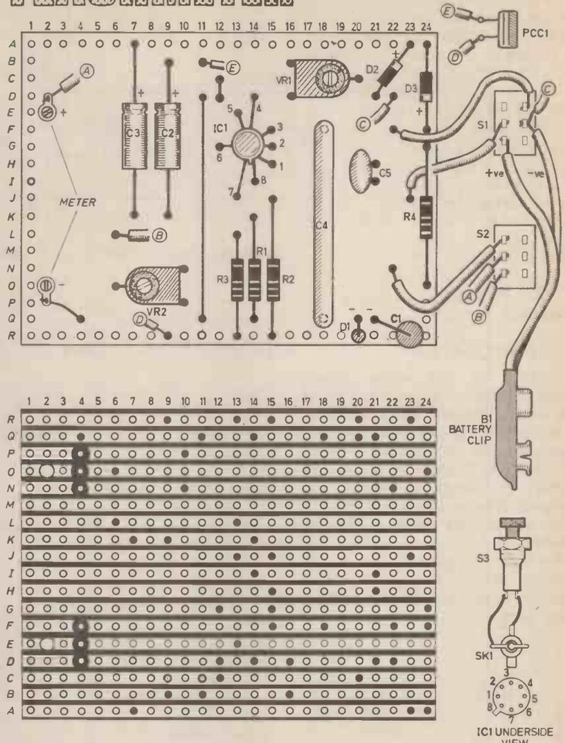
Fig. 3. Wiring details for the unit. Take extra care when soldering the i.c. as a socket cannot be used in this particular layout.
