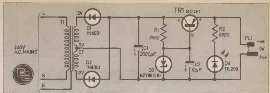
Fig. 2. The complete circuit diagram of the 9V d.c. Power Pack.
