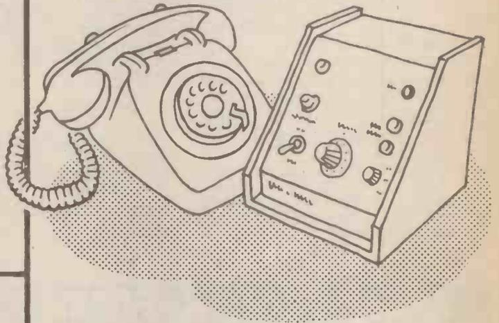
This sound-triggered device will let you know when your telephone is ringing if you are out of range of the in-built telephone bell, when working for example in the garden shed, garage or other remote location. Will find many other uses in and around the home.
