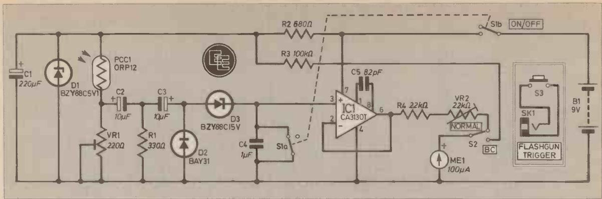
Fig. 2. Complete circuit diagram for the Flashmeter. Socket SK1 (Flashgun Trigger) and switch S3 are used to fire the flashgun.
