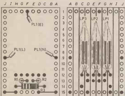
Fig. 2. Layout of components on the stripboard.
