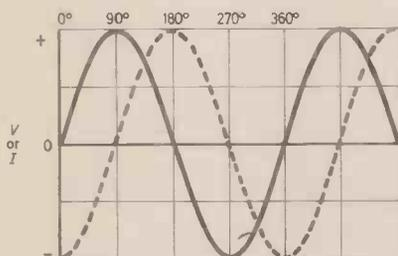
Fig. 8.2. Illustrating phase difference. Here the dotted line lags the wave shown solid by 90 degrees.
