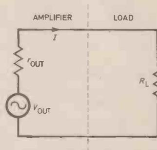
Fig. 8.4. For calculating the output current from an amplifier a simple equivalent circuit as here can be used.
