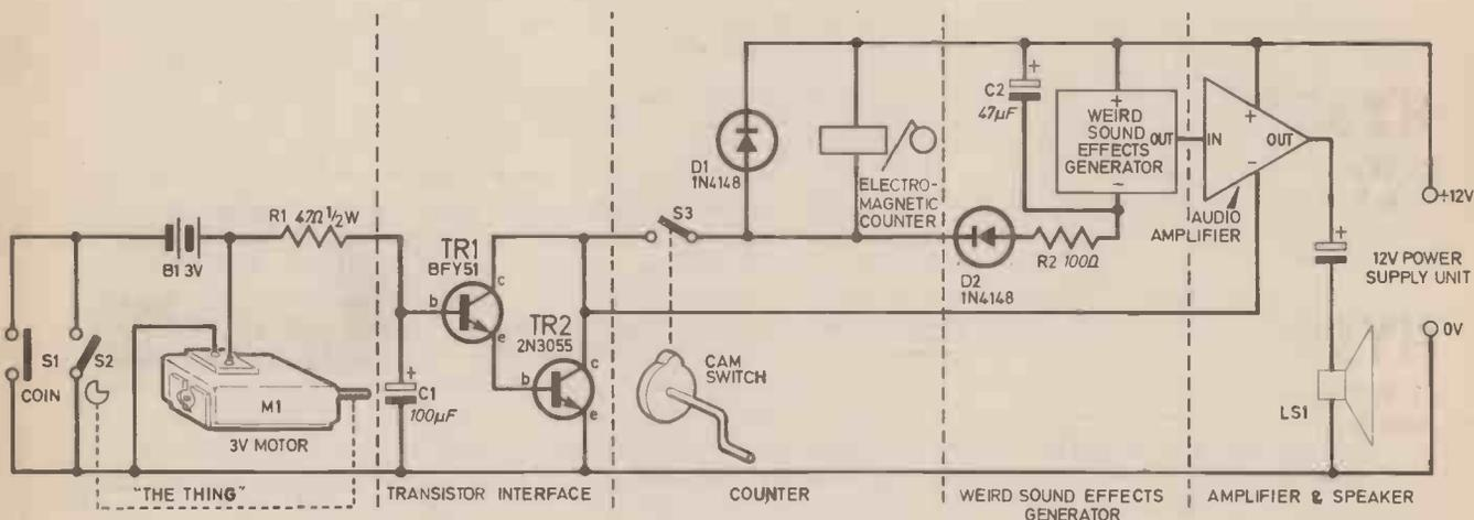
Fig. 4. Final circuit of *The Thing*. In this design all the extras have been included, namely the *Weird Sound Effects Generator*, and an amplifier.
