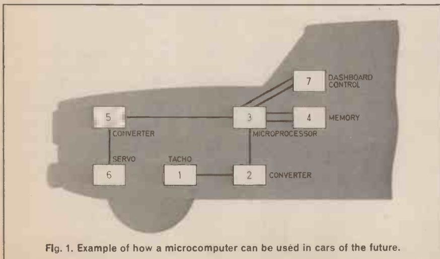
Fig. 1. Example of how a microcomputer can be used in cars of the future.
