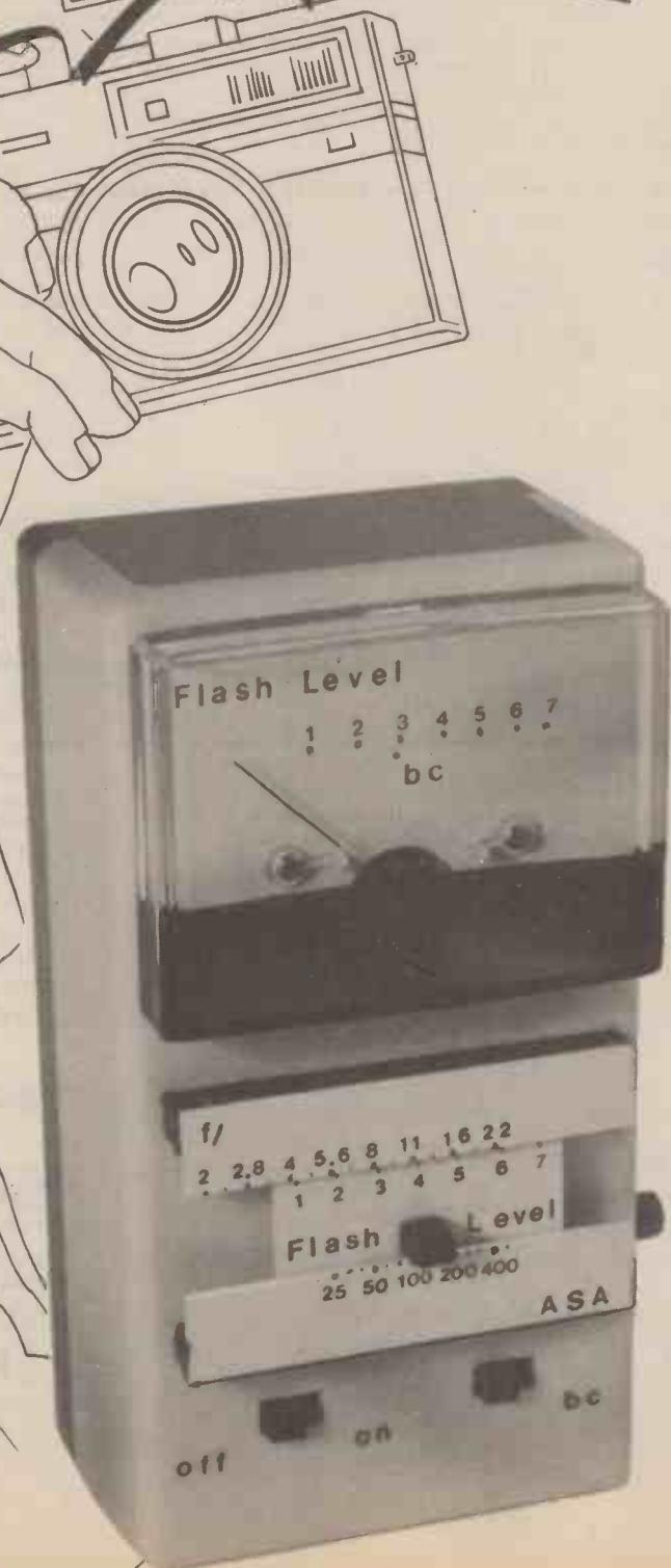
when the photocell receives the light from a flashgun a voltage spike will be produced.
