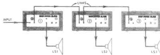
Fig. 1. Using the parallel-wired input sockets to link up three power slaves producing a 300 watt system.
