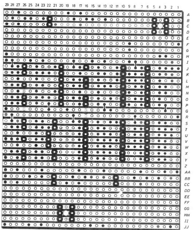
Fig. 4c. The underside of the stripboard showing breaks in the copper tracks and link connections to be made.
