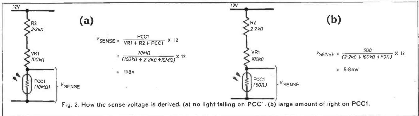
Fig. 2. How the sense voltage is derived. (a) no light falling on PCC1. (b) large amount of light on PCC1.
