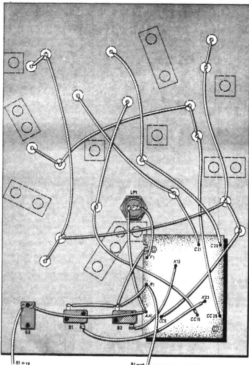
Fig. 7. Underside view of the top panel showing complete wiring details from board to touch-plates and other panel mounted components. Note that the unused drawing pins have insulation tape covering them before the aluminium foil is laid.
