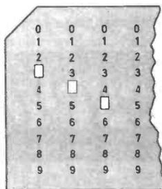
Fig. 10.1. Part of a punched card, showing the holes to register the number 345.
