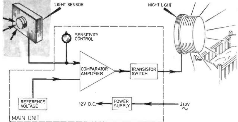
The Light Sensor is a light-dependent resistor (I.d.r.). Together with the Sensitivity Control VR1 it forms a potential divider across the 12V supply. Voltage is tapped off this divider and applied to one input of the Comparator Amplifier.
