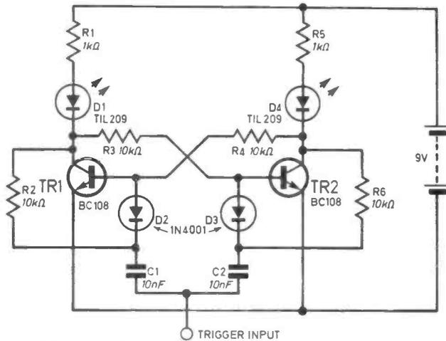
Fig. 10.10. A modified flip-flop circuit can be changed by adding a few extra components to form a "Triggered flip-flop".
