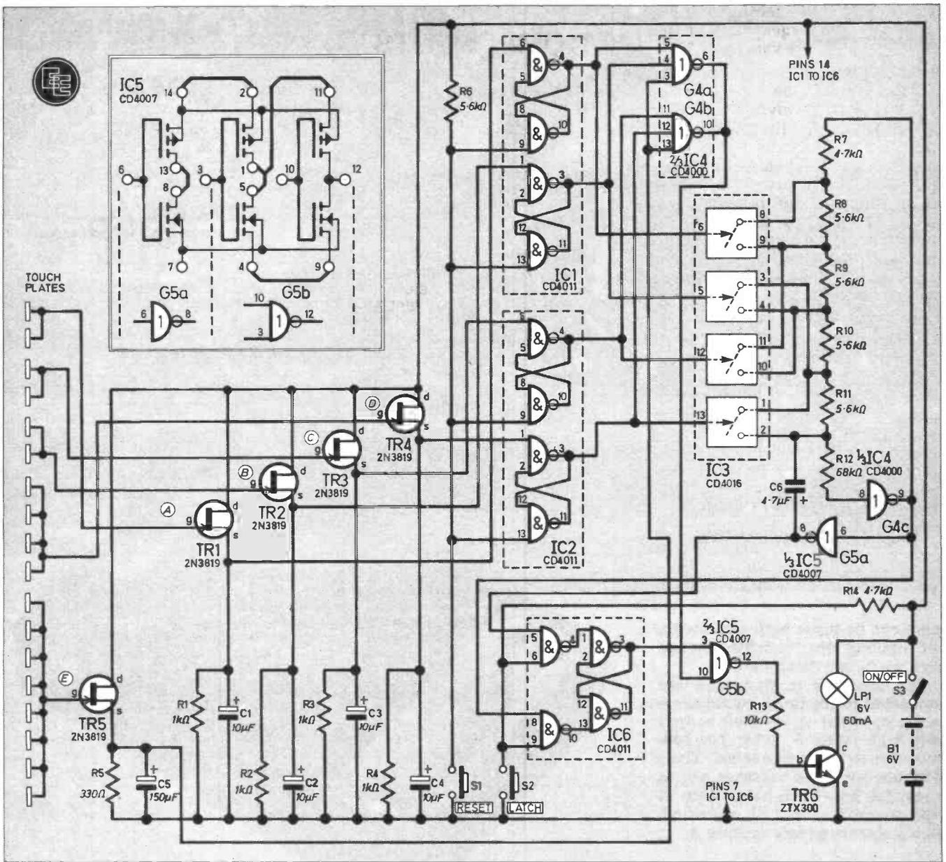
Fig. 1. The complete circuit diagram of the Quagmire game. The inset contains internal details of IC5 and the necessary linking to realise the two gates, G5a and G5b.
