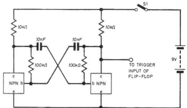
Fig. 10.12. For building a practical circuit using your NPN modules, a slight change is necessary for the circuit to function correctly.
