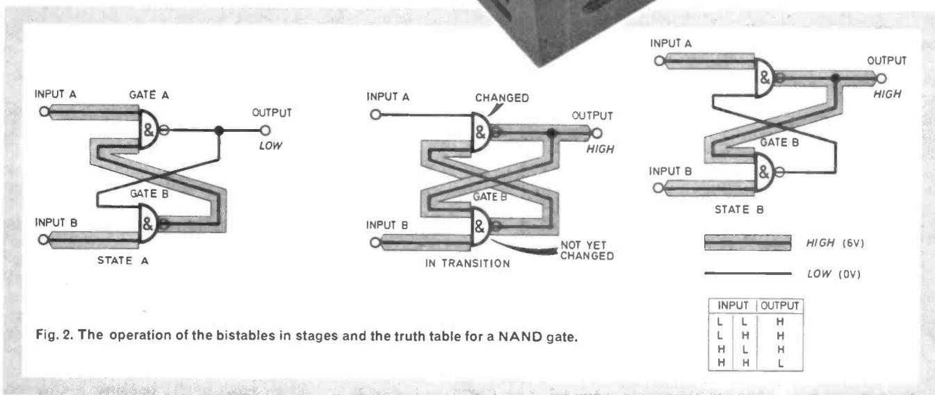
Fig. 2. The operation of the bistables in stages and the truth table for a NAND gate.
