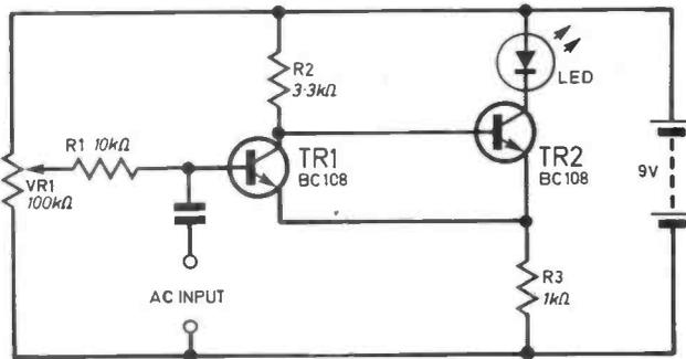
Fig. 10.13. A very popular "building" circuit, the Schmitt trigger. By biasing one transistor hard on, a large a.c. input causes periodic changes of state. The output is a square wave.
