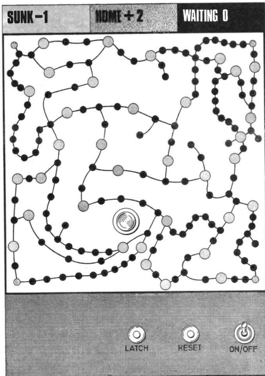
Fig. 5. A plan view of the playing area showing the pathways used on the prototype (half-scale) and the position of the panel mounted switches and lamp.
