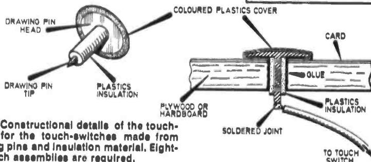
Fig. 6. Constructional details of the touch-plates for the touch-switches made from drawing pins and insulation material. Eighteen such assemblies are required.
