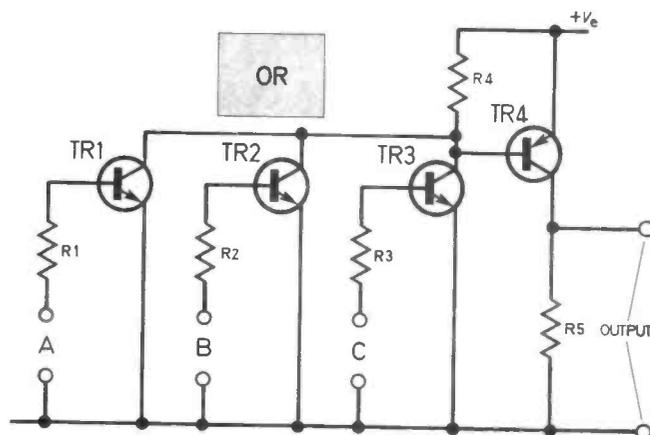
Fig. 10.5. An OR gate. An output results when the inputs A or B or C go positive.
