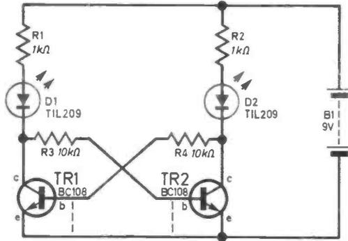
Fig. 10.9. A practical flip-flop circuit can be built using standard components. The action can be proved by shorting the base of each transistor (shown dotted) to earth.
