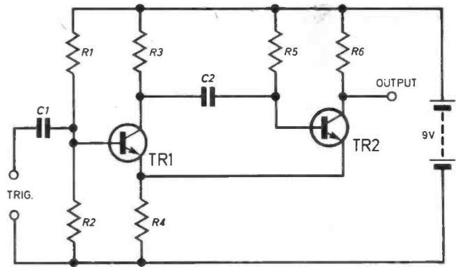
Fig. 10.14. A monostable circuit. When an a.c. input is applied, pulses of fixed duration are produced.
