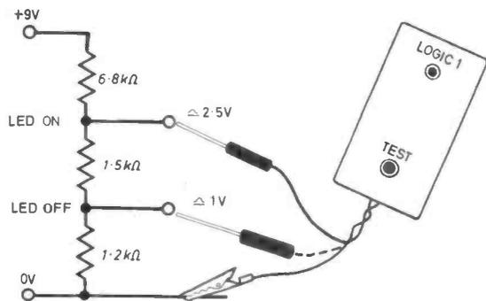
Fig. 4. Testing the Logic Probe using a potential divider to define the two logic levels. In this test we are only concerned with the "high" logic function of the Probe.
