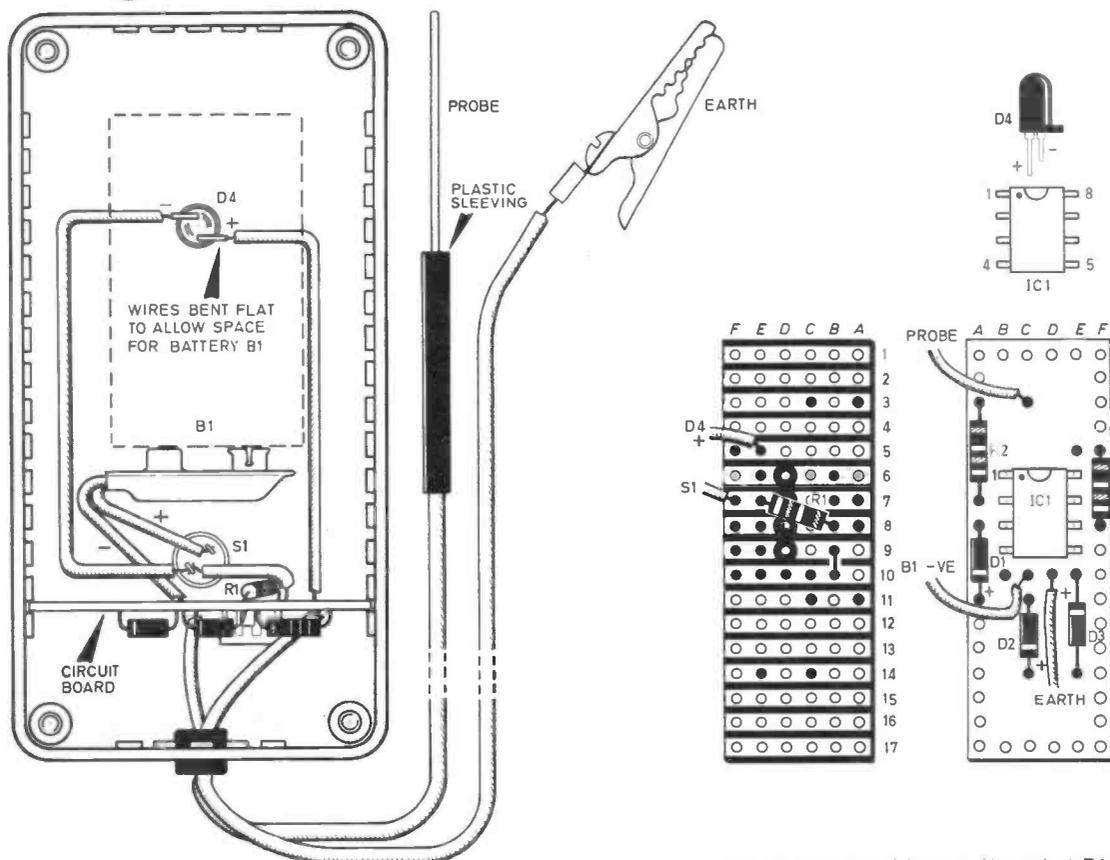
Fig. 2. Remainder of the wiring and construction of the probe. It is advisable to place a small piece of sticky tape over the wires of D4.
