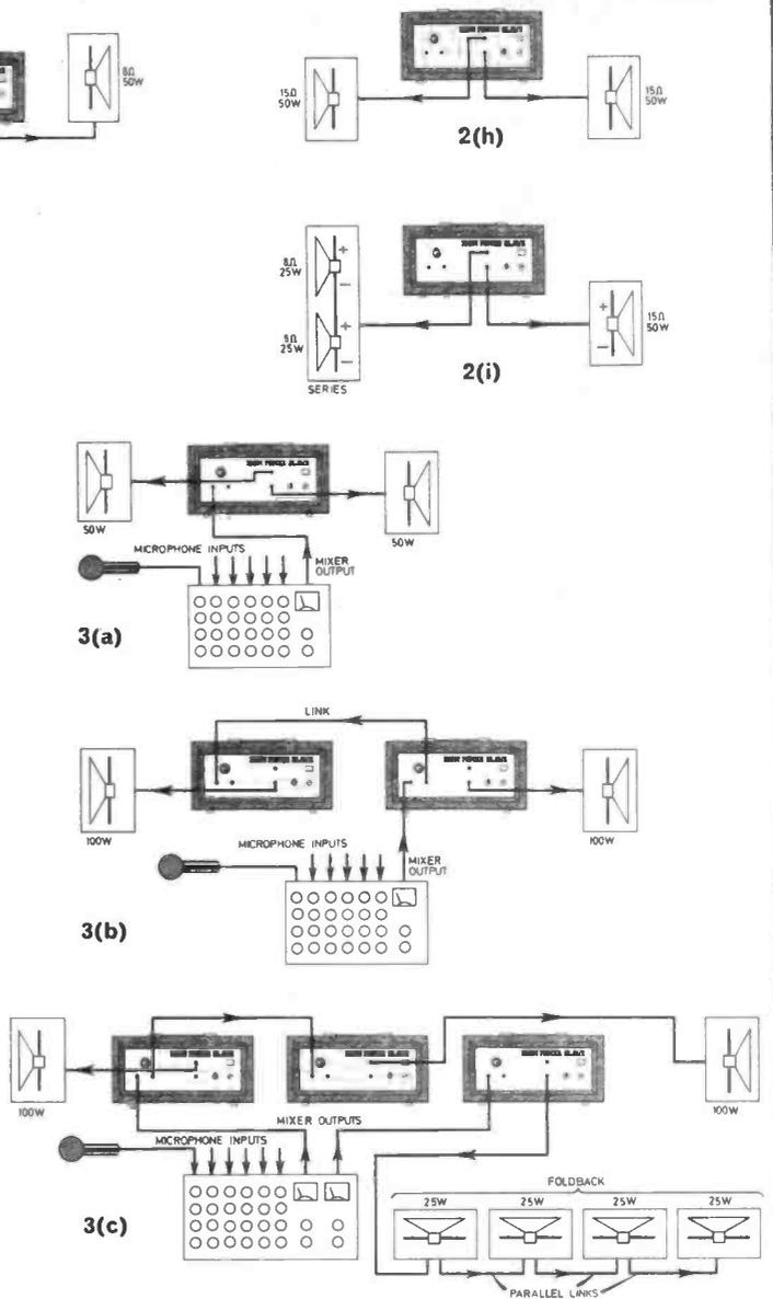
**Fig. 3.** Use of the power slaves in a pop group PA system incorporating a multichannel mixer; (a) 100 watt, (b) 200 watt, (c) 200 watt main channel with 100 watt foldback system.
