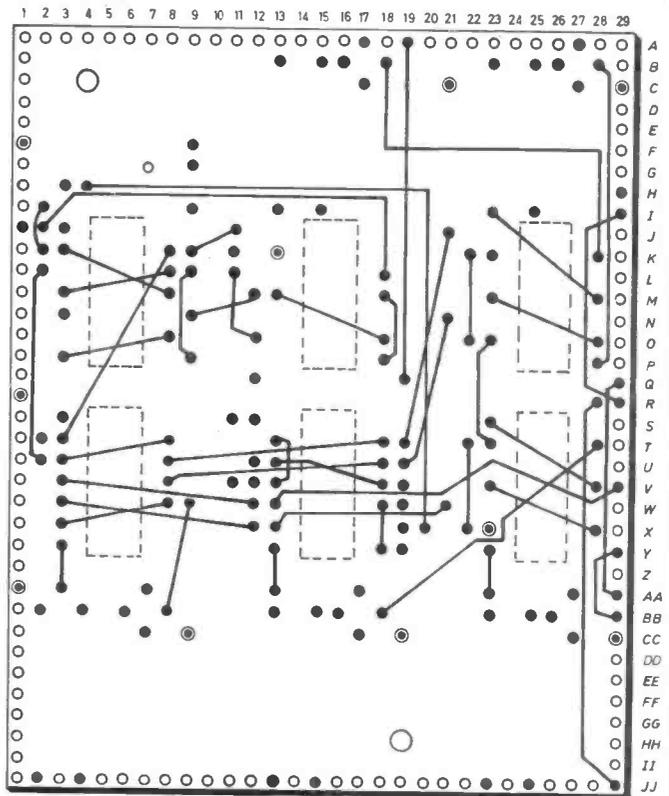
Fig. 4b. The circuitry to be carried out on the topside of the stripboard after components have been positioned and according to instructions.
