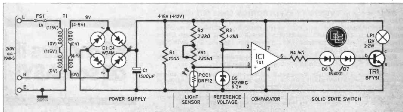
the inverting input, then the output swings high, almost to the voltage of the supply rail.
