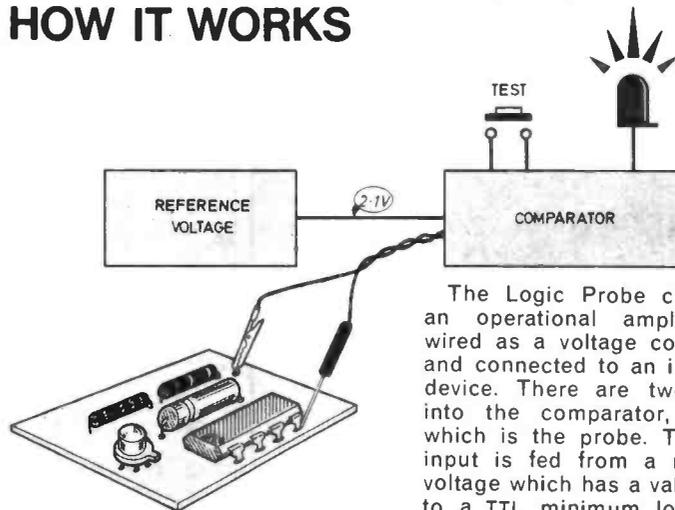
The Logic Probe comprises an operational amplifier i.c. wired as a voltage comparator and connected to an indicating device. There are two inputs into the comparator, one of which is the probe. The other input is fed from a reference voltage which has a value equal to a TTL minimum logic level "1". This voltage is about 2.1V.
