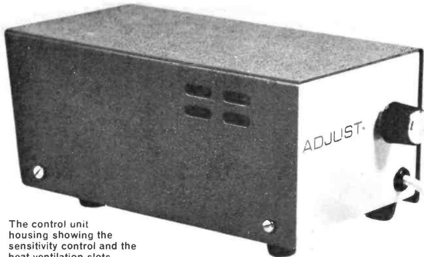
The control unit housing showing the sensitivity control and the heat ventilation slots.
