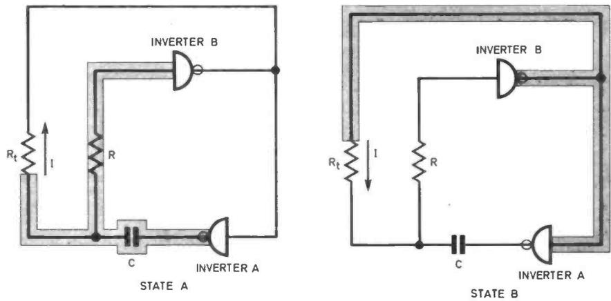
Fig. 3. The operation of the oscillator circuit composed of two CMOS inverter gates.
