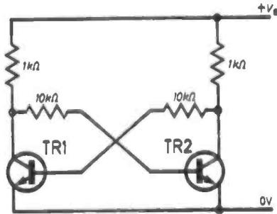
Fig. 10.8. The flip-flop is normally seen in most text books as above. The symmetry is clearly seen.
