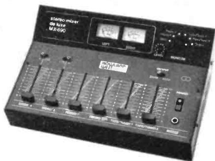
A mini stereo mixer, the Howland West MX690 with facilities for two microphones, two record deck cartridges and two tape tuners.
