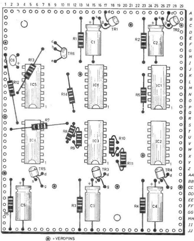
Fig. 4a. The layout of the components on the topside of the stripboard. Orientate the i.c.s. with reference to the indentation at one end.
