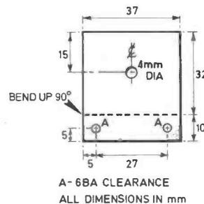
Fig. 4. Bracket required for mounting C2. Material used in the prototype was 18 s.w.g. aluminium.
