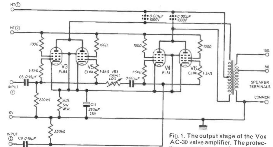
Fig. 1. The output stage of the Vox AC-30 valve amplifier. The protection capacitors are shown dotted.
