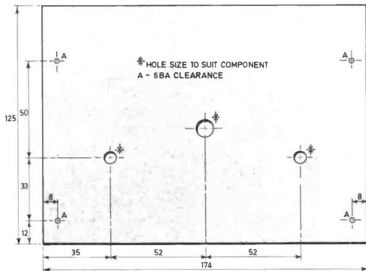
Fig. 3. Drilling arrangement for the front panel. The position of the centre hole (for C3) depends on the actual component used, hence no vertical measurement has been given.
