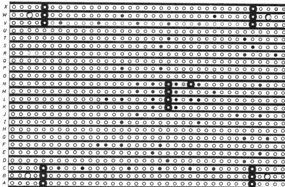
Fig. 3. The component board. Breaks in the copper strips must be made before components are mounted on the other (plain) side of the 0.1 in matrix stripboard. Note that the TR1 heatsink must be fitted before this component is soldered in position.
