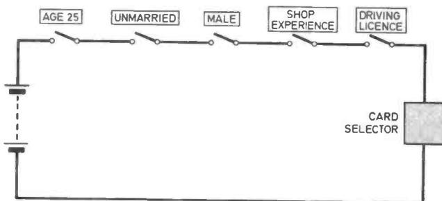
Fig. 10.2. Switch contacts are arranged as shown to select a candidate with all the necessary qualifications. This arrangement represents the AND function.
