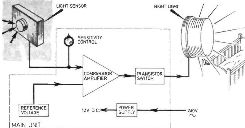
The Light Sensor is a light-dependent resistor (l.d.r.). Together with the Sensitivity Control VR1 it forms a potential divider across the 12V supply. Voltage is tapped off this divider and applied to one input of the Comparator Amplifier.
