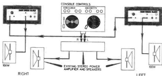
Fig. 5. Increasing the output power of a stereo disco set-up by 200 watts—100 watts per channel. All the necessary equalisation will have been taken care of in the console pre-amplifier.
