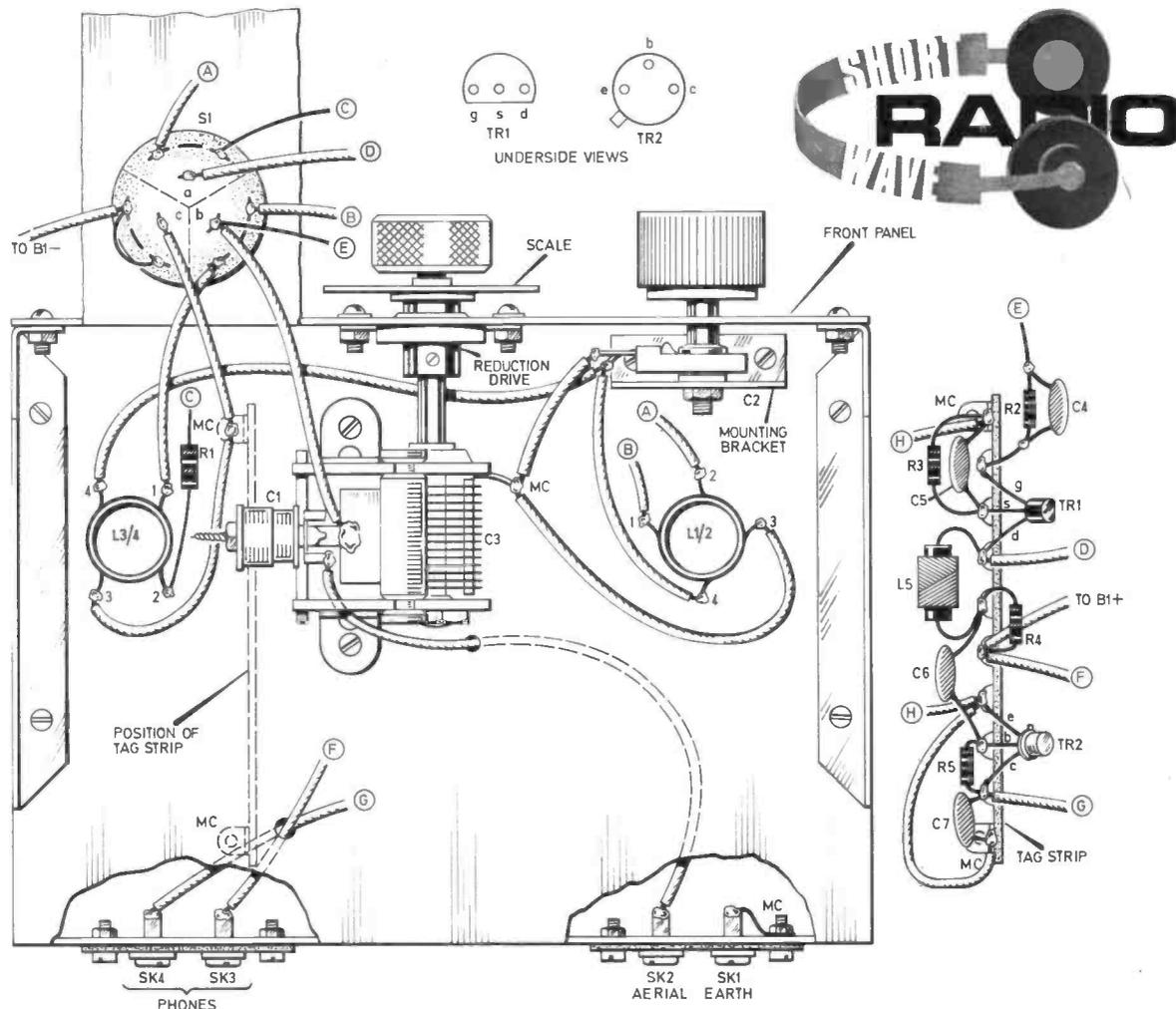
Fig. 2. Complete wiring for the radio. Note that for clarity the front panel has been "opened out" to show the connections to S1. The position of the tag strip is shown dotted, the wiring of which is shown to the right. MC denotes a connection to the chassis.
