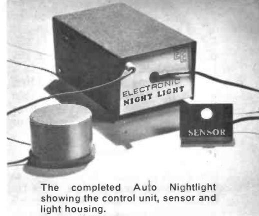
The completed Auto Nightlight showing the control unit, sensor and light housing.
