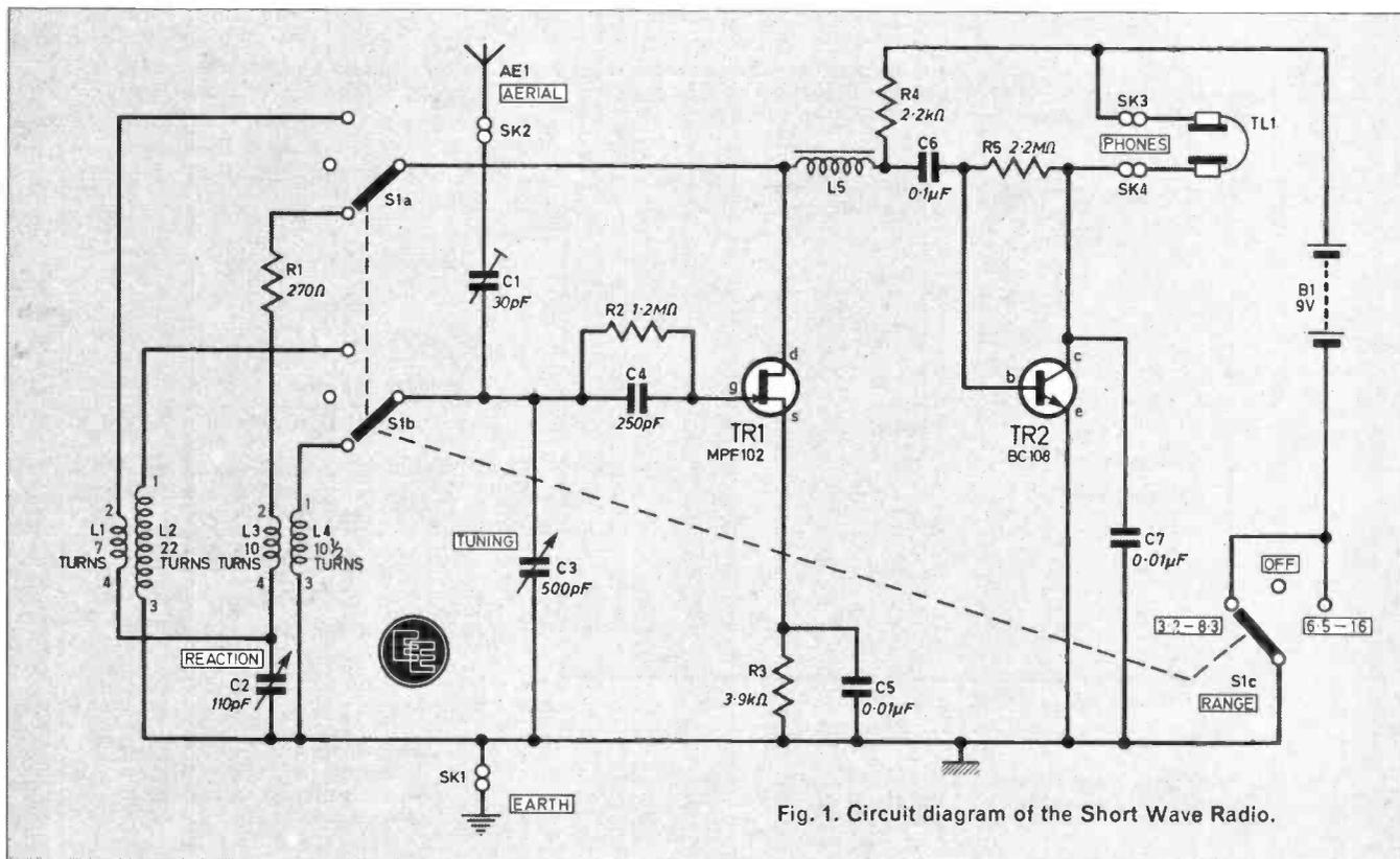
Fig. 1. Circuit diagram of the Short Wave Radio.
