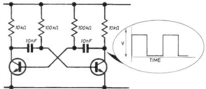
Fig. 10.11. By "cross coupling" the two transistors the basic flip-flop circuit can be changed into a multivibrator.
