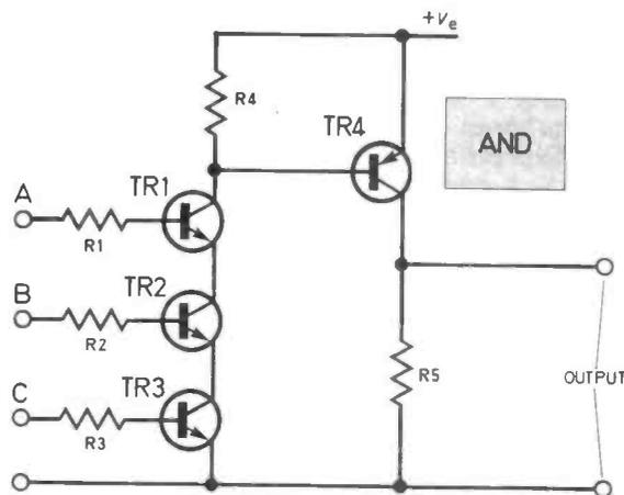
Fig. 10.4. An example of an AND gate. An output is only given when the inputs A and B and C are positive.
