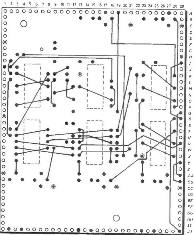
Fig. 4b. The circuitry to be carried out on the topside of the stripboard after components have been positioned and according to instructions.
