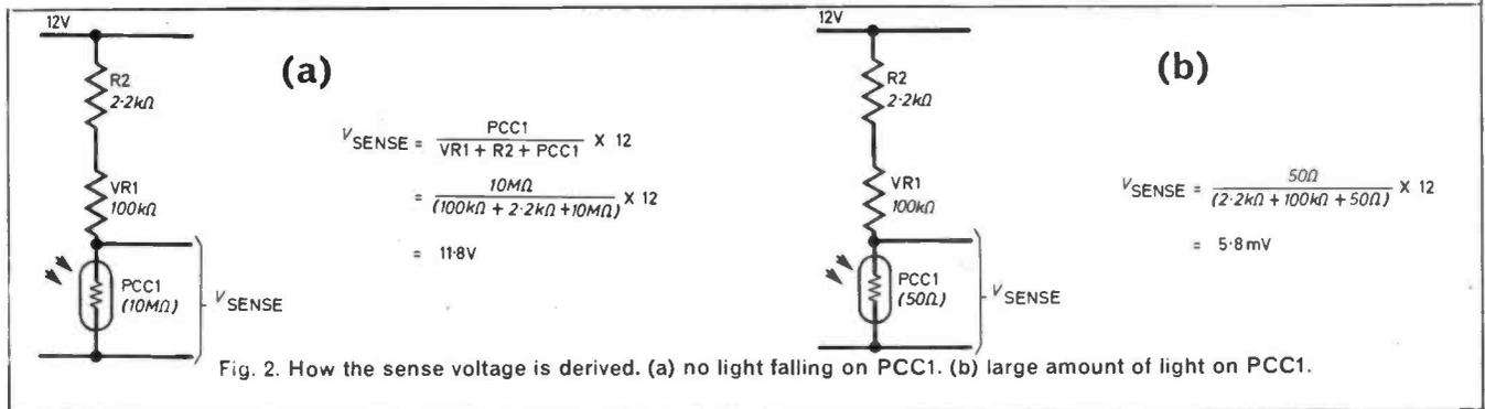
light being received by PCC1, an ORP12 light-dependent resistor—the "electric eye" of the system.
