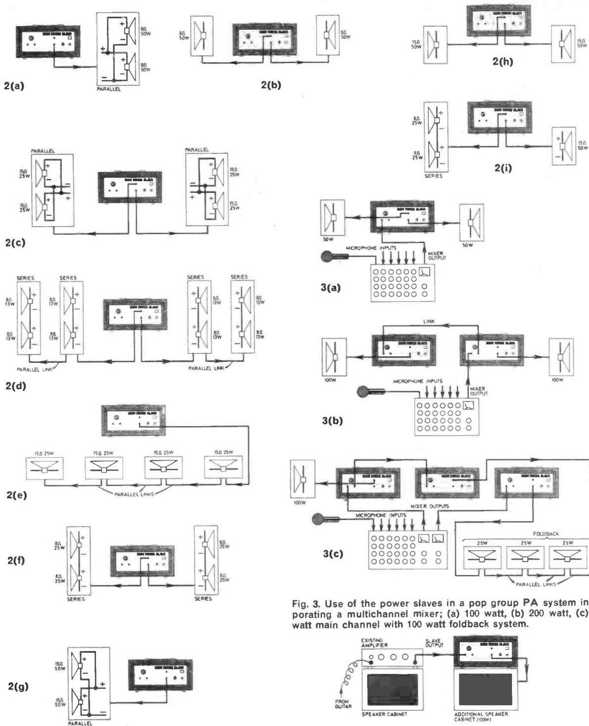
**Fig. 2.** Arrangements of 8 ohm and 15 ohm loud-speaker drive units to produce suitable systems for the two versions of the power slave; (a) to (e) are suitable for the 4 ohm version and (f) to (l) are suitable for the 8 ohm version. The total load as seen by the slave amplifier in each of these arrangements is: (a) 4 ohms, (b) 4 ohms, (c) 3.75 ohms, (d) 4 ohms, (e) 3.75 ohms, (f) 8 ohms, (g) 7.5 ohms, (h) 7.5 ohms, (i) 7.7 ohms.
