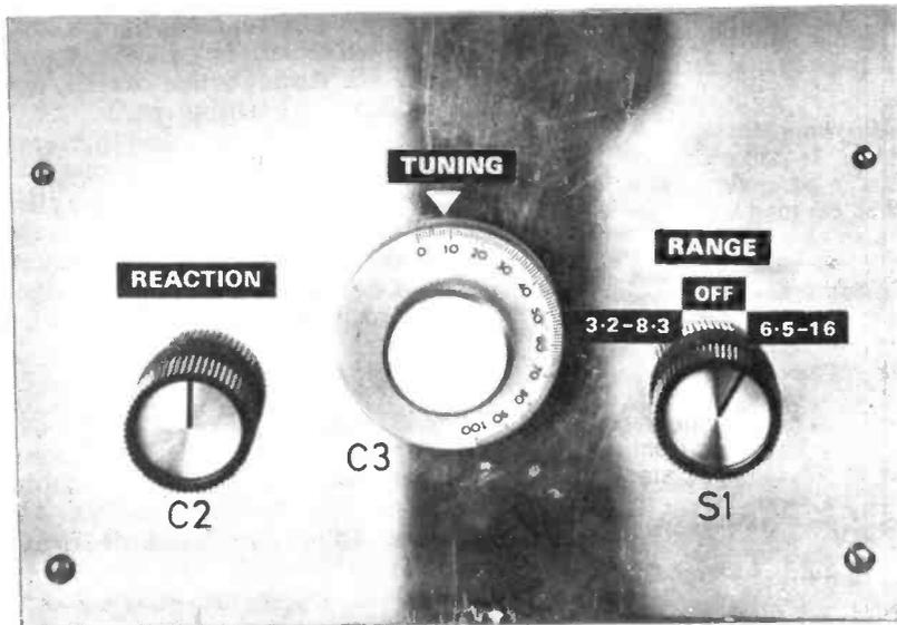
Front panel layout for the Shortwave Radio showing the reaction and tuning controls and the range selector switch.
