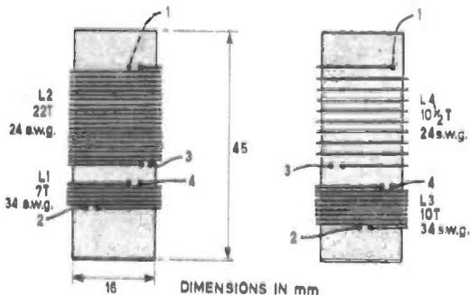
Fig. 5. Winding details for the two sets of coils. The completed coils are mounted on the chassis using small sections from a wooden dowel forced into the base of each coil and glued. The coil is then mounted vertically on the chassis using short wood screws.
