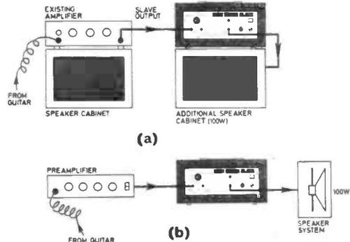
**Fig. 4 (a).** Increasing the output power capability for an electronic instrument (or PA) via the slave output socket on the existing equipment and (b) forming the amplification equipment for Instrument with a suitable pre-amplifier.
