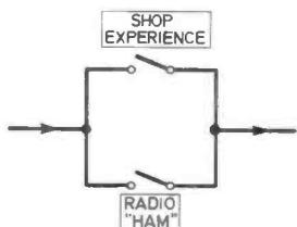
Fig. 10.3. In this arrangement the switches select a candidate who has either of two alternatives. This represents the OR function.
