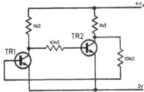
Fig. 10.7. A flip-flop circuit, drawn to show the d.c. feedback arrangement.
