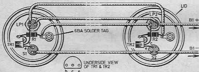
Fig. 2. Wiring details for the two units. All components are mounted on the lids, and wired direct. The length of connecting cable between the units is a matter of choice, but one metre, seems reasonable.
