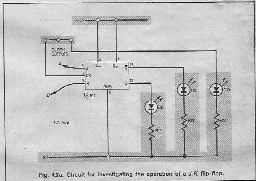
Fig. 4.2a. Circuit for investigating the operation of a J-K flip-flop.
