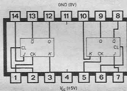
Fig. 4.1. Pinning details for the 7473 dual J-K flip-flop integrated circuit. Note that power supply pins are at pin 4 and pin 11.
