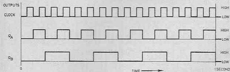
Fig. 4.4. Output sequence of the series flip-flop and the clock of Fig. 4.3a.
