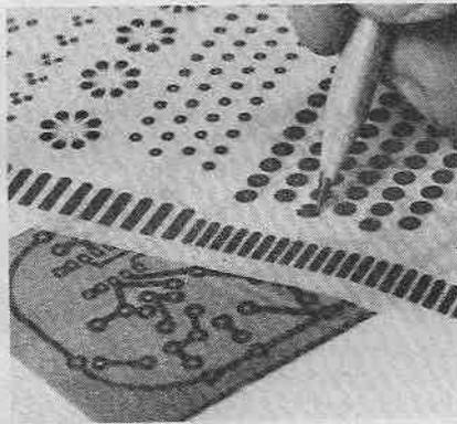
(h) Rubbing the transfers directly onto the copper.
