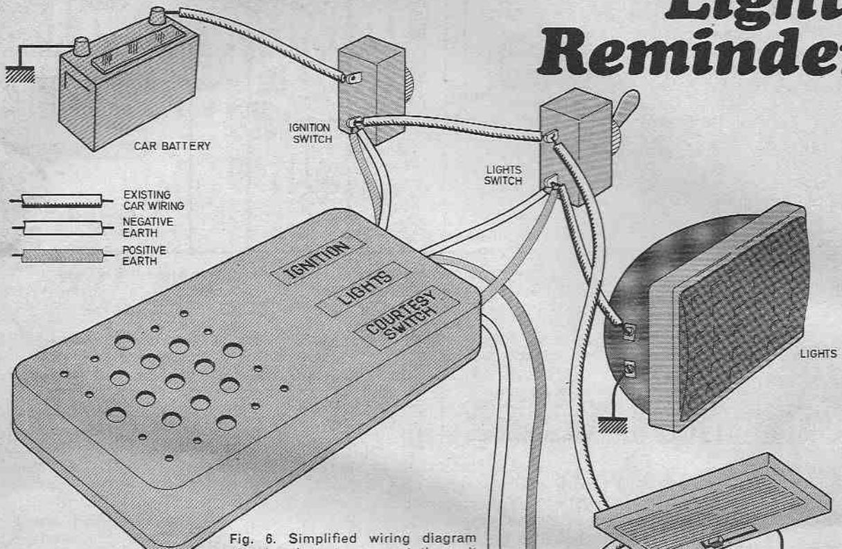
Fig. 6. Simplified wiring diagram showing how to connect the unit into the car electrical system.
