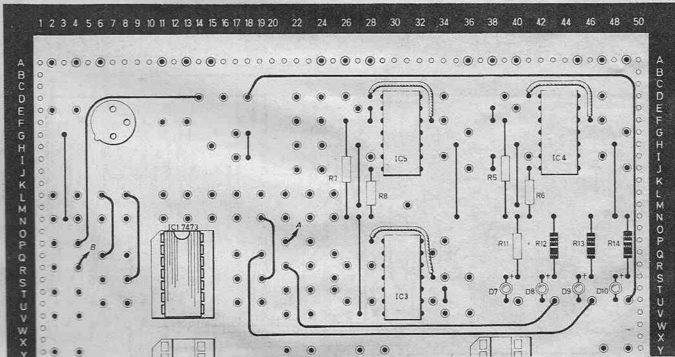
Fig. 4.3b. The circuit of Fig. 4.3a wired on the Test-Bed.
