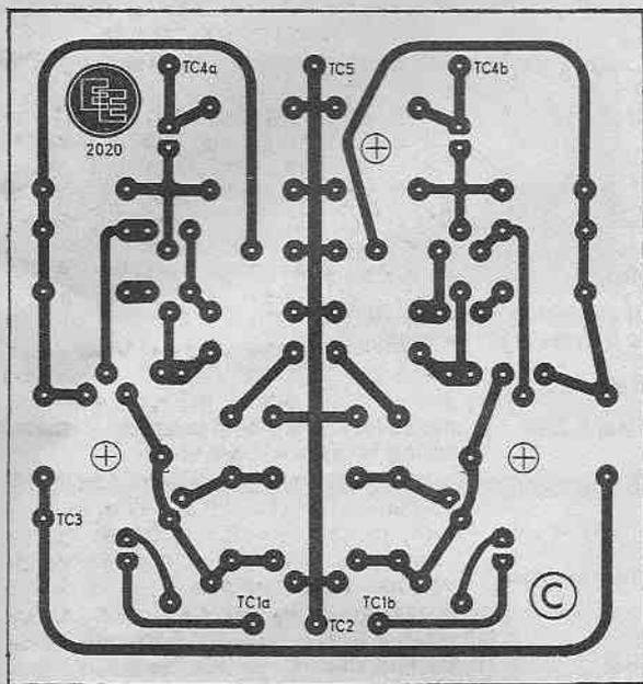
Fig. 2-3. Board C of the 2020 Tuner Amplifier: underside view showing printed circuit (full size).
