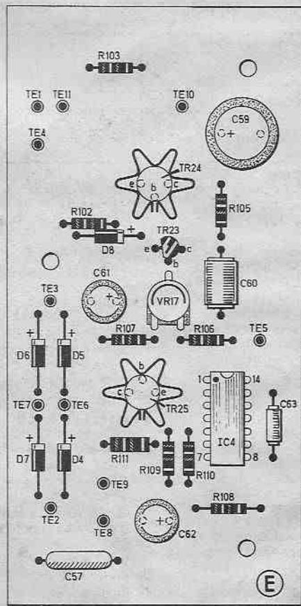
Fig. 2-6. Board E of the 2020 Tuner Amplifier: top view showing components in position.
