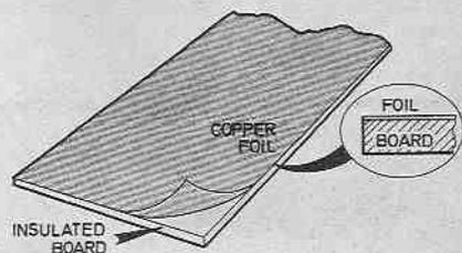
Fig. 1. Printed circuit board consists of a copper foil bonded to an insulating material.
