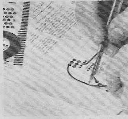
(n) Laying tape for interconnecting the pads on a tracing paper master.
