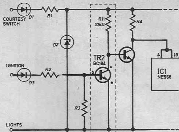
Fig. 3. The original circuit is modified slightly to enable it to operate on positive earth car systems.
