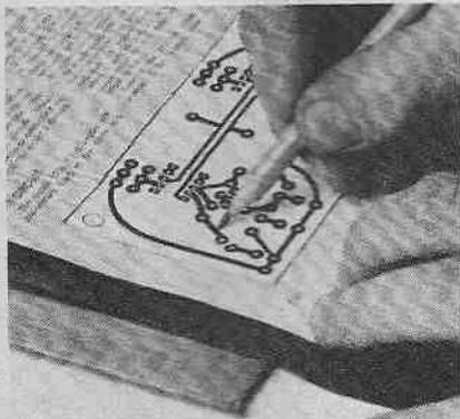
(d) Tracing the copper pattern directly onto the copper side of the board.
