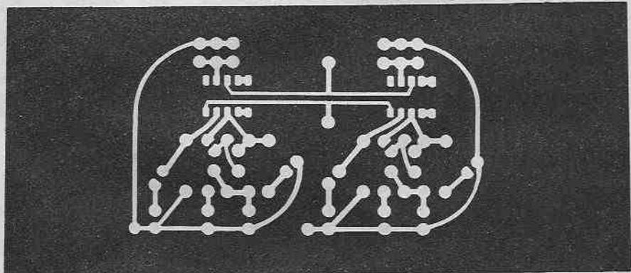
(k) A stencil made for the copper pattern appearing in Fig. 3.
