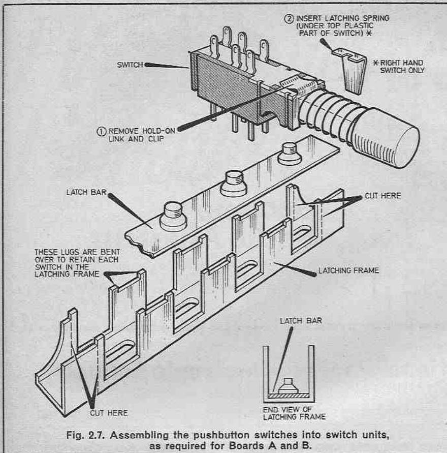
the clips and links to be removed without damage to the switches. The clips and links can then be discarded.
