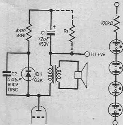
Fig. 2. In this circuit a diode is used to re-route the inductive surges. Using series neons the protection circuit can to some extent be regulated.
