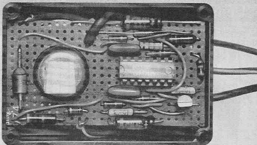
The completed circuit board for the Lights Reminder mounted in a suitable case.
