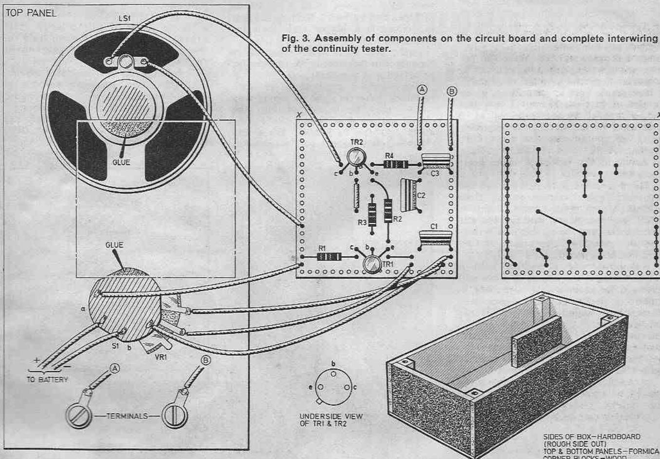
Fig. 3. Assembly of components on the circuit board and complete interwiring of the continuity tester.
