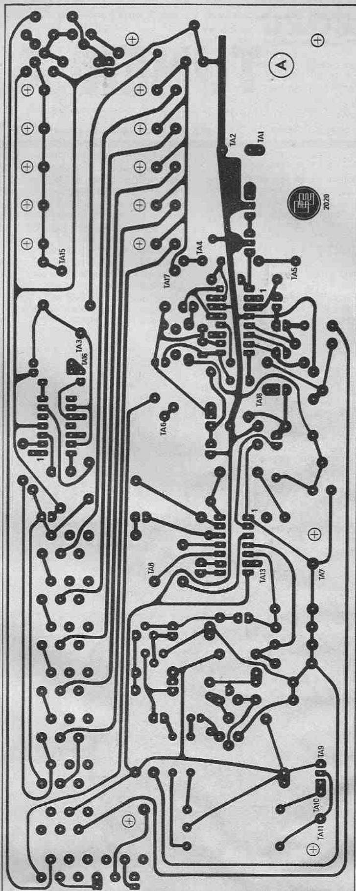
Fig. 2.1. Board A of the 2020 Tuner Amplifier: underside view showing printed circuit (full size).
