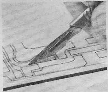
(c) Cutting around the self-adhesive pattern glued to the copper side.
