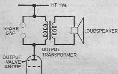
Fig. 1. Using spark gap protection on a simple output stage.
