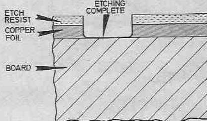
Fig. 2. The exposed copper areas will be etched away.
