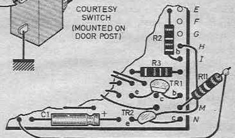
Fig. 4. (Left). Stripboard layout showing the breaks to be made on the underside and the topside wiring.
