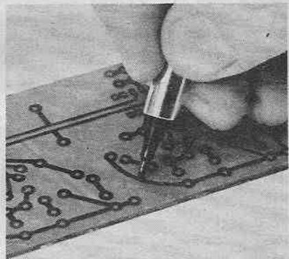
(i) Interconnections between the pads being made with resist pen.
