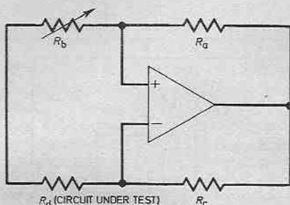
Fig. 1. General principle. Positive feedback set by  $R_a$  and  $R_b$  is offset by negative feedback via  $R_c$  and  $R_d$ .
