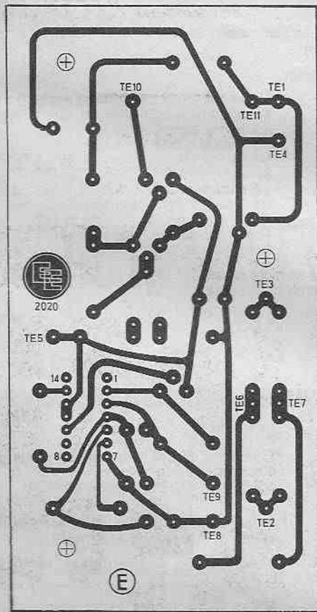
Fig. 2-5. Board E of the 2020 Tuner Amplifier: underside view showing printed circuit (full size).
