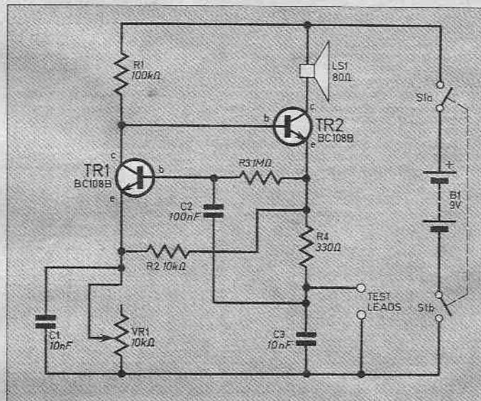
Fig. 2. The circuit of the continuity tester.
