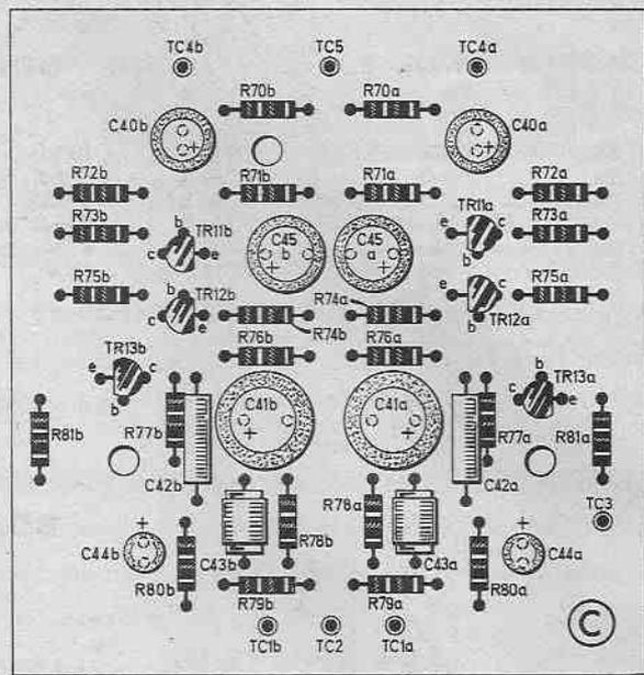
Fig. 2-4. Board C of the 2020 Tuner Amplifier: top view showing components in position.
