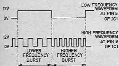
Fig. 2. Typical waveforms appearing at the outputs of the two oscillators.
