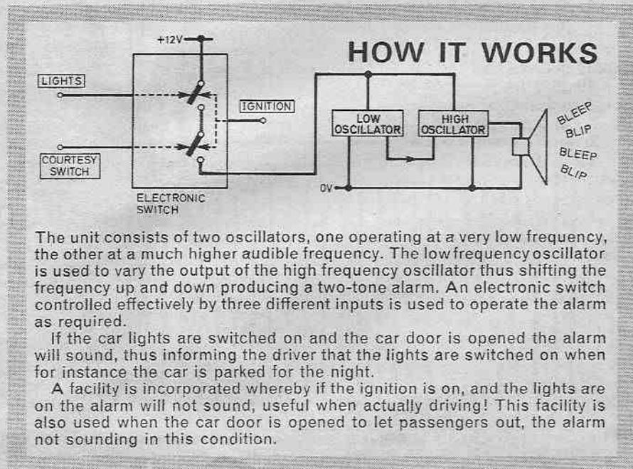
The unit consists of two oscillators, one operating at a very low frequency, the other at a much higher audible frequency. The low frequency oscillator is used to vary the output of the high frequency oscillator thus shifting the frequency up and down producing a two-tone alarm. An electronic switch controlled effectively by three different inputs is used to operate the alarm as required.
