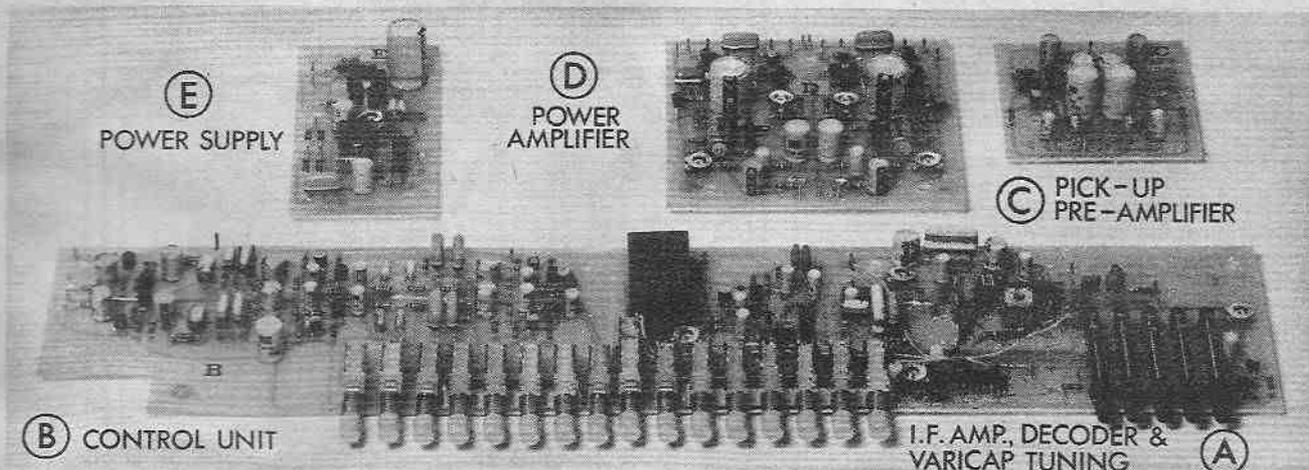
The five circuit boards of the 2020 Tuner Amplifier arranged in their relative chassis positions.
