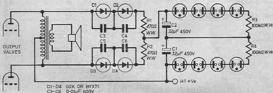
Fig. 3. Applying the protection methods just discussed to the VOX AC30 amplifier.
