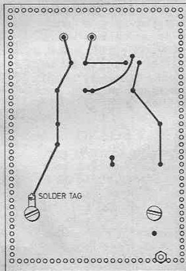
Fig. 2. The layout of the components on the main circuit board, showing inter-track links and breaks to be made on the underside.
