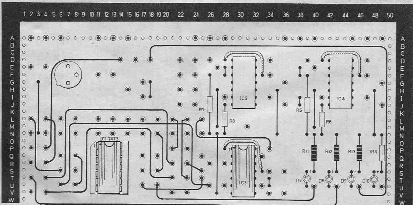
Fig. 4.5b. The circuit of Fig. 4.4a wired up on the Test-Bed.
