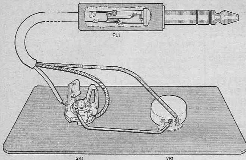
Fig. 3. Layout of the components on the back of the front panel of the case and interwiring.
