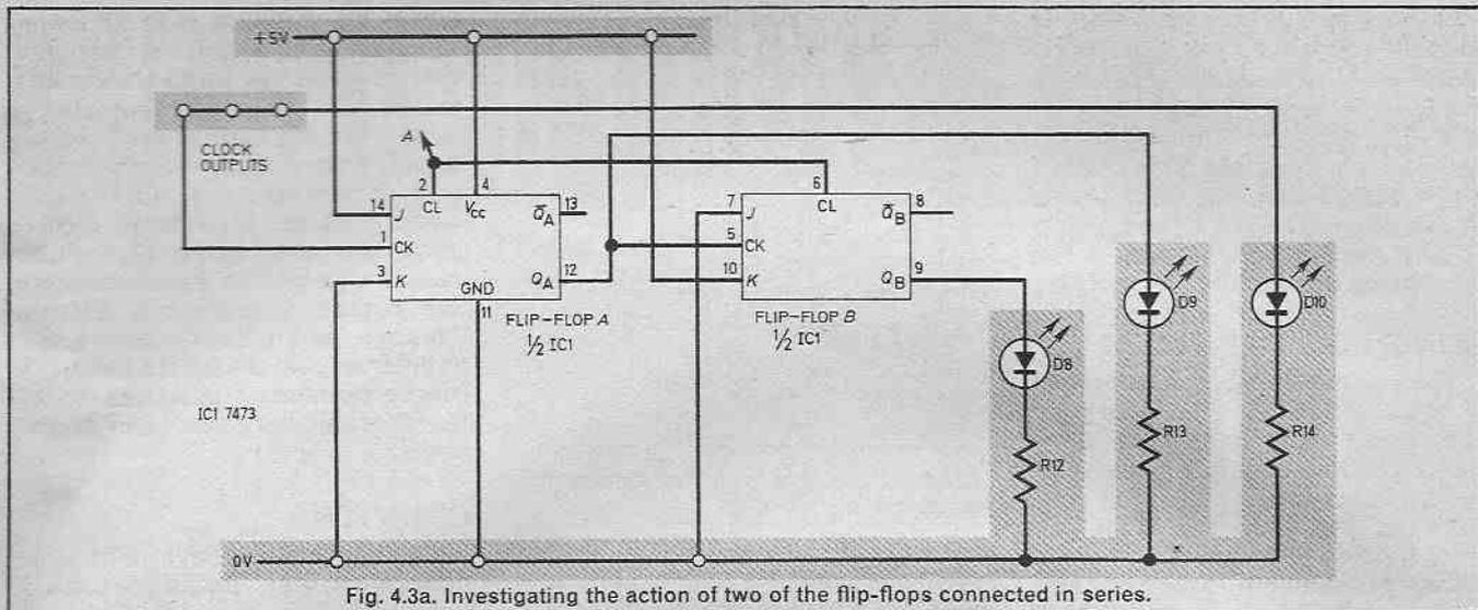
Fig. 4.3a. Investigating the action of two of the flip-flops connected in series.
