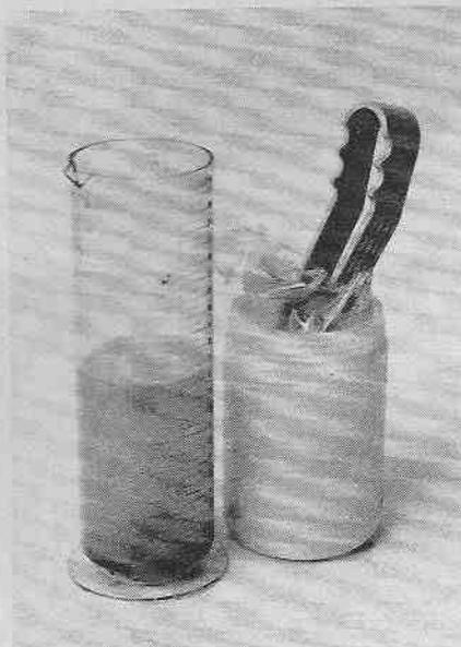
(g) Making up a solution of ferric chloride in a measuring cylinder.
