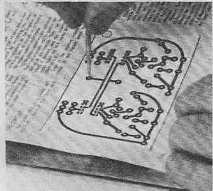
(f) Pricking through the pad centre points onto the copper board.
