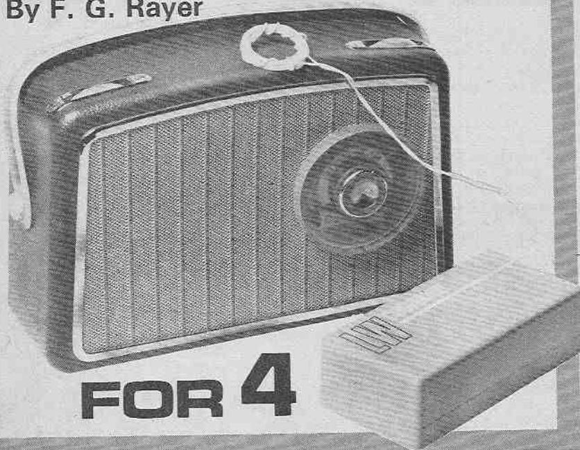
If you have a radio in use which does not include long waves, you cannot receive Radio 4 on 200kHz or 1500 metres with it. The single transistor convertor described here overcomes this.
