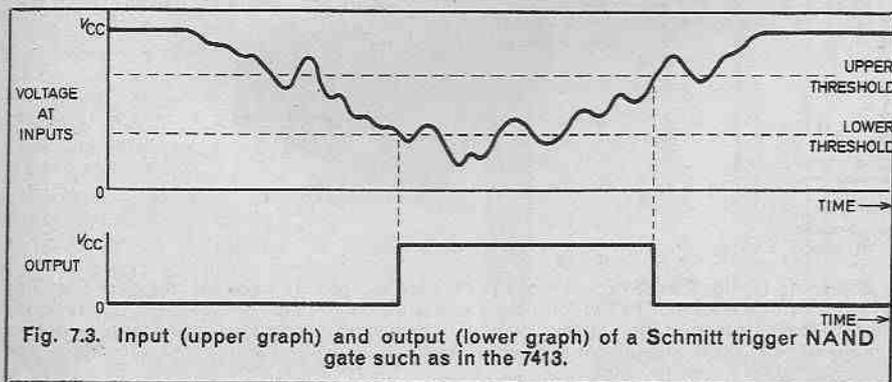
Fig. 7.3. Input (upper graph) and output (lower graph) of a Schmitt trigger NAND gate such as in the 7413.
