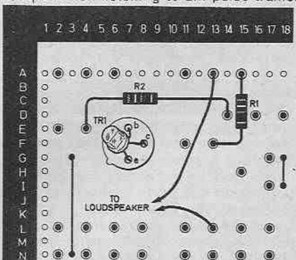
Fig. 7.5 (b). The circuit of Fig. 7.5 (a) wired up on the Test-Bed.
