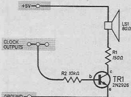
Fig. 7.5 (a). Circuit diagram of a Loudspeaker Module for increasing volume output when listening to a.f. pulse trains.
