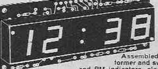
Assembled and pre-tested, just add transformer and switches. Features include alarm and PM indicators, sleep, snooze timers and variable brightness.
