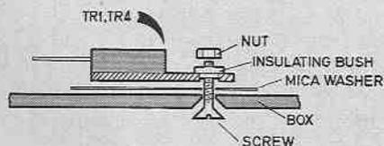
Fig. 4. Power transistor mounting details.
