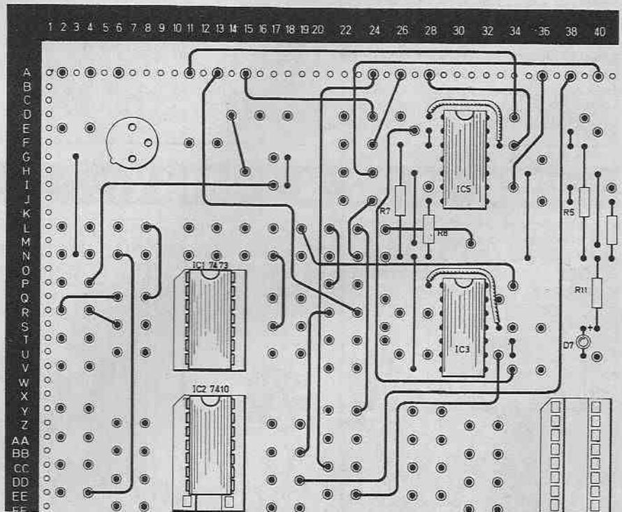
Fig. 7.8 (b). The circuit of Fig. 7.8 (a) wired up on the Test-Bed.
