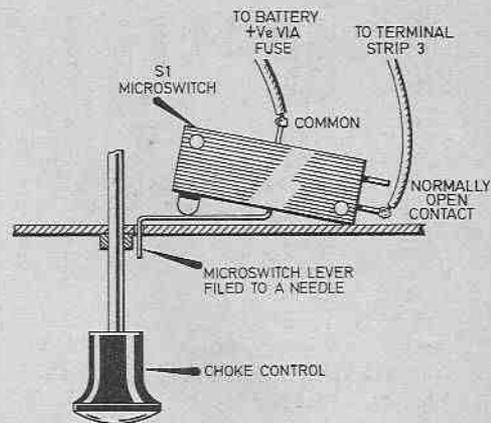
Fig. 2. One method of mounting the micro-switch.
