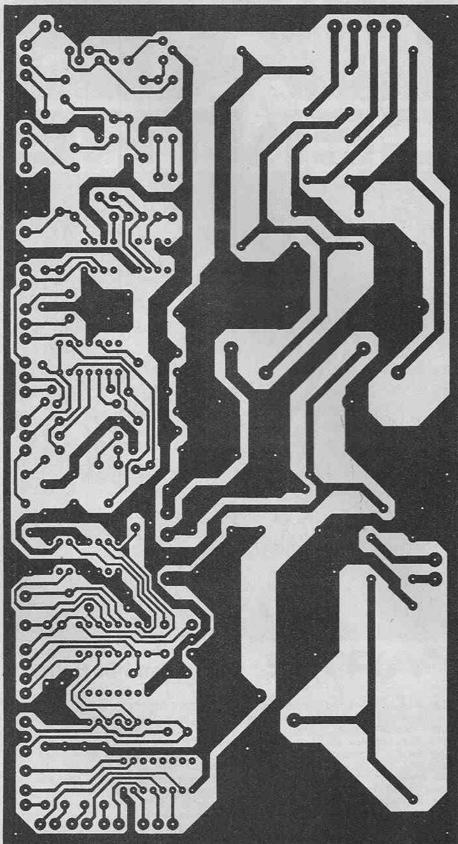
Fig. 2.1. The full-size master of the printed circuit pattern viewed from the copper side of the board. The black regions are the areas of copper to remain after etching.
