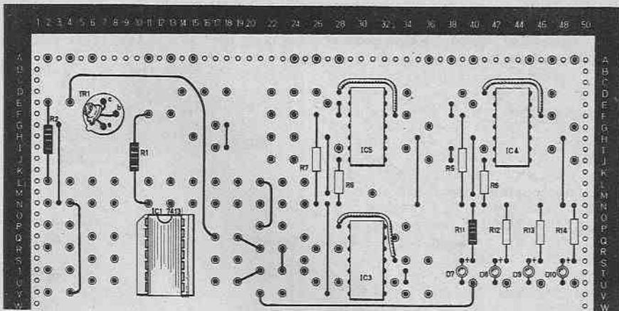
Fig. 7.10 (b). The circuitry of Fig. 7.10 (a) wired up on the Test-Bed.
