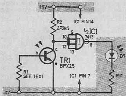
Fig. 7.10 (a). The circuit of a High Speed Light Sensor using a phototransistor which can respond rapidly to light intensity variations.
