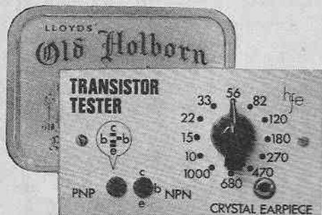
THE MAJORITY of simple transistor testers are very sensitive to variations in battery voltage. For example, a tester designed to operate from 9V will usually read low by at least 33 per cent if the battery voltage falls to 6V. Some testers require individual calibration. Some use expensive meters.
