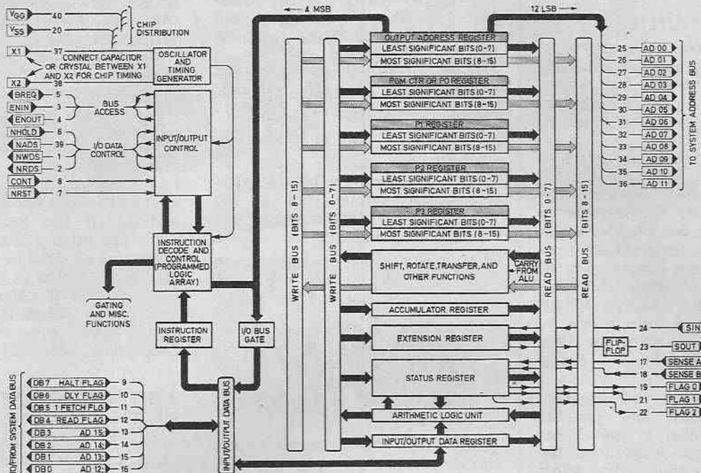
Fig. 2.3. Block diagram of the National SC/MP microprocessor.
