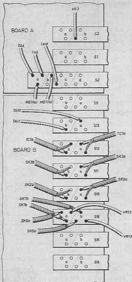
Fig. 5.5. Pushbutton switches: wiring details. Observe carefully the screen arrangements for each individual cable. The screening on cables associated with S16 is NOT connected at this end.
