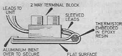
Fig. 3. A small holder is constructed as shown to accommodate the thermistor.
