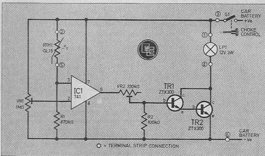
Fig. 1. Complete circuit diagram of the Choke Warning Device.
