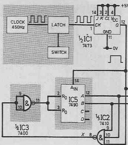
Fig. 7.8 (a). Circuit for a Digital Dice. The tinted systems are built-in on the Test-Bed.
