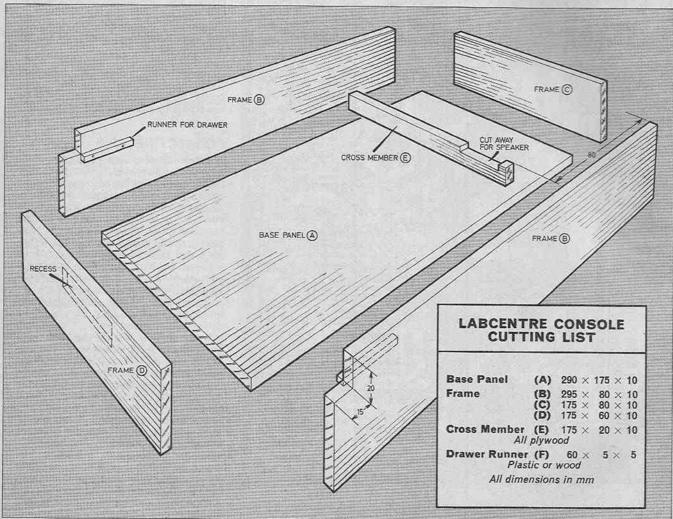
Fig. 2.3. Exploded view of the woodwork construction of the Console with a component drawer.
