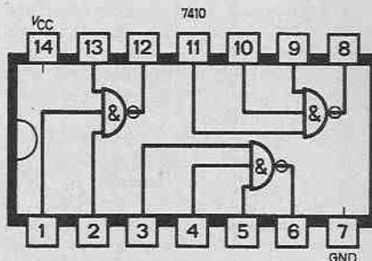
Fig. 7.9. Pinning details for the 7410, triple 3-input NAND gate i.c.
