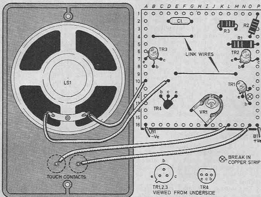
Fig. 2. Complete wiring details for the unit. There is only one break to be made, and is at O12. Resistor R3 is a vertically mounted component.
