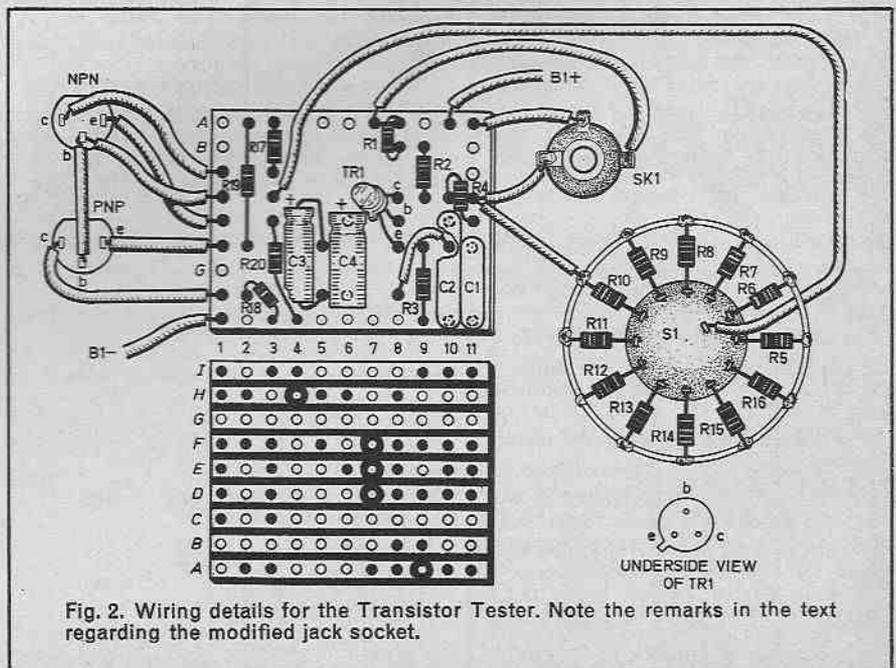
Fig. 2. Wiring details for the Transistor Tester. Note the remarks in the text regarding the modified jack socket.
