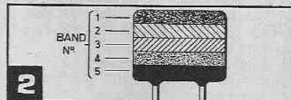
For example, a C280 capacitor with band colours (from top) reading YELLOW, VIOLET, ORANGE, BLACK, RED, has a value of  $47 \times 10^3$  pF  $\pm 20\%$  250V;  $47 \times 10^3$  pF = 47,000 pF which is more usually written as 0.047 $\mu$ F (microfarads).
