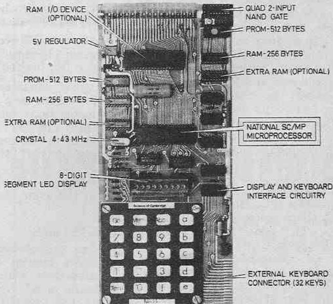
One unusual and useful feature is a DELAY instruction which causes the chip to pause for a time count which can be selected by the programmer. Accurate time periods can easily be generated with this instruction, provided that a crystal is used with the on-chip clock oscillator.
