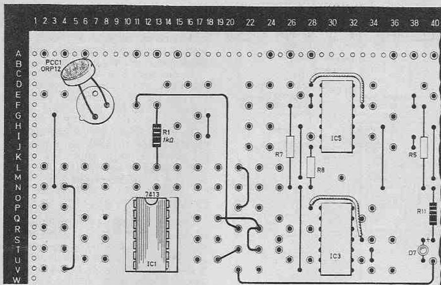
Fig. 7.2 (b). The circuit of Fig. 7.2 (a) wired up on the Test-Bed.
