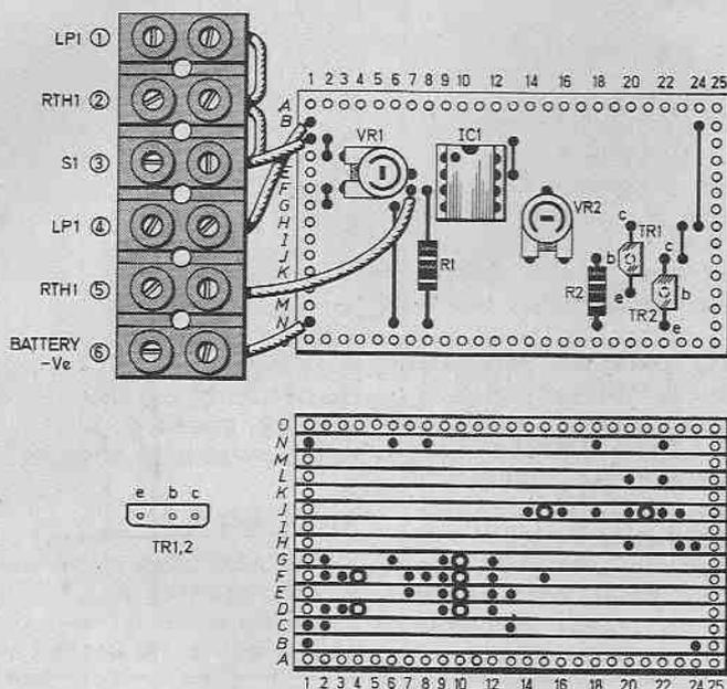
Fig. 4. Stripboard layout, also showing the breaks to be made and other wiring.
