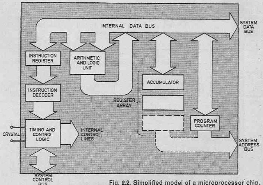
Fig. 2.2. Simplified model of a microprocessor chip.
