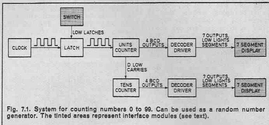
Fig. 7.1. System for counting numbers 0 to 99. Can be used as a random number generator. The tinted areas represent interface modules (see text).
