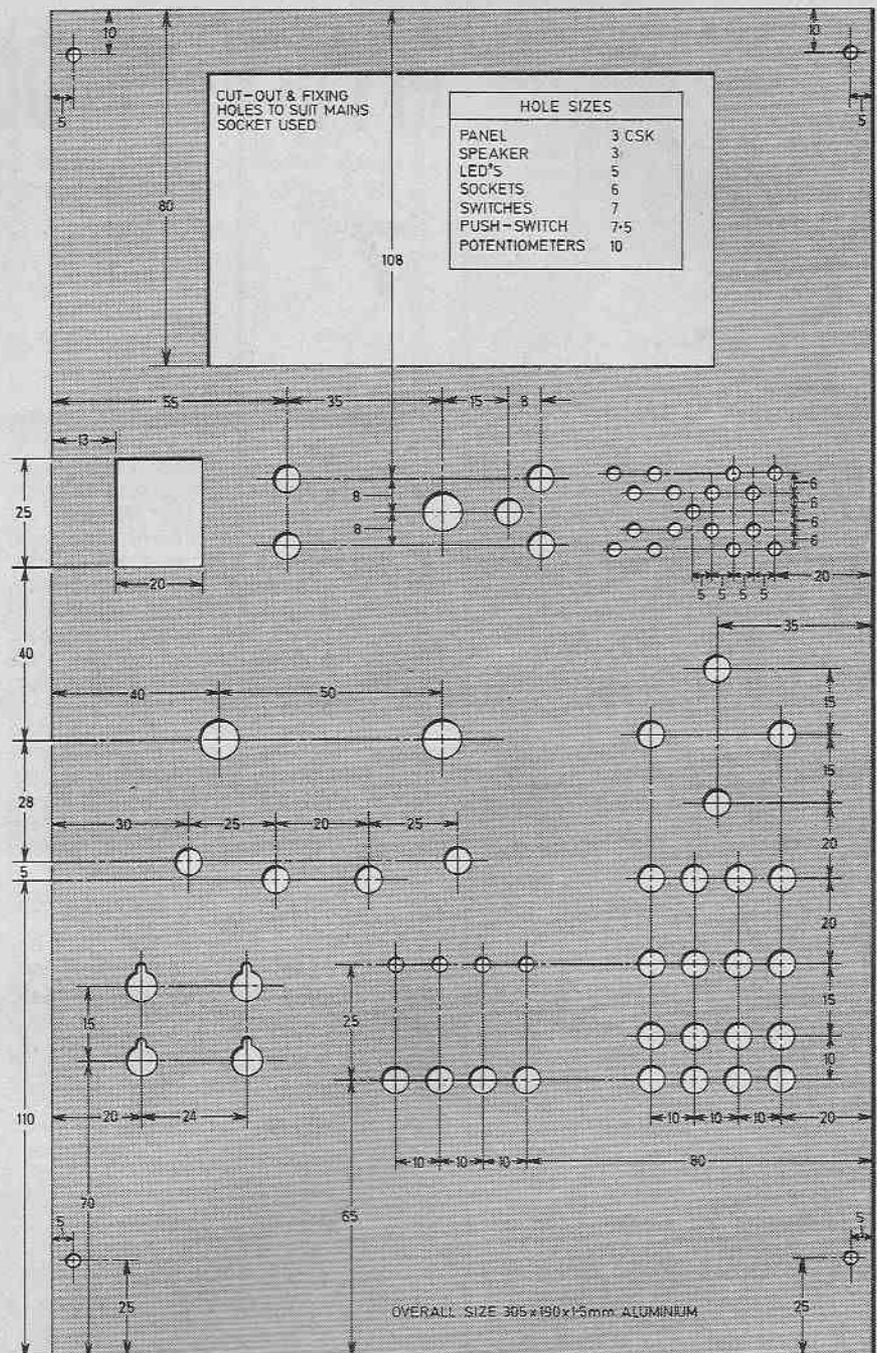
Fig. 2.4 Complete drilling details for the top panel of the Console. Dimensions in mm.
