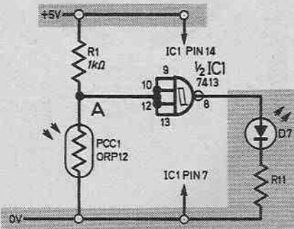
Fig. 7.2 (a). The circuit diagram for a Light Sensor.
