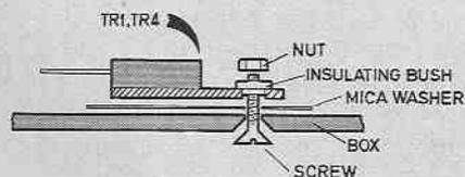
Fig. 4. Power transistor mounting details.
