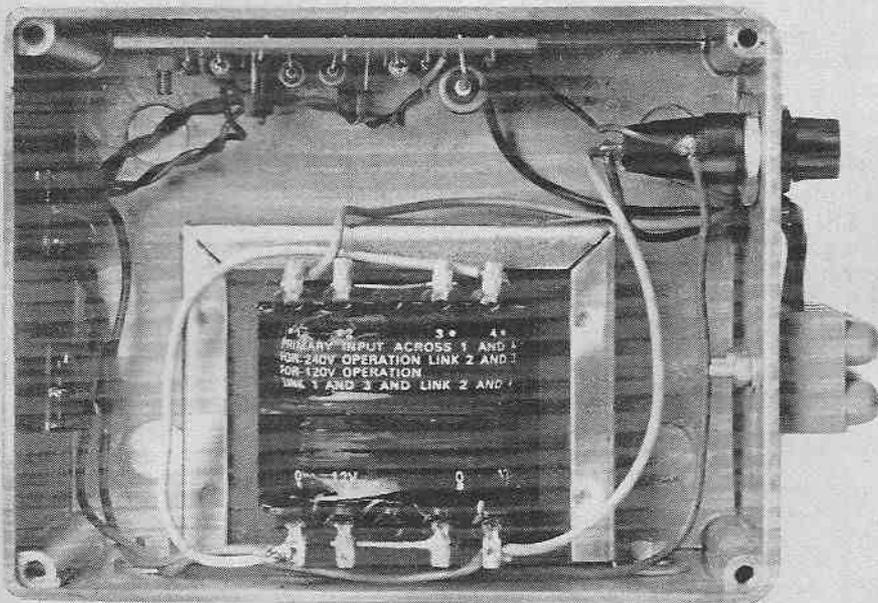
Internal view of the Shaver Inverter showing the relative positions of the components. Note how the component board is mounted using 6BA hardware. As a further safety measure to that already mentioned, some insulating tape can be stuck to the inside of the lid to prevent the tags of the transformer touching, and possibly causing a short circuit.
