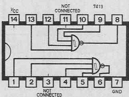
Fig. 7.4. Pinning details for the 7413 dual 4-input NAND Schmitt i.c.
