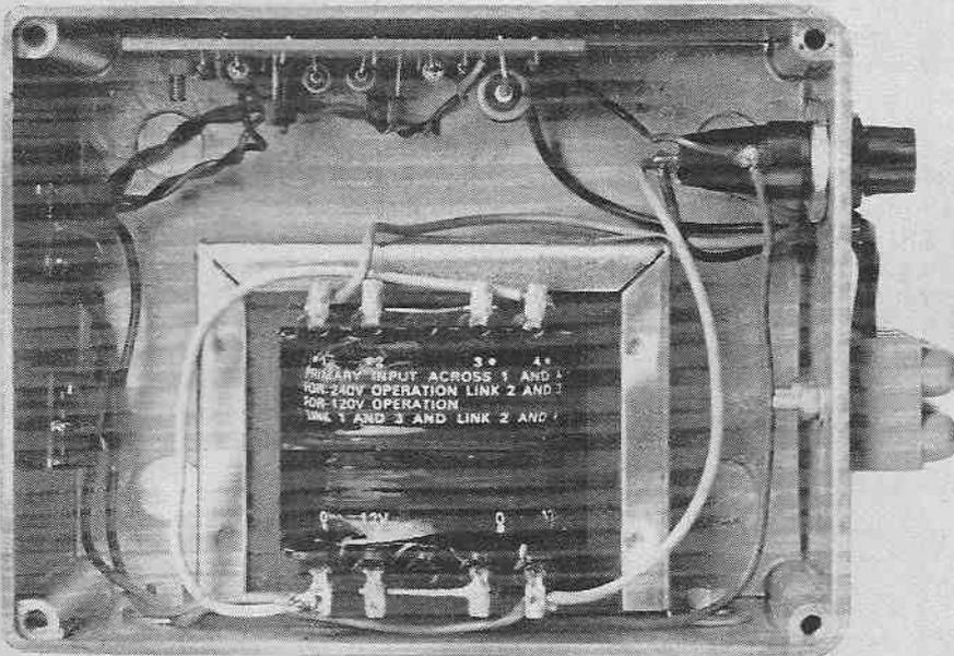
Internal view of the Shaver Inverter showing the relative positions of the components. Note how the component board is mounted using 6BA hardware. As a further safety measure to that already mentioned, some insulating tape can be stuck to the inside of the lid to prevent the tags of the transformer touching, and possibly causing a short circuit.
