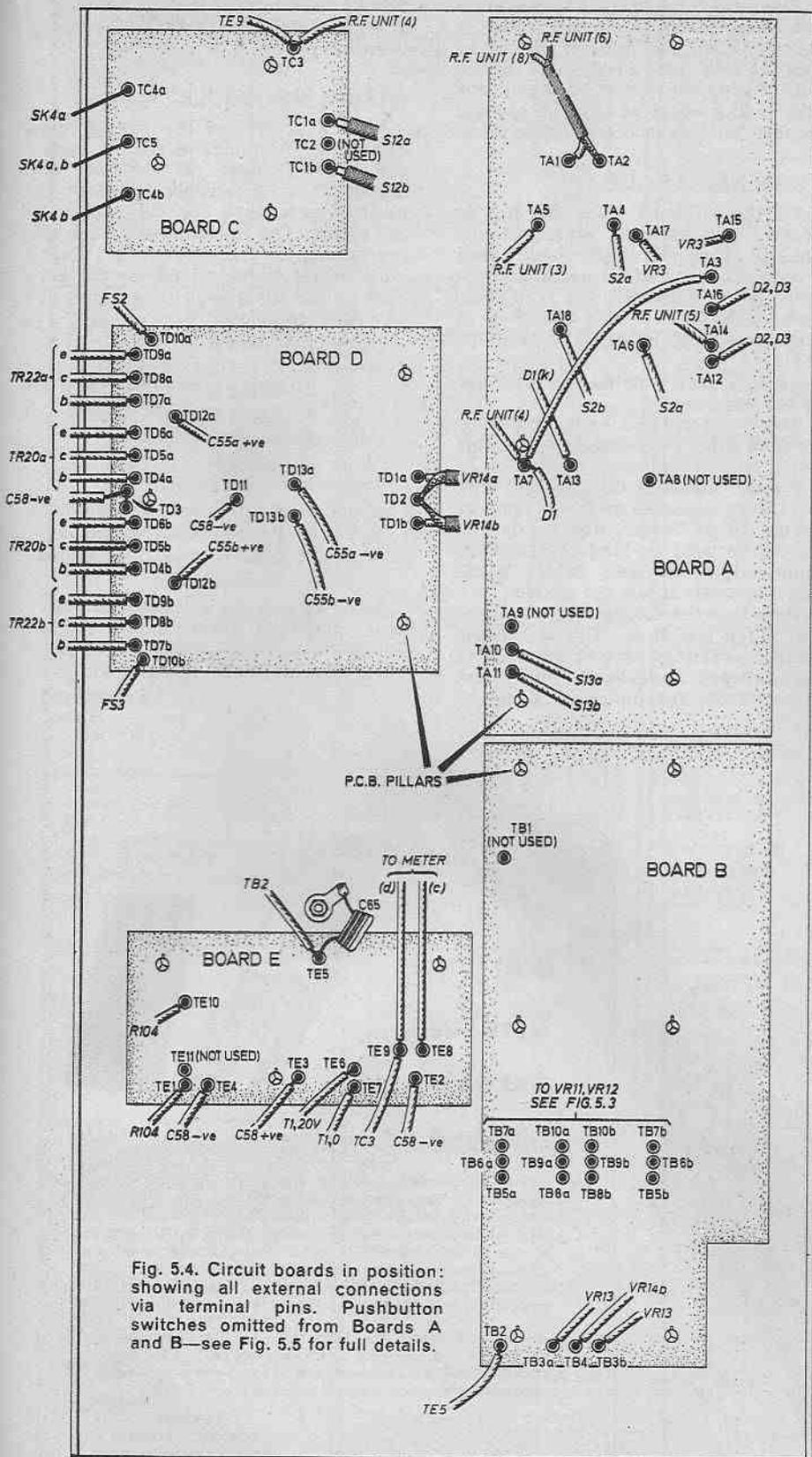
Fig. 5.4. Circuit boards in position: showing all external connections via terminal pins. Pushbutton switches omitted from Boards A and B—see Fig. 5.5 for full details.
