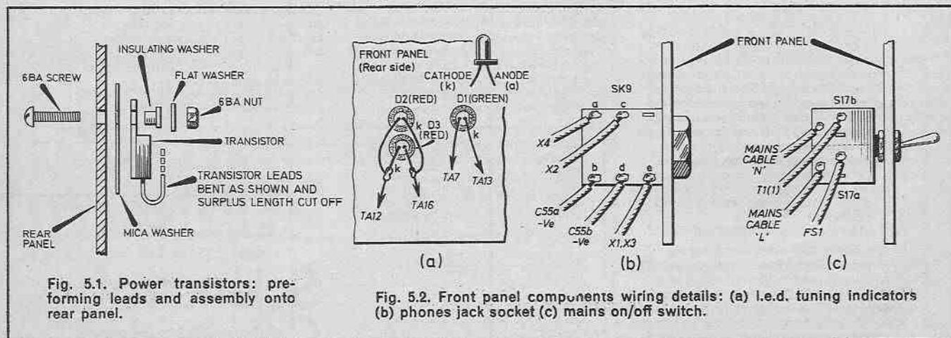
Fig. 5.1. Power transistors: performing leads and assembly onto rear panel.
