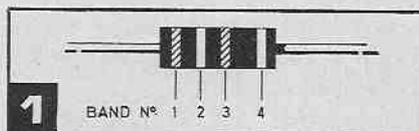
For example, a resistor coded RED, VIOLET, YELLOW, GOLD, has a value of  $27 \times 10^4$  ohms  $\pm 5$  per cent. For those unfamiliar with index notation,  $10^4$  is the same as 10,000, so the resistor value is 270,000 ohms abbreviated usually to 270 kilohms (270k $\Omega$ ). As can be seen, a number of zeros equal to the power of ten (in our example—four) is written after the first two digits.
