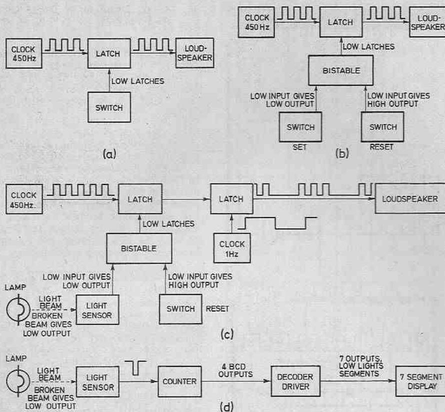
Fig. 7.6. Logical systems. (a) Morse practice buzzer (b) Alarm activated by SET switch (c) Light activated intruder alarm with intermittent tone (d) system for counting goods on a conveyor belt, or people passing through a doorway.
