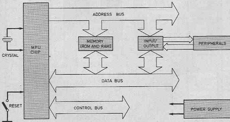
Fig. 2.1. A simple microprocessor system.
