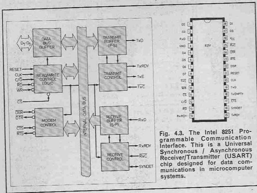
Fig. 4.3. The Intel 8251 Programmable Communication Interface. This is a Universal Synchronous / Asynchronous Receiver/Transmitter (USART) chip designed for data communications in microcomputer systems.
