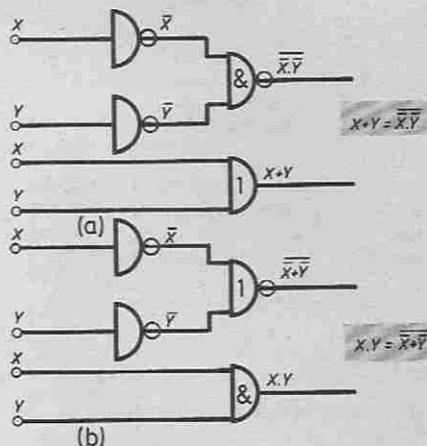
Fig. 9.1. Using basic logic gates to illustrate De Morgan's Laws.
