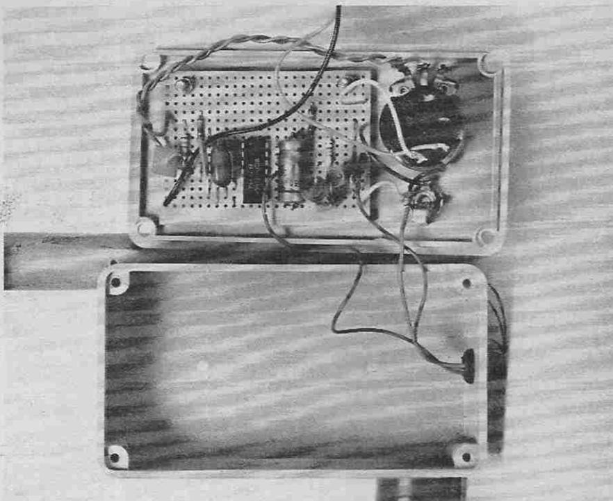
The case is a small plastic box which measures about 111 x 60 x 27mm, and VR1 and the output socket are mounted at one end of the lid. This leaves sufficient room for the completed component panel to be mounted on the lid using two short 6BA screws.
