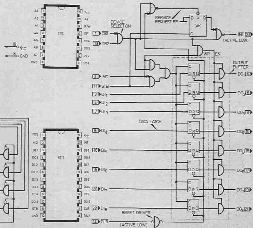
Fig. 4.2. The Intel 8212 8-bit Input/Output Port. All principal functions of a microprocessor system can be implemented.
