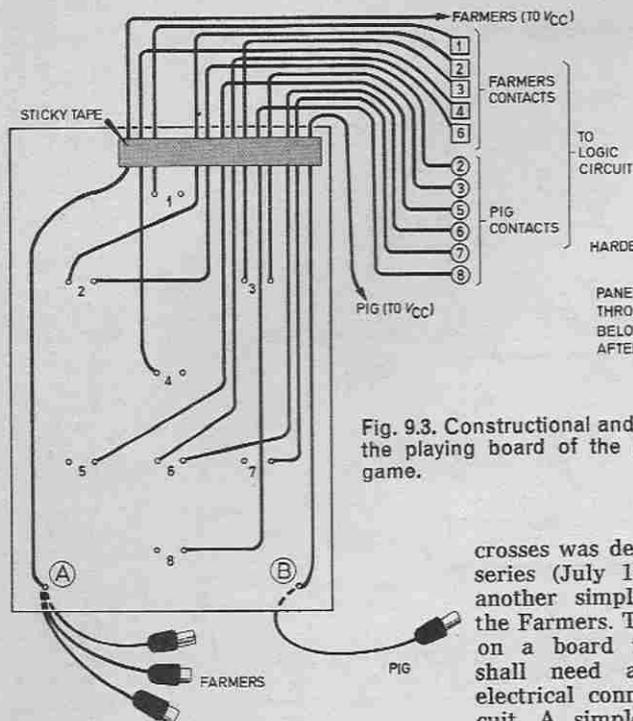
Fig. 9.3. Constructional and wiring details for the playing board of the Pig and Farmers game.
