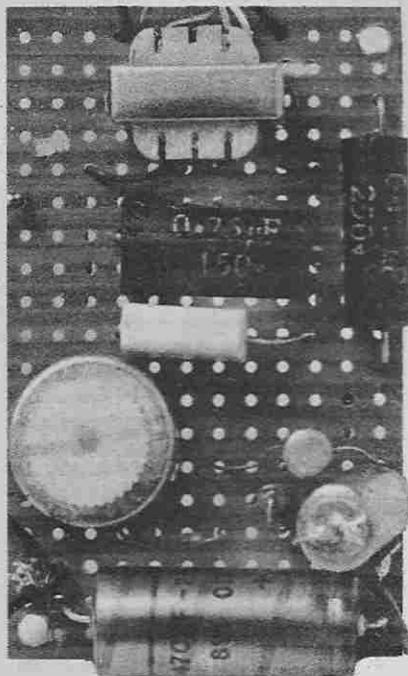
Layout of components on the completed circuit board.
