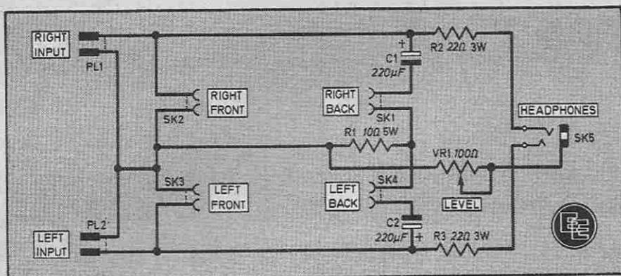
Fig. 3. Circuit diagram of the Quad Simulator. This is suitable for systems up to 10W r.m.s. output.
