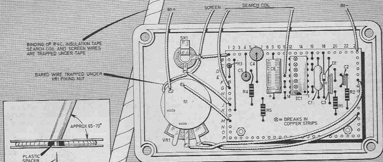
Fig. 4. Stripboard layout also showing connections to VR1 and the output socket. The board is mounted on the lid of the case using short 6BA screws.
