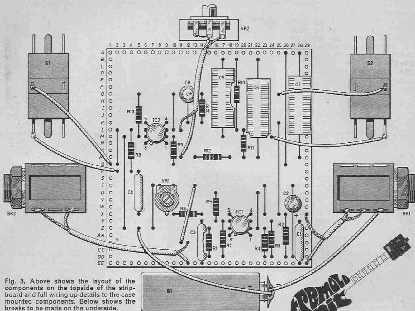
Fig. 3. Above shows the layout of the components on the topside of the strip-board and full wiring up details to the case mounted components. Below shows the breaks to be made on the underside.
