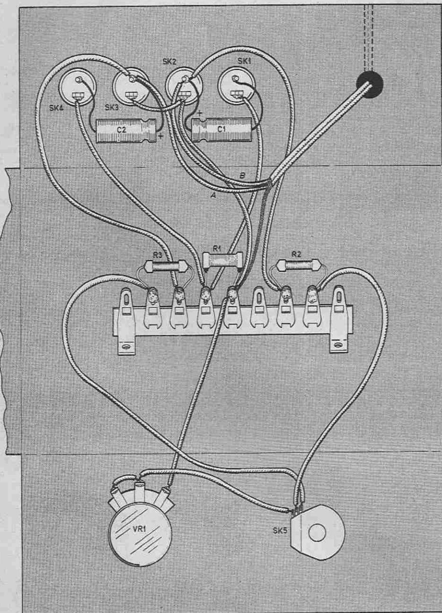
Fig. 4. Complete wiring details for the unit. Note the case has been "opened out" for clarity. There is nothing critical about the layout and could be varied as required.
