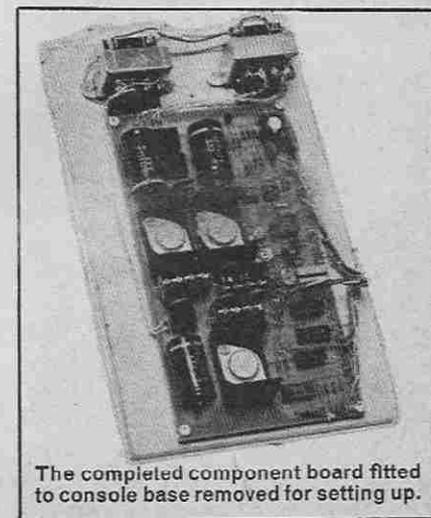
The completed component board fitted to console base removed for setting up.
