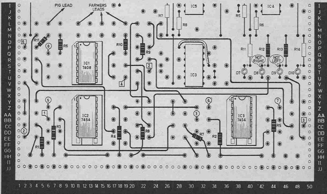
Fig. 9.4b. The circuit of Fig. 9.4a wired up on the Test-Bed.
