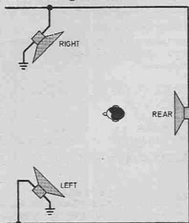
Fig. 1. Hafler's basic idea of adding a single speaker.
