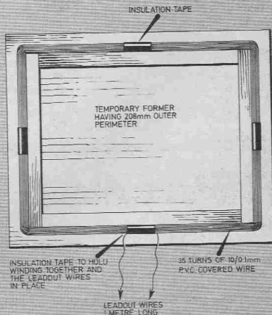
Fig. 5. Construction details for the coil. About 15 metres of wire is required. If a shield is required it should be fitted at this stage.
