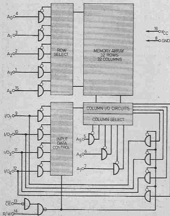
Fig. 4.1. The Intel 2112 1,024-bit Static Random Access Memory. No "refreshing" is required with this type of RAM.
