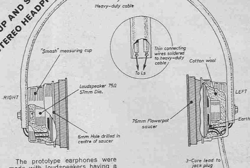
The prototype earphones were made with loudspeakers having a nominal impedance of 75 ohms, which allows them to be used of course with any output up to that impedance, and the higher rating means that they are slightly reduced in sensitivity, which is an asset particularly when the phones are to be connected to the loudspeaker outputs of equipment that does not boast an earphones socket.
