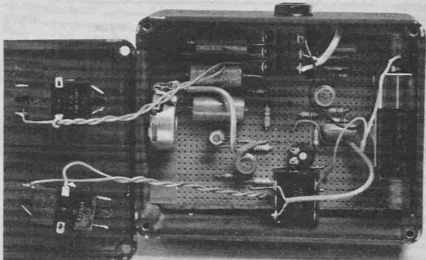
The completed prototype unit with lid removed showing case mounted components, board positioning and wiring to the lid mounted switches.
