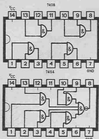
Fig. 9.5. Pinning details for the 7408 and 7454 logic i.c.s.
