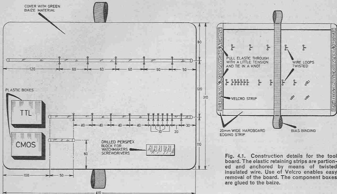
Fig. 4.1. Construction details for the tool board. The elastic retaining strips are partitioned and anchored by means of twisted insulated wire. Use of Velcro enables easy removal of the board. The component boxes are glued to the baize.
