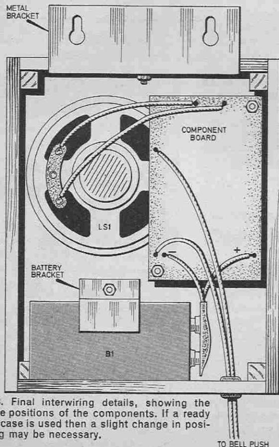
Fig. 3. Final interwiring details, showing the relative positions of the components. If a ready made case is used then a slight change in positioning may be necessary.
