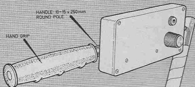
Fig. 6. Constructional details for the framework as used on the prototype. Dimensions are not critical and if required can be varied to suit individual requirements.
