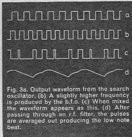
Fig. 3a. Output waveform from the search oscillator. (b) A slightly higher frequency is produced by the b.f.o. (c) When mixed the waveform appears as this. (d) After passing through an r.f. filter, the pulses are averaged out producing the low note beat.
