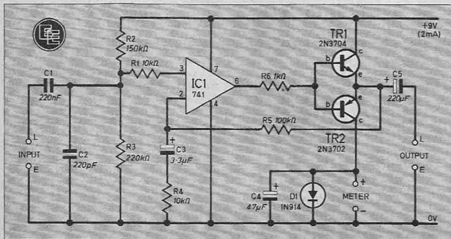
use a new value for R4, calculated from:  $R4 \text{ (new)} = 100 \text{ kilohms} (A - 1)$  where  $A$  is the required gain.
