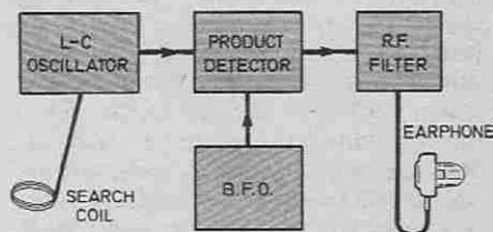
Fig. 1. Principle of the beat frequency oscillator circuit. Here two oscillators run at very nearly the same frequency thus producing an audible beat note in the earpiece. Any slight shift in the LC oscillator frequency will cause a change in the beat note heard. This change in frequency is caused by bringing a piece of metal in the vicinity of the search coil. This alters the inductance of the coil, thus changing the frequency of the tuned circuit.
