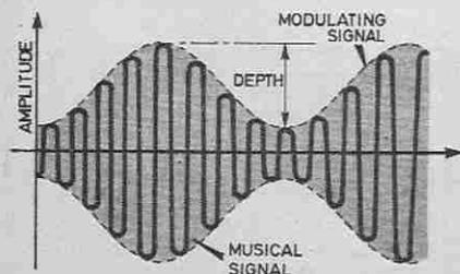
Fig. 1. The tremolo effect in graphical form. A sinewave “music signal” has been shown for clarity.
