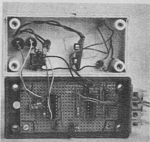
Fig. 3. Complete wiring details for the unit, also showing the stripboard and breaks to be made. There is nothing critical about the layout and can be varied if required.
