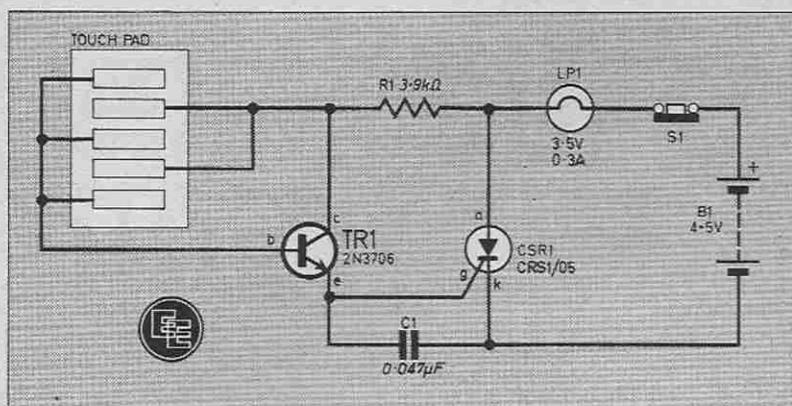
Fig. 1. Complete circuit diagram for the Touch-on Pilot Light.
