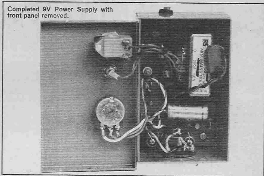
using a mica washer insulation kit and silicon grease. It will be found that the box will get quite warm if the output is left short-circuited for any length of time, and if the temperature of the box is thought to be excessive it can be painted matt black to allow it to dissipate the heat more readily.
