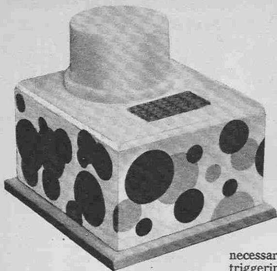
**T**HE SIMPLE project described here operates from a 4.5V dry battery and so is completely safe. It is not necessary to locate and operate a switch in darkness, as the light is put on by light finger contact with a touch pad. The lamp remains on until extinguished by a switch fitted on the unit.
