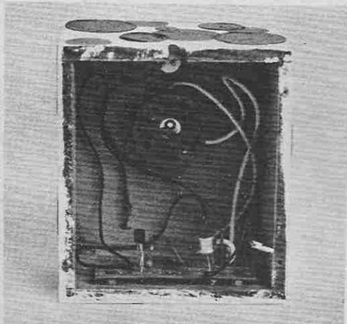
The completed Touch-on Pilot Light showing positioning of components and circuit board.
