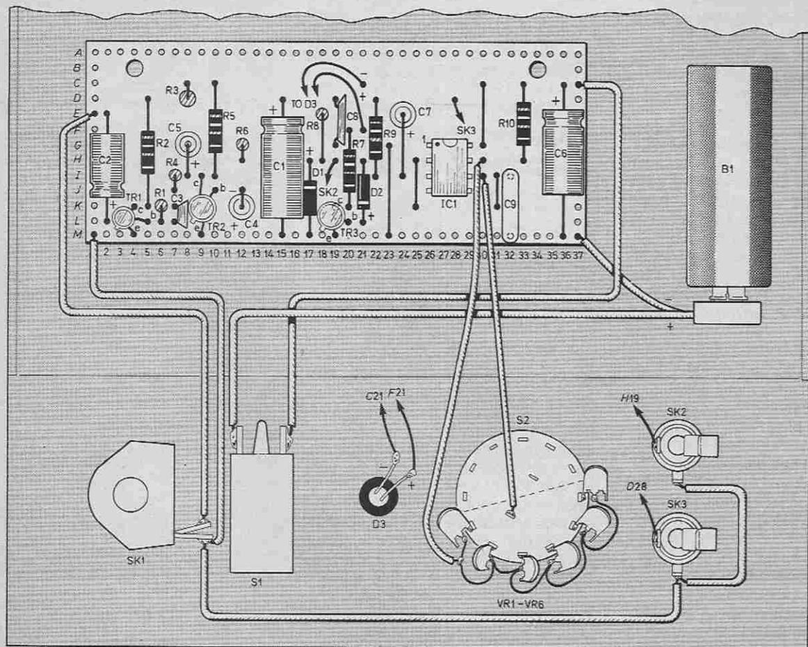
Fig. 2. Complete wiring details for the unit also showing the stripboard layout and breaks to be made. All the tuning presets are mounted on the switch to save space on the board. It is not necessary to use screened wire when wiring to the sockets, as the metal case provides sufficient screening.
