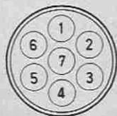
Fig. 4. Pin connections to Trailer Socket. The pin numbers are usually marked on the socket.
