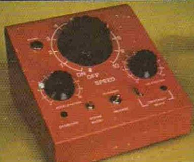
A pulse width trim controller for smooth slow running plus inertia braking and acceleration. Full construction details in our catalogue.
