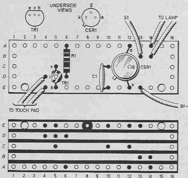
Fig. 2. Stripboard layout. Only one break is required. Insure that the thyristor and transistor are inserted correctly. If a metal case is used then it is necessary to isolate the mounting holes by means of breaks either side of the holes.
