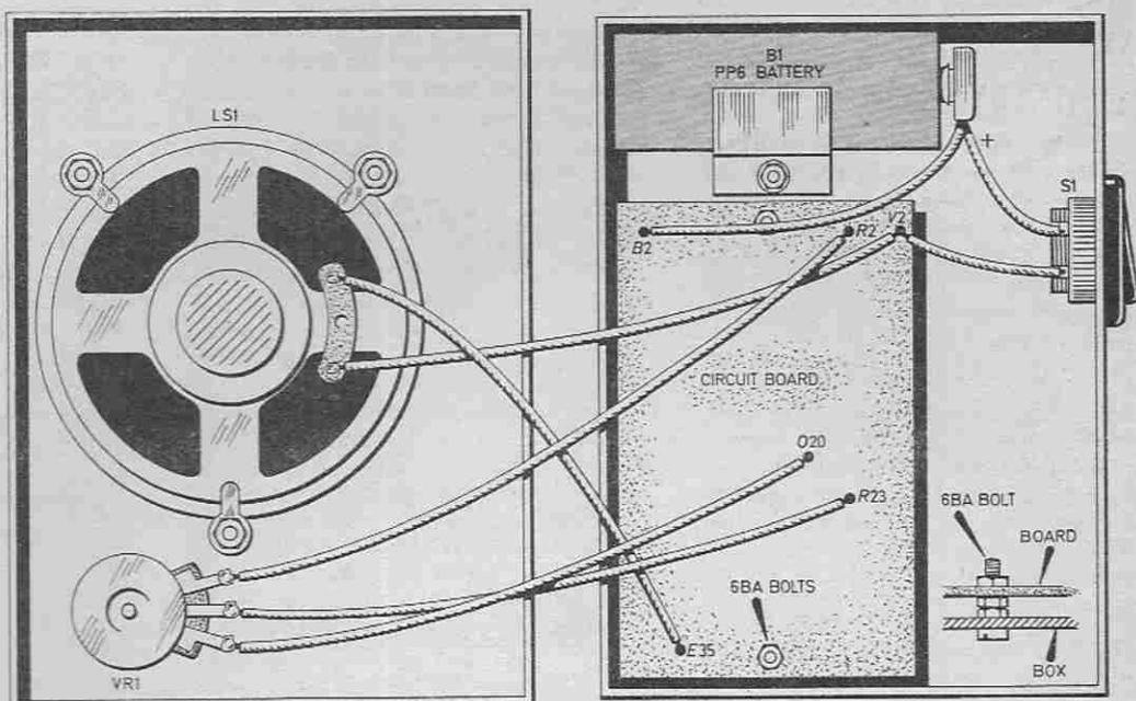
Fig. 6. The complete assembly with inter-wiring between the circuit board and the other components mounted directly onto the aluminium box.
