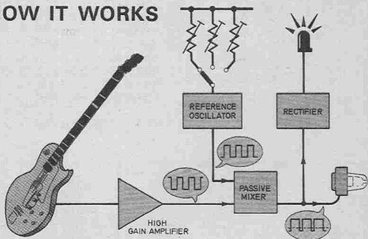
A note from either an acoustic or electric guitar is applied to a *high gain amplifier* which turns the very low input from the guitar into a much larger signal which is sufficient to be applied to one input of a *mixer*. The other input is connected to a stable *reference oscillator* having six switched frequencies which correspond to the six notes of a guitar.
