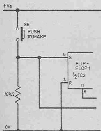
Fig. 2. Modification required to the circuit of Fig. 1 if the timing period option is not required.
