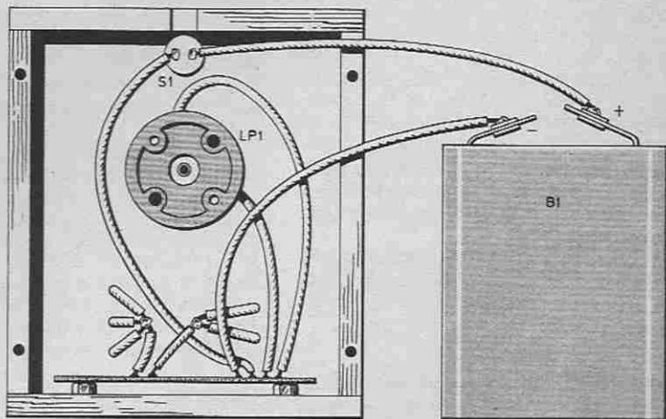
Fig. 3. The remainder of the wiring is completed as shown here. The holder for the bulb is simply glued into place.
