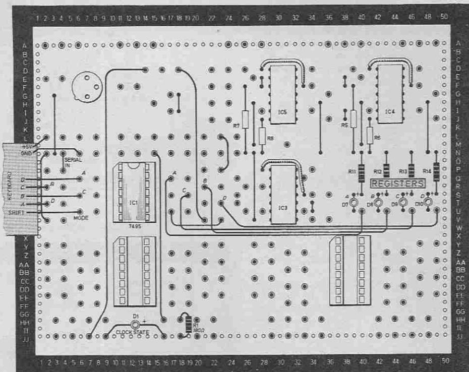
Fig. 11.5b. The circuit of Fig. 11.5a wired on the Test-Bed for testing the 7495.
