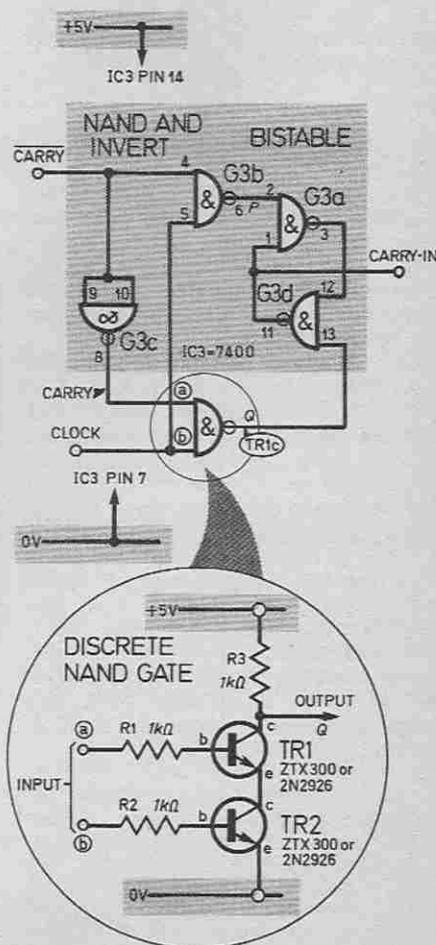
Fig. 11.8a. Circuit diagram for carry function and circuit of a discrete NAND gate.
