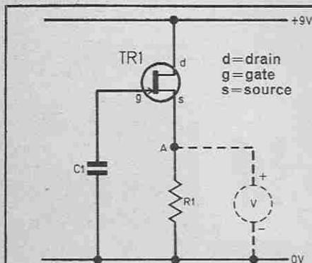
Fig. 1. The timing circuit. Changes of potential at point A may be examined by a voltmeter as shown.
