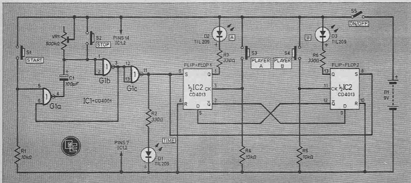
is normally low. When S3 is pressed, a pulse is applied to the clock terminal, pin 3. This causes the flip-flop to change state, producing a low output at pin 1 and a high output at pin 2. The low at pin 1 illuminates D2 thus indicating that player A has answered the question first. At the same time the high condition at pin 2 is applied to pin 9 of Flip Flop 2 preventing it from changing state if player B presses his button.
