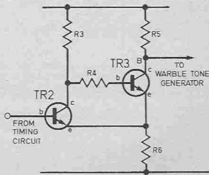
Fig. 3. The trigger circuit: b=base, c=collector, e=emitter.
