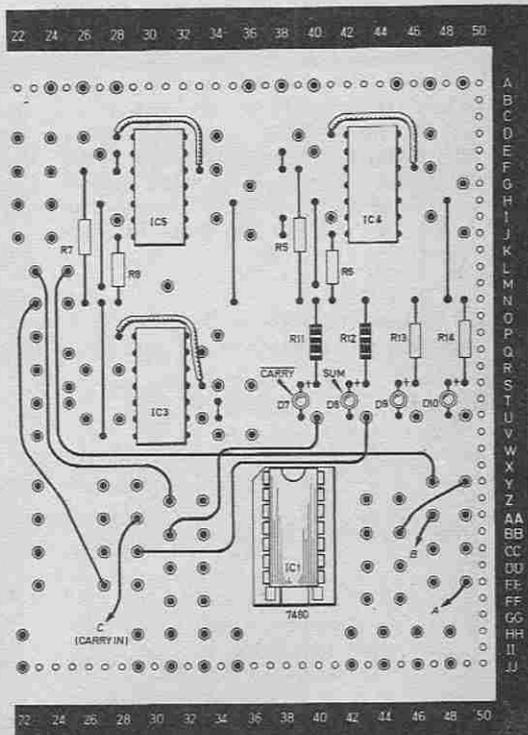
Fig. 11.3b. The circuit of Fig. 11.3a wired on the Test-Bed for testing the 7480 Full-adder.
