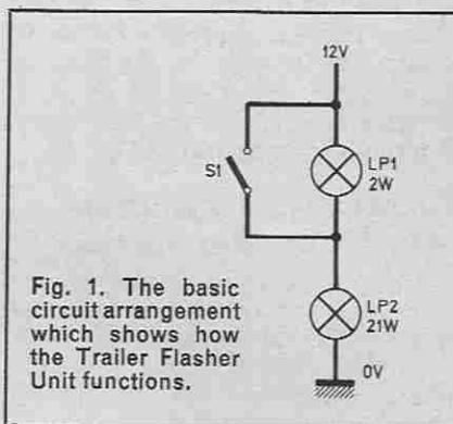
Fig. 1. The basic circuit arrangement which shows how the Trailer Flasher Unit functions.
