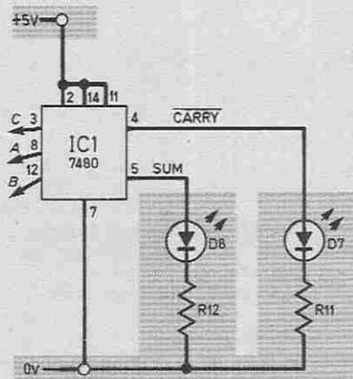
Fig. 11.3a. Circuit diagram for a Full-adder using the 7480.
