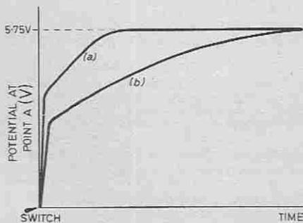
Fig. 2. Rise in potential at point A: (a) with low value capacitor (b) with capacitor of greater value.
