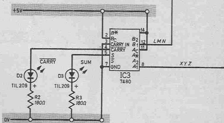
Fig. 11.6a. Circuit diagram for a simple calculator (without carry facility).
