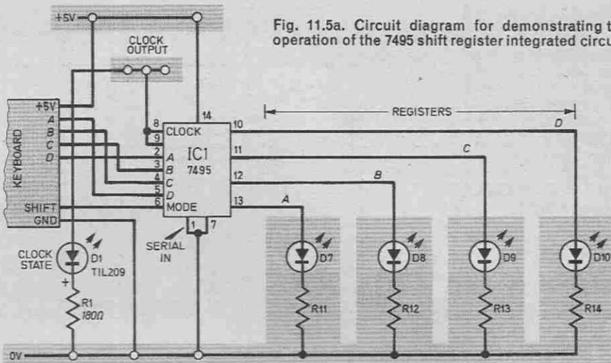
Fig. 11.5a. Circuit diagram for demonstrating the operation of the 7495 shift register integrated circuit.
