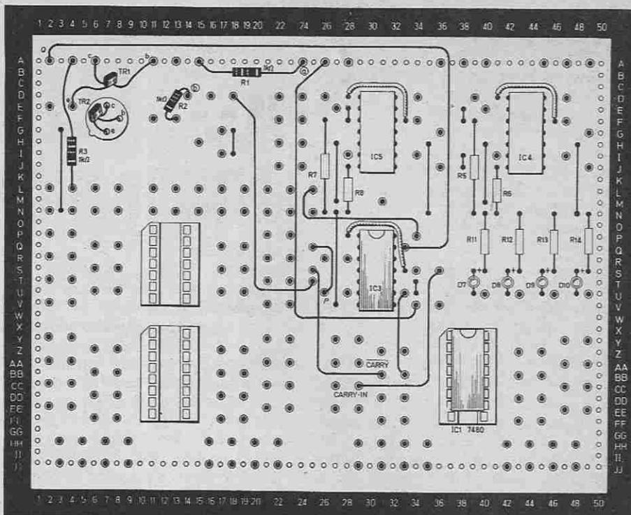
Fig. 11.8b. The circuit of Fig. 11.8a wired on the Test Bed.
