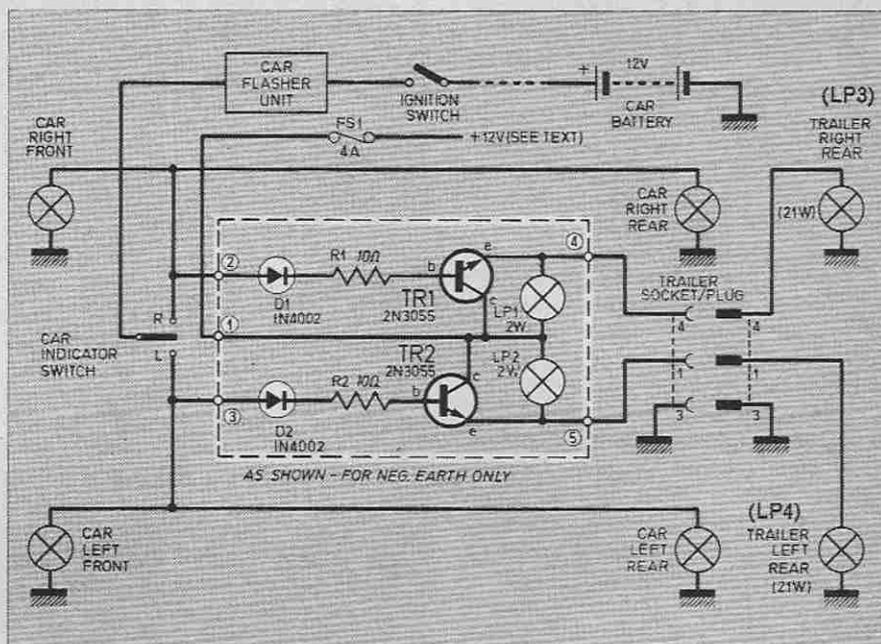
Fig. 2. Full circuit diagram of the Trailer Flasher Unit (within broken line) shown connected to the car circuits and, via trailer socket, to the trailer or caravan circuits. For positive earth TR1 and TR2 must be replaced by *pnp* types.
