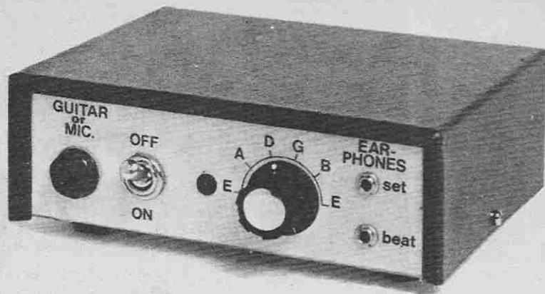
to VR6, are each tuned to a different open string guitar note, with the desired preset and note being selected using S2. A rough square-wave output is obtained at pin 3 of IC1, and this is fed to an earphone socket by way of a simple top cut filter comprised of R9 and C8. The purpose of the filtering is to attenuate the harmonics on the output which are otherwise excessive, and tend to drown the fundamental frequency.
