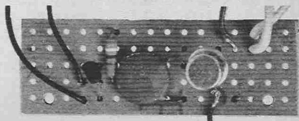
The completed circuit board for the Touch-on Pilot Light.
