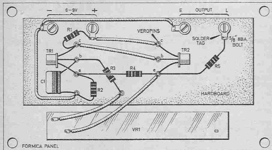
Fig. 2. Component layout on hardboard base. This is secured to the Formica panel by the four 8BA bolts.
