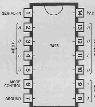
Fig. 11.4. Pinning details for the 7495 shift register.
