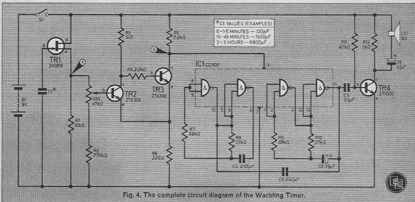
Fig. 4. The complete circuit diagram of the Warbling Timer.
