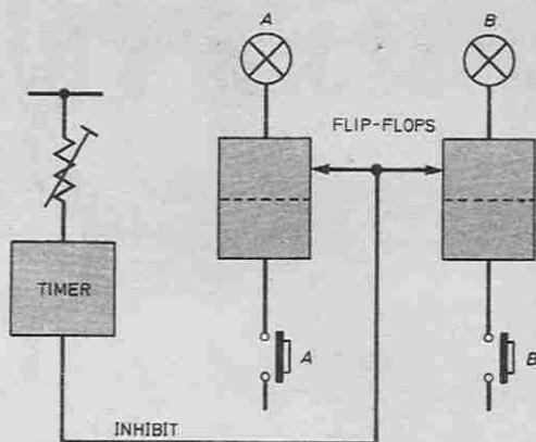
The unit consists of two flip flops, one for each player or teams. A flip flop is an electronic circuit which has two stable states; a short clock pulse applied to the input will cause the device to change state. In this circuit, if player A presses his button the flip flop will change state and illuminate the light. At the same time a second output from the flip flop will inhibit player B's flip flop.
