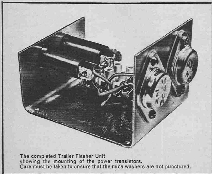
The completed Trailer Flasher Unit showing the mounting of the power transistors. Care must be taken to ensure that the mica washers are not punctured.
