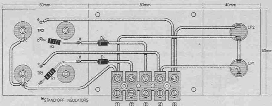
Fig. 3. The complete Flasher Unit shown "opened up" for clarity. The chassis is made from a single piece of 18 or 20 s.w.g. aluminium, with two bends as indicated. All drilling should be carried out before bending. See text for further details.
