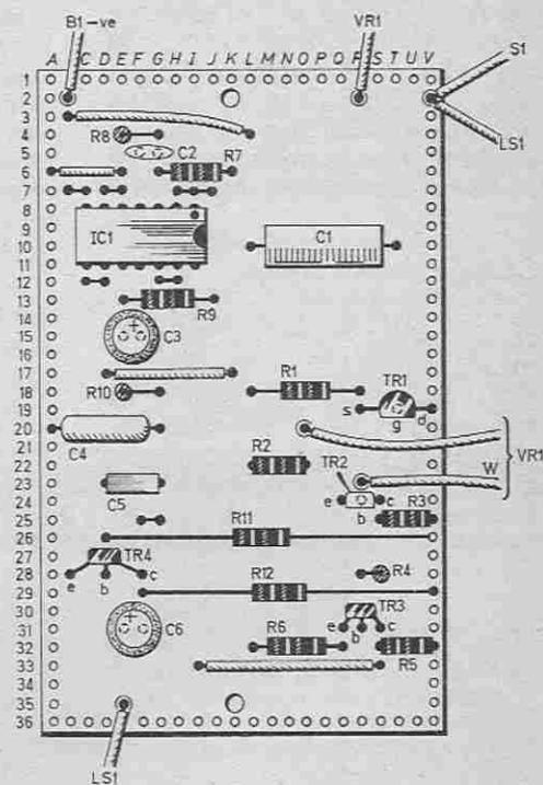
Fig. 7. Underside and top view of the stripboard. Note the breaks required in the copper strips, also the wire links.
