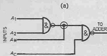
Fig. 11.2a Pinout details for the 7480 Full-adder i.c. and (b) gating on  $A$  inputs ( $B$  input gating is identical).
