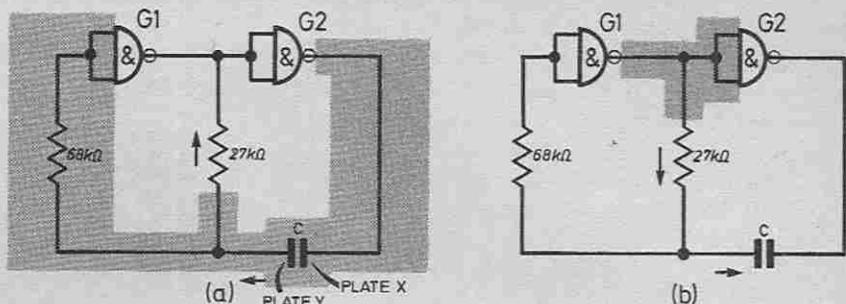
Fig. 5. The two states of an astable multivibrator, as used in the warble-tone generator. Parts of the circuit shaded are at "high" potential; other parts are at "low" potential.
