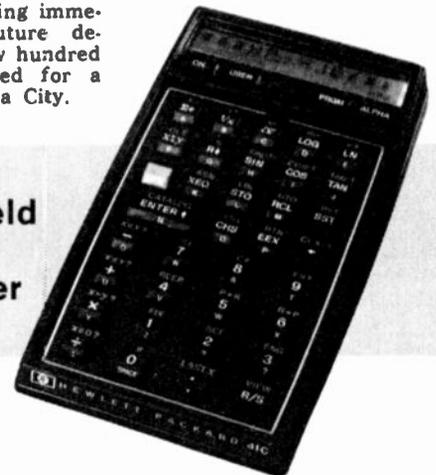
The new Hewlett-Packard HP-41-C programmable calculator has so many facilities, including substantial built-in memory, that it is already being hailed as the world's first hand-held computer.
