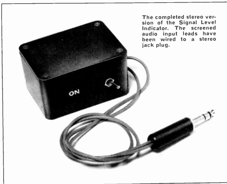
The completed stereo version of the Signal Level Indicator. The screened audio input leads have been wired to a stereo jack plug.
