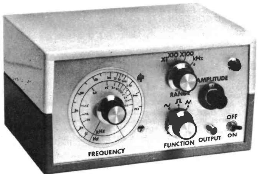
The sinewave signal has a minimum harmonic distortion factor of about 2 per cent when correctly adjusted but lower than this is not possible as the sinewave is obtained by electronic shaping within IC1 and not by pure generation.
