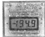
Based on the ICL7106. This Kit contains a PCB resistors, presets capacitors, diodes, IC and 0.5" liquid crystal display.
