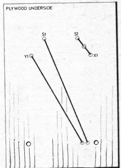
Fig. 2. Component layout of charger board showing (a) top side before covering with Formica, (b) top side after covering, (c) the underside.
