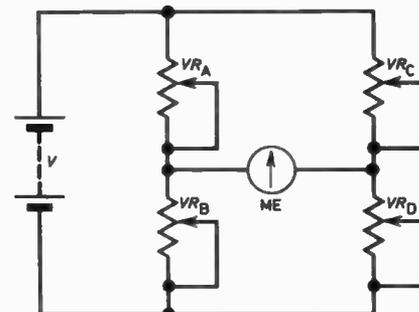
Fig. 3.7. A simple electronic slide-rule can be achieved using four variable resistors (or potentiometers connected as variable resistors).
