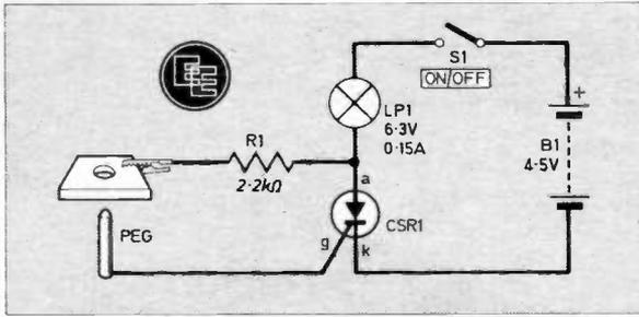
Fig. 1. Circuit diagram of the Peg-a-Hole game.
