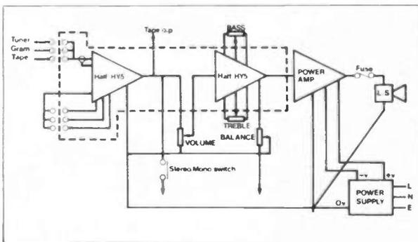
The HY5 pre-amp is compatible with all I.L.P. amplifiers and P.S.U.'s. It is contained within a single pack 50 x 40 x 15 mm. and provides multi-function equalisation for Magnetic/Ceramic/Tuner/Mic and Aux (Tape) inputs, all with high overload margins. Active tone control circuits; 500 mV out. Distortion at 1KHz—0.01%. Special strips are provided for connecting external pots and switching systems as required. Two HY5's connect easily in stereo. With easy to follow instructions.
