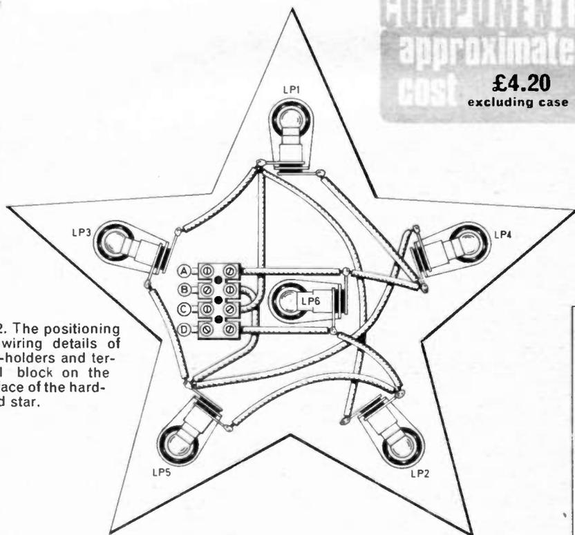
Fig. 2. The positioning and wiring details of lamp-holders and terminal block on the rear face of the hard-board star.
