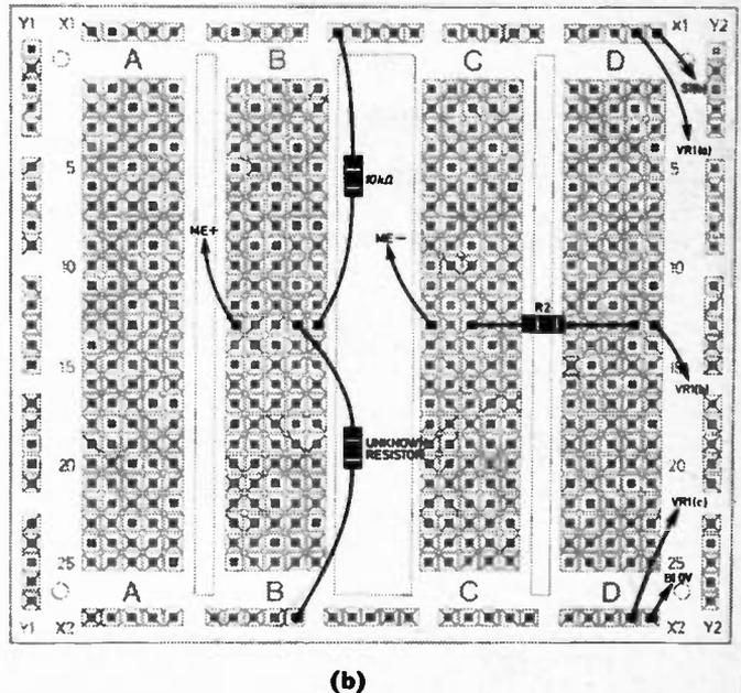
varying the ratio  $R_C/R_D$  since  $R_C$  is now the resistance from the wiper to the top of the potentiometer and  $R_D$  is the resistance from the wiper to the bottom of the potentiometer—both varying as the wiper is moved. Imagine the scale of this potentiometer calibrated so that the ratio  $R_C/R_D$  can be read directly. We have now built a simple ohmmeter.
