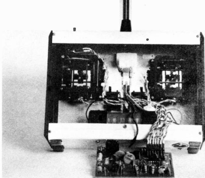
those constructors not using the sockets. Fig. 2.2 shows the points to connect to. For tidiness sake the wires should be twisted together to form a trio; 6in lengths should be sufficient to attach to the board for now, final trimming to length can be performed at a later date when the board is inserted into the case.
