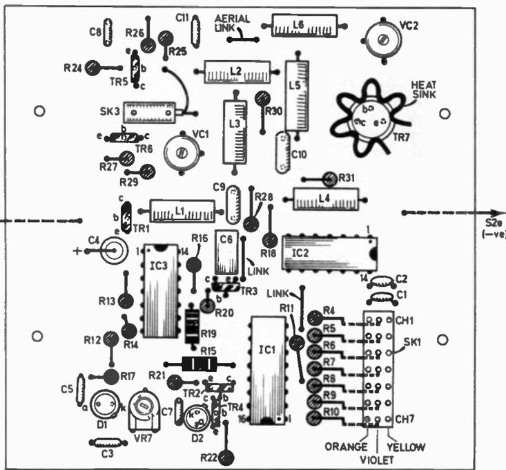
Fig. 2.2. Top view of the printed circuit board with all components in situ (full 7-channel version).
