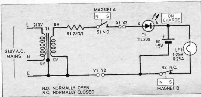
Fig. 1. Complete circuit diagram of the Everlasting Candle.
