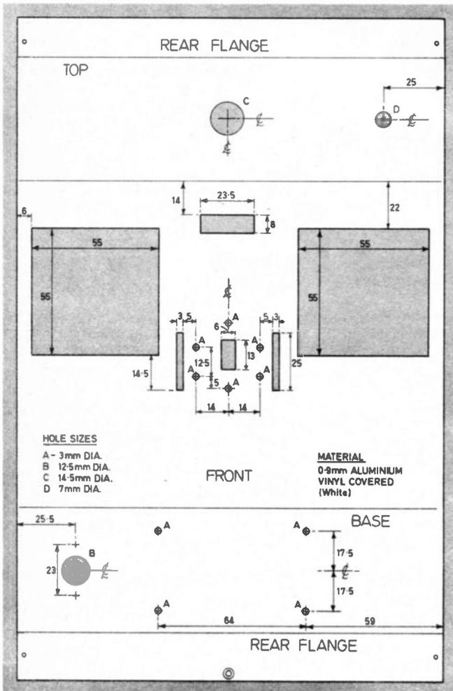
Fig. 2.5. Transmitter case panel opened out flat. Cut-out and drilling details to accommodate controls for seven channels.
