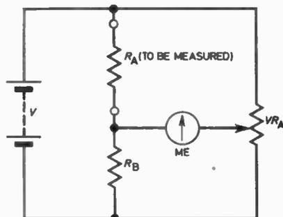
Fig. 3.6. The simple bridge can be converted into an ohmmeter by using a potentiometer and fixing  $R_B$ .
