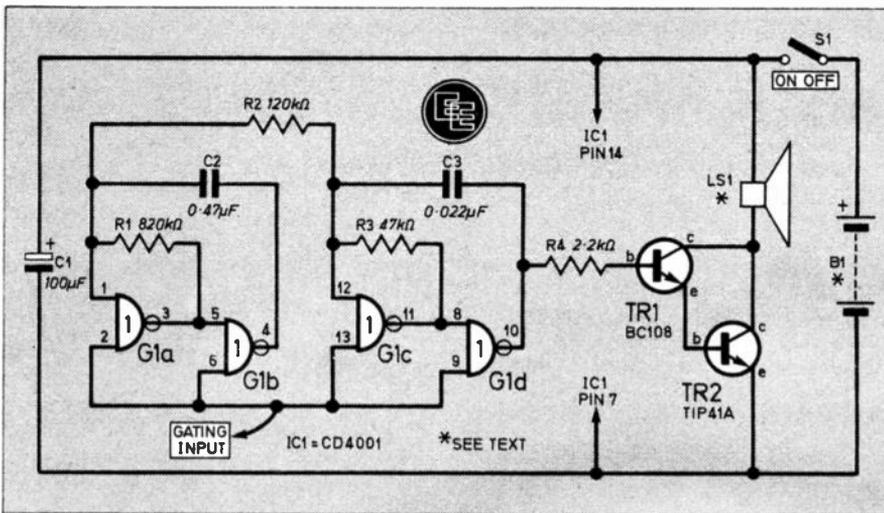
Fig. 1. The complete circuit diagram of the Modulated Tone Generator.
