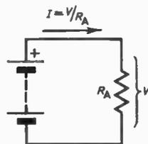
Fig. 3.1. (left) In this simple circuit all the voltages and currents are defined by application of Ohm's Law. An imaginary cut at any point in the circuit would show the same number of electrons crossing per second i.e. the same current.
