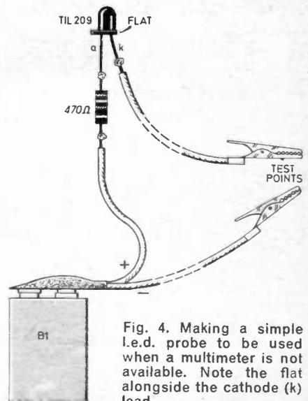
Fig. 4. Making a simple i.e.d. probe to be used when a multimeter is not available. Note the flat alongside the cathode (k) lead.
