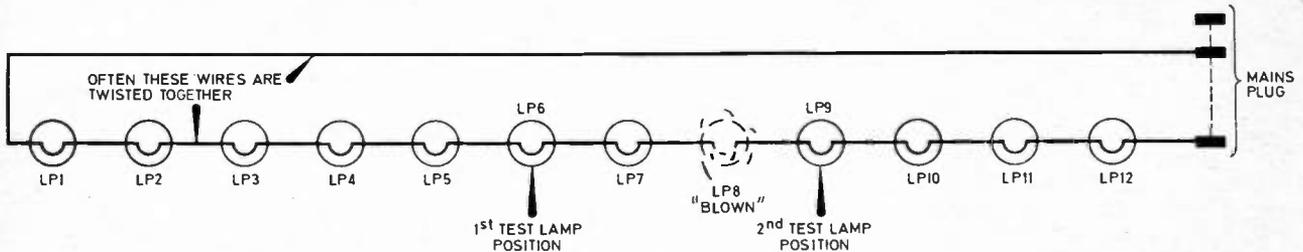
Fig. 5. Procedure for tracing a faulty bulb in a string of twelve series connected bulbs.
