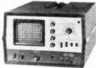
IO 4105 — Single Beam 5 MHz Oscilloscope
