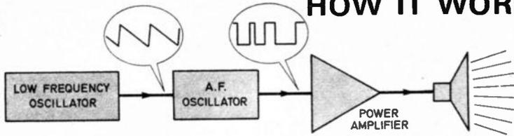
The circuit utilizes two oscillators; one to produce an audio tone, and the other to automatically vary the pitch of this tone. The modulating oscillator operates at a frequency of about 1 to 2Hz, and its output therefore causes the pitch of the tone oscillator to rise and fall about once or twice per second. This rapidly varying of the output note produces a very noticeable and effective alarm signal.
