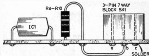
Fig. 2.4. Edge-on view of p.c.b. showing resistors R4 to R10 and their connection to the 7-way socket block.
