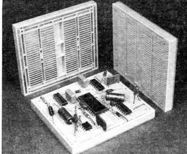
Logically laid out to accept both 0.3" and 0.6" pitch DIL packages as well as Capacitors, Resistors, LED's, Transistors and components with leads up to .85mm dia.
