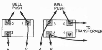
Fig. 3. Typical connections to two of the most popular types of bell systems. These connections are for guidance only and will not necessarily be correct in all cases.
