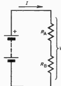
Fig. 3.2. This circuit shows two resistors in series with the battery.
