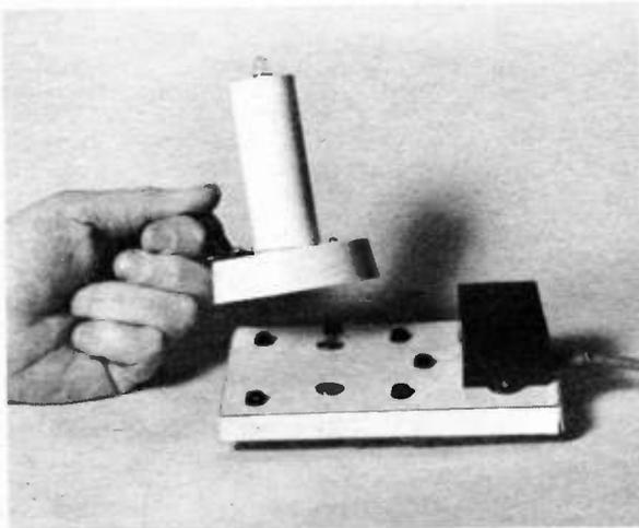
The "candle" being removed from the charger base. For safety reasons a plastic cover **must** be placed over the mains transformer.
