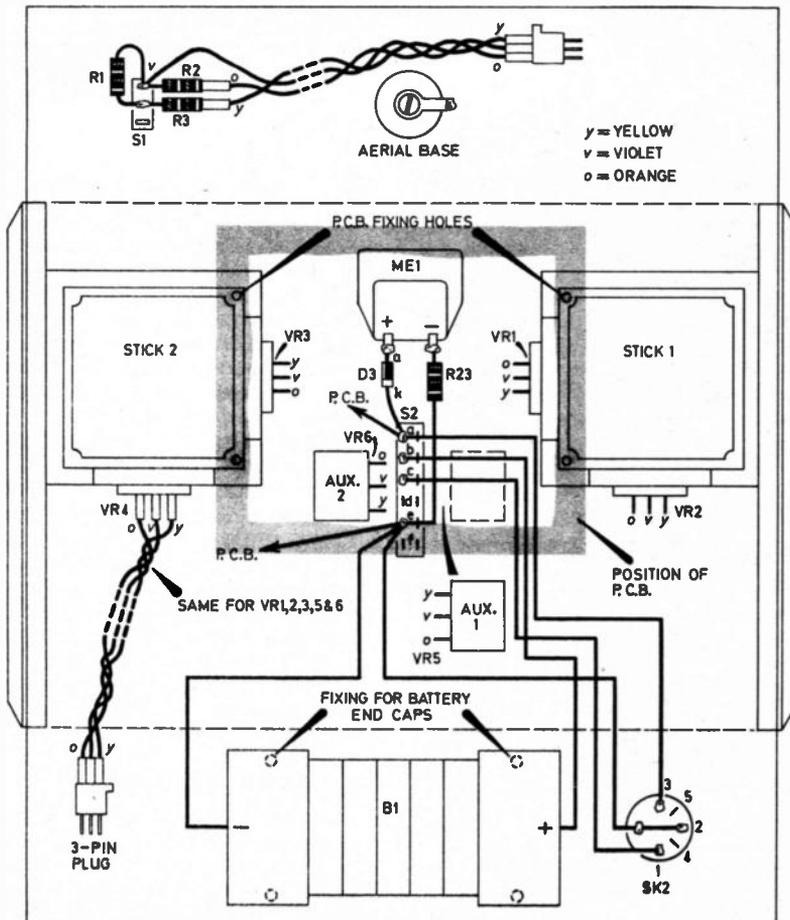
Fig. 2.6. Wiring within the case, to be completed before fitting the p.c.b.
