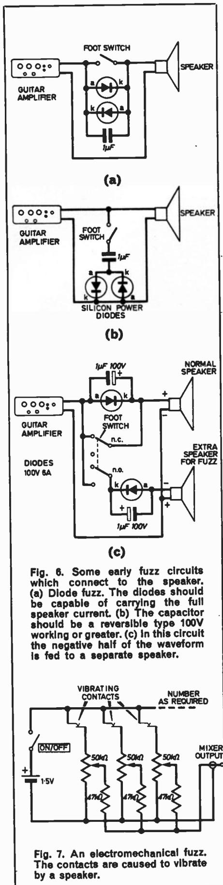
Fig. 6. Some early fuzz circuits which connect to the speaker. (a) Diode fuzz. The diodes should be capable of carrying the full speaker current. (b) The capacitor should be a reversible type 100V working or greater. (c) In this circuit the negative half of the waveform is fed to a separate speaker.
