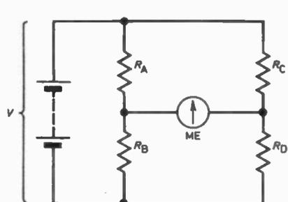
Fig. 3.5. A simple Wheatstone bridge circuit.
