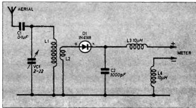
Fig. 2.9. Circuit diagram of the simple Field Strength Meter.
