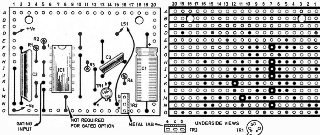
Fig. 2. The layout of the components on the topside of the stripboard and the breaks to be made on the underside.
