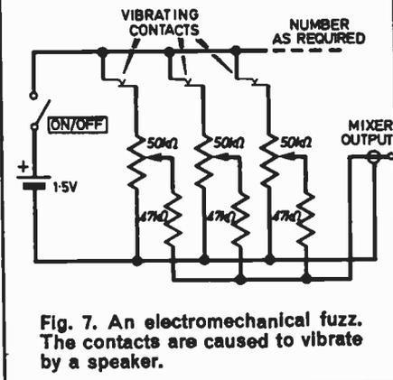
Fig. 7. An electromechanical fuzz. The contacts are caused to vibrate by a speaker.
