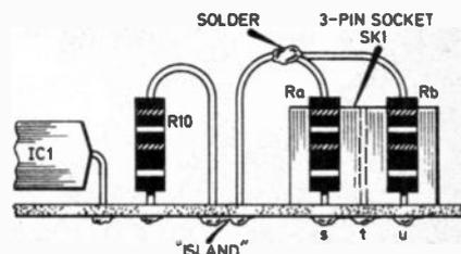
Fig. 2.3. (b) Edge-on view of p.c.b. showing how the additional resistors are mounted in place of the 7-way socket block. (Individual 3-pin sockets are installed for each channel used).
