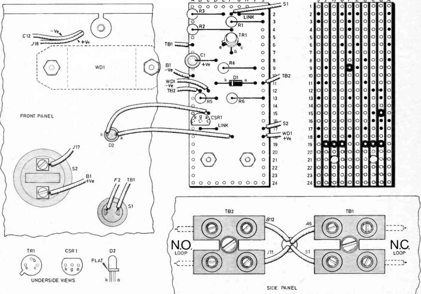
Fig. 2. Complete construction details showing interwiring between board and case mounted components, and layout of the components on the top side of the stripboard.
