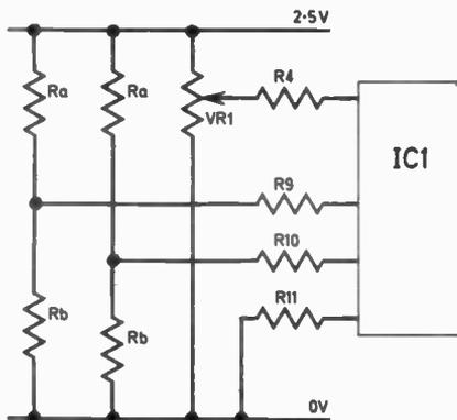
Fig. 2.3. (a) Part of channel switching circuit (see Fig. 1.3) showing additional resistors Ra and Rb fitted to unused channels.
