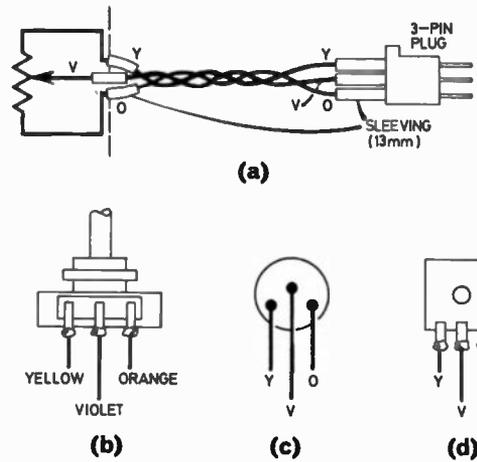
Fig. 2.8. Stick Potentiometers (a) connections to 3-pin plug (b) standard pot (c) cermet or plastic film pot (d) carbon film pot.
