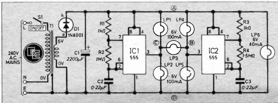
Fig. 1. The complete circuit diagram of the Twinkling Star including an integral power supply unit. Alternately, a battery eliminator can be employed, see text.
