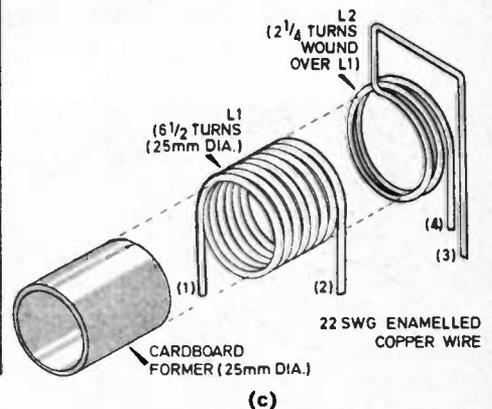
Fig. 2.10. Construction of the Field Strength Meter (a) top view of stripboard (b) underside of stripboard (c) details of coil construction.
