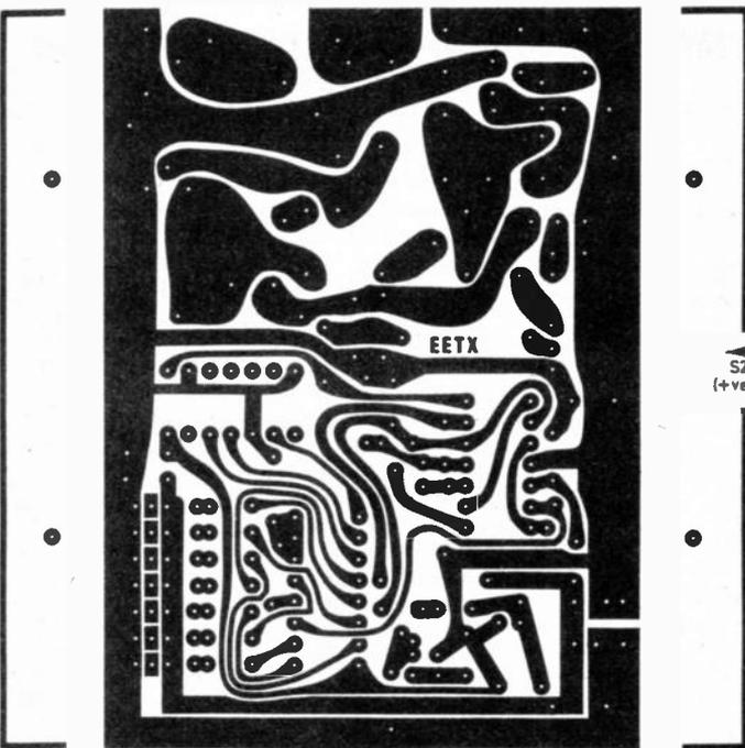
Fig. 2.1. Printed circuit board for the EE Radio Control Transmitter. This is actual size. Note the fixing holes on the outer "plain" or completely etched areas.
