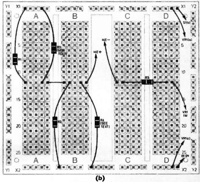
Fig. 3.8. (a) Circuit diagram of the experiment for investigating series and parallel connections. (b) layout of the components on the Tutor Deck.
