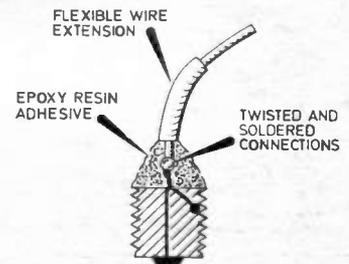
Fig. 3. Construction details for making a test lamp.
