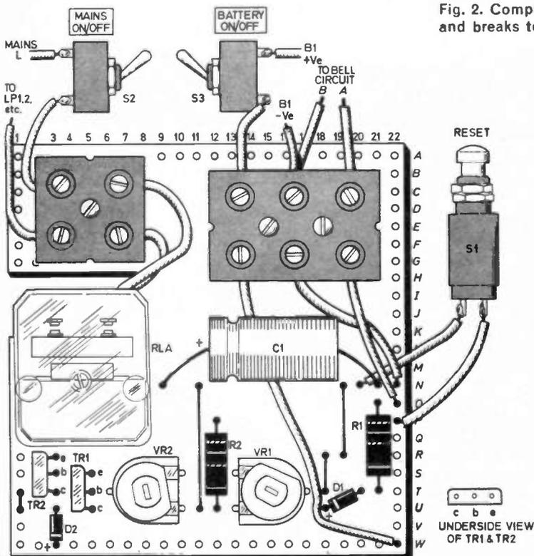
Fig. 2. Complete wiring details for the unit, also showing the stripboard and breaks to be made.
