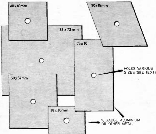
Fig. 2. Completed game showing interwiring and suggested dimensions for the metal pieces.
