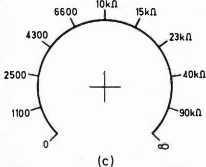
Fig. 3.9. (a) Circuit diagram of the simple ohmmeter (b) Layout of the components on the Tutor Deck. (c) Scaling for the potentiometer so that resistance can be measured directly.
