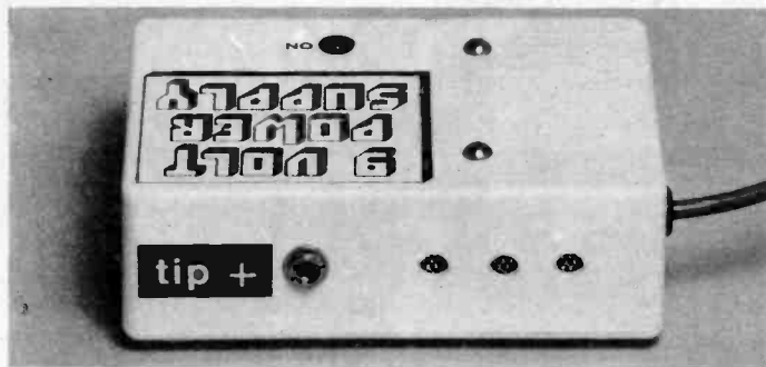
The finished power supply showing the small ventilating holes and the 9V output jack socket.
