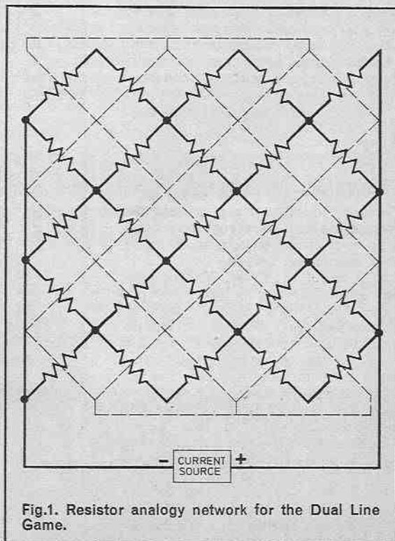
Fig.1. Resistor analogy network for the Dual Line Game.
