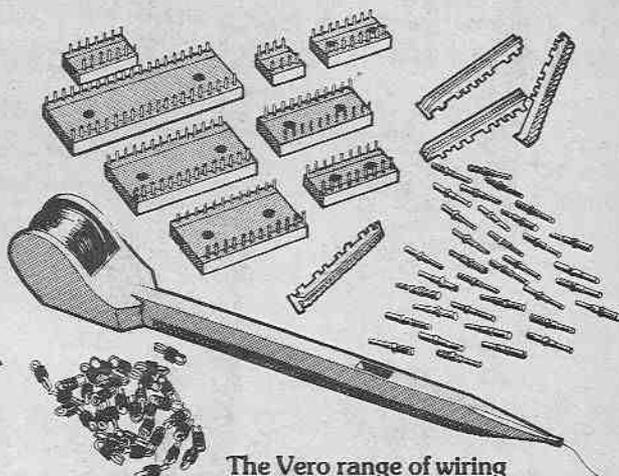
The Vero range of wiring accessories are all highest quality 'professional' products, carefully selected to ease your interconnection problems. There's a full range of pins and DIP sockets (including low-profile) for solder or wire wrapping techniques and the popular Verowire prototype wiring system. Add these to our established range of boards, boxes, frames and cases and you've got all you need for your project. It's all in our catalogue — just send 40p. and it's yours by return.
