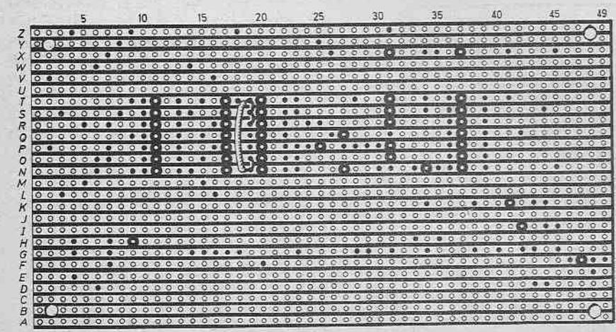
Fig. 2. Complete wiring details for the Auto Fade Unit. Be extra careful when wiring the links, as a mistake will be difficult to trace later on. Note the four links on underside.
