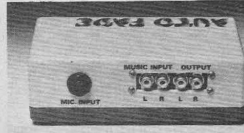
Rear view of the unit showing the phono socket strip and mic. input jack socket.
