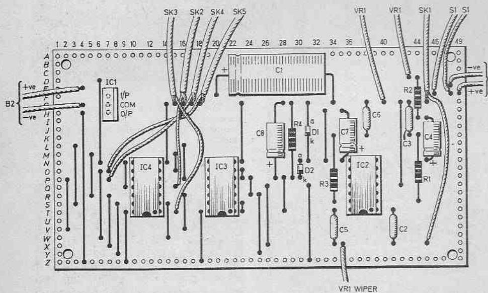
Also shown in this diagram is the front and rear panel wiring details. The case used was a small Verobox type 65-2520J, with dimensions of 150 x 80 x 50mm, although any similar size case can be used. It does not have to be metal to provide screening for the circuit.
