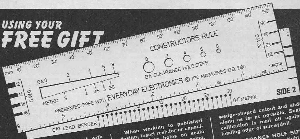
Pocket size instrument with Imperial and metric scales 0-6 inches (0-153mm), plus four gauges of particular usefulness to electronics conductors.
