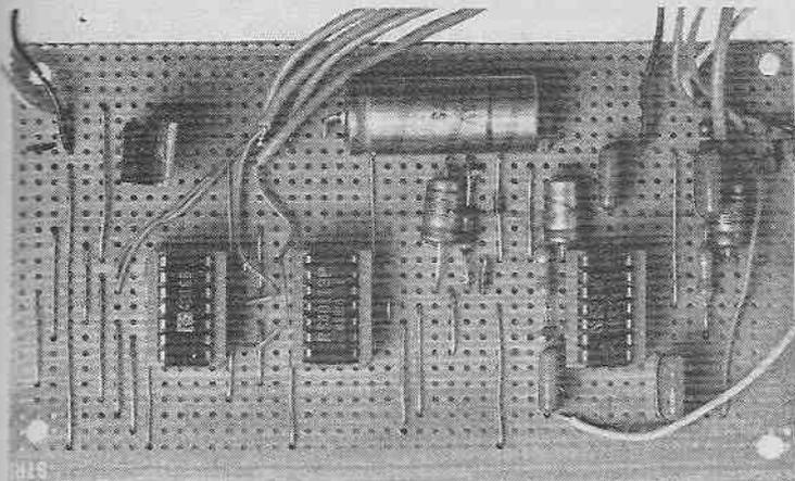
Layout of components on the completed circuit board for the Auto Fade. We strongly recommend the use of i.c. sockets as the i.c.s can easily be damaged during soldering.
