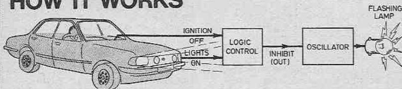
The logic control circuitry normally provides an output to inhibit the operation of the oscillator (it does not oscillate). However, when a condition arises where the lights are on and the ignition is turned off, the logic output changes and allows the oscillator to operate. This activates a warning lamp (or buzzer) inside the car to flash (or sound). The logic circuitry has a built-in parking facility which is enabled by turning the lights off and then on after the alarm has sounded.
