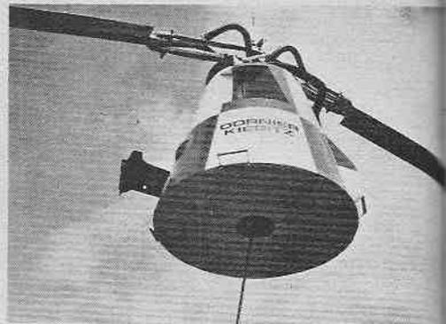
Spy in the sky. A German Dornier "Kiebitz" tethered rotor platform goes aloft from its support truck. Unmanned, it takes electronic equipment up to 1,000ft greatly increasing its operation range.
