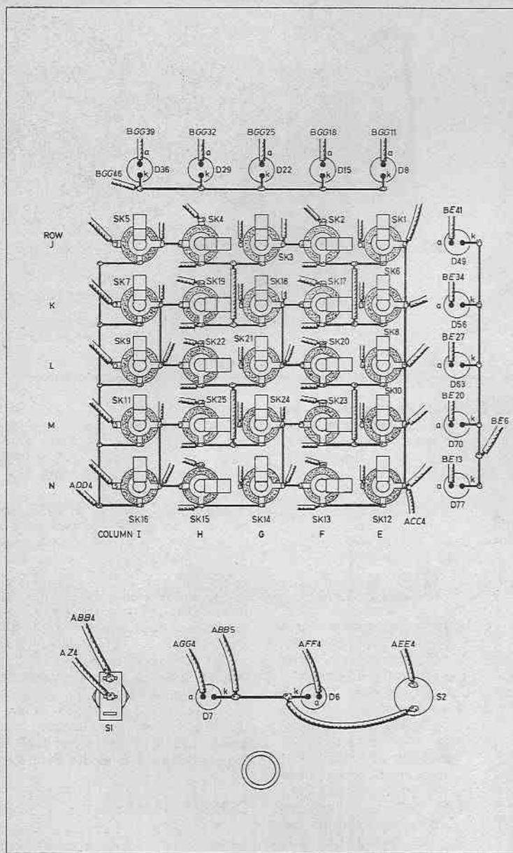
Fig. 9. Wiring of the rear of the front panel.
