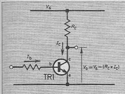
Fig. 8.3. A simple transistor switch using the common emitter configuration. The base current must be greater than that just needed to saturate the transistor.
