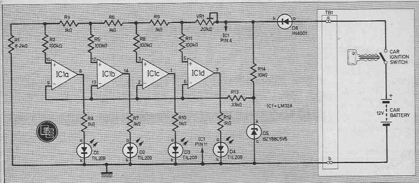
Fig.1. Complete circuit diagram for the Battery Voltage Monitor.
