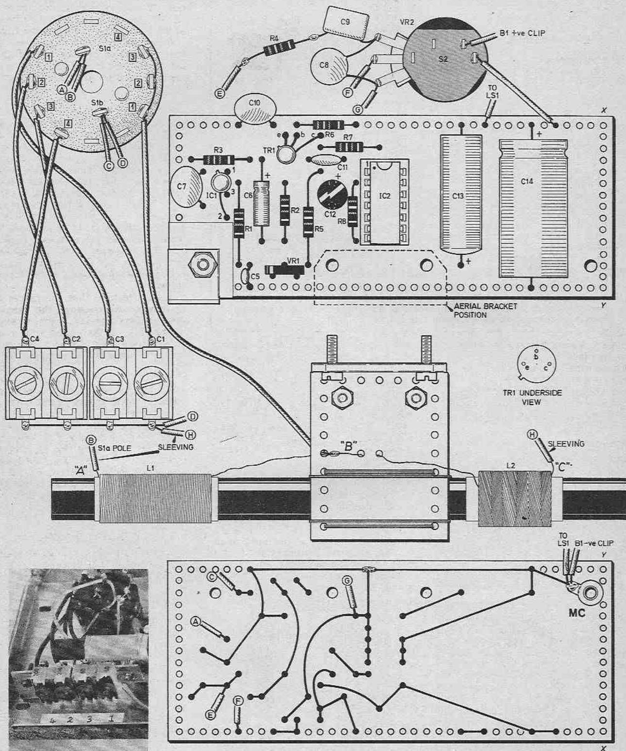
A close-up view of the trimmer capacitor bank showing fixing brackets used in the prototype.
