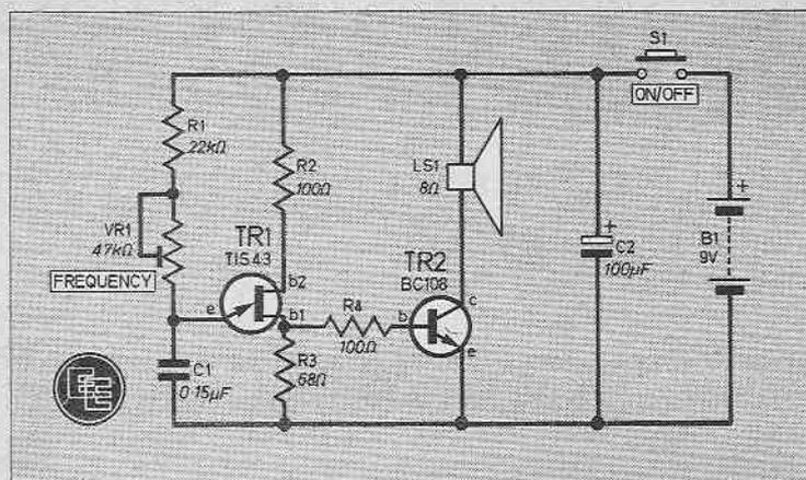
Fig. 1. Circuit diagram for the Audio Tone Generator.
