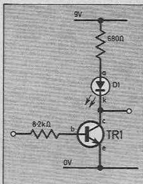
Fig. 8.7. If it is desired to drive a light emitting diode from one of our switches then the circuit shown can be used.
