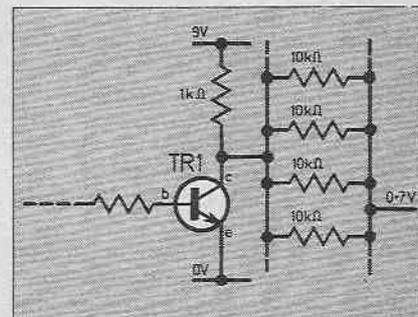
Fig. 8.5. The loading on the switch in Fig. 8.4 can be redrawn thus. The load appears as a number of 10kΩ resistors in parallel all to 0.7V.
