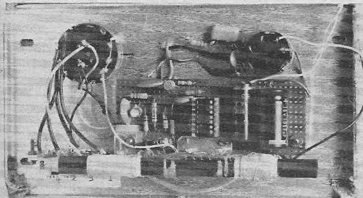
The fully wired chassis assembly with aerial secured to board.
