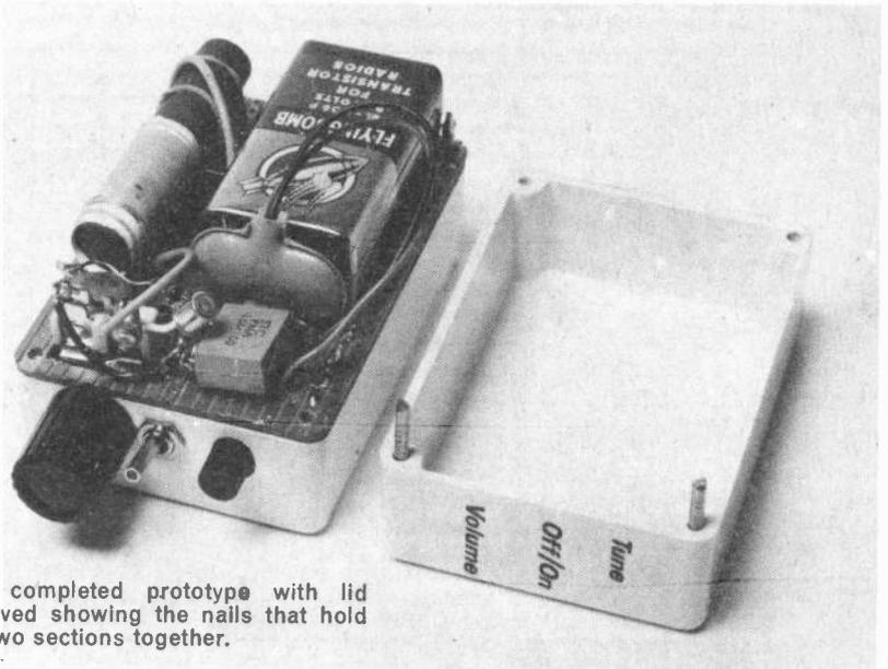
The completed prototype with lid removed showing the nails that hold the two sections together.
