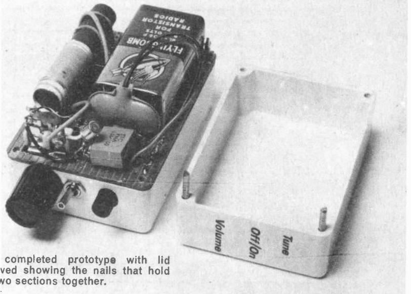
The completed prototype with lid removed showing the nails that hold the two sections together.
