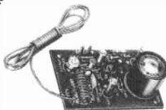
**KS200 MINIATURE F.M. TRANSMITTER.** 88-108MHz complete with dynamic microphone, operates from 9V D.C. (PP3), semiconductors 2N708 & BC208-B. Not Licenceable in U.K. £7.57 inc VAT
