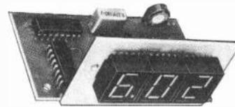
**KS420 DIGITAL VOLTMETER.** 3 Digit .75 Inch L.E.D display ranges 0-999mV-0.9-99V-0.99-9V-0.999V, uses 2 x CA3162E I.C. & 3 x BC307 semiconductors, operates from 5V D.C. £19.38 inc VAT
