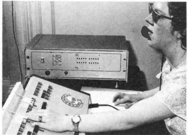
the position of keys indicates the Operator's actions. With this information the system is able to follow an Operator's progress through the handling of each call.
