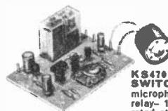
**KS470 SOUND OPERATED SWITCH.** Complete with dynamic microphone, adjustable sensitivity, relay-1 pole change over contracts rated at 5 amp, operates from 9-12V D.C. semiconductors 2 x BC208 & 1 x I.C. 741. **£11.22 inc VAT**
