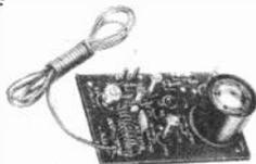
**KS200 MINIATURE F.M. TRANSMITTER.** 88-108MHz complete with dynamic microphone, operates from 9V D.C. (PP3), semiconductors 2N708 & BC208-B. Not Licenceable in U.K. **£7.37 inc VAT**
