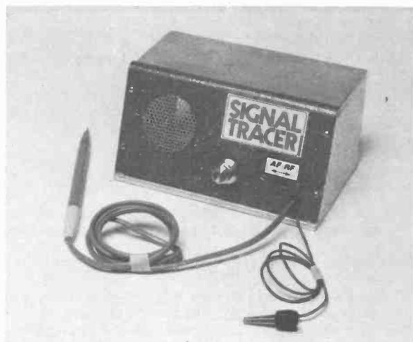
Exterior of the completed unit showing earth lead and probe in foreground.
