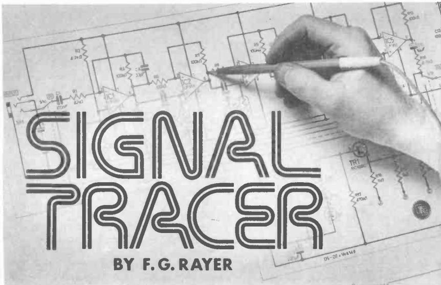
A QUICK means of locating faults in radio frequency, intermediate frequency and audio frequency stages of receivers, or in amplifiers used with microphone, pick-up or other input, is to use a signal tracer. The tracer described here can be switched at once for r.f. or a.f. circuits, and has enough sensitivity for low signal levels.
