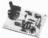
**KS100 MINIATURE V.H.F./A.M./F.M. RECEIVER.** Varicap tuned, 88-108 MHz earphone output 240mV, sensitivity 1uV, operates from 9V D.C. (PP3) 2.5mA semiconductors EET/E300 & BC205-G. **£5.31 inc VAT**
