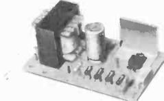
**KS490 "NICAD BATTERY CHARGER".** Constant current in five ranges, 10-20-45-100-150mA. Max. charge voltage 15V. Operates from 240V A.C. **£9.82 inc VAT**
