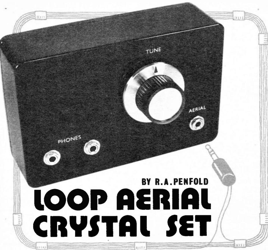
**A**LTHOUGH a crystal set does have advantages over other types of receiver, such as low cost, simplicity, and no running costs, unfortunately there are also drawbacks to this type of receiver. The main ones are the need for a longwire aerial in order to obtain an adequate signal pick-up, and the low output level which is only sufficient to drive an efficient pair of headphones or earpiece.
