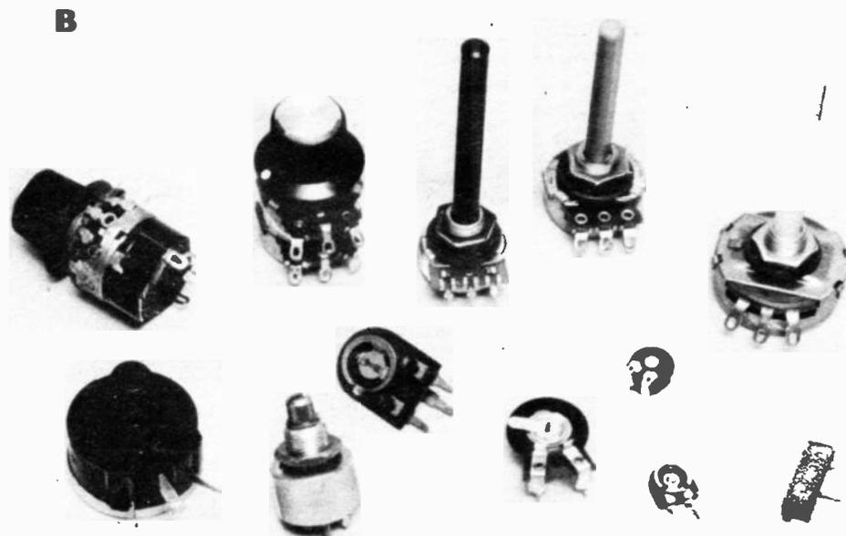
**B** A selection of potentiometers. In the front row we can see several preset types. On the far left is an old-fashioned enclosed type once common in TV sets, then a more modern enclosed type. After that is a vertical mounting skeleton preset followed by a similar horizontal mounting type. Just above that is a sub-miniature sealed trimmer below which is a miniature vertical skeleton preset. Finally on the right is a multi-turn trimmer.
