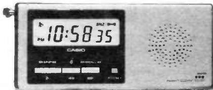
Large LC Display of full digital time. Symphonic alarm (Mozart, No. 40), or buzzer, with snooze facility. Hourly time signal option. Integral speaker and amplifier. Rapid setting. Accuracy +/- 15 secs/month. One lithium battery lasts approx. 12 months. Dims: 9.3 × 108 × 48mm. (1 1/4 × 4 1/4 × 1 7/8"). 53g (1.9oz).
