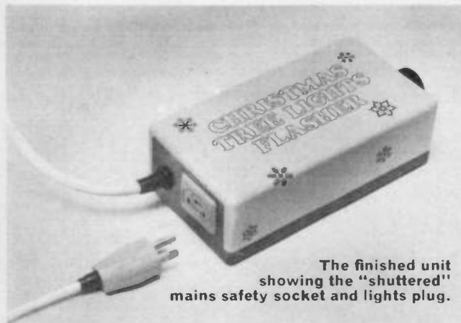
The finished unit showing the "shuttered" mains safety socket and lights plug.
