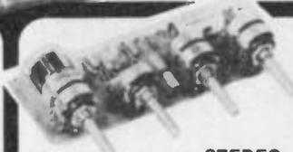
The PA200 is basically our popular PA100 modifications being made to make it compatible with the higher output amplifiers i.e. AL120 & AL250. The unit boasts six push button selectors giving a choice of 3 inputs, 2 filters, for both high and low frequencies and a stereo or mono button, all combining to give a top quality stereo pre-amplifier and tone control.
