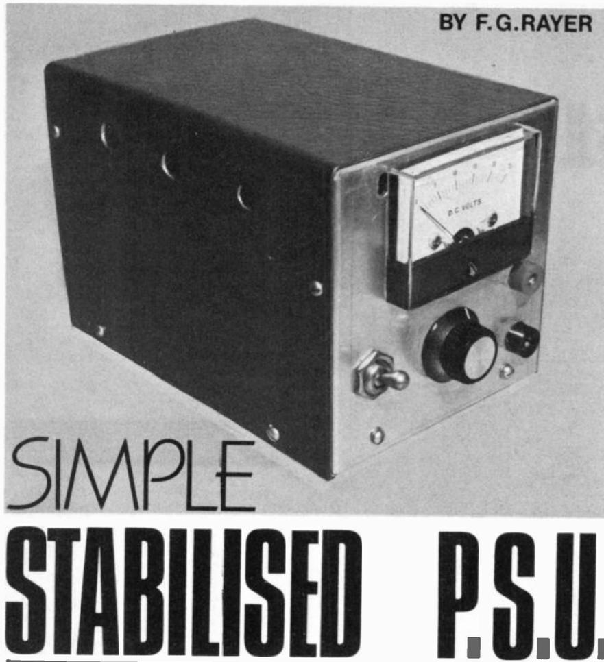
There is no doubt that a regulated and adjustable power supply unit is of immense utility to the constructor and experimenter of electronic projects. Some thought has been given to easing constructional work to make this project suitable for the beginner. Regulation is so good that if wished the cost can be reduced by omitting the meter—but more about this later. Output voltage is 1.2V to 20V at currents up to 1 ampere, adequate for very many purposes.
