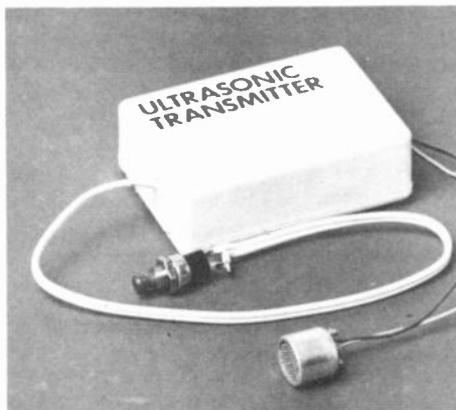
The finished Ultrasonic Transmitter with remotely wired transducer and switch.
