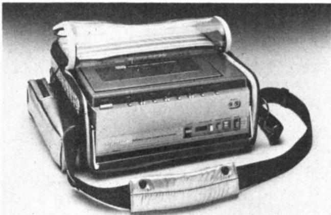
too. Most video recorders provide an audio dub facility which replaces the original sound track with new sound, but the VT6500 goes a stage better by enabling the user to blend new sound material with the original sound track and not replace it, although this is still possible.
