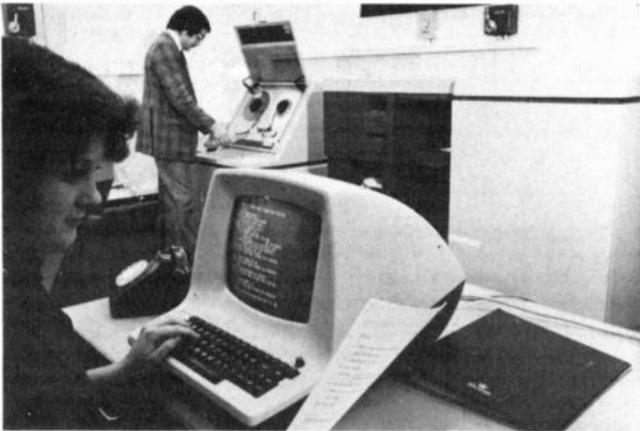
A London operator keys in customer's identification to be transmitted to the computer in Manchester. Meanwhile, magnetic tape containing the customer's mailing list is loaded into the computer prior to transmission
