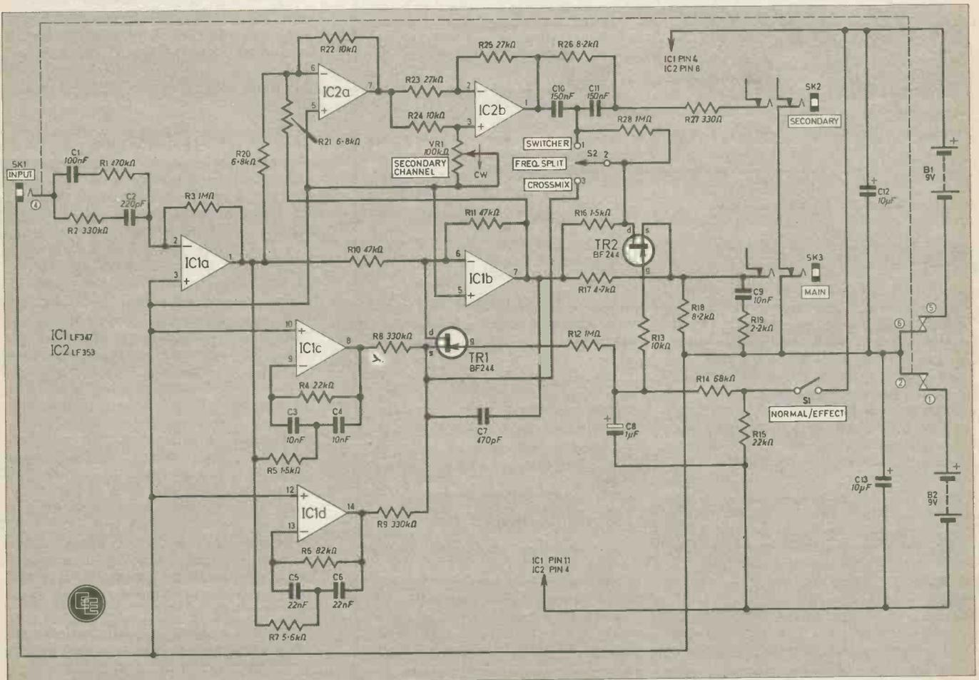
CROSSMIX mode is selected thus preventing bass signals from the main output getting into the secondary output. R27 is included to isolate the output of the op-amp from cable capacitance which could otherwise cause instability.
