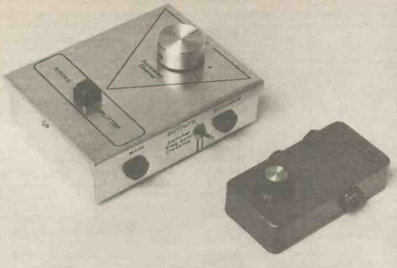
Prototype Sound Splitter and Two-Way Remixer,
