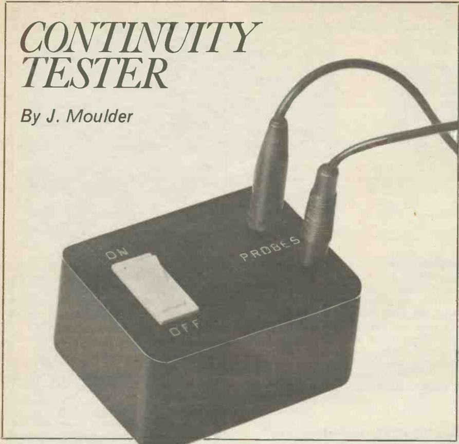
A CONTINUITY tester is a valuable piece of equipment used to determine whether a component or circuit has a broken connection. That is, it tests for the continuity of current flowing.
