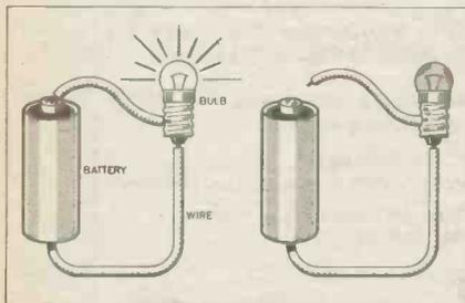
Fig. 1. Demonstration of current flow.
