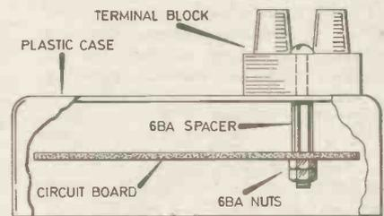
Fig. 3. A suggested method of mounting the component board in the case.
