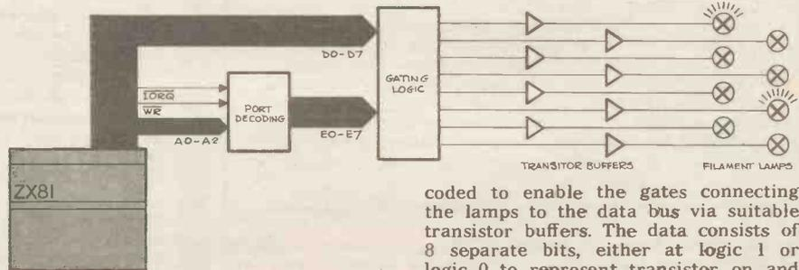
The existing software commands the computer to repeatedly send data to a particular port number, 0C. The port number appears on the lower half of the address bus at this time and is de-
