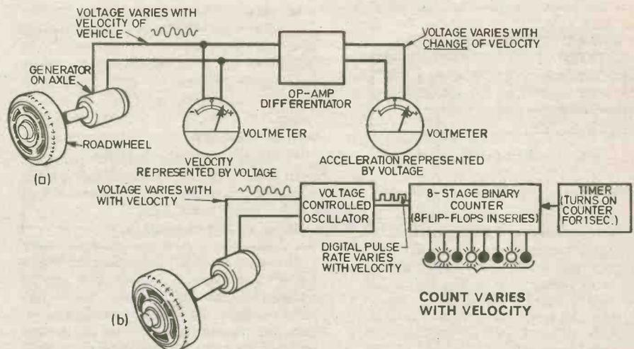
Fig. 12.8. Analogue and digital quantities. (a) a wholly analogue system using an analogue computer (b) analogue input converted to digital form. The digital output can be fed to a digital computer to calculate other quantities (for example, acceleration).
