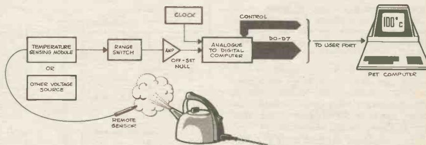
clocked into the chip to provide a digital representation of the input voltage level in the form of an 8-bit word (eight binary bits). The number of samples taken is dependent on the clock rate which has been selected to give a conversion rate of 28,000/sec. The 8-bit wide information reaches the microcomputer data bus when enabled by a command from the software.
