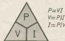
Fig. 3. Power equation triangle.
