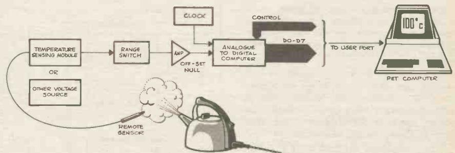
clocked into the chip to provide a digital representation of the input voltage level in the form of an 8-bit word (eight binary bits). The number of samples taken is dependent on the clock rate which has been selected to give a conversion rate of 28,000/sec. The 8-bit wide information reaches the microcomputer data bus when enabled by a command from the software.
