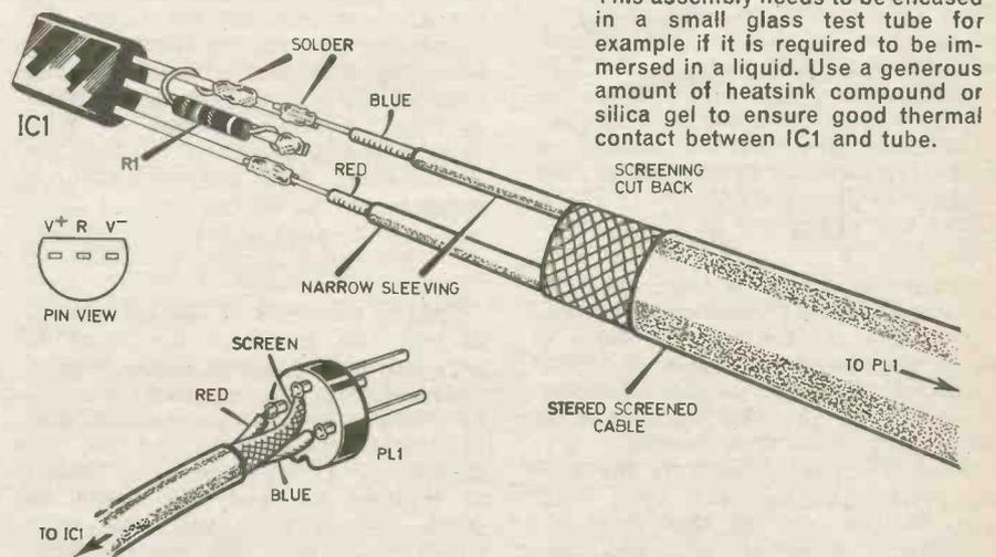
This assembly needs to be encased in a small glass test tube for example if it is required to be immersed in a liquid. Use a generous amount of heatsink compound or silica gel to ensure good thermal contact between IC1 and tube.
