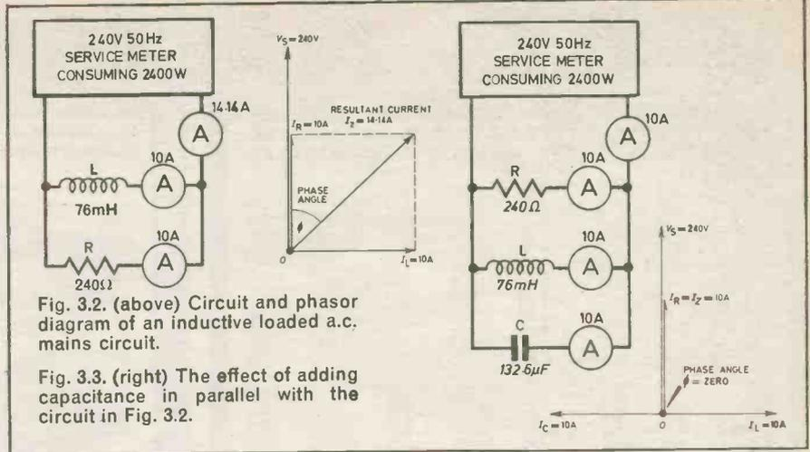
Fig. 3.2. (above) Circuit and phasor diagram of an inductive loaded a.c. mains circuit.
