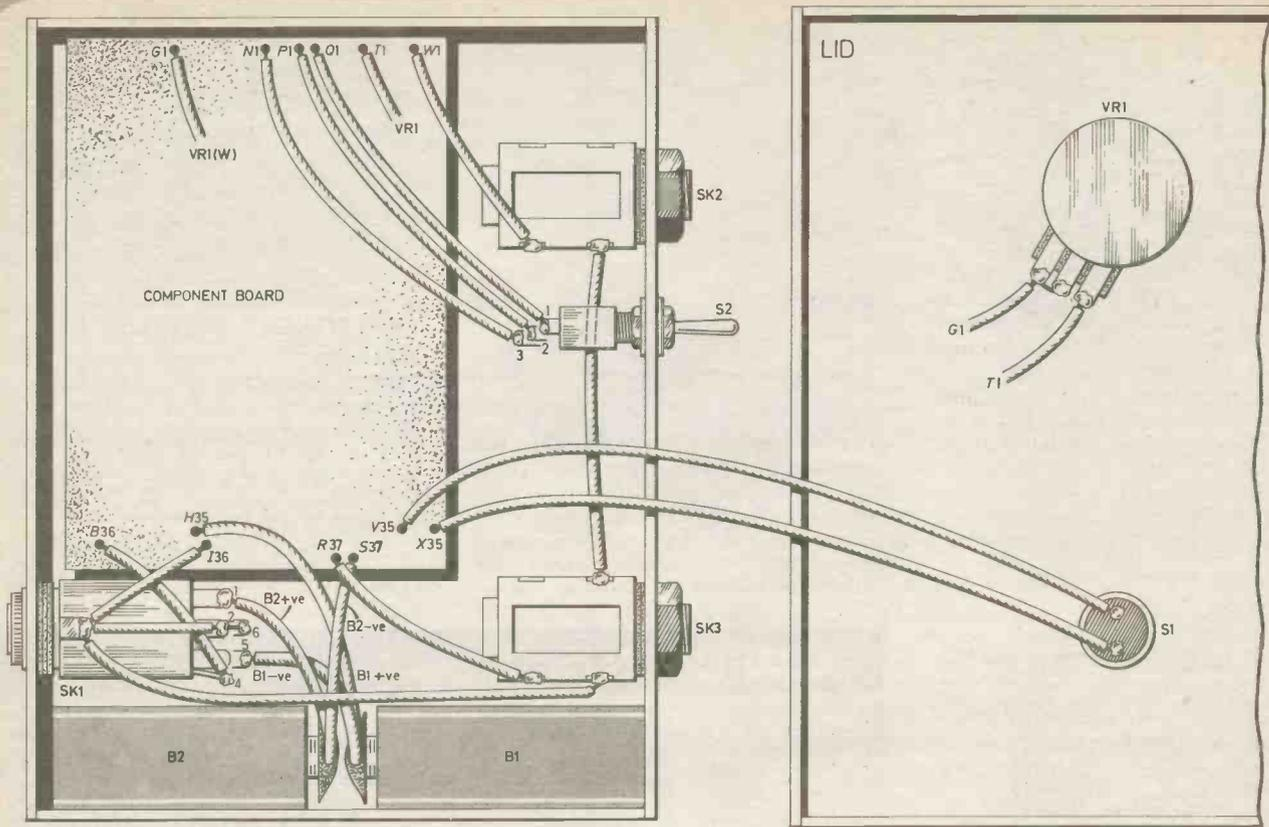
Fig. 5. Complete interwiring details.
