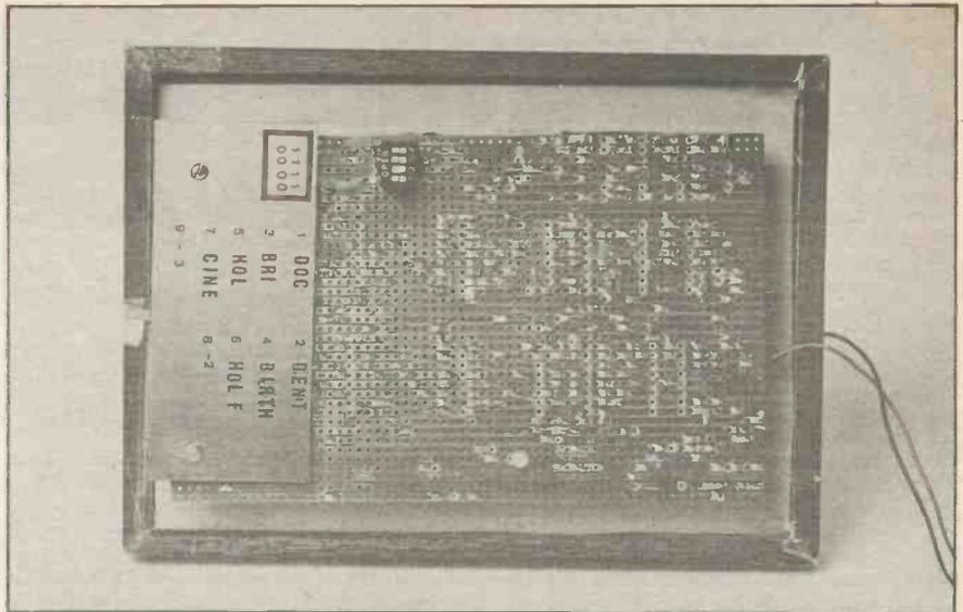
Rear view of the framed Monthly Planner showing the position of d.i.l. switches S3 to S6. An additional board was fixed to the rear of the prototype unit to show the codes for each event (given here as a decimal number). Note the use of the nylon screw in hole //26.
