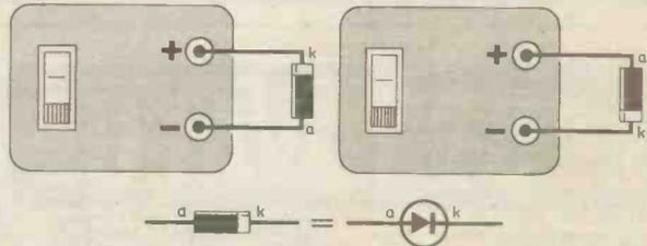
Fig. 3. Method of testing a diode with the Continuity Tester unit. If the cathode (k) is first connected to the positive (red) terminal as shown, the diode should not conduct. By reversing the diode across the terminals as shown in the right hand diagram, the tone should sound, indicating conduction. If the tone sounds for both tests or does not sound at all, then the diode is defective.
