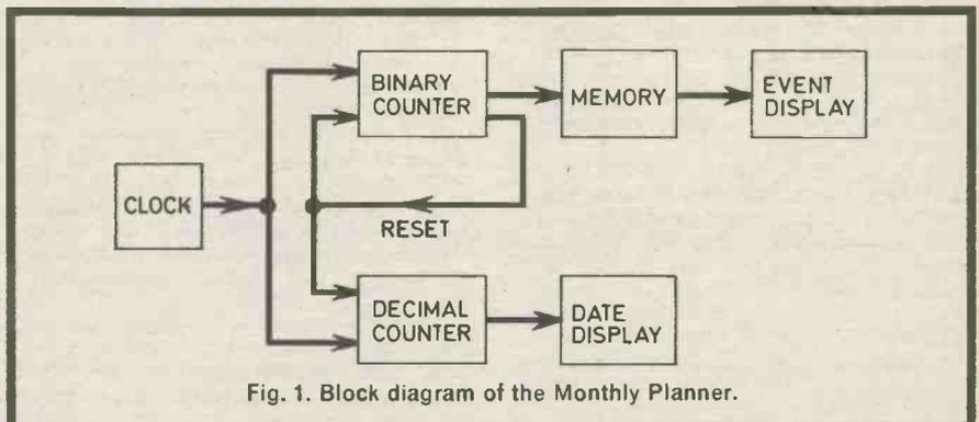
Fig. 1. Block diagram of the Monthly Planner.
