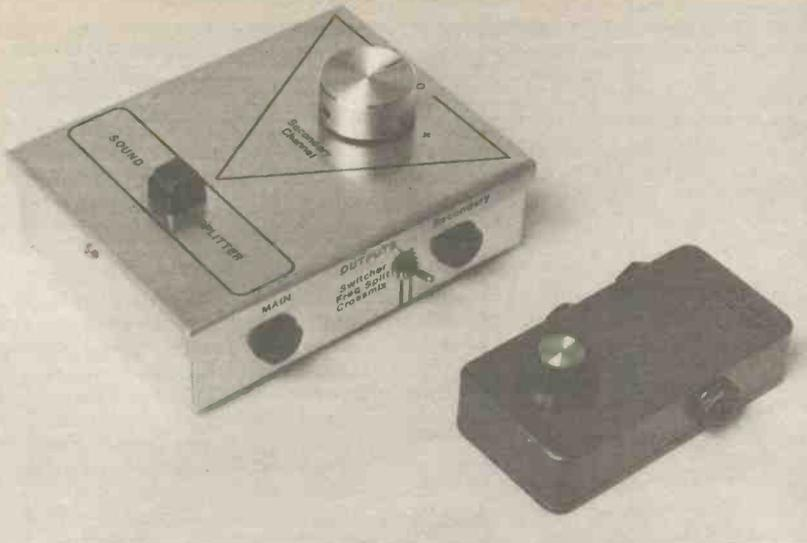
Prototype Sound Splitter and Two-Way Remixer,
