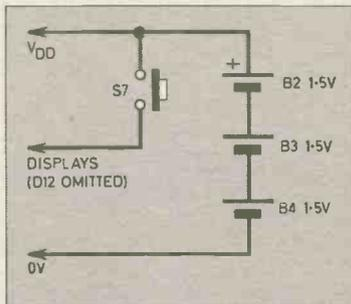
Fig. 4. Optional battery only power supply. The display is enabled with S7.
