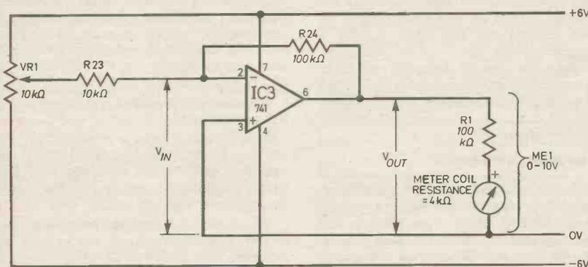
Fig. 12.1. Using an op-amp as an inverting amplifier. Offset null compensation is not essential and is omitted. You could connect up this circuit on *Minilab* and test its action. For positive input voltages from  $VR_1$ , reverse the connections to the meter.
