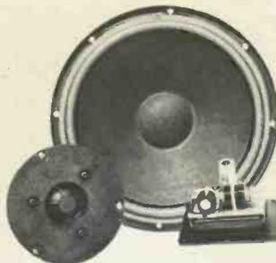
**12" 80 watt R.M.S. loudspeaker.** A superb general purpose twin cone loudspeaker. 50 oz. magnet, 2" aluminium voice coil. Rolled surround. Resonant frequency 25Hz. Frequency response to 13KHz. Sensitivity 95dB. Impedance 8ohm. **Attractive blue cone with aluminium centre dome.**
