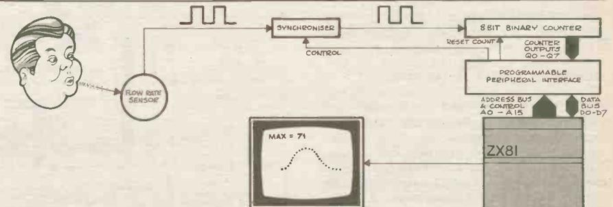
portional to the applied pressure. Internal Hall effect switches in the sensor produce a train of pulses at its output. The pulse rate is thus proportional to the applied pressure.
