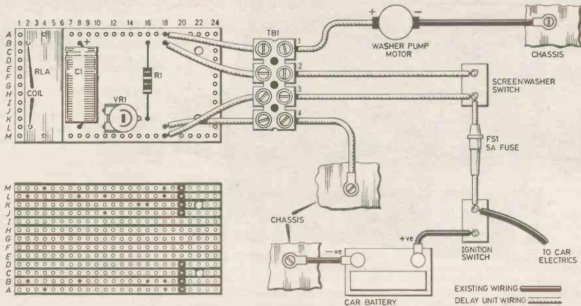
Fig. 2. Layout of the components on the stripboard, breaks to be made on the underside and wiring details to the existing car electrics.
