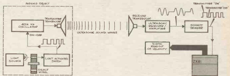
source on one side of the wheel and a light activated switch on the other. As the trolley moves, the light activated switch operates and turns the ultrasonic oscillator on. The on-to-off rate of the ultrasonic transmitter is therefore proportional to the velocity of the trolley. The transmitter on and off periods are
