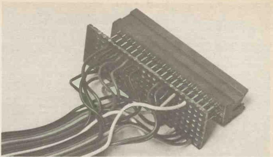
The stripboard/edge connector fully wired. The two outermost connector positions should be fitted with inserts to act as alignment guides.
