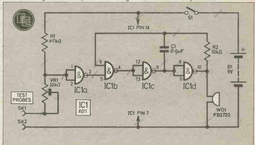
Next, the flying leads of 7/0.2mm equipment wire should be added, and these should be about 100mm long. Finally solder the leads from the piezo ceramic transducer into position, taking great care as these tend to be a little fragile, and to complete this stage of construction, add the battery clip (remember that the red lead goes to switch S1).
