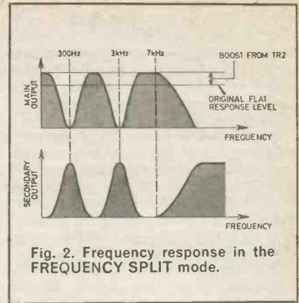
Fig. 2. Frequency response in the FREQUENCY SPLIT mode.
