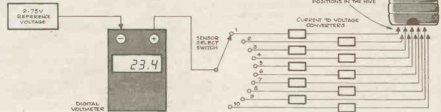
voltage directly proportional to the absolute temperature ( $^{\circ}\text{K}$ ). The output voltage obeys a linear relationship with temperature and is equal to  $10\text{mV}/^{\circ}\text{K}$ . On board calibration circuitry provides an accuracy of  $1^{\circ}\text{K}$ .
