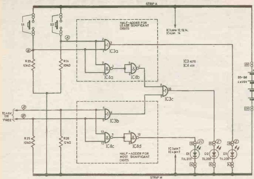
Fig. 12.11. Logic diagram of a 2-digit full adder.
