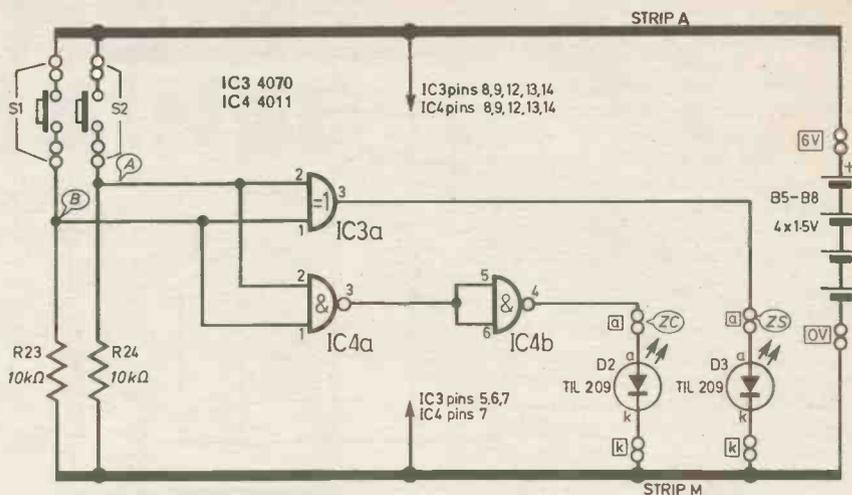
Fig. 12.9. Circuit of a half-adder.
