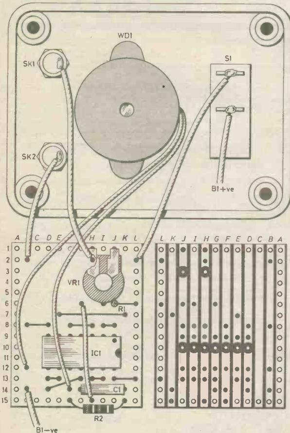
Fig. 2. Stripboard layout and inter-wiring diagram.
