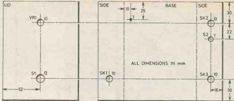
Fig. 6. Case drilling details.
