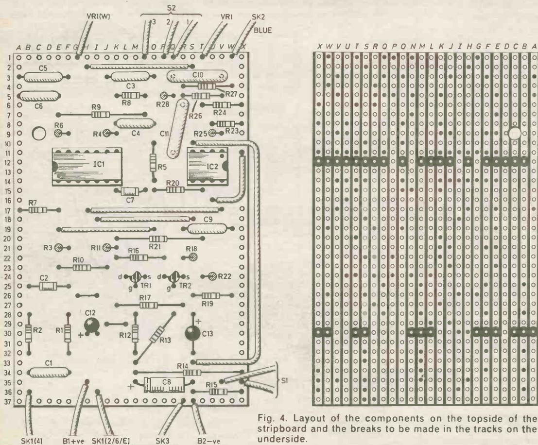
Fig. 4. Layout of the components on the topside of the stripboard and the breaks to be made in the tracks on the underside.
