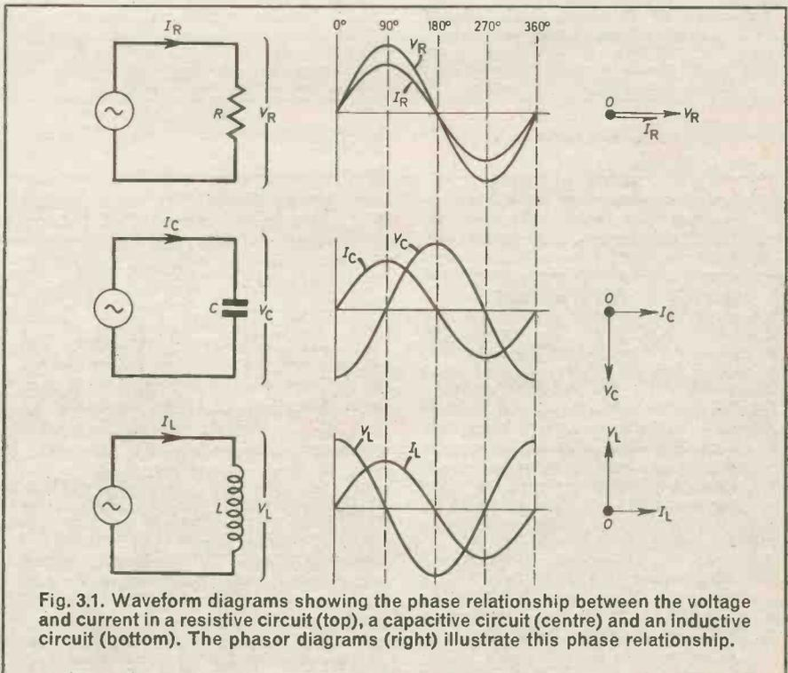
Fig. 3.1. Waveform diagrams showing the phase relationship between the voltage and current in a resistive circuit (top), a capacitive circuit (centre) and an inductive circuit (bottom). The phasor diagrams (right) illustrate this phase relationship.
