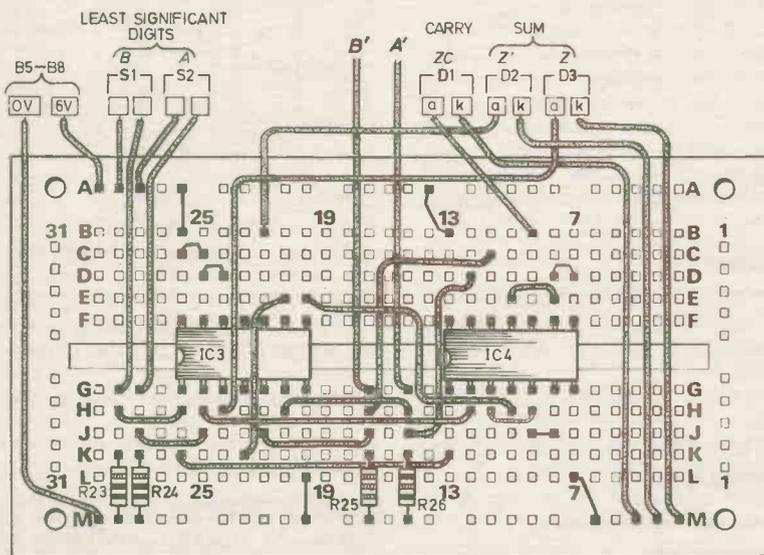
Fig. 12.12. The layout of the components on the Verobloc for the circuit of Fig. 12.11.
