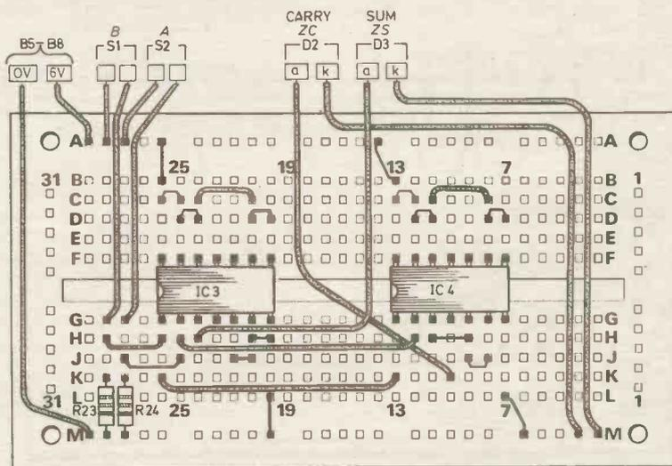
Fig. 12.10. The layout of the components on the Verobloc for the circuit in Fig. 12.9. Unused inputs are connected to 0V or +6V so that the i.c.s operate correctly.
