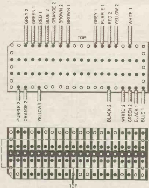
Fig. 8. Wiring and connection details to the strip-board holding the 22 + 22 way edge connector. The labelling of the wires assumes that two 10-way ribbon cables have been used, called 1 and 2.
