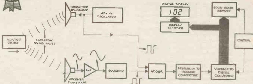
The circuitry computes the difference in transmitted and reflected frequencies to calculate the speed of the object.
