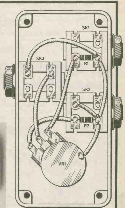
Fig. 8. Layout and wiring of the Remixer components in the diecast aluminium box.
