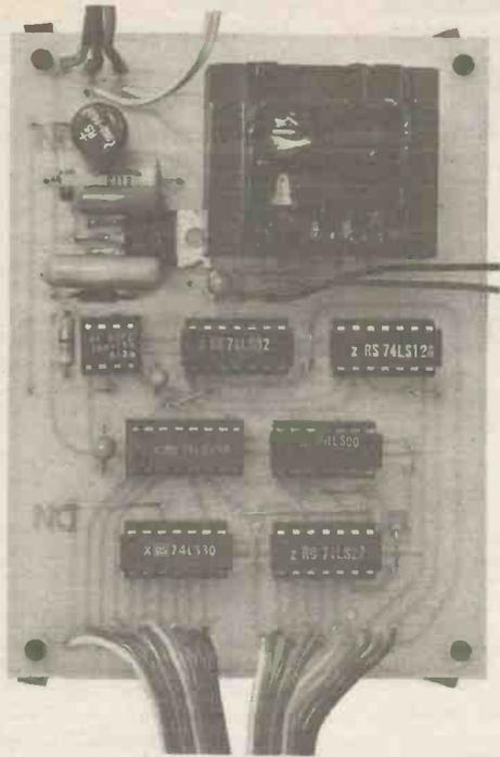
Above and below. Shows the assembled prototype p.c.b. fitted with the snap-fixing stand-off pillars.
