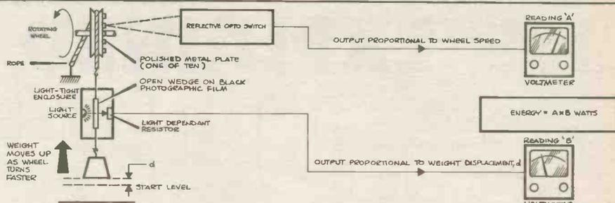
mined using an optical method. An l.e.d. was situated on one side of a photographically produced and calibrated clear wedge on black film. On the other side of the film was a light dependent resistor. The assembly was mounted in a light-tight box. The film was attached to the rope. As the rope was made to lift the mass, the film
