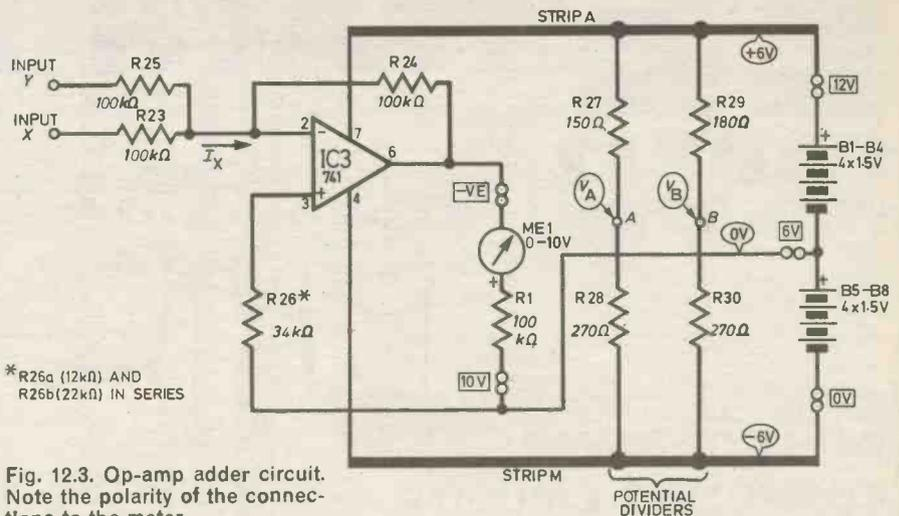
Fig. 12.3. Op-amp adder circuit. Note the polarity of the connections to the meter.
