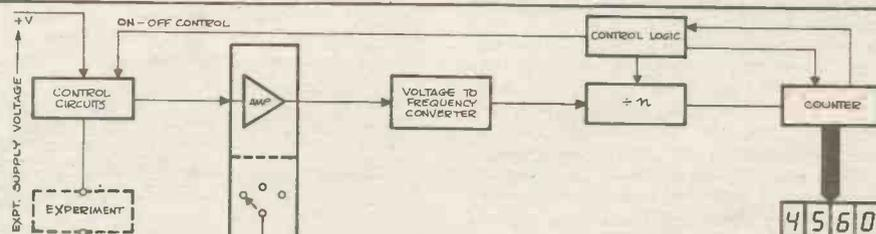
to/from a preset value. When the preset value is reached, the unit switches off power to the experimental apparatus.
