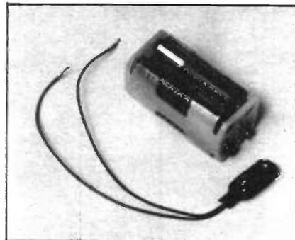
Fig. 1.1. A suitable battery holder fitted with 4 × 1.5V (type AA) cells. Also shows battery clip with flying leads.
