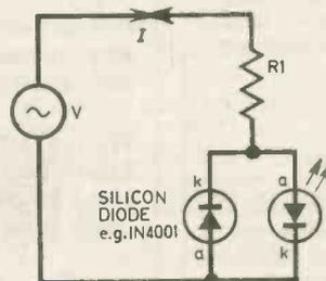
Fig. 2. A.c. circuit. Reverse current is removed from the l.e.d. by a silicon diode.
