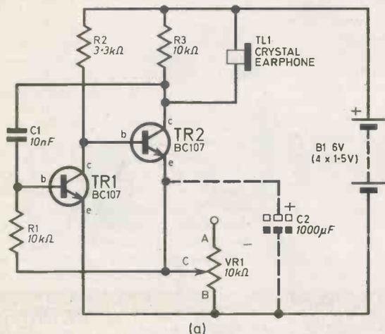
(a) Fig. 4.6(a). A simple circuit to produce intermittent oscillations. When C1 is removed, the circuit acts as a white noise generator and amplifier.
