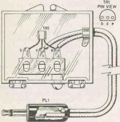
Fig. 4. Assembly of the phototransistor unit. Note that the curved face of TR1 is photosensitive.
