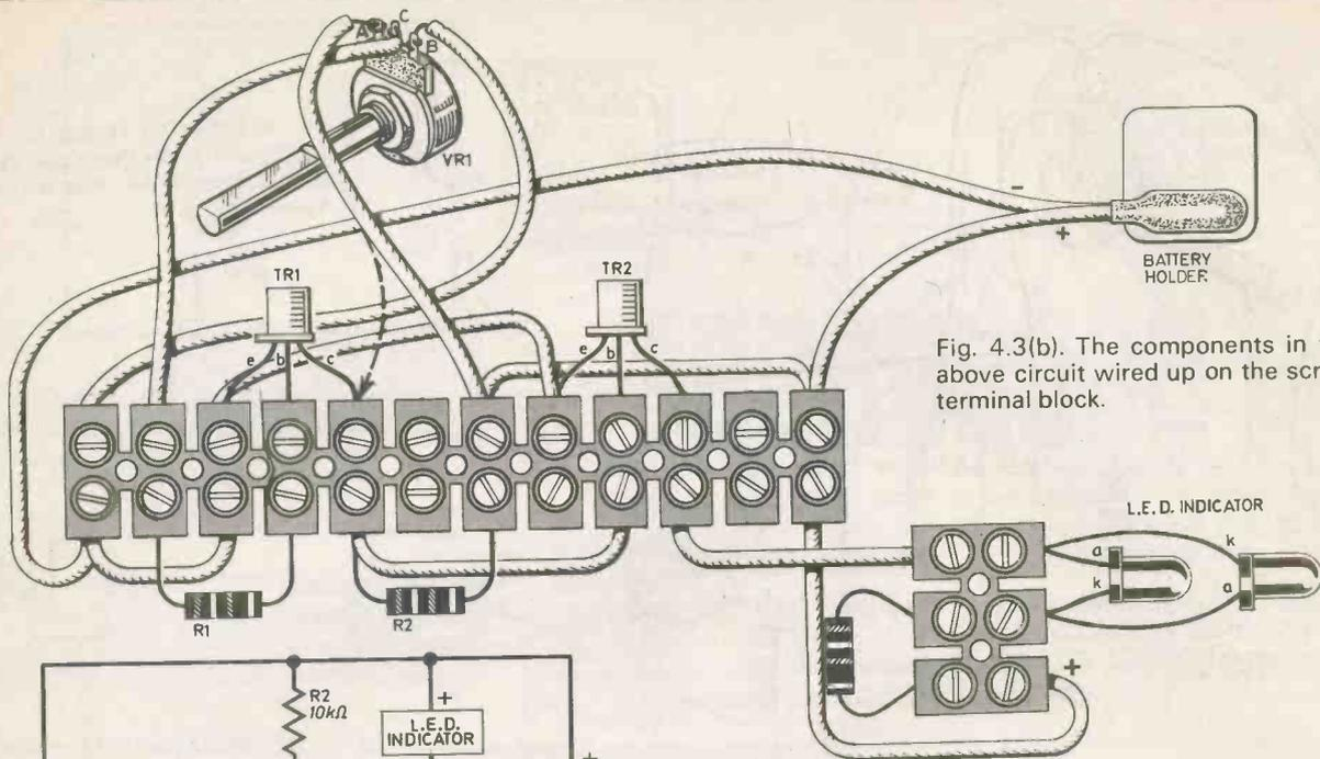
Fig. 4.3(b). The components in the above circuit wired up on the screw terminal block.
