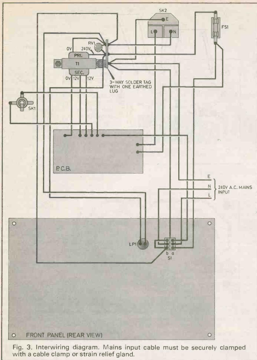
Fig. 3. Interwiring diagram. Mains input cable must be securely clamped with a cable clamp or strain relief gland.
