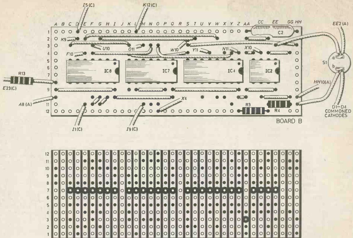
Fig. 3 (Above). The layout of the components on the topside of board B, the breaks to be made on the underside and interboard wiring details. Below shows the component layout and wiring details for board C and the breaks to be made on the underside. Also shown is the matrix of display i.e.d.s and complete wiring details to board C.
