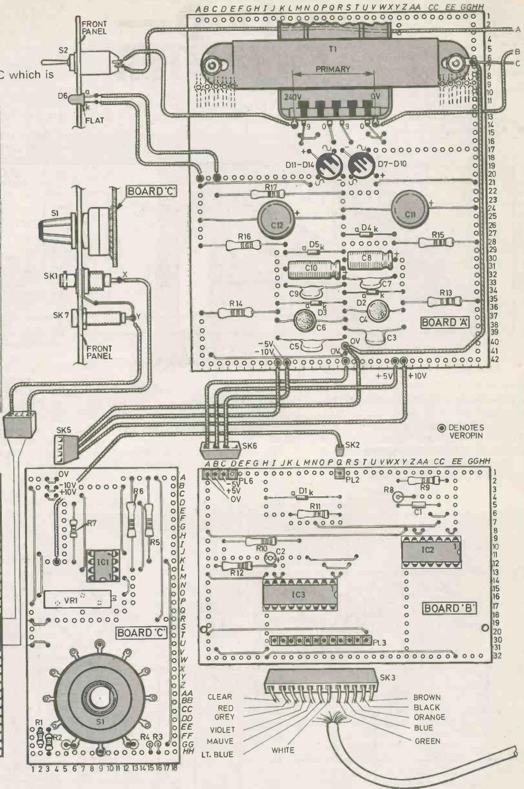
Fig. 3. (Above, top right, bottom right). Full layout and constructional and interwiring details of the A to D Converter and wiring up of the PET User Port connector.
