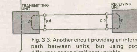
Fig. 3.3. Another circuit providing an information path between units, but using potential difference as the significant variable.
