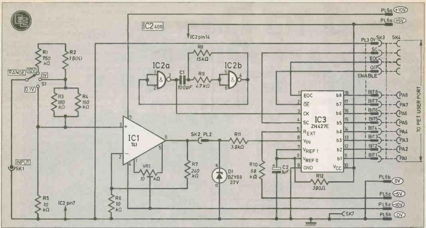
Fig. 1. Circuit diagram of the A to D Converter.
