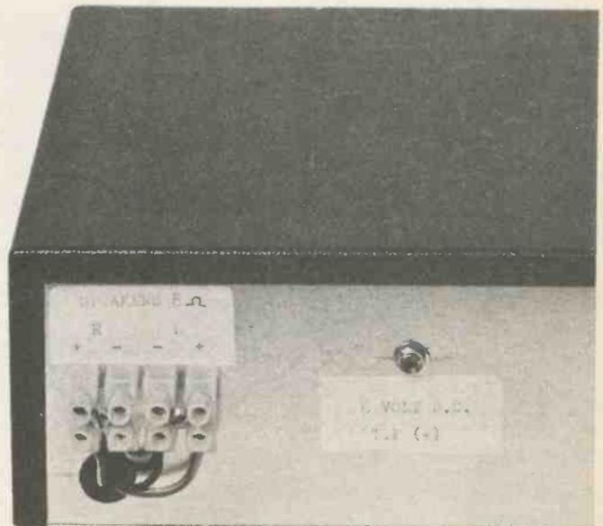
(Right). Close-up view of the screw terminal block and its label used for connecting to the two speakers.
