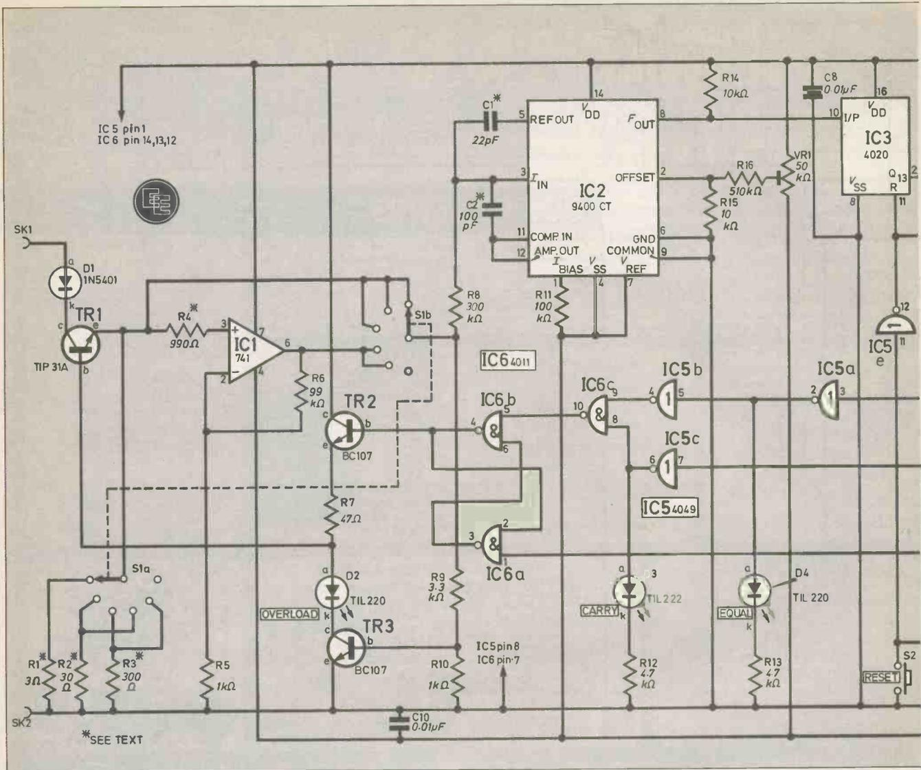
from the  $Q_{13}$  output (divide by  $2^{13}$ ). This is IC3 on the circuit diagram.
