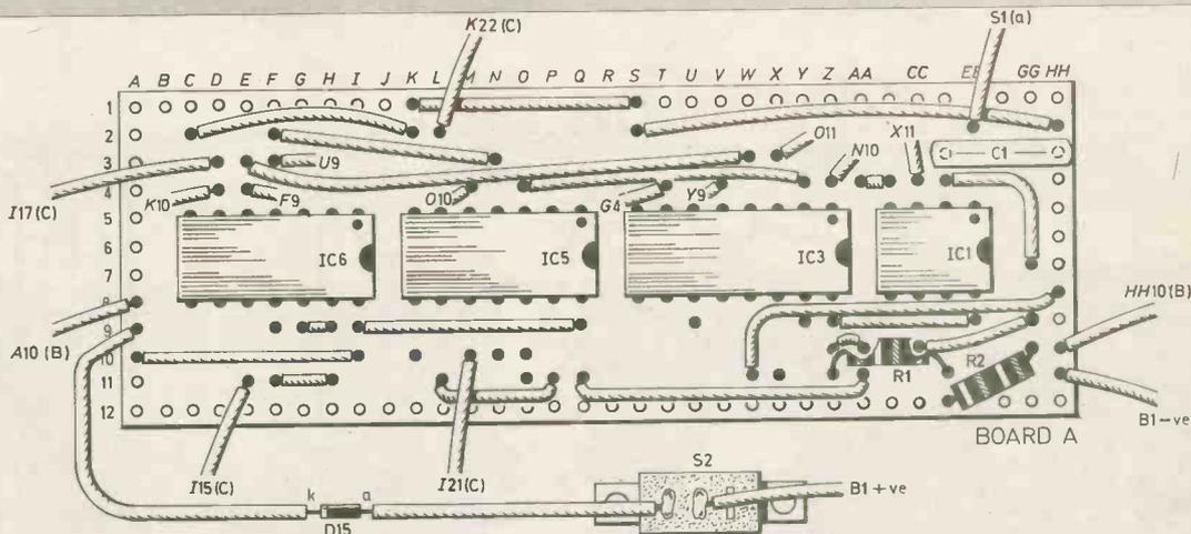
Fig. 2. The layout of the components on the topside of board A, breaks to be made in the strips on the underside and interboard wiring details. Letter in parenthesis indicates board destination of flying leads.
