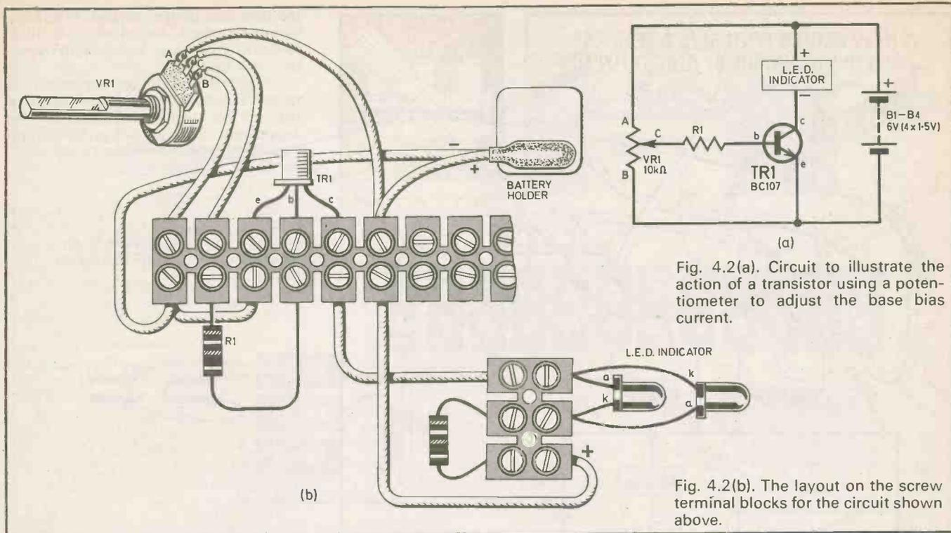
Fig. 4.2(a). Circuit to illustrate the action of a transistor using a potentiometer to adjust the base bias current.
