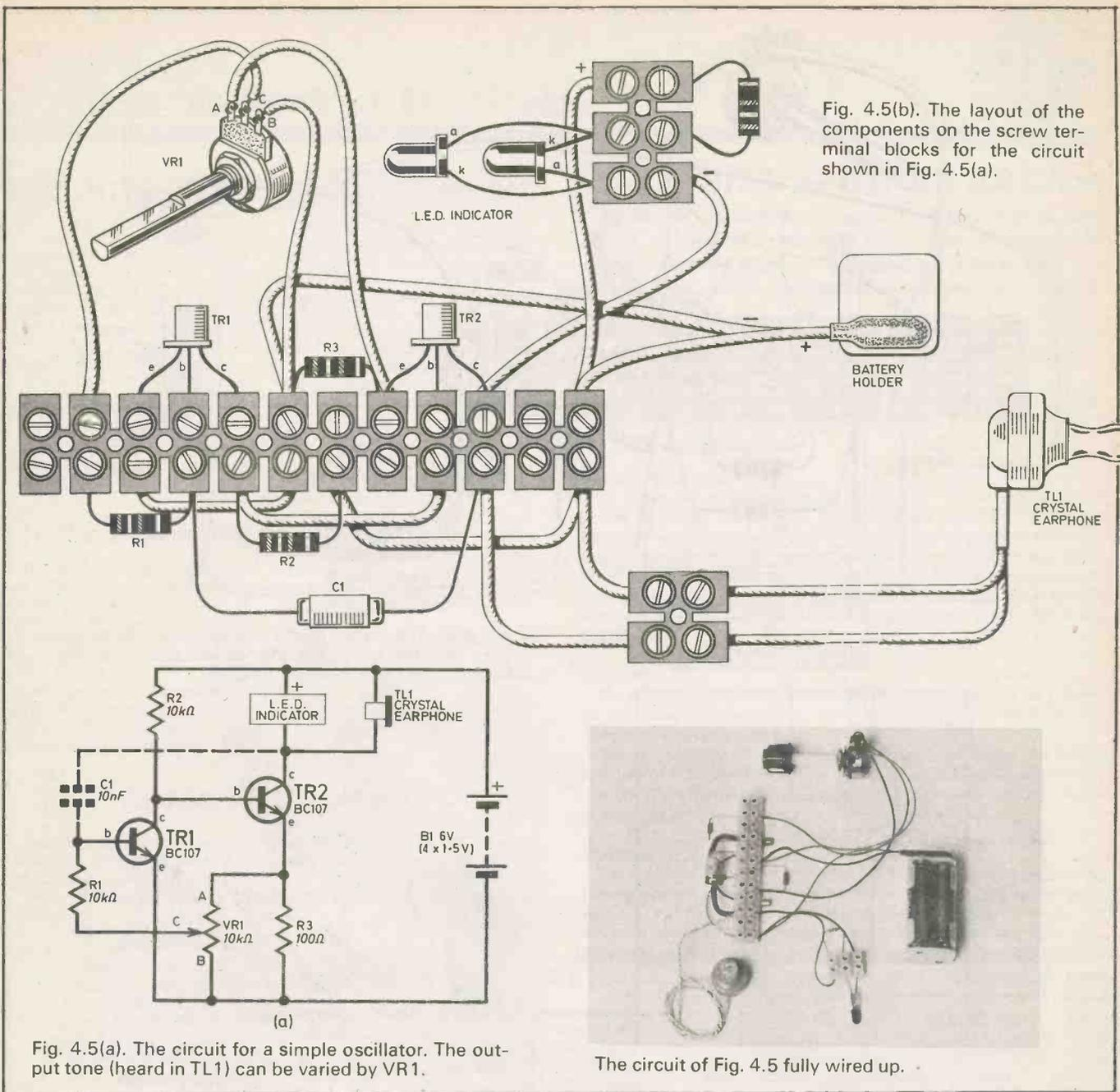
Fig. 4.5(b). The layout of the components on the screw terminal blocks for the circuit shown in Fig. 4.5(a).
