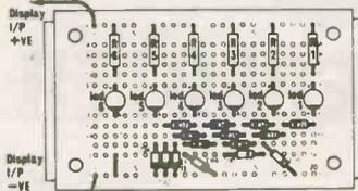
You will need: One EXP 300 or EXP 350 breadboard 15 silicon diodes 6 resistors 6 Light Emitting Diodes
