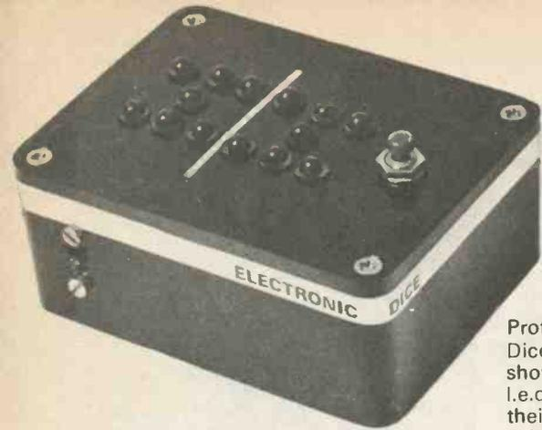
Prototype Double Dice clearly showing the l.e.d.s secured by their plastic fixing clips.
