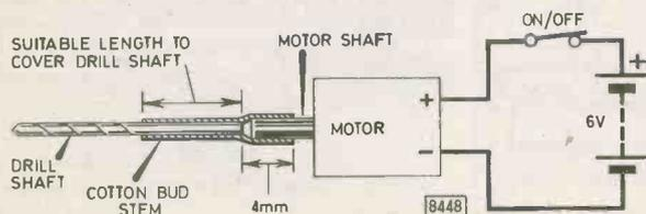
The prototype drill runs on four HP2 batteries in series, and can be used with drills up to 1.6mm diameter. It copes effortlessly with 1mm drills and has sufficient torque to drill holes up to 1.6mm diameter.
