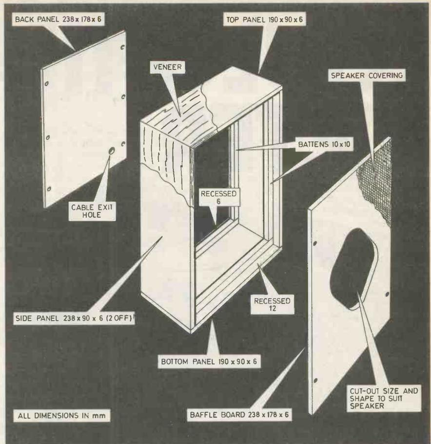
Fig. 5. An exploded view (dimensioned) of a suitable sized cabinet similar in size and shape to those seen in the photographs. This will accommodate the speakers (kit C) specified.
