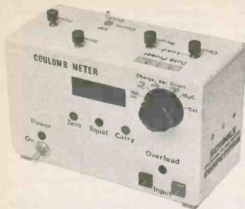
Finished Coulomb Meter showing the marking of the controls. Note how the unit has been designed for use in the classroom with the display visible from the front and controls accessible from the top. Photograph (right) shows the inside of the case and the use of spiral cable wrapping for neatness.
