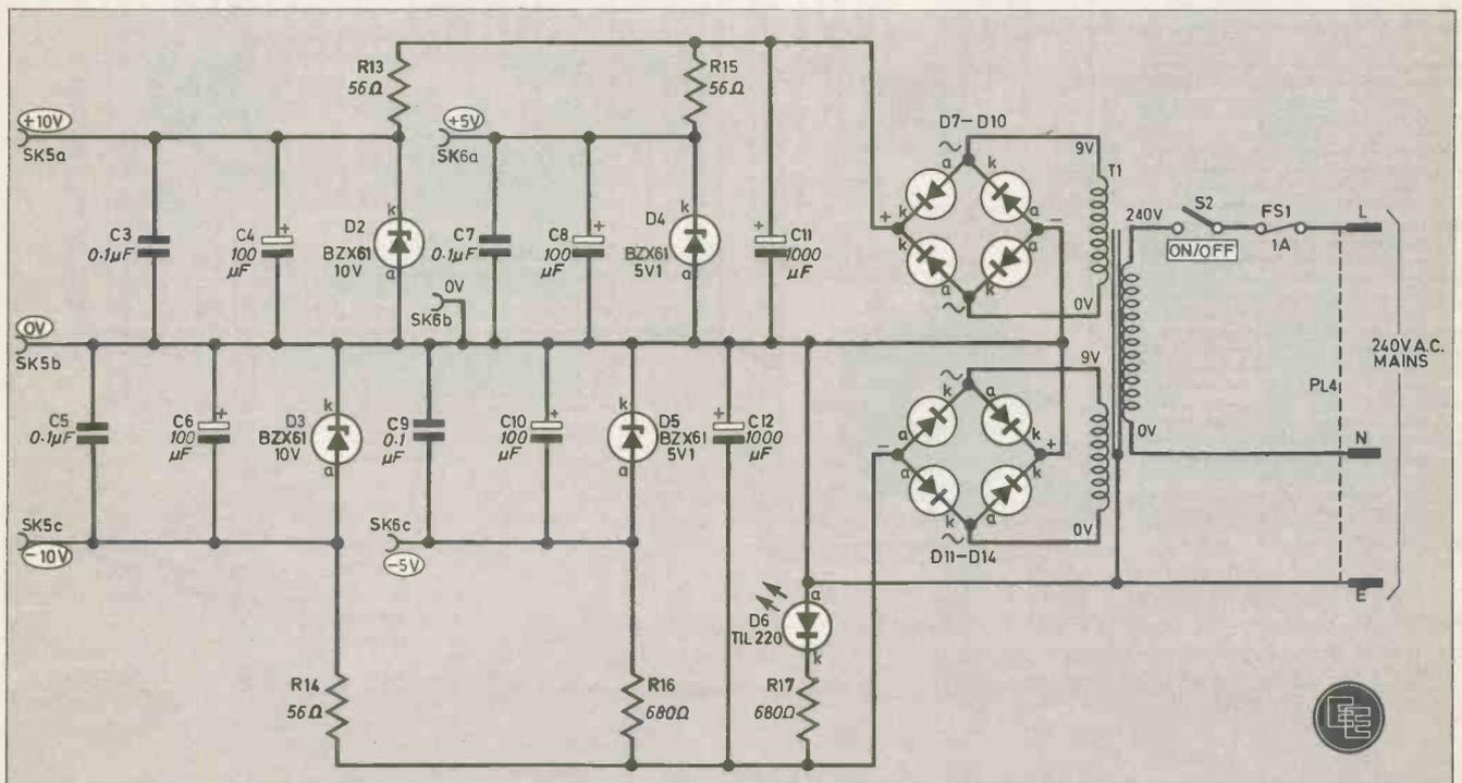
Fig. 2. Circuit diagram of the Power Supply section of the A to D Converter.
