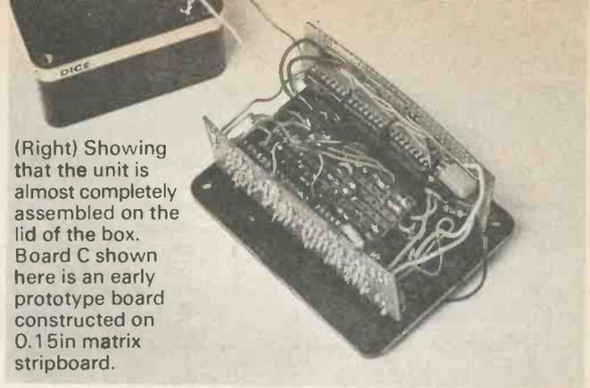
(Right) Showing that the unit is almost completely assembled on the lid of the box. Board C shown here is an early prototype board constructed on 0.15in matrix stripboard.
