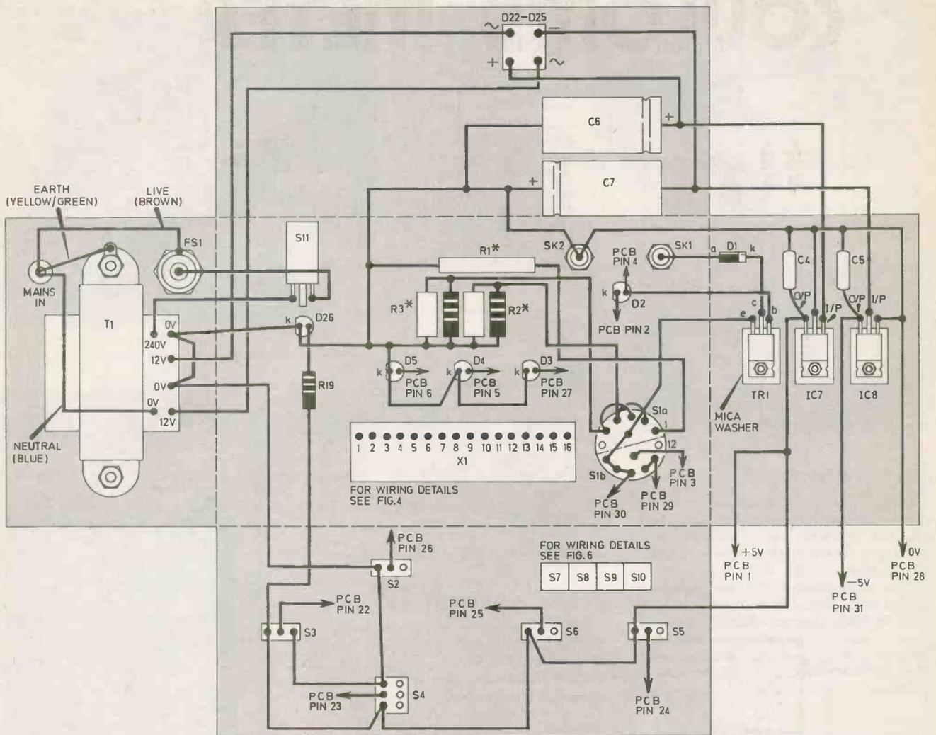
Fig. 5. Interwiring diagram. Note that discrete components are shown in relative positions only and should ideally be mounted on tag strips before being soldered. IC7, IC8 and TR1 must all be isolated from the case and mounted on mica washer insulating kits. See also Figs. 4 and 6 for wiring information of the display, X1 and the Data Preset switches, S7 to S10.
