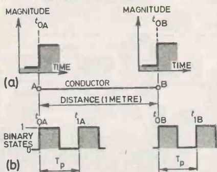
Fig. 3.1. Illustrating the difference between transmission time due to the physical nature of the medium—electrical conduction in the wire AB at (a)—and transmission time due to engineering parameters—such as the interval  $T_p$  between transitions in the binary data sequence (b). For convenience, time and distance scales are made to coincide at A and B.
