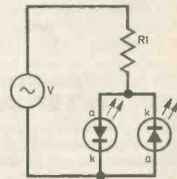
Fig. 3. Two-l.e.d. a.c. circuit. The l.e.d.s light alternately.
