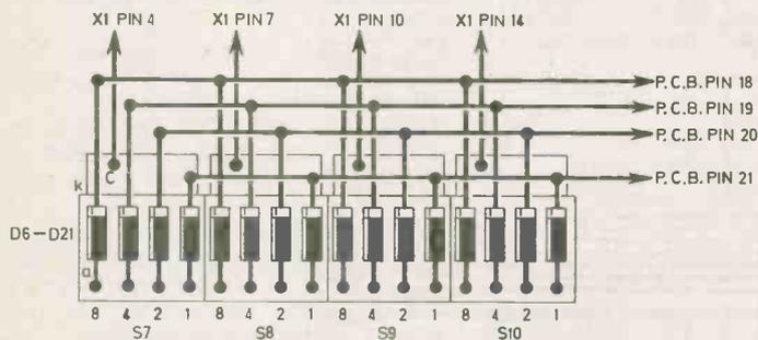
Fig. 6. Wiring of the Data Preset switches with cross-talk prevention diodes. The switches are actually mounted on a 0.1in. matrix stripboard, 24 holes by 5 strips (with suitable trackbreaks), but this has been omitted from this diagram for clarity.
