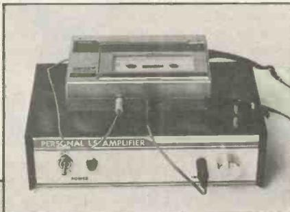
The "Personal" plugged into the Amplifier and powered by the 6V d.c. outlet socket.
