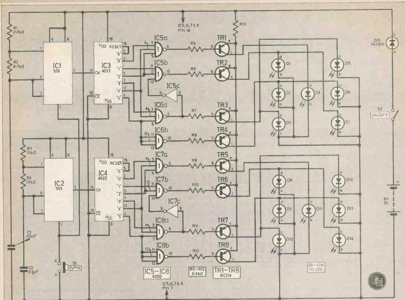
Fig. 1. The complete circuit diagram for the Double Dice.
