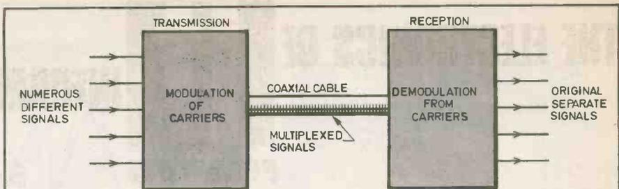
Fig. 3.4 (above). Basis of a carrier transmission system as used in telecommunications for multiplexing different signals on a common medium such as a coaxial cable (known as frequency division multiplex). For two-way transmission, modulation and demodulation of carriers is needed at both ends.
