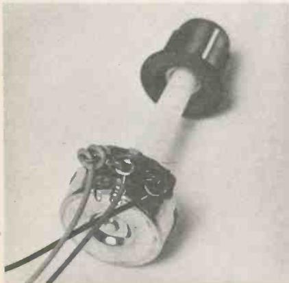
With VR1 slider at B the Indicator l.e.d. lights. As the control is turned clockwise (C moving towards A) the l.e.d. suddenly goes out. This is the reverse of what happens in the circuit of Fig. 4.2 where clockwise rotation turns the l.e.d. on.
