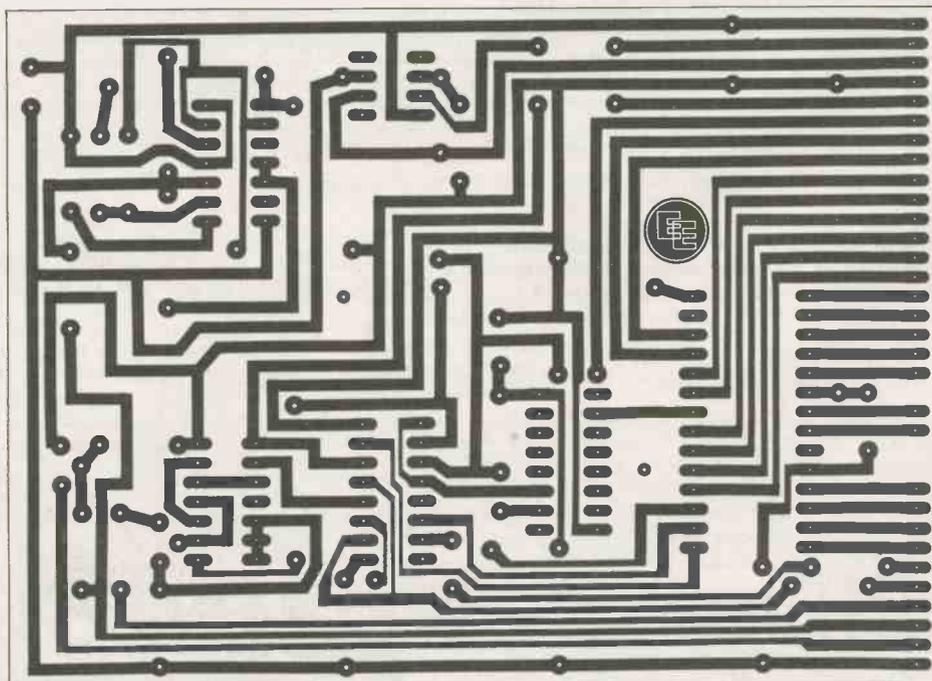
Fig. 4. Full size printed circuit board artwork and component layout for the Coulomb Meter. Note the use of sleeved wire for the long links and Veropins for all wired connections.
