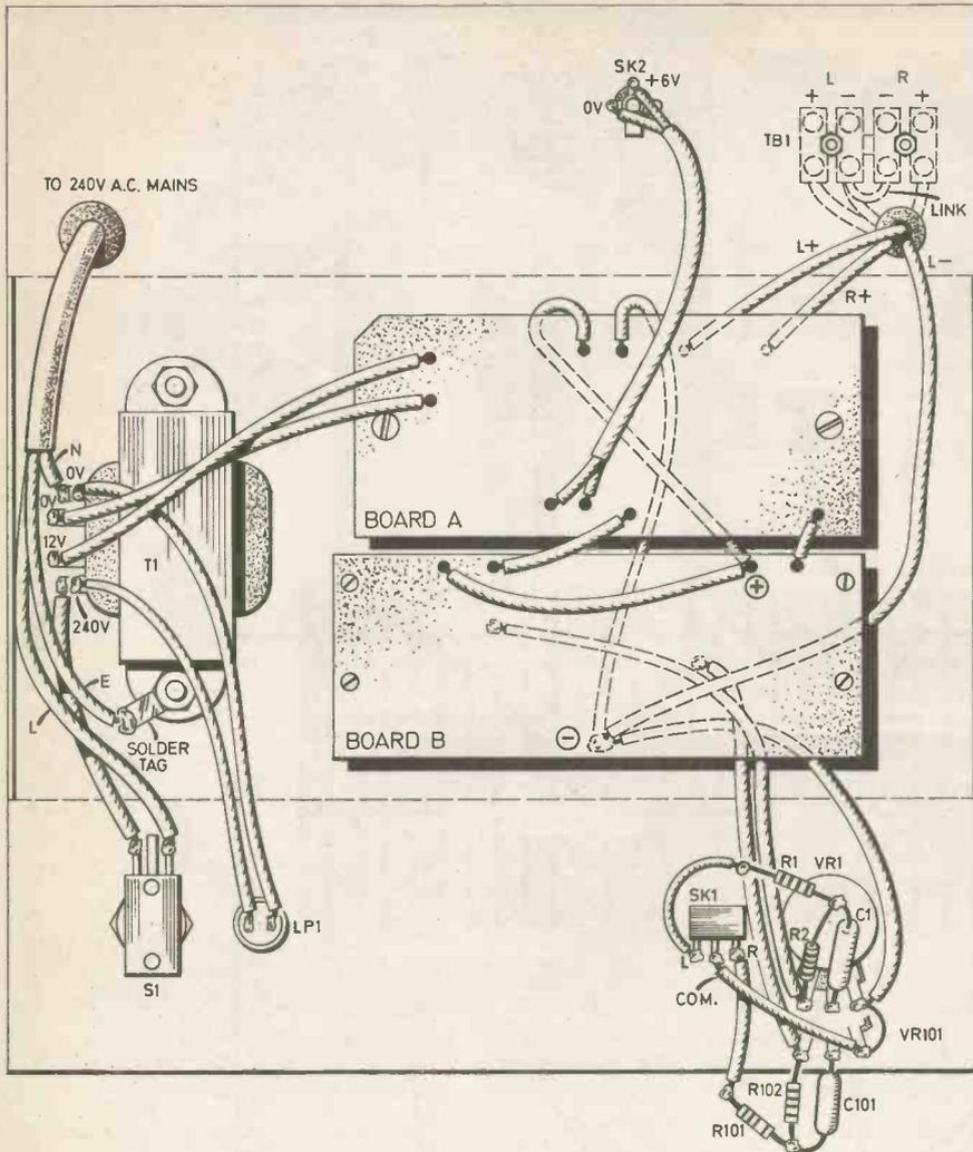
Fig. 4. Layout of the boards and other components in the prototype with complete interwiring details. Front and rear panels have been drawn folded down for clarity. The L-shaped bracket beneath SK1 is not shown.
