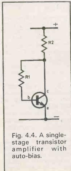
Fig. 4.4. A single-stage transistor amplifier with auto-bias.
