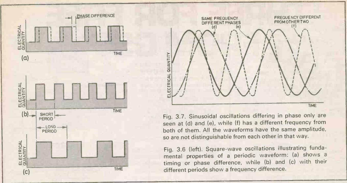
Fig. 3.7. Sinusoidal oscillations differing in phase only are seen at (d) and (e), while (f) has a different frequency from both of them. All the waveforms have the same amplitude, so are not distinguishable from each other in that way.
