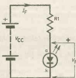
Fig. 1. L.e.d. circuit showing the usual symbols.
