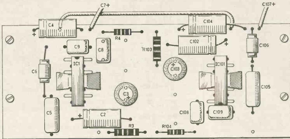
Fig. 2 (above). Shows the layout of the components on the topside of the p.c.b. (board B) and the master p.c.b. pattern to be etched on the underside (full-size).
