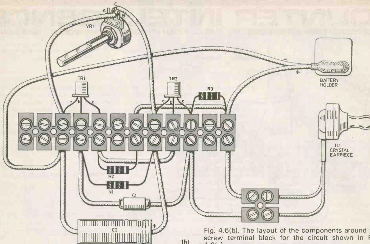
(b) Fig. 4.6(b). The layout of the components around the screw terminal block for the circuit shown in Fig. 4.6(a).
