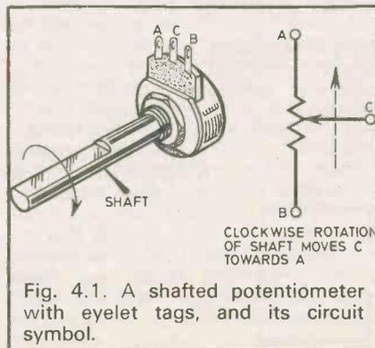
Fig. 4.1. A shafted potentiometer with eyelet tags, and its circuit symbol.
