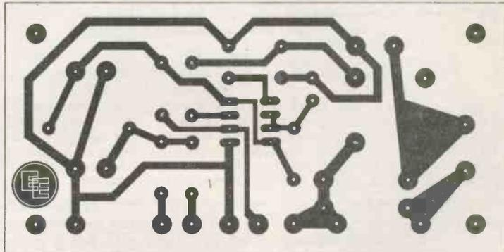
Fig. 2. Full size track pattern and component layout for the Opto Repeater circuit board. Note that the board is designed to accept the Maplin "ultra miniature high power mains relay".
