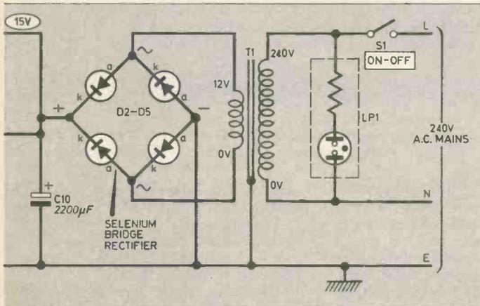
D5 to produce a 16V d.c. smooth level across C10. This is the positive supply to both left and right amplifiers.
