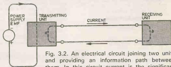
Fig. 3.2. An electrical circuit joining two units and providing an information path between them. In this circuit current is the significant quantity.
