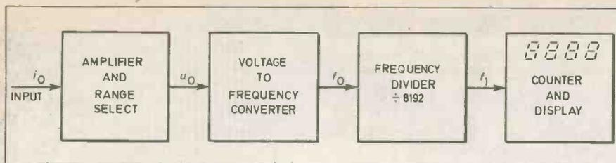
Fig. 1. Block diagram of the Coulomb Meter showing the basic theory of operation. The voltage-to-frequency converter produces an output frequency of 81.92kHz for an input current of 1A.
