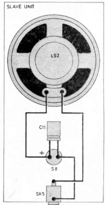
Fig. 6. Interwiring details for the master control and one slave unit. The case mounted components have been laid "flat" for clarity of wiring.
