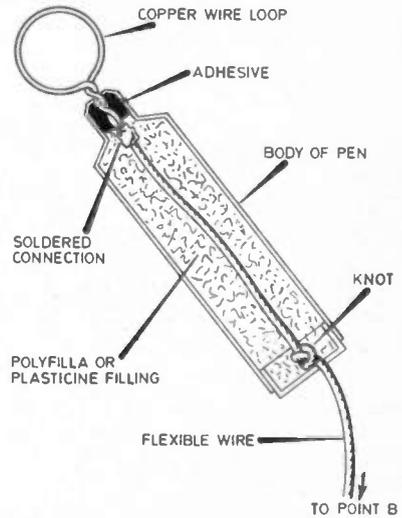
Fig. 5 (Right). Suggested method of construction for the hand-held loop.
