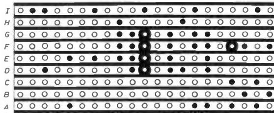
Fig. 4 (Above). Component layout, interwiring details and underside of the stripboard showing breaks (5 off) in the copper strips. Note that there should be 22 holes not 21 as shown.
