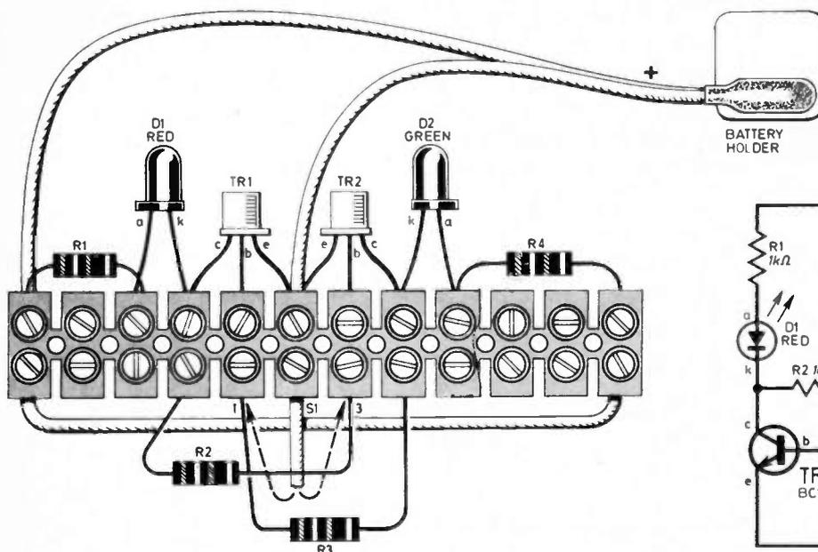
Fig. 6.4. Circuit diagram and demonstration model using another transistor to control the flip-flop circuit of Fig. 6.3.
