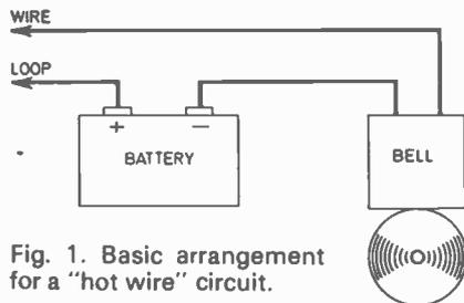
Fig. 1. Basic arrangement for a “hot wire” circuit.
