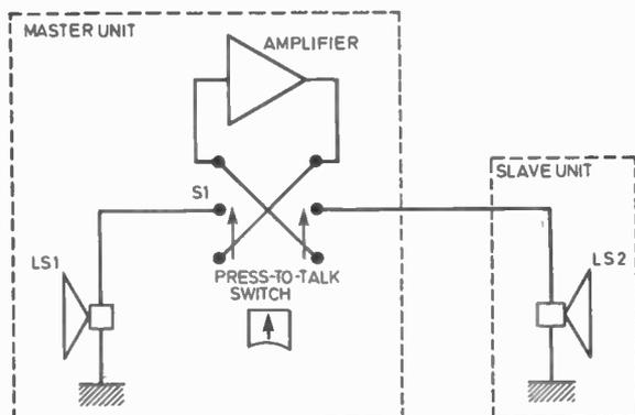
Fig. 1. Block schematic of the basic intercom circuit.
