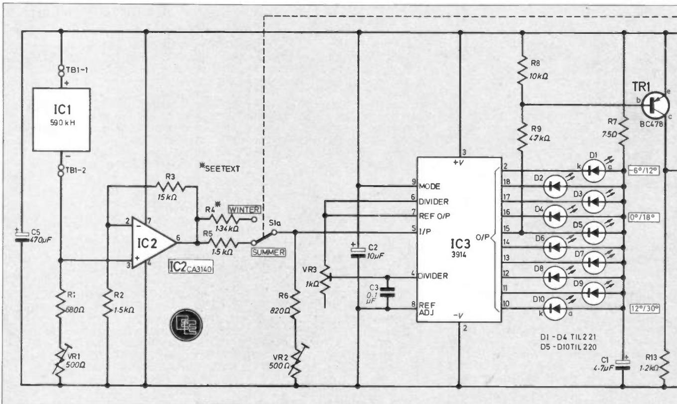
Fig. 1. Complete circuit diagram of the Car Thermometer. Note that the temperature sensor, IC1, is connected to the terminal
