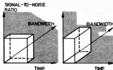
Fig. 5.6. Three-dimensional analogy in which the box is a quantity of information (bits). In transmitting a given quantity of information (the volume of the box), the time taken, bandwidth and signal-to-noise ratio may be exchanged with each other. These two examples illustrate an exchange of time and bandwidth (signal-to-noise ratio remaining constant).
