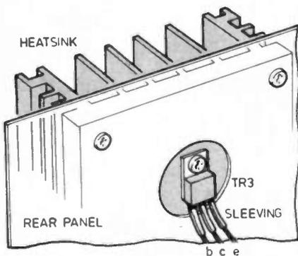
Fig. 5 (Left). Mounting details for transistor TR3. Note that no insulating kit is used on this transistor so the rear panel and the heatsink are connected to the collector and should not be "earthed".
