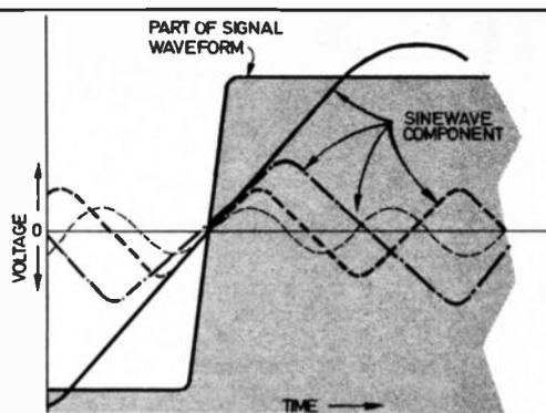
Fig. 5.5. How a signal waveform may be analysed into a set of sine-wave components (Fourier analysis). Not all of the components that make up this signal waveform are shown here.
