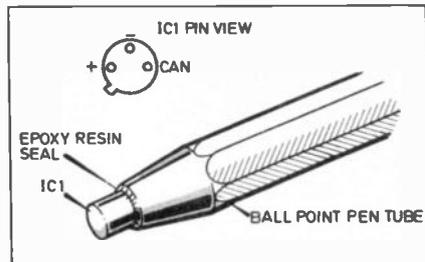
Fig. 4. Method of mounting the temperature sensor, IC1, in a plastic ball point pen tube.
