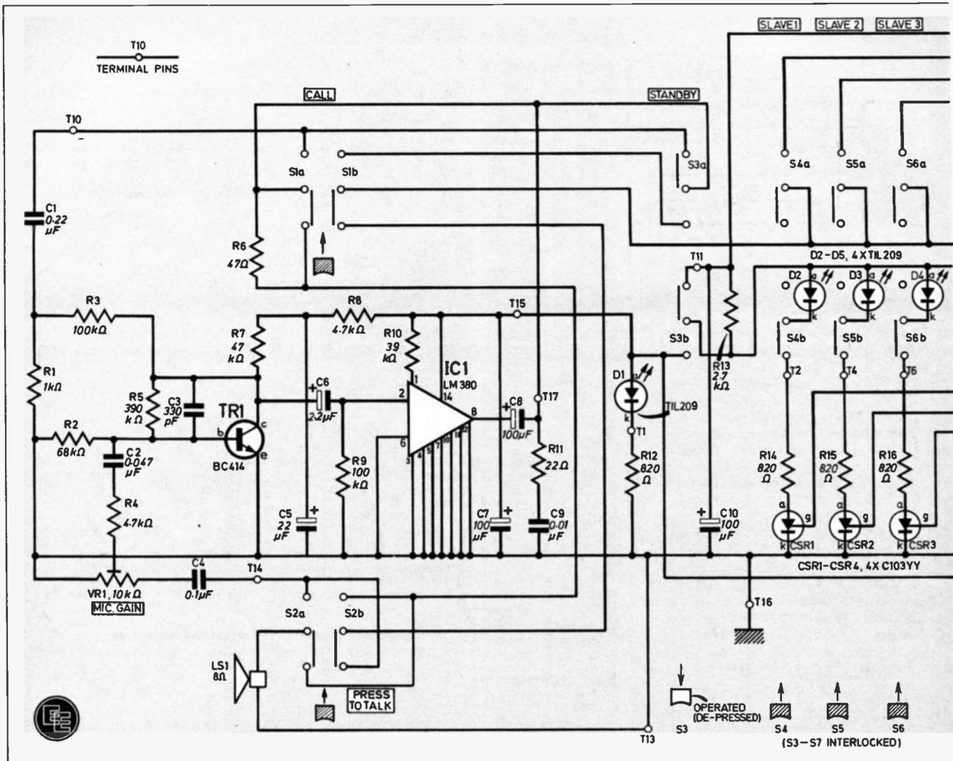
Fig. 4. Complete circuit diagram for the Multi-Station Intercom. All switches are shown in the standby position. The circuit for the slave unit is shown in the panel on the far right.
