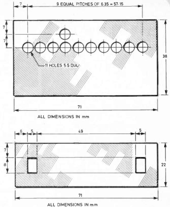
Fig. 3. Drilling details for the display panel and switch label. Both are specifically designed for the Lascar hand-held case.
