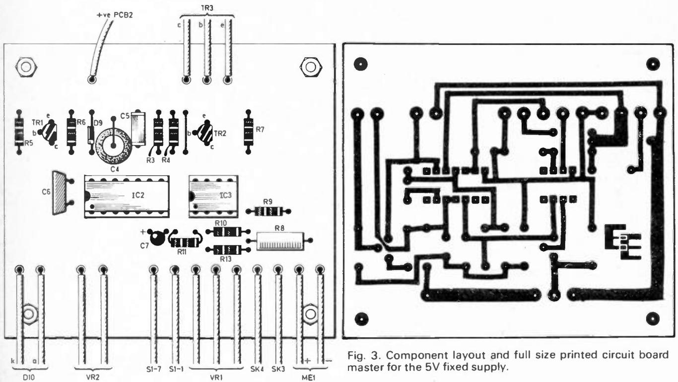
Fig. 3. Component layout and full size printed circuit board master for the 5V fixed supply.
