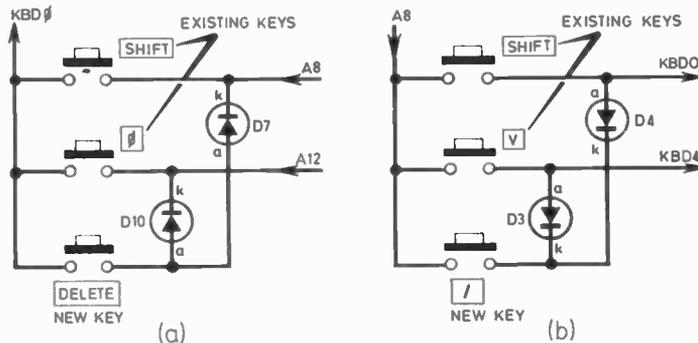
Fig. 3. Two of the three different switch-circuits used in the design, re-drawn for clarity.
