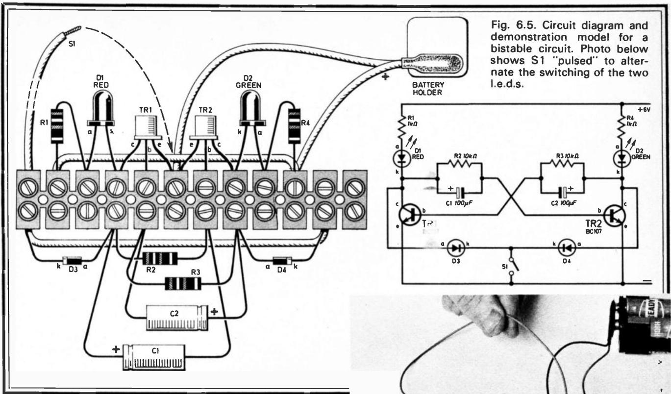
Fig. 6.5. Circuit diagram and demonstration model for a bistable circuit. Photo below shows S1 "pulsed" to alternate the switching of the two l.e.d.s.
