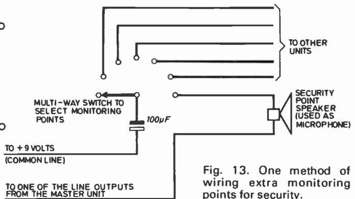
Fig. 13. One method of wiring extra monitoring points for security.
