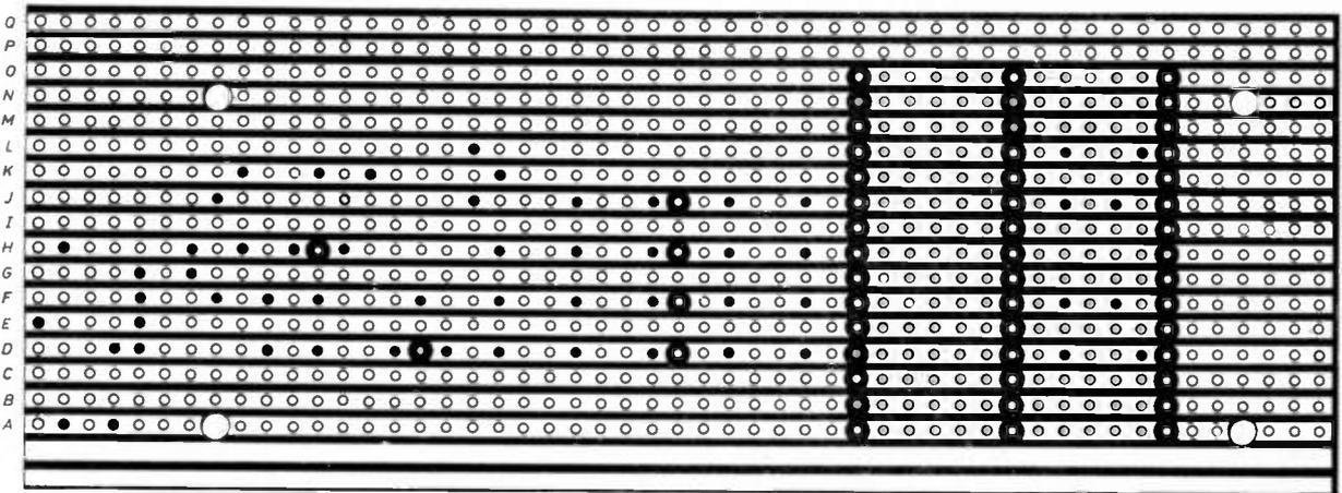
Fig. 3. The layout of the components for the power supply section of the Eprom Programmer and the breaks to be made on the copper side of the board, with drilling details.
