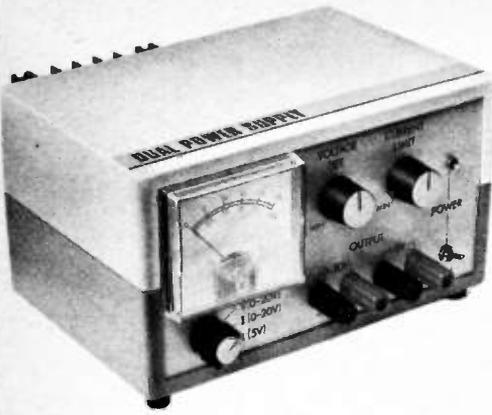
The a.c. input is provided by the transformer and is rectified and smoothed by the bridge rectifier D1-D4, and capacitor C1, respectively. The low value resistor R1 is used to sense the output current for the meter.
