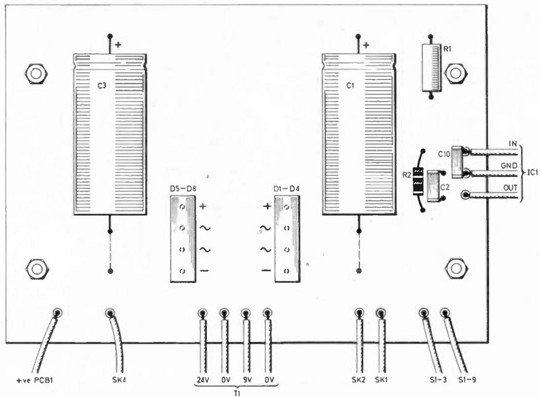
Fig. 2. Component layout and full size printed circuit board master (opposite page) for the 0-20V variable supply.
