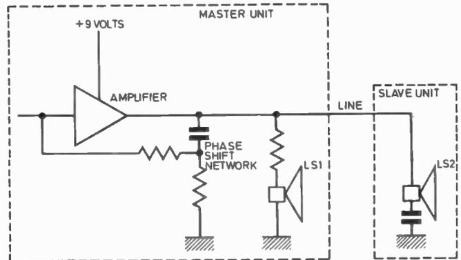
Fig. 2. Basic circuit when the master "calls".
