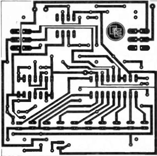
Fig. 2. Full size p.c.b. artwork and component layout. All the l.e.d.s are soldered into the board at the same height of approximately 20mm (to the top of the lens).
