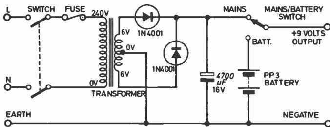
Fig. 12. Suggested circuit diagram for a mains/battery power supply.
