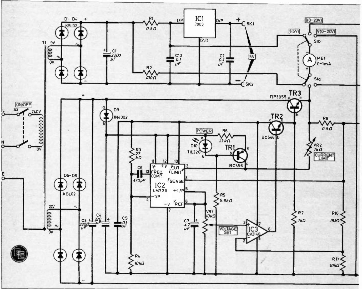
driving a constant current of 0.75mA from the current source TR1 and its associated components, through VR2. The voltage across VR2 is added to that across the sense resistor, increasing the current limits sensitivity.
