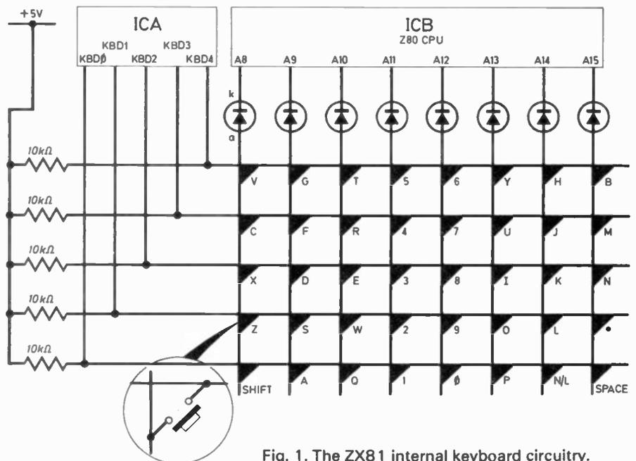
Fig. 1. The ZX81 internal keyboard circuitry.
