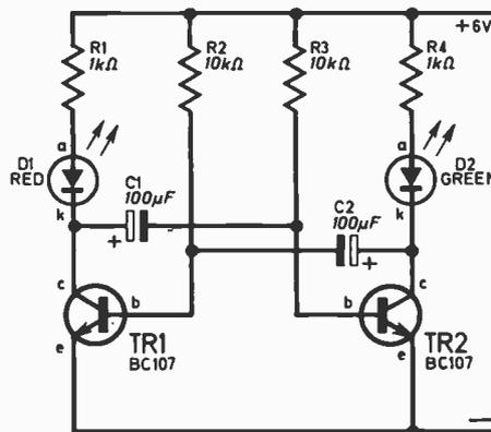
Fig. 6.6. Circuit diagram for an "astable" oscillator which can be built from components from Fig. 6.5.
