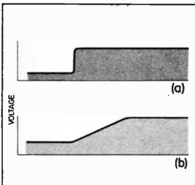
Fig. 5.4. Parts of two signals, illustrating different rates of change of voltage with time.
