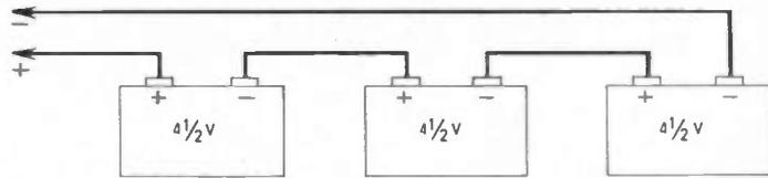
Fig. 3. Connecting three batteries in series to power the Buzz Off! circuit.
