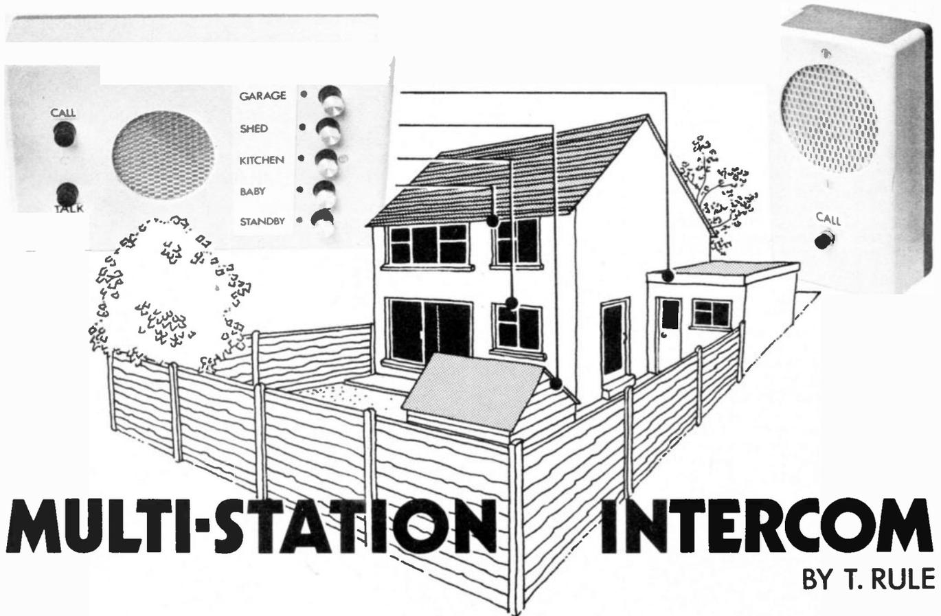
THE unit to be described can be built to connect to any number of slave units via a two-wire interconnecting lead. Designed to provide private intercommunication between the master unit and any slave, it can also be used as a baby alarm or a general security system, and provides a means of listening into the slave units. For example, if a slave unit is mounted outside somewhere in the grounds of the property, it is possible to listen in on that unit for any intruders who may be nearby.
