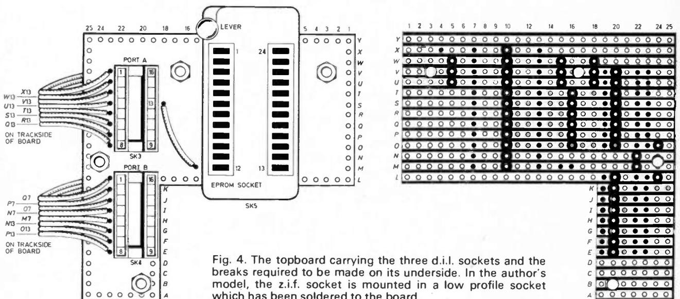
Fig. 4. The topboard carrying the three d.i.l. sockets and the breaks required to be made on its underside. In the author's model, the z.i.f. socket is mounted in a low profile socket which has been soldered to the board.
