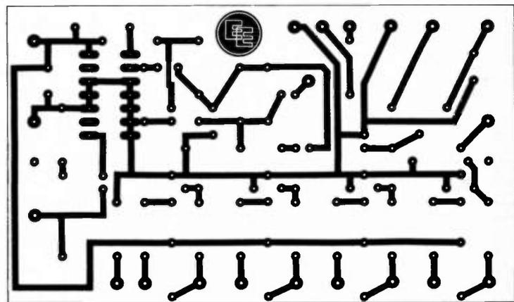
Fig. 5. Component layout on the topside of the circuit board and full size printed circuit board master.
