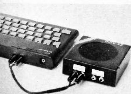
Completed amplifier plugged into the ZX Spectrum.
