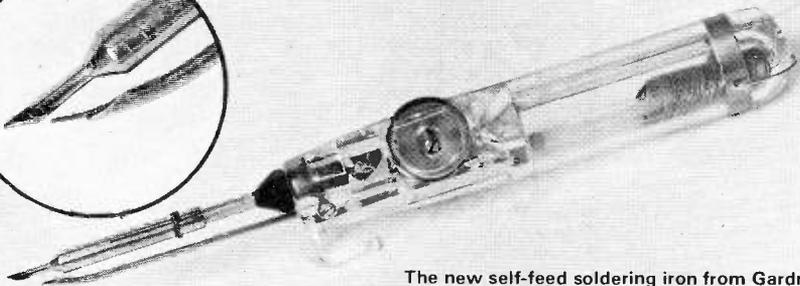
The new self-feed soldering iron from Gardner Precision Engineering.
