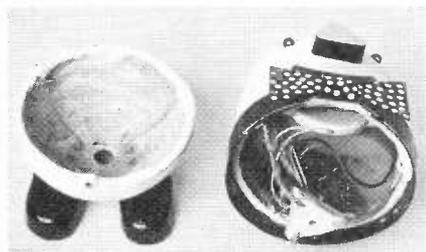
The two halves of the case can be clearly seen, the bottom half showing the wire frame. Photograph (right) shows a close-up of the wiring inside the top half of the case.
