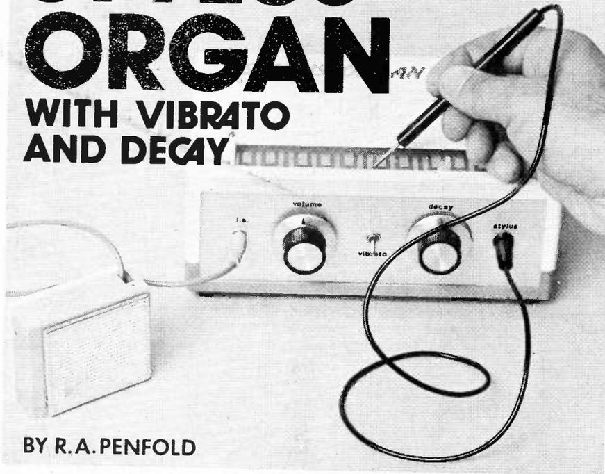
THE Stylus Organ is basically a conventional instrument which covers two octaves (including sharps or flats), one octave either side of middle C. It has a switchable vibrato oscillator, the use of which gives a more "rich" and pleasant sound. An unusual feature which can further enhance the sound, is a simple envelope generator circuit, and this gives a fast attack time with a decay time which can be varied from a fraction of a second to several seconds.
