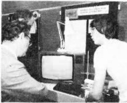
**T**HIS project is intended for use in the chemistry laboratory and is a device which extends the capabilities of a pH meter by linking it to a Research Machine 380Z using Control Basic.
