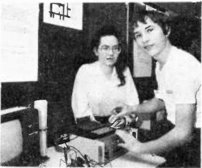
**T**HE circuit is a complete unit for interfacing the ZX81 in a school science laboratory. The unit has its own power supply, supplying 1A to the circuit, and also the external circuitry if connected.
