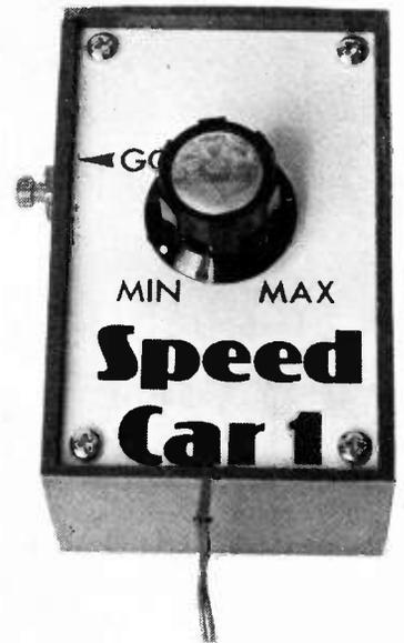
VR1. The hand control is held in one hand while depressing switch S1, and the speed regulated with VR1 using the other hand.
