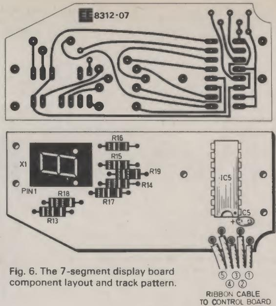
Fig. 6. The 7-segment display board component layout and track pattern.
