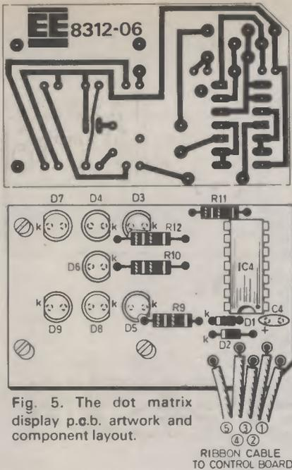
Fig. 5. The dot matrix display p.c.b. artwork and component layout.
