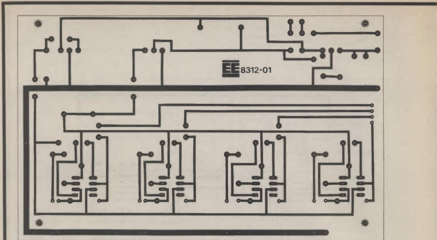
Fig. 6.6. Full-size printed circuit board master for the analogue board.
