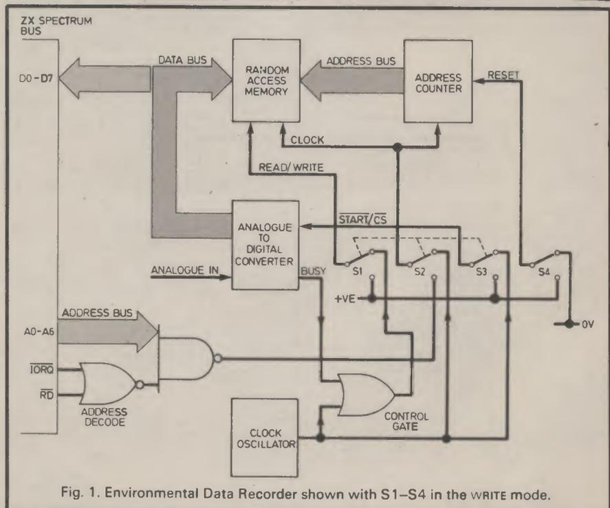
Fig. 1. Environmental Data Recorder shown with S1-S4 in the WRITE mode.
