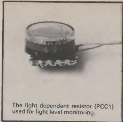
The light-dependent resistor (PCC1) used for light level monitoring.
