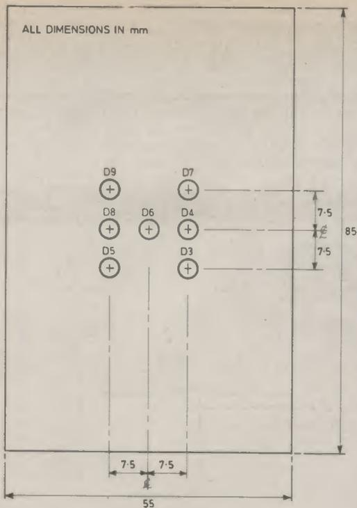
Fig. 7. The face plate drilling details. The mounting holes are positioned using the p.c.b. as a template.
