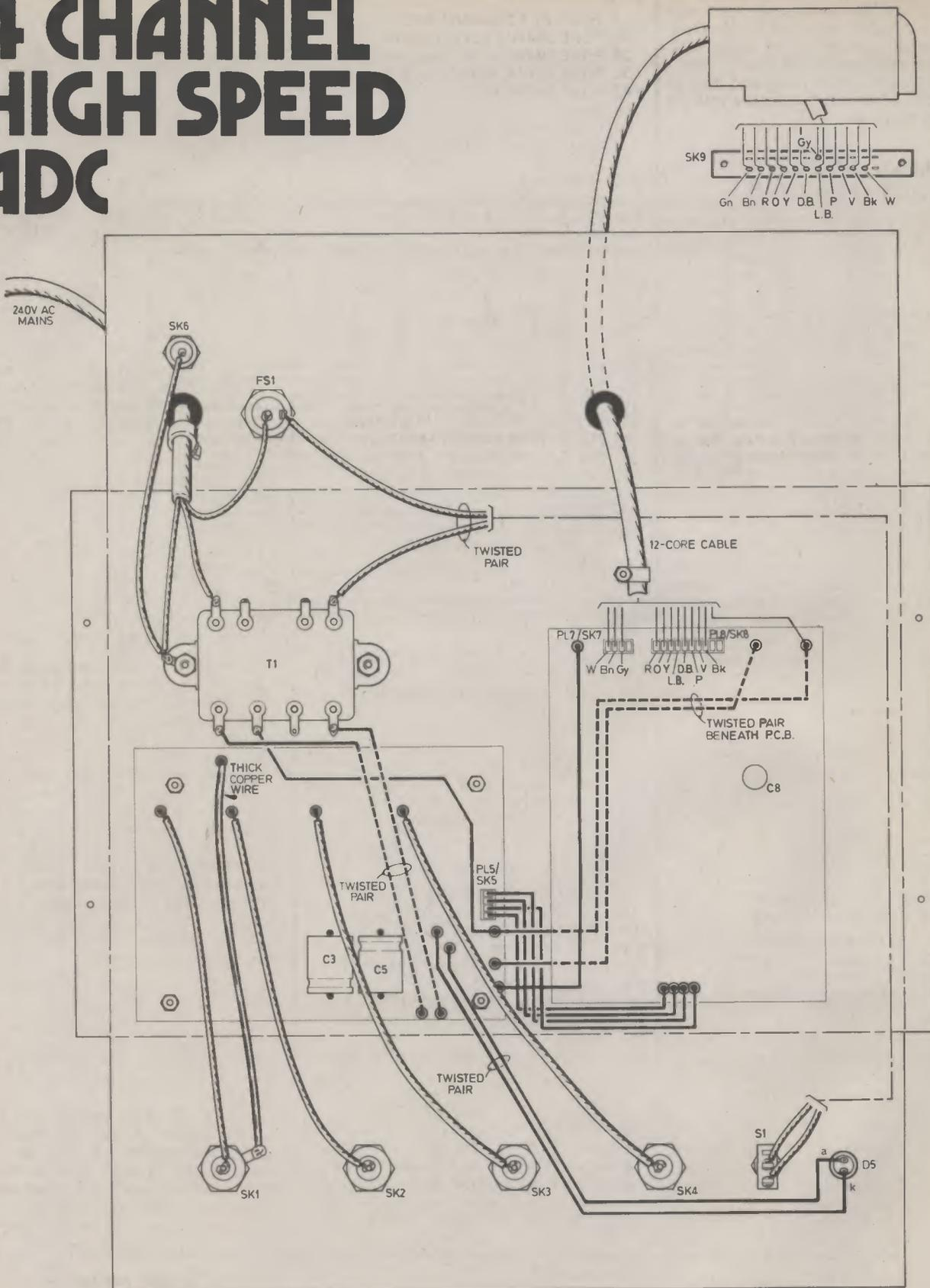
Fig. 6.10. Interwiring diagram for the two boards.
