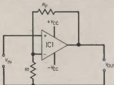
Fig. 6.1b. The configuration for a non-inverting amplifier.
