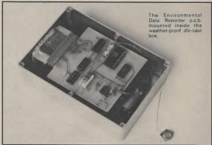
The Environmental Data Recorder p.c.b. mounted inside the weather-proof die-cast box.
