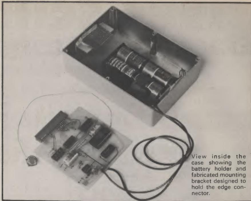
View inside the case showing the battery holder and fabricated mounting bracket designed to hold the edge connector.
