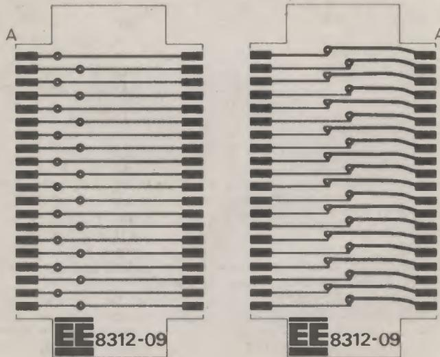
Fig. 6. Full-size track artwork of the double-sided header p.c.b. This board carries the 40-way edge connector (SK1) and also permits additional peripherals to be plugged into the TRS-80 I/O port. Top view shows the ribbon cable wiring.
