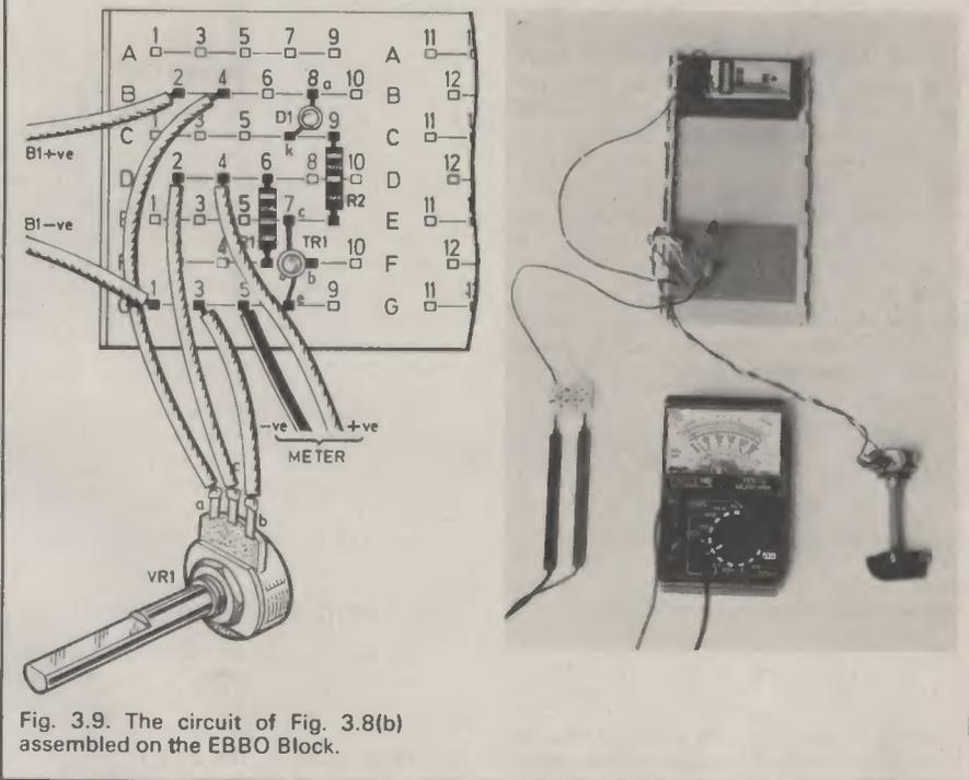
Fig. 3.9. The circuit of Fig. 3.8(b) assembled on the EBBO Block.
