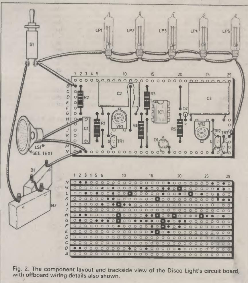
Fig. 2. The component layout and trackside view of the Disco Light's circuit board, with offboard wiring details also shown.
