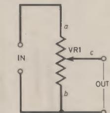
Fig. 3.2. A volume control or "potentiometer" has a resistance track a-b and a sliding contact c.
