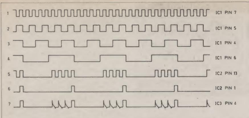
Fig. 3. Shown are the pulses that should be obtained when testing IC1, IC2 and IC3 with an oscilloscope. Note that pin 4 of the oscillator IC3 sees a full width pulse instead of a narrow pulse on the fourth count to produce the "squawk".
