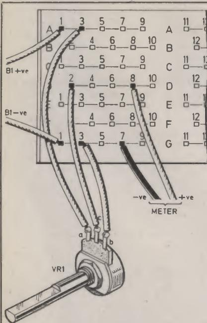
Fig. 3.4. The circuit of Fig. 3.3(a) assembled on the EBBO Block.
