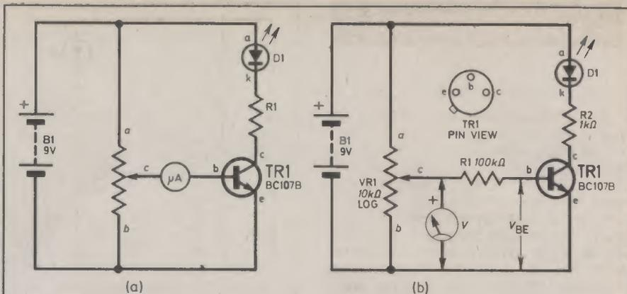
Fig. 3.8. How base current governs collector current; (a) A not very good way of finding out; (b) This way is safer, but the base current must be estimated. (Experiment 3.4).
