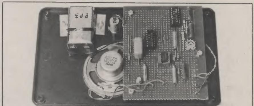
Component board shown fitted to the lid of the case, with off-board wiring details also shown.
