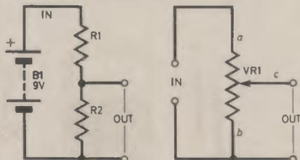
Fig. 3.1. Resistors R1 and R2 form a voltage divider across the 9V battery.
