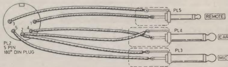
Fig. 7. Wiring of the cassette lead to connect the interface to the cassette player. If the 4-core screen cable is used, the screens must *not* be used for the REMOTE (PL5) connections.
