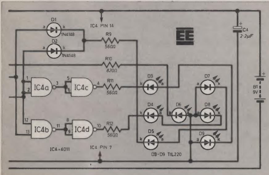
Fig. 3. The 7-segment display circuit.
