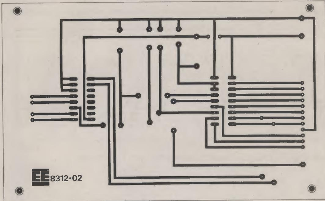
Fig. 6.8. Full-size printed circuit board master for the digital board.
