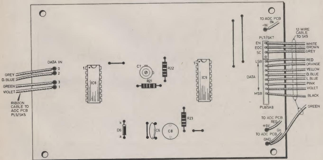
Fig. 6.9. Complete component layout for the digital (clock) board.
