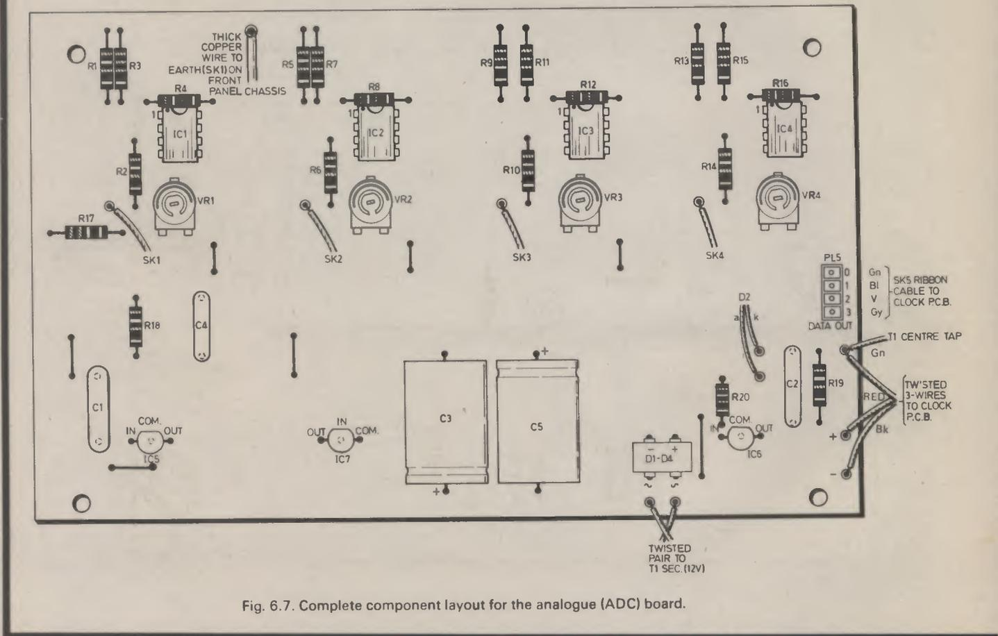
Fig. 6.7. Complete component layout for the analogue (ADC) board.
