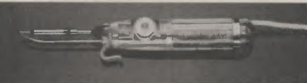
This new development in Soldering Irons combines light weight (80g.) with unique one-handed operation. Solder is housed in the transparent handle and applied directly to the joint by turning the serrated wheel (located in the handle) with the index finger, allowing a clean, bright joint to be made every time. To renew the solder, the spring clip at the end of the handle is released, the cap is removed and a refill is inserted.
