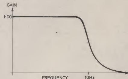
Fig. 6.2. The response for a typical low-pass filter.
