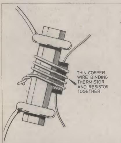
Fig. 2. The method of fixing R1 to RTH1 (and R2 to RTH2) using fuse wire. Note these resistors *must* be  $\frac{1}{8}$ W components.
