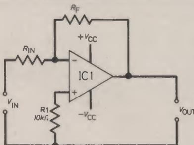
Fig. 6.1a. The operational amplifier shown is being used in the inverting mode.
