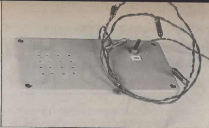
If adjusted too far anti-clockwise, the lamps will be on continuously. VR2 may need final adjustment to obtain the most satisfactory setting. Note that the adjustment of VR2 depends on the number and type of lamps in the chain. When music is played, the lamps should flash in sympathy.
