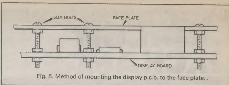
Fig. 8. Method of mounting the display p.c.b. to the face plate.
