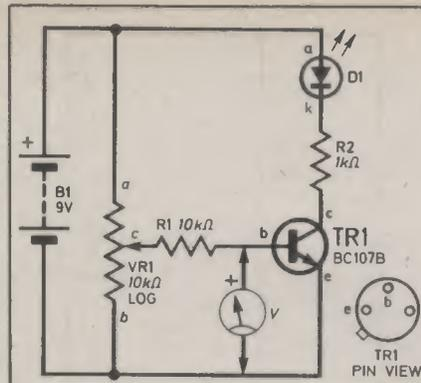
Fig. 3.6. How much base voltage is needed to turn on a transistor? (Experiment 3.3).
