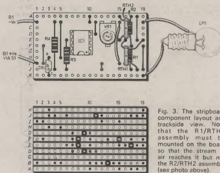
Fig. 3. The stripboard component layout and trackside view. Note that the R1/RTH1 assembly must be mounted on the board so that the stream of air reaches it but *not* the R2/RTH2 assembly (see photo above).
