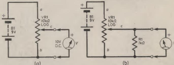
Fig. 3.3(a). How a potentiometer can "tap off" any portion of an input voltage. (Experiment 3.1); (b) Connecting R1 as a relatively low resistance "load" has a marked effect on the output voltage. (Experiment 3.2).
