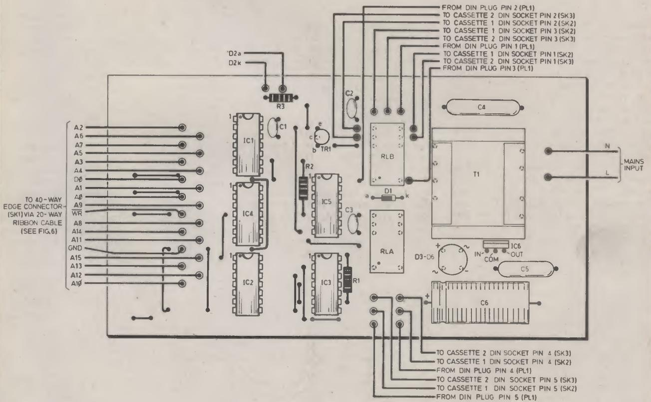
Fig. 5. The full-size p.c.b. track artwork and component layout diagram. This board is available from the *EE PCB Service*, Order code 8312-03. All wires (including the ribbon cable) must be terminated with a Veropin. Note that the mains input cable will require a clamp to act as strain relief at the point of entry on the case.
