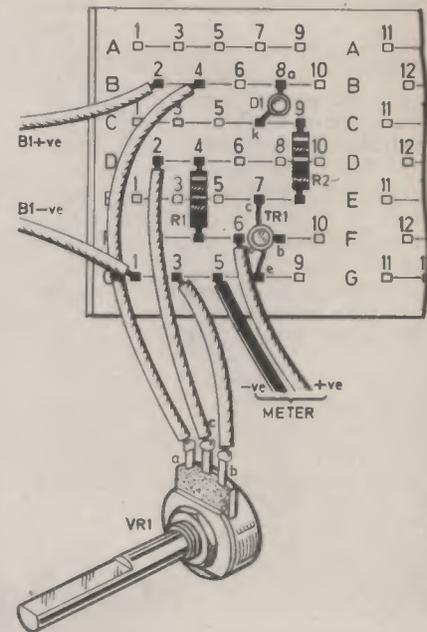
Fig. 3.7. The circuit of Fig. 3.6 assembled on the EBBO Block.
