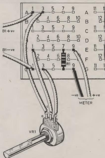
Fig. 3.5. The circuit of Fig. 3.3(b) assembled on the EBBO Block.
