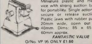
Miniature plastic and metal vice with strong suction base for portability. Single action to secure or release suction. Plastic jaws with rubber pads 20mm wide, open out to 40mm. Dims: 85 x 65 x 60mm approx.
