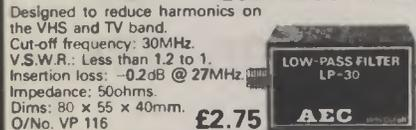
Designed to reduce harmonics on the VHS and TV band. Cut-off frequency: 30MHz. V.S.W.R.: Less than 1.2 to 1. Insertion loss: -0.2dB @ 27MHz. Impedance: 50ohms.
