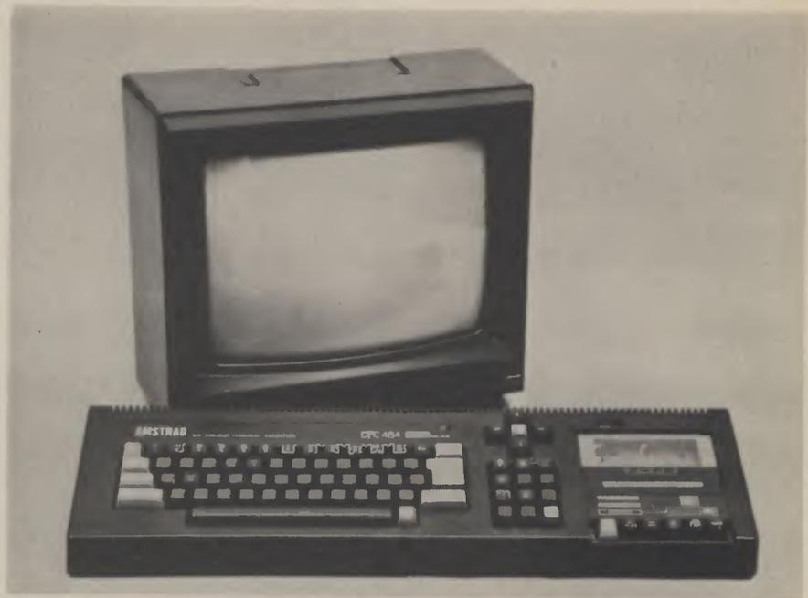
Any microcomputer system requires an input facility (keyboard), a display for output (TV), and some long-term storage medium (cassette or disk).
