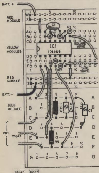
Fig. 10.8. Complete EBBO i.c. board layout for square and sine-wave oscillators and buffers, Fig. 10.6 and Fig. 10.7, respectively.
