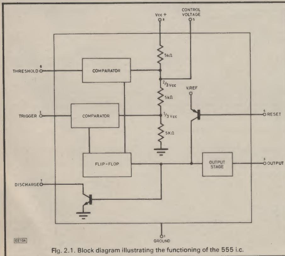
Fig. 2.1. Block diagram illustrating the functioning of the 555 i.c.
