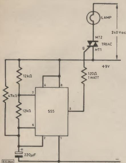
Fig. 2.13. In this circuit a 555 turns on a triac when its output is low.
