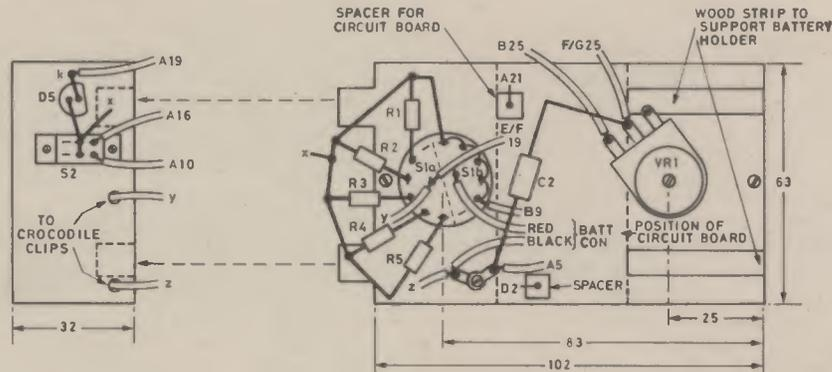
Fig. 4. Components and wiring on the "removable panel". The two sections are glued or screwed together with suitable spacers between. Identical thickness spacers are used between the panel and the case top.
