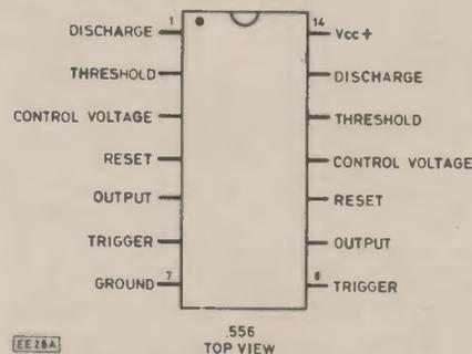
Fig. 2.15. The 556 i.c. comprises two 555s in a single package.
