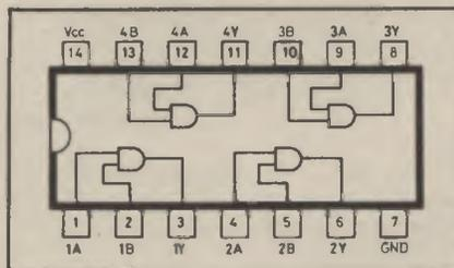
Fig. 3. Internal connections for a 7408 or 74LS08 quad 2-input AND gate.
