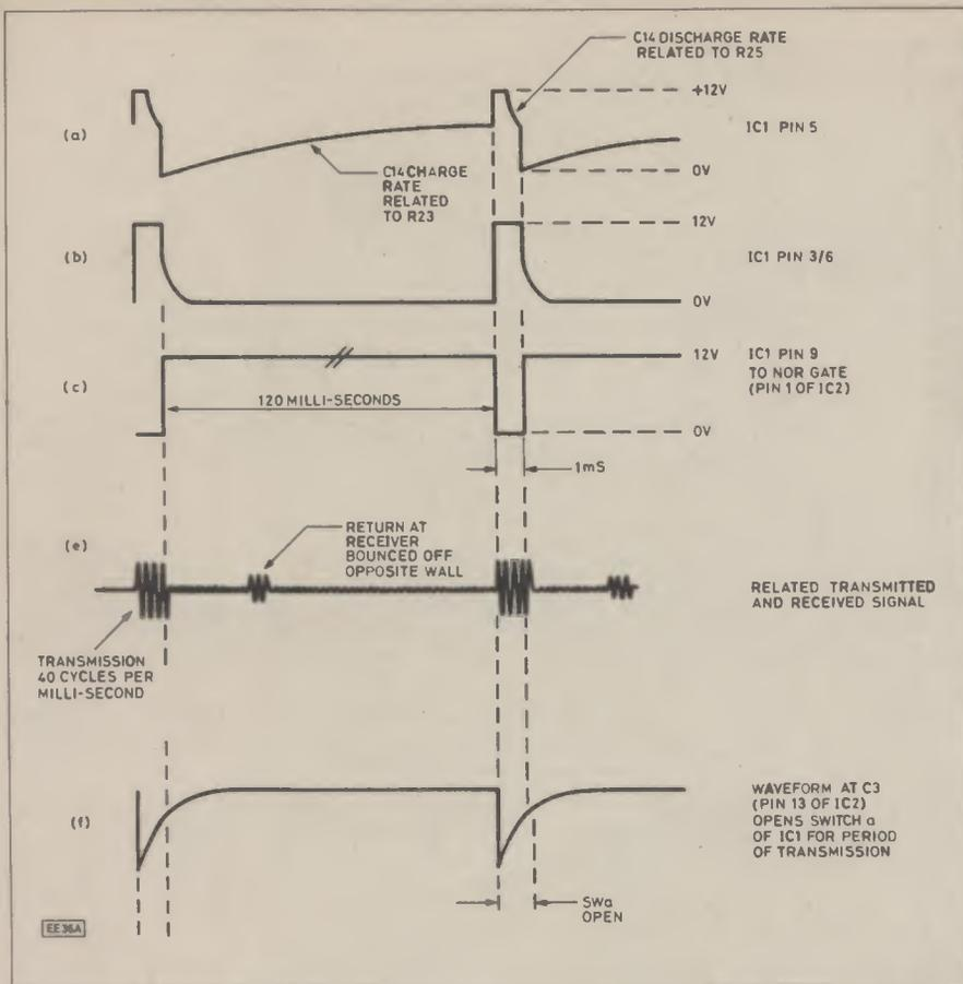
Fig. 2. Timing diagram of the Ultrasonic Burglar Alarm.
