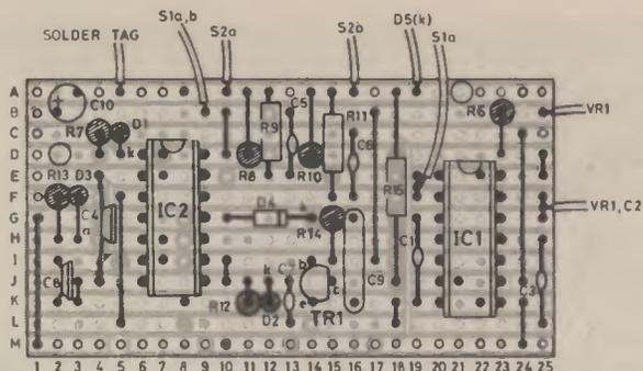
EE556B Fig. 3. Component layout (actual size).
