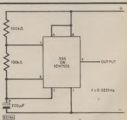
Fig. 2.3(b). The 555 and ICM7555 will oscillate at very low frequencies. The calculated cycle length here is 45.2 seconds.
