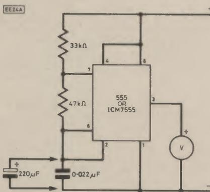
Fig. 2.11(b). The output waveform can be monitored with a voltmeter if the oscillator is slowed down by temporarily connecting a large value capacitor across the frequency control capacitor.
