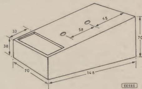
Fig. 5. Case dimensions. The circuit board stands 18mm off the panel, screwed onto pillars of wood, or bolted using spacers.
