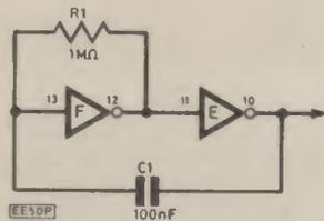
Fig. 10.6(a). Square-wave oscillator made from two inverters ("F" and "E") of a 4069 (IC1). Frequency about 6Hz.
