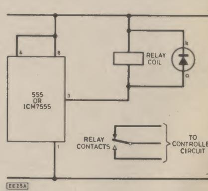
Fig. 2.12. With a very low frequency 555 or ICM7555 oscillator, external high current circuits can be controlled with the aid of a relay.
