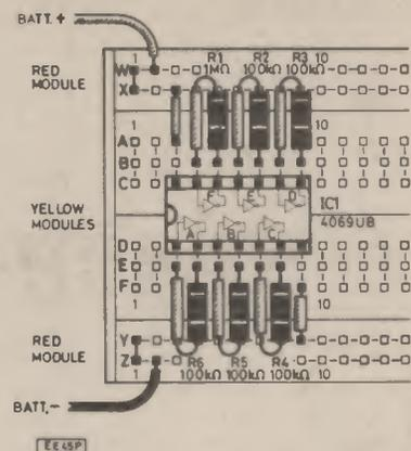
Fig. 10.5. EBO i.c. layout for biasing experiment. The positions of the six inverters are shown on IC1 outline.
