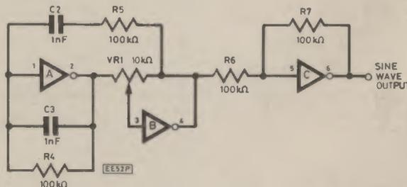
Fig. 10.7. Sine-wave oscillator using two inverters ("A" and "B") followed by unity gain buffer "C". VR1 sets the amplitude, which is greatest when the spindle is turned fully anti-clockwise.
