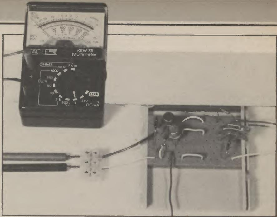
good sinewave, VR1 is set so that the circuit just oscillates steadily. The frequency is about 1-6kHz.
