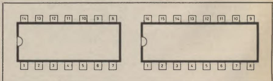
Fig. 2. Dual-in-line 14-pin and 16-pin TTL i.c.s have a notch at the end of the package to identify pin 1.
