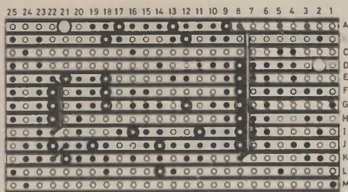
EE556A Fig. 2. Track-side of the circuit board.
