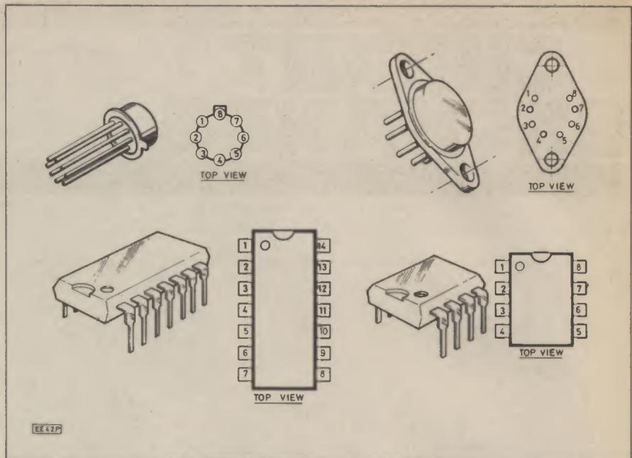
Fig. 1. Pin numbering for linear i.c.s. Metal cans have either a tag or a wider pin spacing to identify pin 8. Dual-in-line packages have a notch and/or a depression to indicate pin 1.
