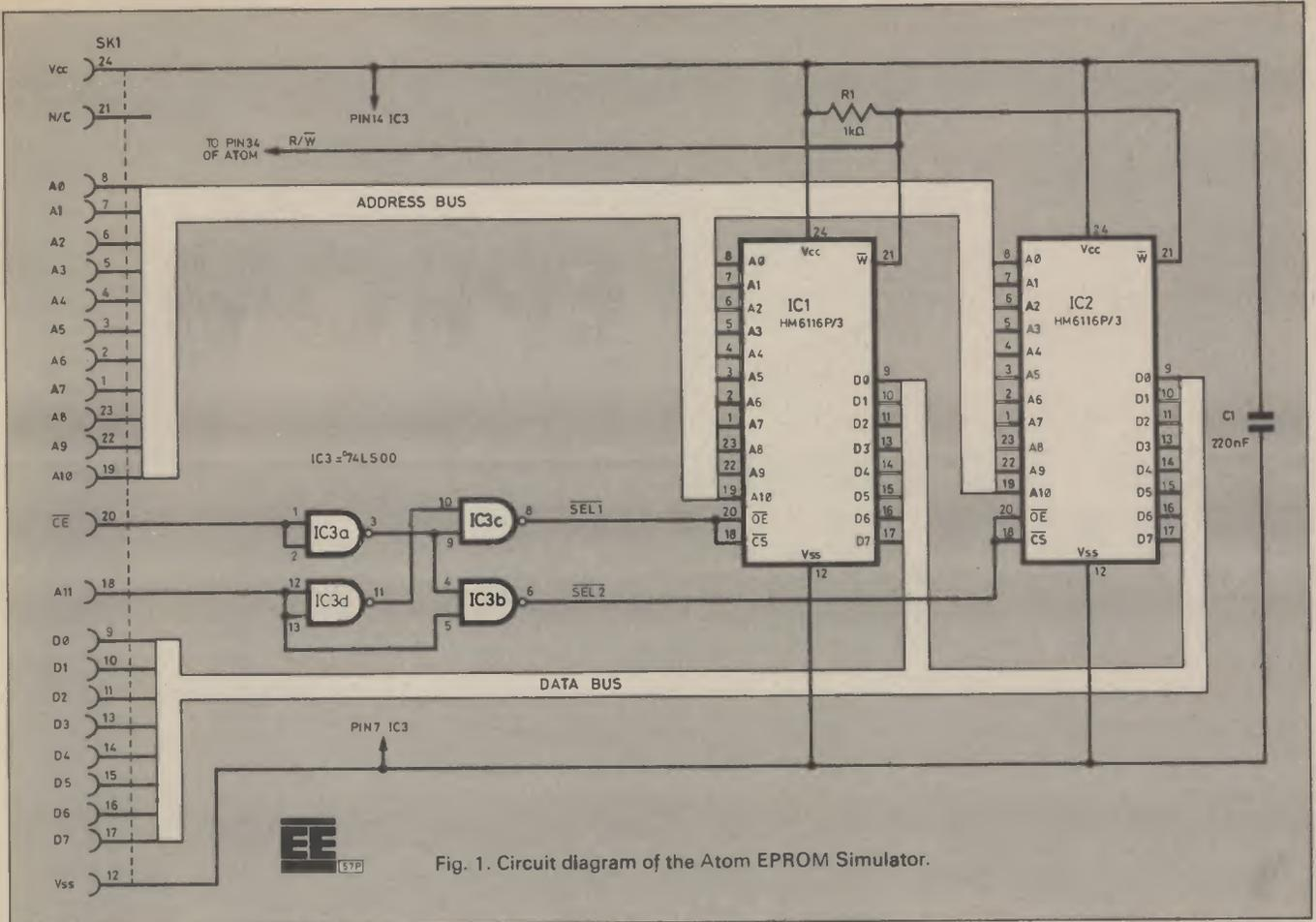
Fig. 1. Circuit diagram of the Atom EPROM Simulator.
