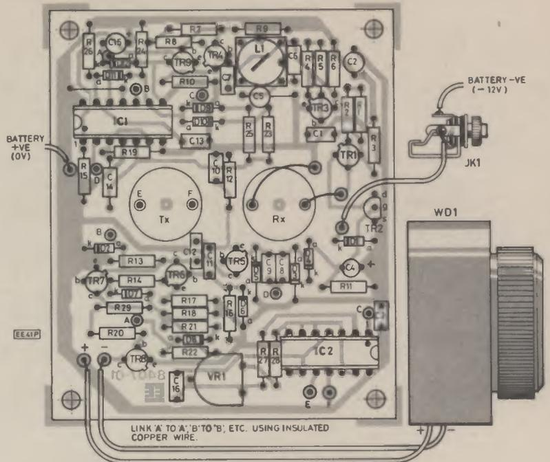
Fig. 4. Layout of components on the top side of the p.c.b. and interwiring to the jack socket/switch and warning device.
