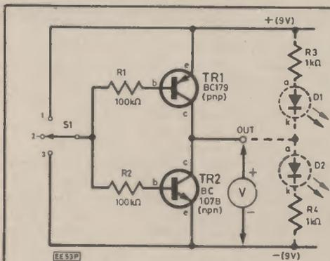
Fig. 10.1. Circuit to illustrate inverter action, with two transistors, one *pnp* and one *npn*, connected "back-to-back" as a complementary pair.
