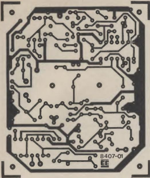
Fig. 3. Actual-size master pattern for the Ultrasonic Burglar Alarm. This board is available from the EE PCB Service, Order code 8407-01.
