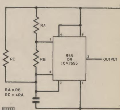
Fig. 2.10. If a third resistor is added and the resistor values are as shown here, the 555 or ICM7555 produces a 50:50 square-wave.
