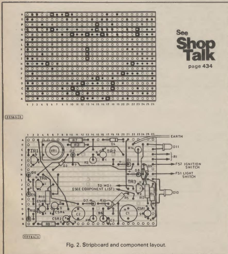
Fig. 2. Stripboard and component layout.
