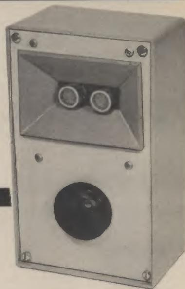
THE Ultrasonic Burglar Alarm has been designed to provide a simple low cost unit which is self-contained, operating from an internal battery. Any person crossing the ultrasonic beam will trigger a screeching piezo-electric sounder mounted in the unit. A relay may be used instead of the sounder to operate an alternative alarm.
