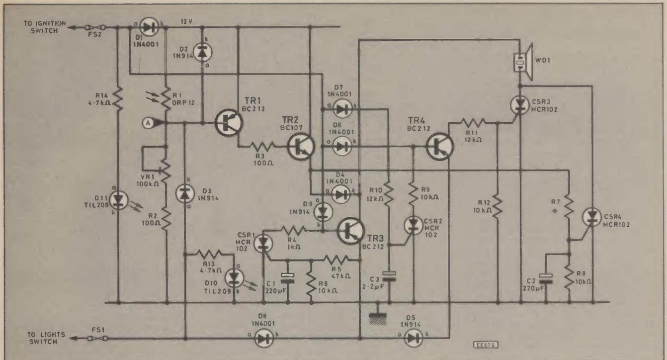
Fig. 1. Circuit diagram of the Car Lights Warning.
