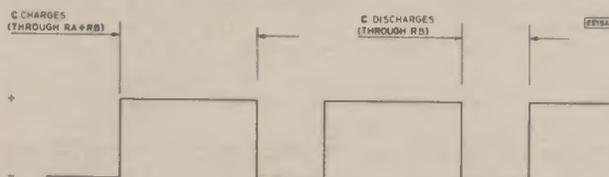
Fig. 2.7 (left). With the basic oscillator circuit of Fig. 2.2, the output is always high for a longer period in the cycle than when it is low.
