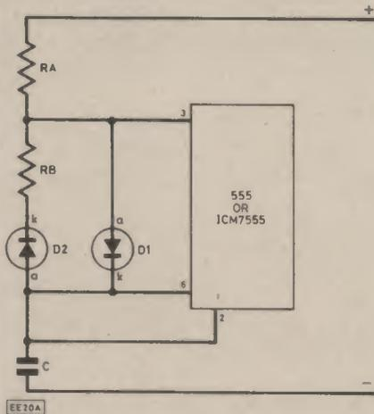
Fig. 2.8. It is possible to obtain duty ratios of less than 50 per cent by adding two silicon diodes. The capacitor charges through D1 and discharges through D2.
