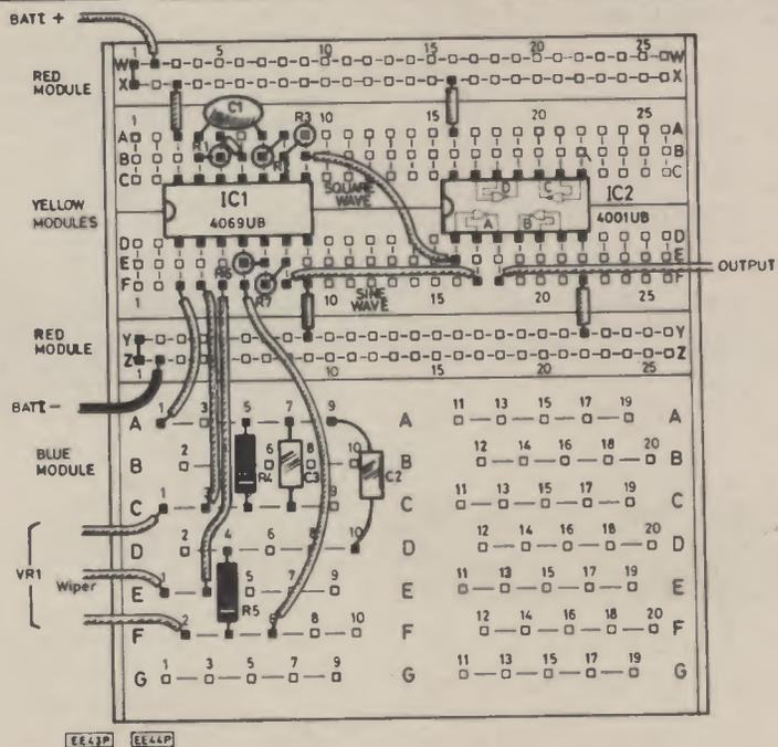
Fig. 10.10. The EBBO i.c. board layout for the 4001UB.
