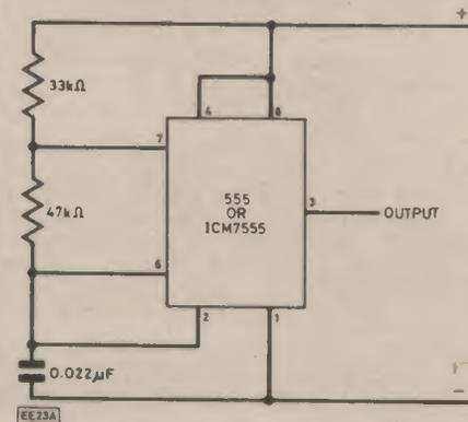
Fig. 2.11(a). An oscillator with a calculated frequency of 523Hz.
