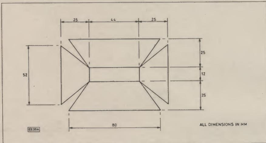
Fig. 6. Window, or horn for the transmitter/receiver aperture. This could be made of stiff card or plastic sheet.
