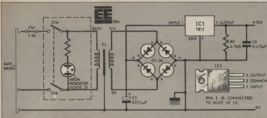
Fig. 1. Complete circuit diagram for the CB Mini PSU.
