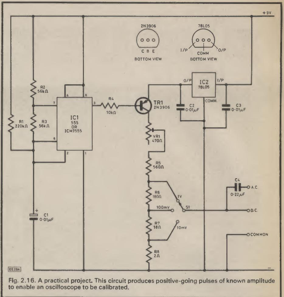
Fig. 2.16. A practical project. This circuit produces positive-going pulses of known amplitude to enable an oscilloscope to be calibrated.
