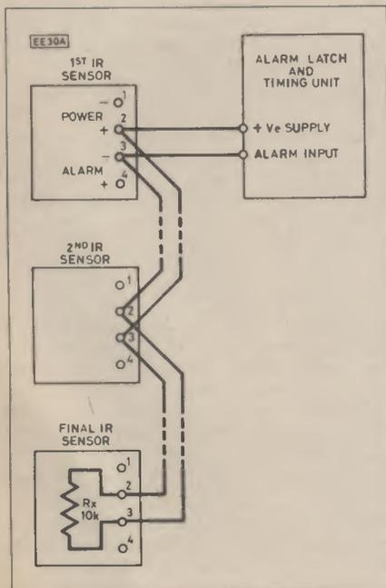
The *Infra-red Alarm System* published last month can incorporate several sensors connected to a single alarm latch unit. Here are some notes on how to do this, and a couple of additional notes on the system's use.
