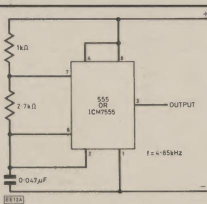
Fig. 2.3(a). A practical example of a 555 or ICM7555 oscillator circuit.
