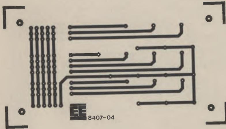
Fig. 4b. Keyboard p.c.b. layout.
