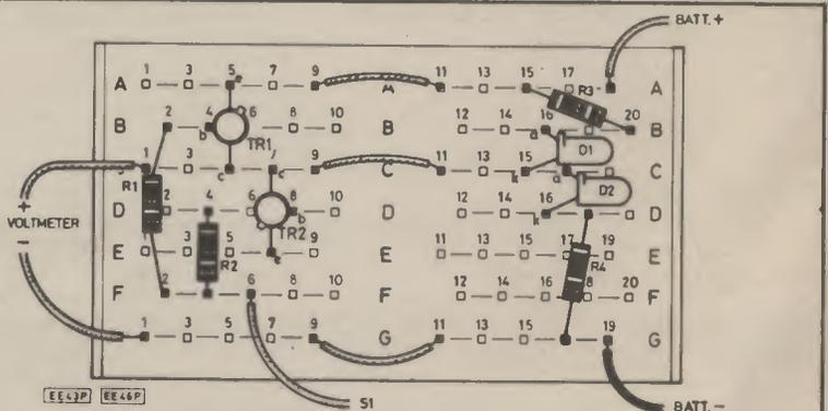
Fig. 10.2. Layout for Fig.10.1 using EBBO discrete module. Note that the layout shows the final circuit: the l.e.d.s and the link between points C9 and C11 are not needed for the first experiment.
