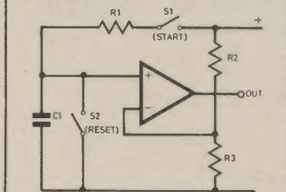
Fig. 10.12. Essentials of a timer circuit. Closing S1 allows C1 to charge via R1. Closing S2 discharges C1 and so resets the circuit. In timer i.c.s the functions of S1 and S2 are performed electronically.
