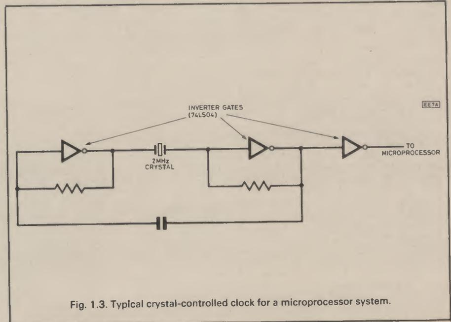
Fig. 1.3. Typical crystal-controlled clock for a microprocessor system.
