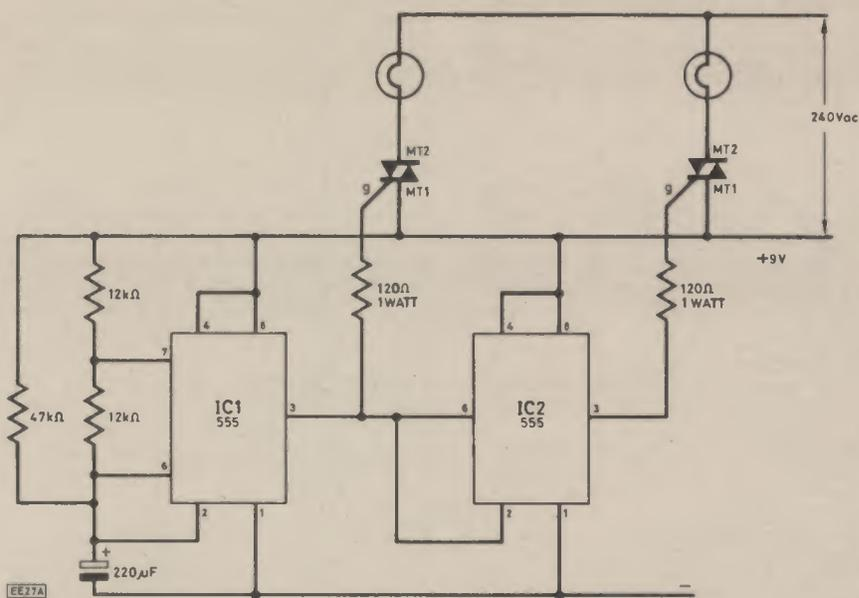
Fig. 2.14. Two 555s are used here to turn on two lamps, or sets of lamps alternately.
