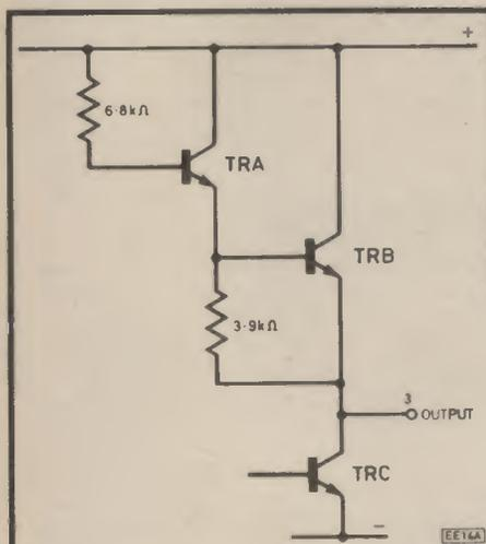
Fig. 2.4 (left). The internal output circuitry of the 555.
