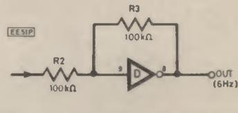
Fig. 10.6(b). Unity gain buffer amplifier (inverter "D").
