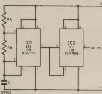
Fig. 2.9. Another way of obtaining duty ratios of less than 50 per cent is to employ a second 555 or ICM7555 as an inverter.
