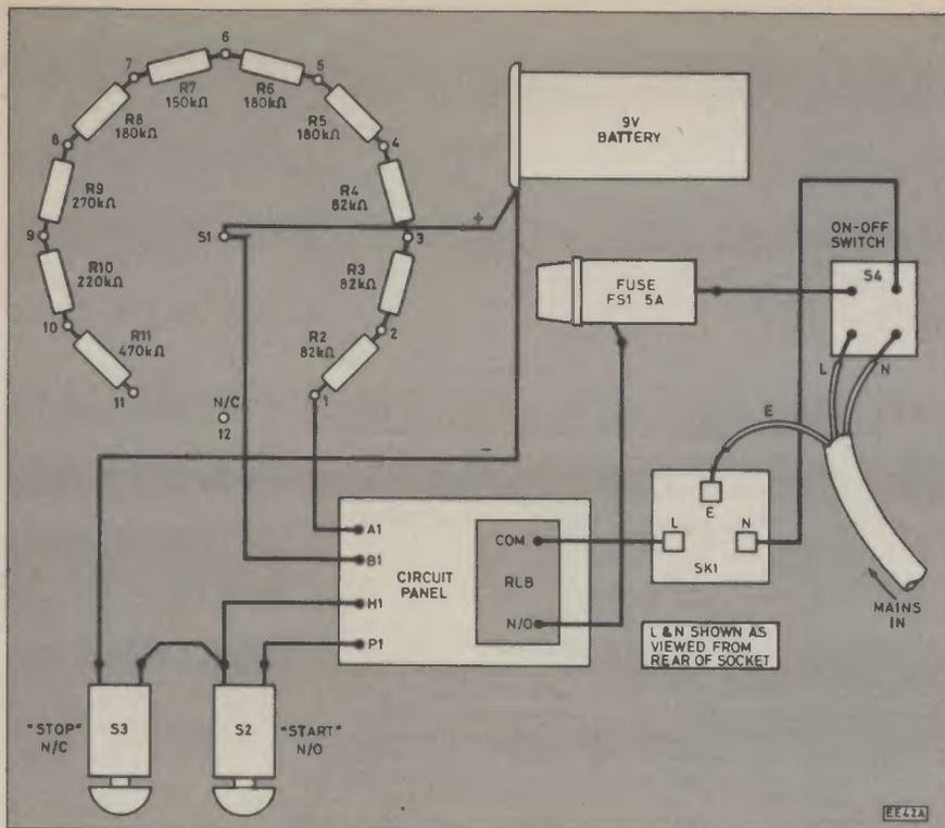
Fig. 2. Wiring details of the Kitchen Appliance Timer.
