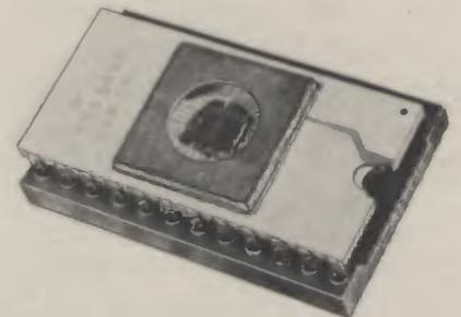
A typical UV EPROM, showing the circular quartz window above the memory circuit. When exposed to ultra-violet light, the whole memory is erased.
