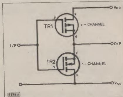
Fig. 4. CMOS inverter circuit.
