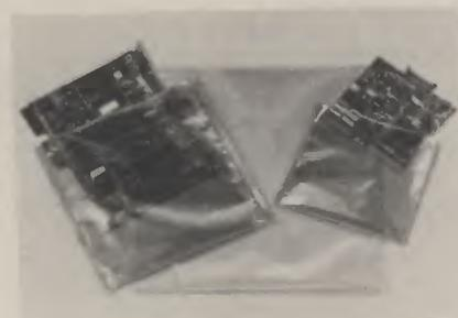
Anti-static packaging for circuits that include static-sensitive devices.
