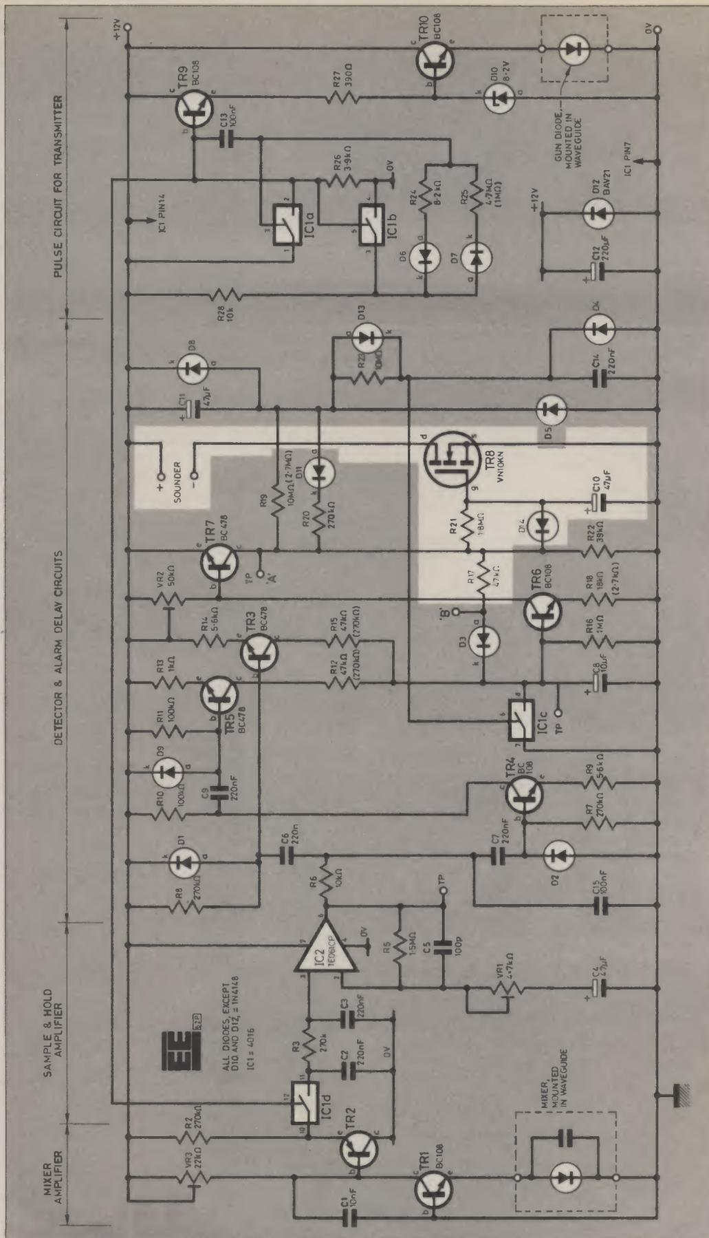
Fig. 4. Circuit diagram of the Microwave Intruder Alarm System as available from Avionic Systems. The non-tinted area shows the components which must be removed by the constructor when incorporating the adaptor kit featured in this article.
