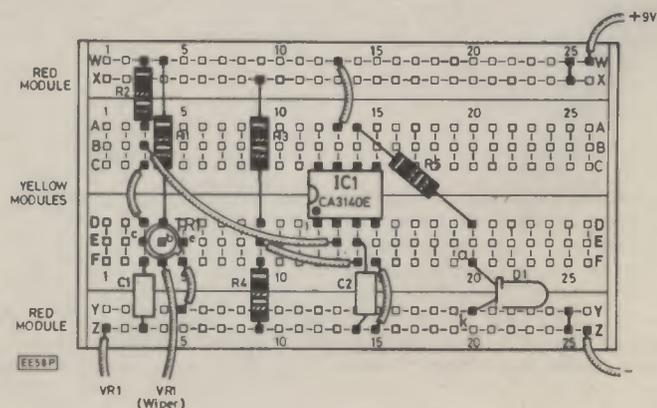
Fig. 11.3. EBBO i.c. board layout for Fig. 11.2.
