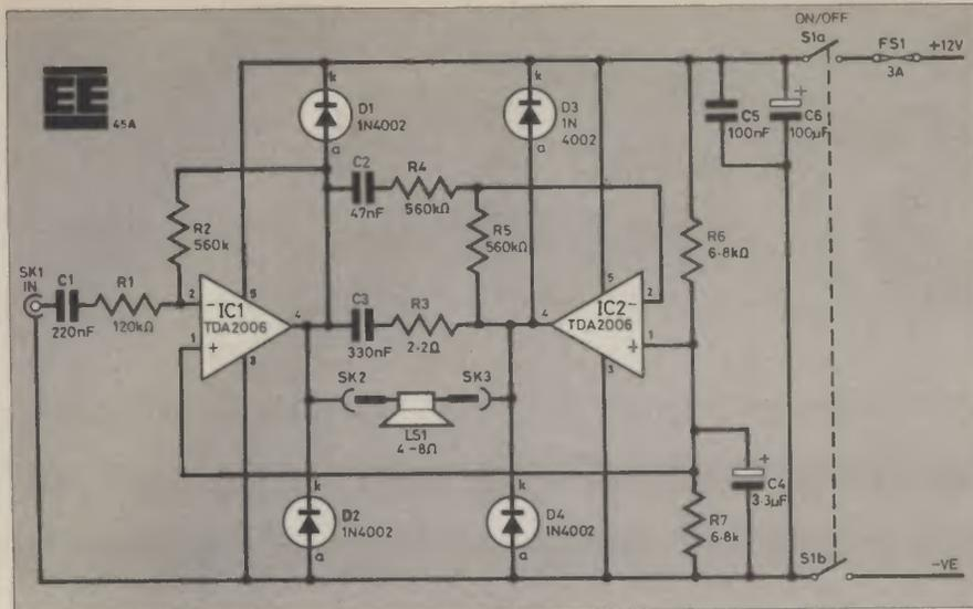
Fig. 2. Circuit diagram of the Car Radio Booster.
