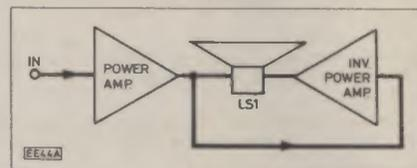
Fig. 1. Schematic diagram of bridge circuit.
