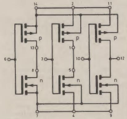
Fig. 3.6(b). The 4007 provides three inverters if its pins are connected as shown here.
