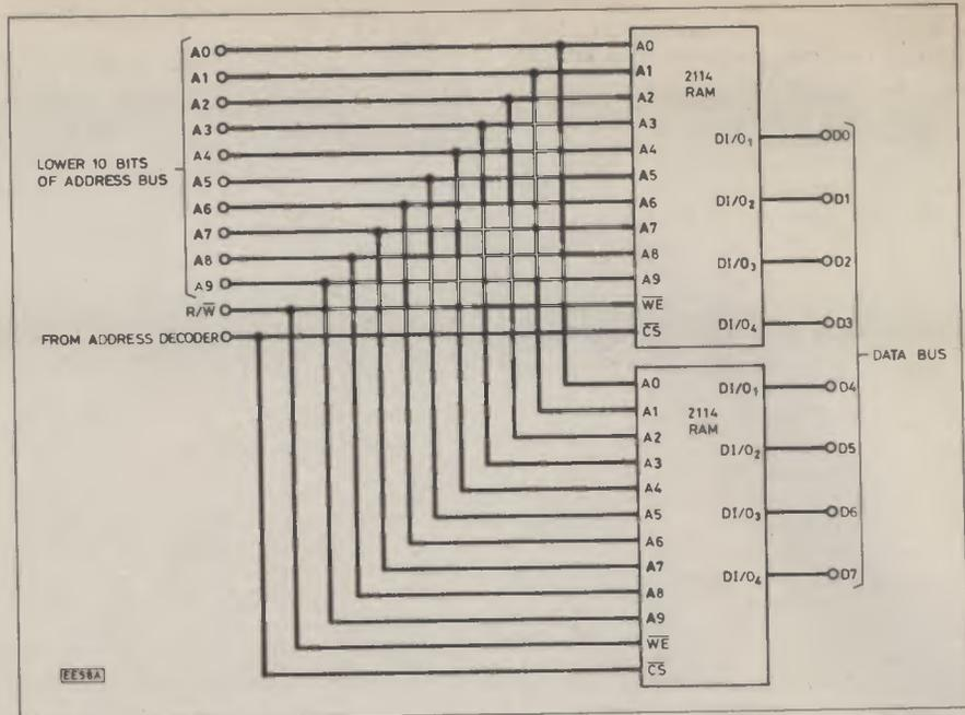
Fig. 2.3. Two 2114 RAM i.c.s wired to store 1 kilobyte of data.
