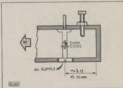
Fig. 2. Waveguide resonant cavity.
