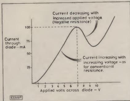
Fig. 1. Typical gunn diode negative resistance characteristics.
