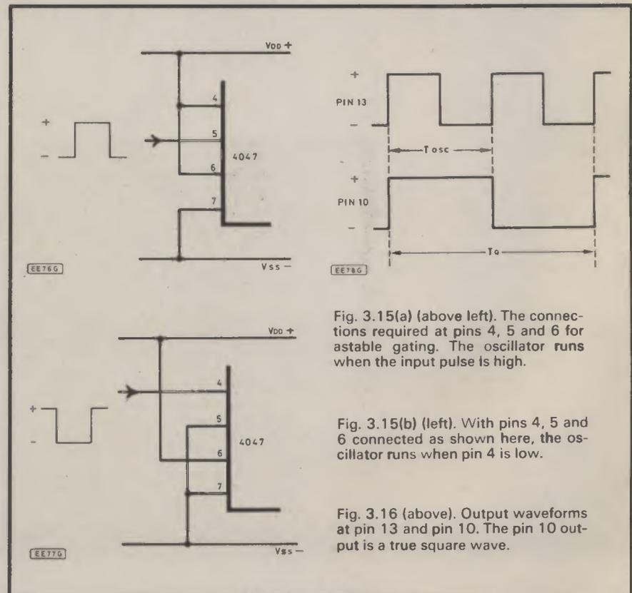
Fig. 3.15(a) (above left). The connections required at pins 4, 5 and 6 for astable gating. The oscillator runs when the input pulse is high.
