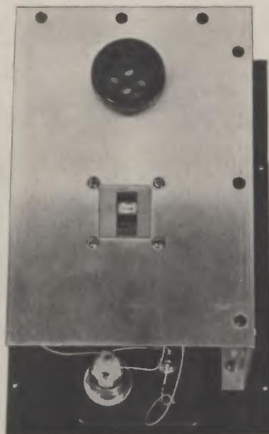
View, showing the gunn diode in its resonant cavity, and the audible sounder.
