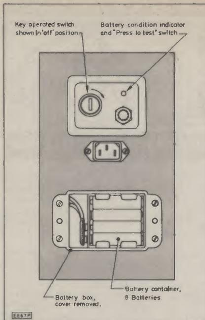
Fig. 10. Rear view of the unit, showing the added mains input socket.
