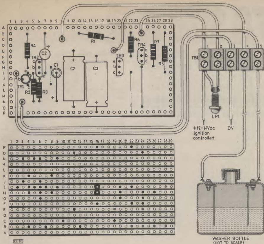
Fig. 2. Veroboard layout, wiring diagram and sensor construction.
