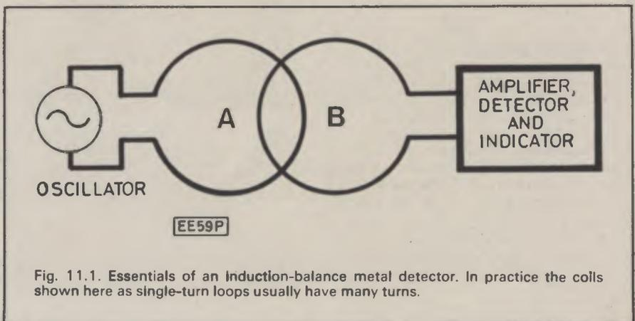
Fig. 11.1. Essentials of an induction-balance metal detector. In practice the coils shown here as single-turn loops usually have many turns.
