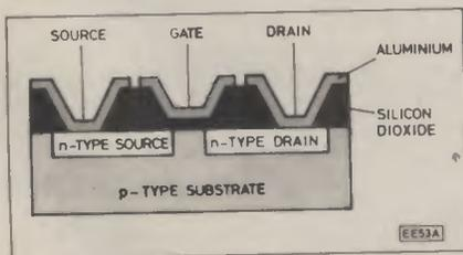
Fig. 1. Basic MOSFET structure.
