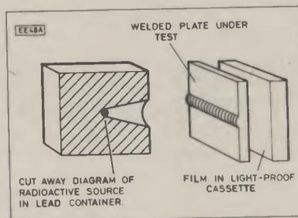
Gamma radiography: the first effect of radiation to be discovered is still used in industry to detect faulty welds.
