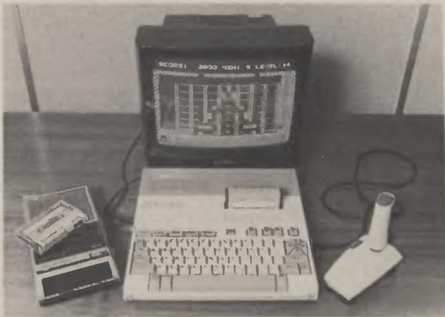
*The Hitachi H-1 model MSX microcomputer on which will be based the MB-H80 family computer for the UK market.*
