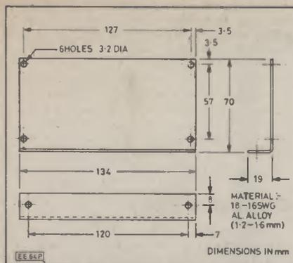
Fig. 9. Mounting bracket for the adaptor p.c.b.
