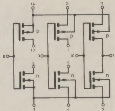
Fig. 3.6(a). The internal circuitry of the 4007.
