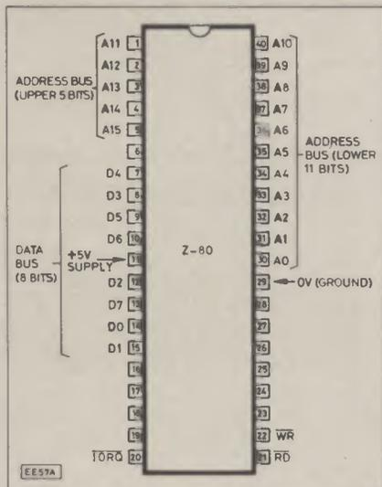
Fig. 2.1. The Z80 microprocessor, showing the connections referred to in the text.
