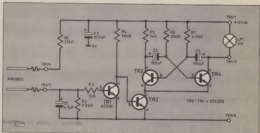
Fig. 1. Circuit diagram of Washer Fluid Monitor
