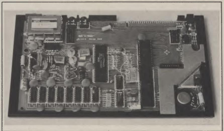
Inside the Sinclair ZX Spectrum. The three large chips are the microprocessor, Read-Only Memory, and an Uncommitted Logic Array (ULA). The ULA is a specialised device which takes the place of a large number of discrete logic components. The rest of the circuitry comprises the RAM chips, and the interfacing for the cassette recorder and TV output.
