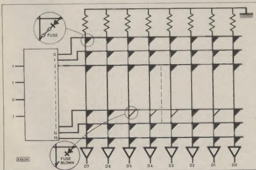
Fig. 2.6b. Programmed EPROM. Address 1101 (thirteen) is shown with fuses blown to give bit pattern 11000101 on the data bus.
