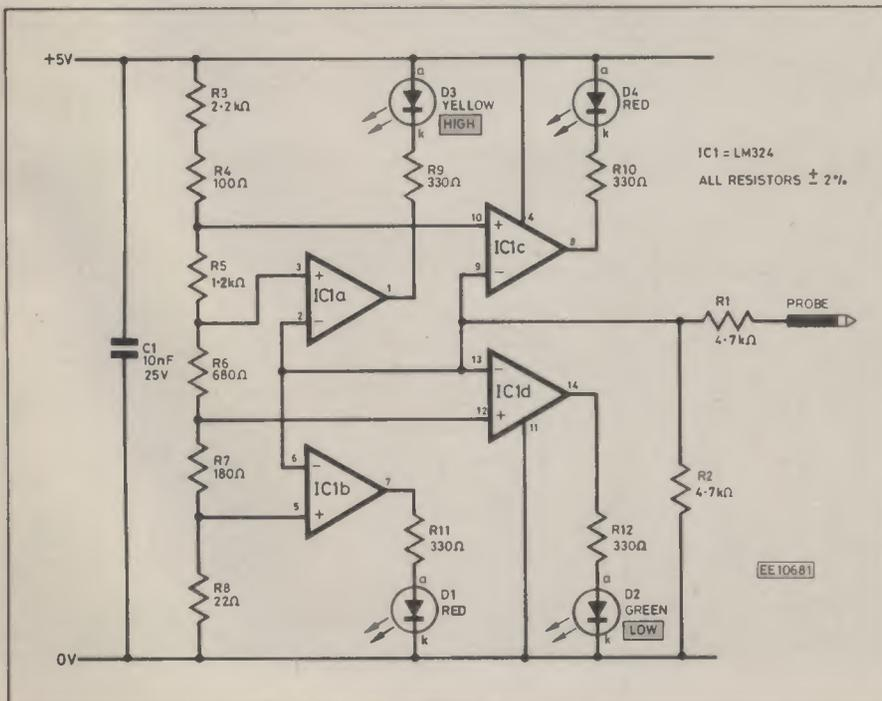
THE Intelligent Logic Probe, unlike any other probe I know of, can distinguish between a logic 0 and ground, or between logic 1 and Vcc. This is achieved by comparing various reference voltages with the probe voltage.
