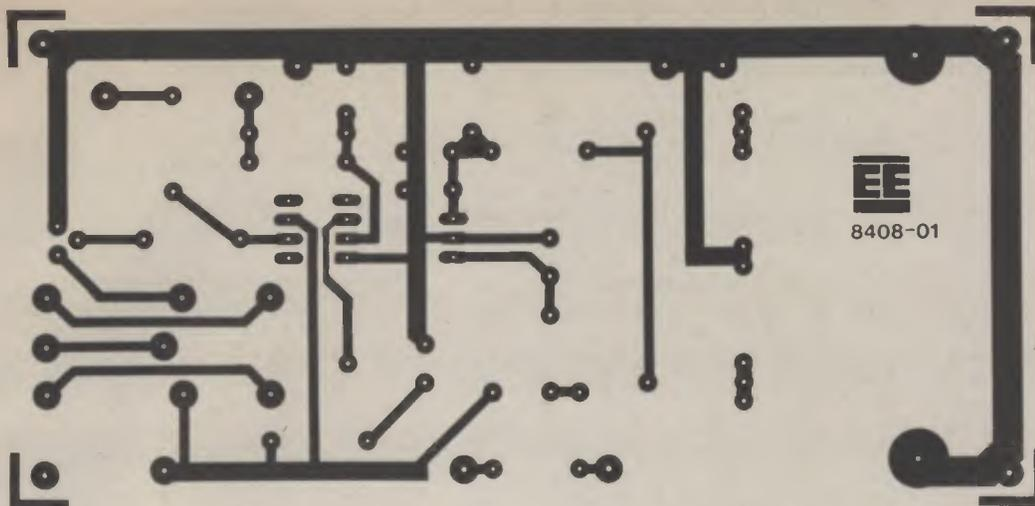
Fig. 7. P.c.b. layout of the adaptor board (actual size). This board is available from the *EE PCB service*, Order code 8408-01.
