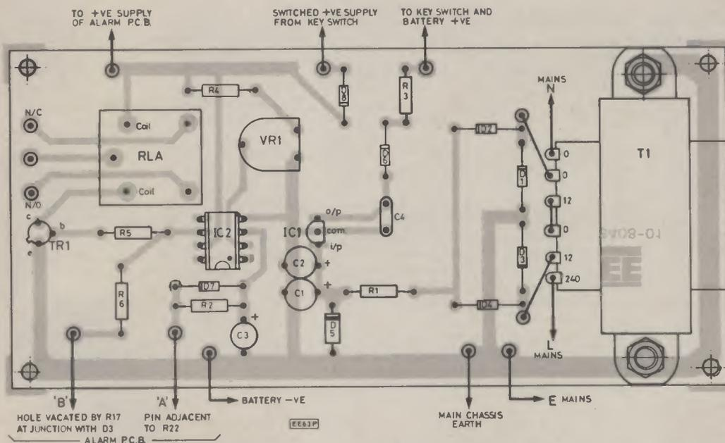
Fig. 8. Component layout of the adaptor board.
