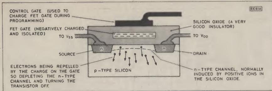
Fig. 2.5. MOSFET with isolated gate, as used in an EPROM.
