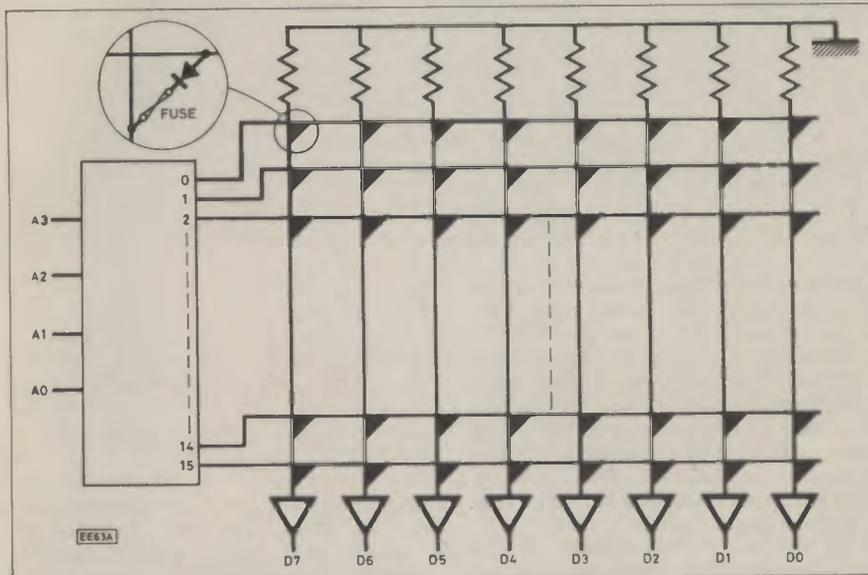
Fig. 2.6a. Unprogrammed 16-byte fusible-link PROM. The address decoder is part of the chip, and as any of the 16 rows is selected (addresses 0000 to 1111), the "1" on the output from the selected row of the address decoder will appear, via the diodes and fusible links as all "1s" on the data bus.
