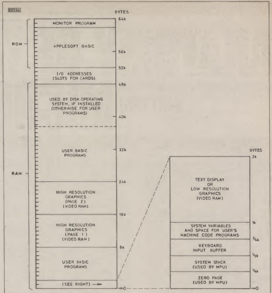
Fig. 2.2. The memory map of a Apple II. Apart from the lower 2K, the whole of RAM is available for BASIC programs, unless part of it is taken over for the Disk Operating System or for High Resolution Graphics. Note the relatively large amount of memory required for high-resolution colour graphics.
