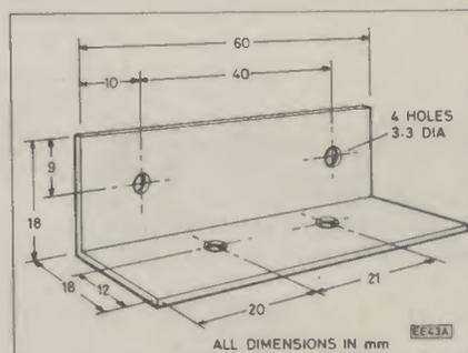
Fig. 3. Dimensions of mounting bracket/heatsink.
