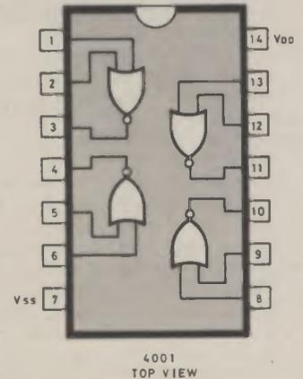
Fig. 3.7. The pin-outs of the 4011 quad NAND gate and the 4001 quad NOR gate.
