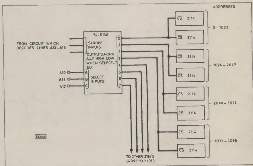
Fig. 2.4. Using the 74LS138 to decode the addresses for 1 kilobyte blocks of RAM.
