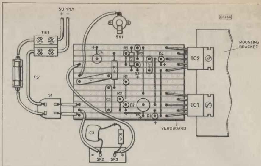
Fig. 4. Stripboard and wiring diagram.
