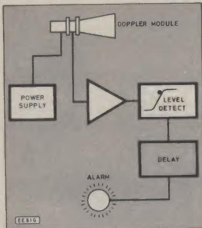
Fig. 5. Block diagram of the doppler module applications system.
