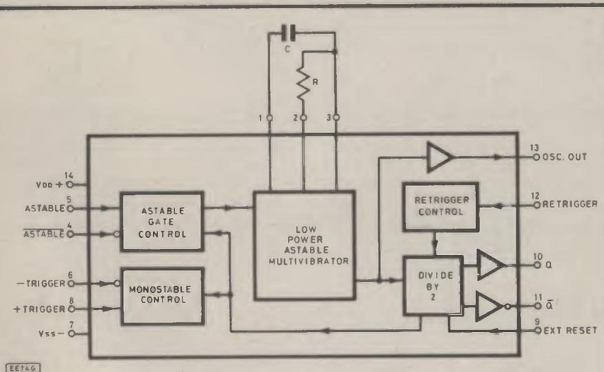
Fig. 3.13 (above). Block diagram illustrating 4047 internal logic circuitry.
