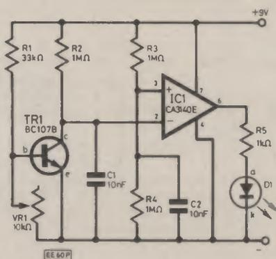
Fig. 11.2. Circuit of Temperature Alarm.
