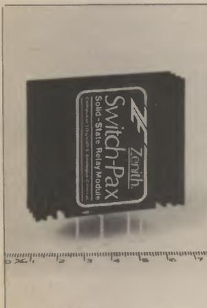
THE new range of Zenith I/O Modules are designed to interface between 5V logic microprocessor control systems and 240V mains and low voltage d.c. load devices. Optically isolated between Inputs and Outputs, the modules are moulded in epoxy compound and mounted on heavy duty heatsinks.
