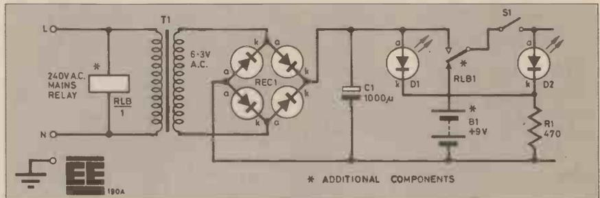
Fig. 7. Additional protection provided by 'mains fail' circuit.
