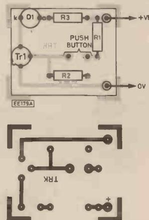
Fig. 3. Track layout and component overlay for the simple pushbutton circuit.
