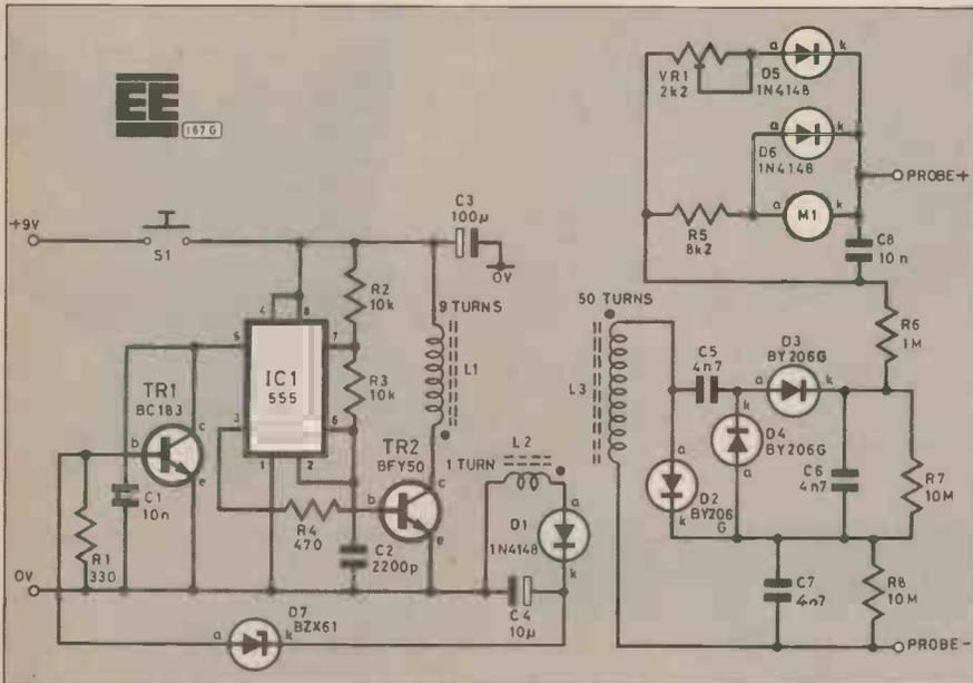
Fig. 1. Complete circuit diagram for the Insulation Tester.
