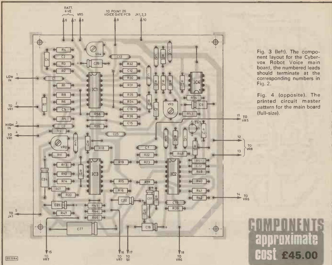
Fig. 3 (left). The component layout for the Cybervox Robot Voice main board, the numbered leads should terminate at the corresponding numbers in Fig. 2.
