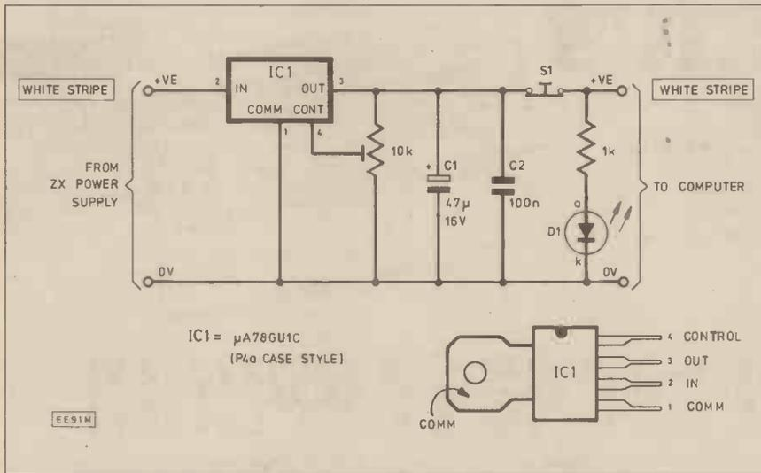
The ZX Power Supply Add-On also provides a reset facility.
