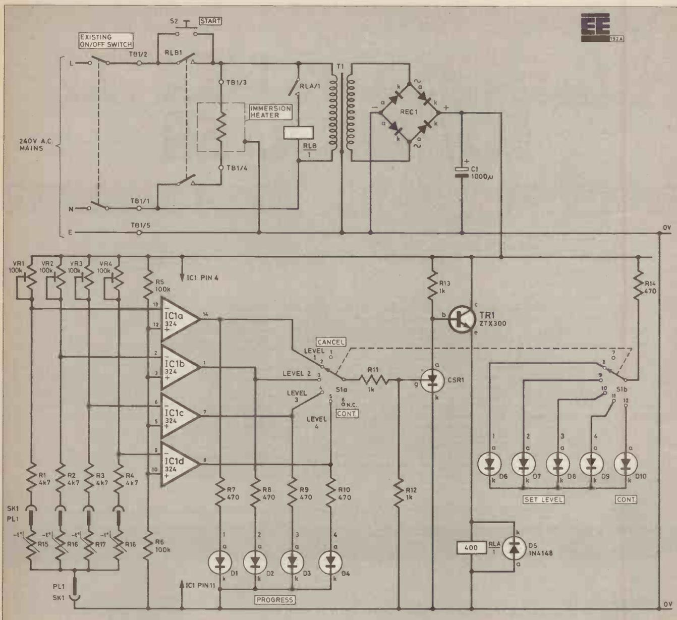
Fig. 1. Circuit diagram. Note: If the mains supply does not come from a 13A fused plug, then a fuse should be inserted in the supply LIVE wire.
