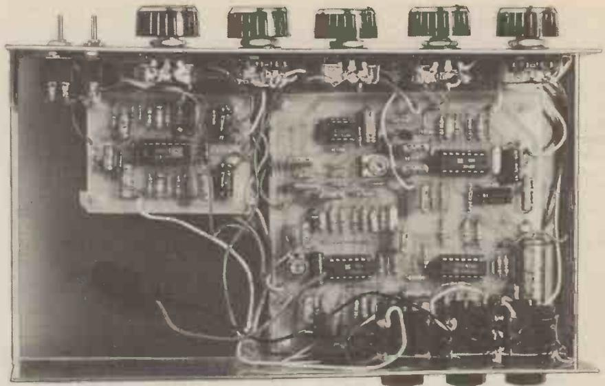
Internal view of the Cybervox Robot Voice with all interwiring complete.
