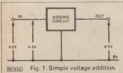
Fig. 1. Simple voltage addition.
