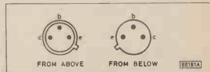
Fig. 2. Pin-out of BC109 from above and below the p.c.b.
