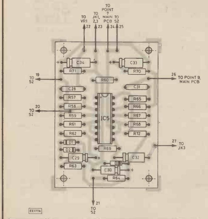
Fig. 5 (left). The layout of components on the topside and (below) actual-size master pattern for the Voice Gate board. See also previous page, for details of the internal layout and wiring.
