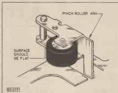
Fig. 2. Pinch roller assembly. Its surface should be flat. Clean with same solvent used for the heads.
