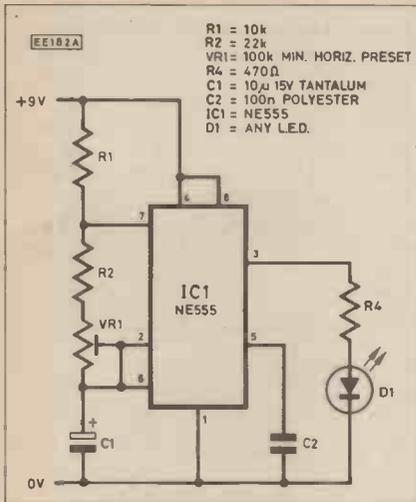
Fig. 4. Circuit diagram for i.e.d. flasher circuit.
