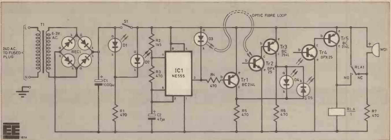
Fig. 2. Complete circuit diagram of the Fibelarm.
