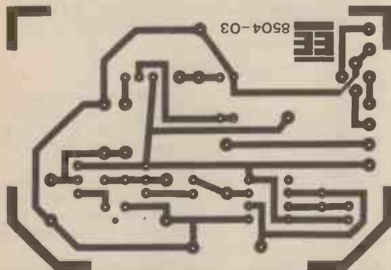
Fig. 3. Actual-size master pattern of the p.c.b. Available from EE PCB Service: Code 8504-03.
