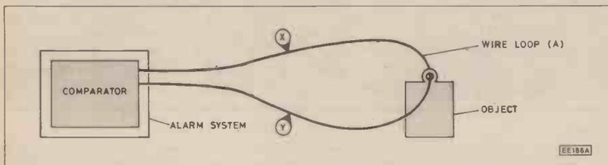
Fig. 1. Conventional loop alarm. The loop can easily be bridged between X and Y, which would foil the system.
