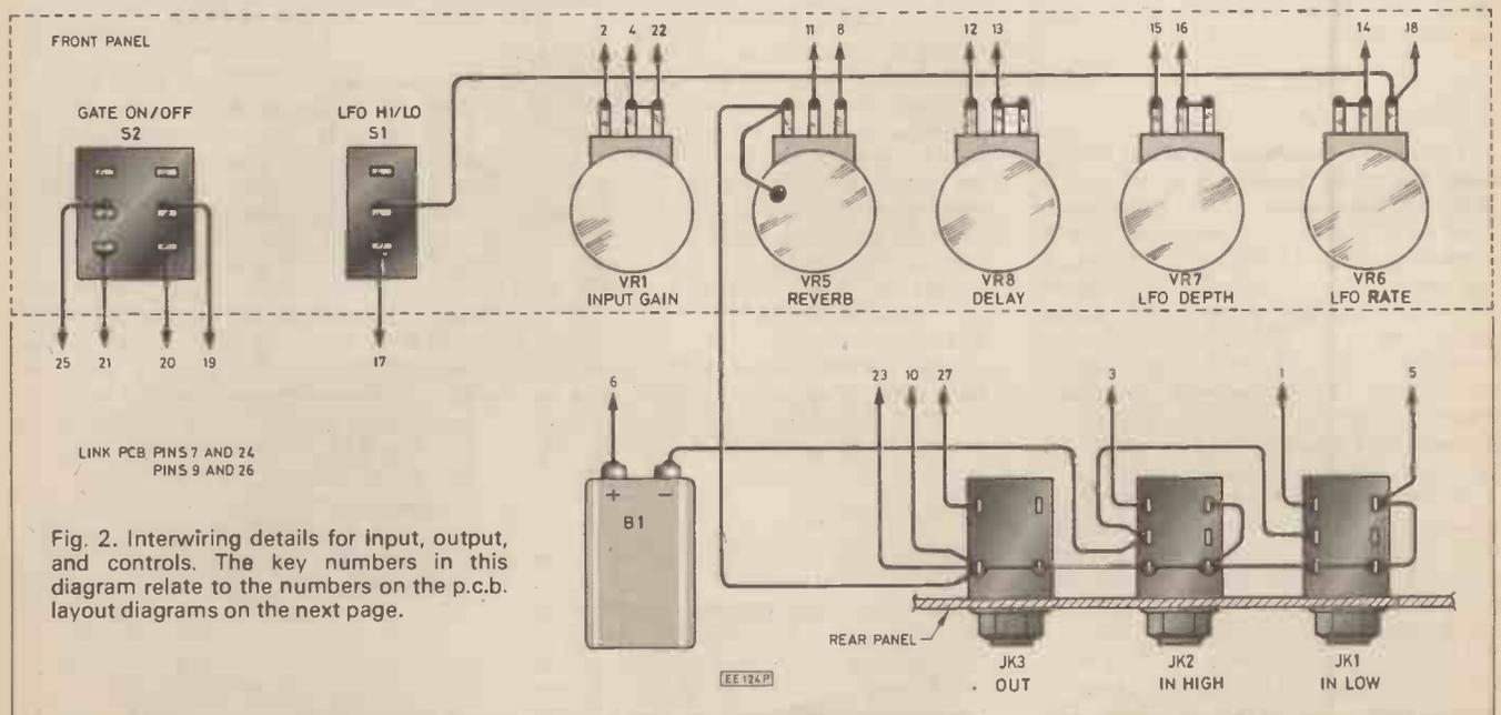
Fig. 2. Interwiring details for input, output, and controls. The key numbers in this diagram relate to the numbers on the p.c.b. layout diagrams on the next page.
