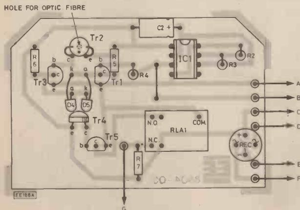
Fig. 4. Component layout of the Fibelarm.
