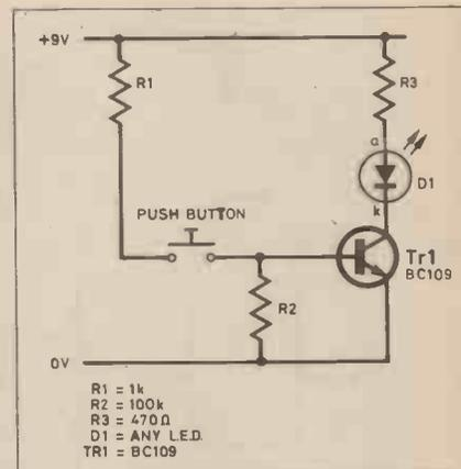
Fig. 1. Simple pushbutton circuit diagram.
