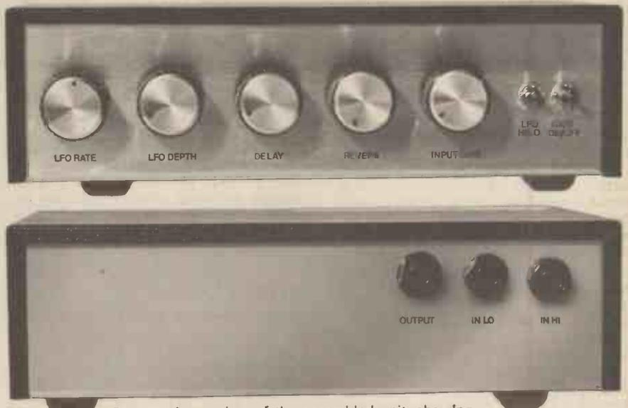
Front and rear view of the assembled unit, showing front panel controls, and the input and output jack-sockets on the rear panel.
