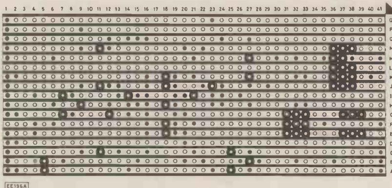
Fig. 2. Stripboard layout of Immersion Heater Controller.
