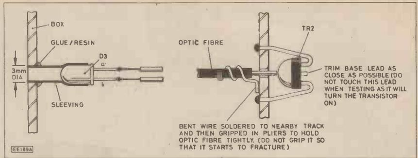
Fig. 6a. The sleeving mounted in the box.
