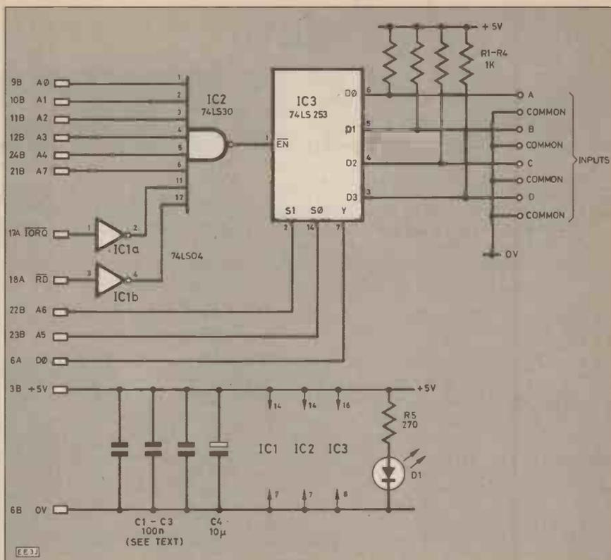
Fig. 1. Circuit diagram of the four-channel interface for the intruder-detection system.
