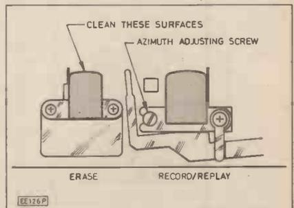
Fig. 3. Enlarged view of heads. These should be cleaned with a specialised head cleaning fluid, such as Bib Video head cleaning fluid.
