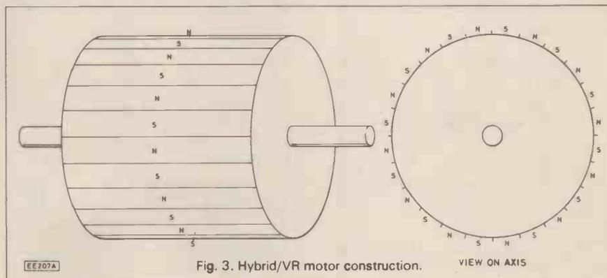
Fig. 3. Hybrid/VR motor construction.
