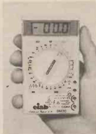
Nine functions and 29 measuring ranges are available from the multimeter. The resistance ranges are from 200 ohm to 20 megohm, in six switched ranges. The a.c. and d.c. amps ranges cover from 200µ to 200mA, in four ranges. There is also a position for 10A measurement.
