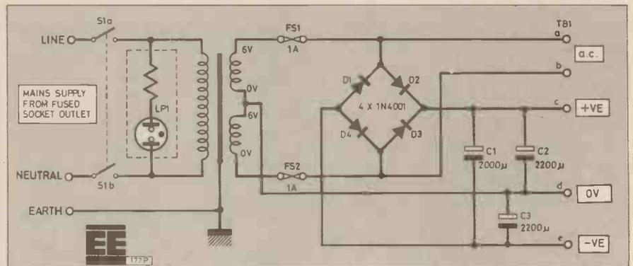
Fig. 11. Complete circuit diagram of the Low Cost PSU.
