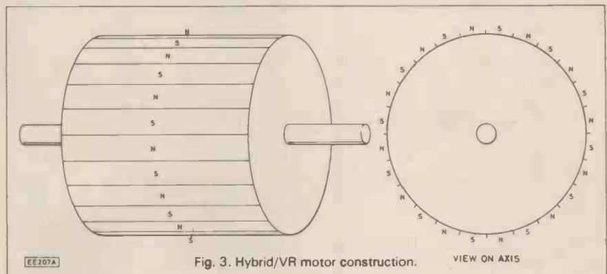
Fig. 3. Hybrid/VR motor construction.
