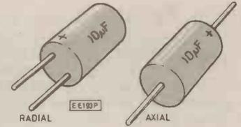
Fig. 9. Two types of electrolytic capacitor.
