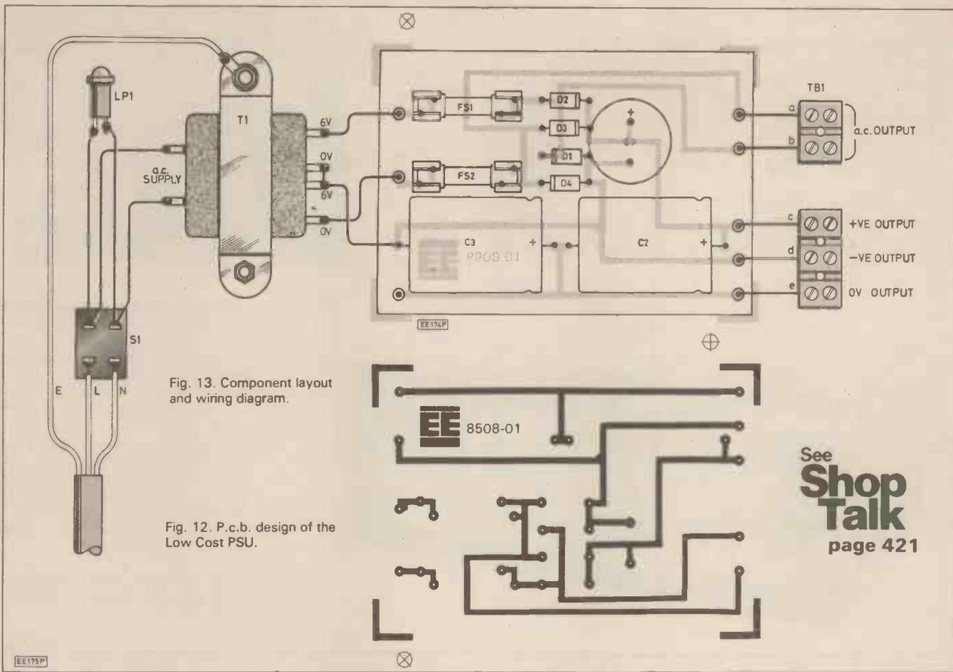
Fig. 13. Component layout and wiring diagram.
