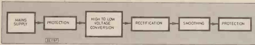
Fig. 4. Components of basic low voltage supply.
