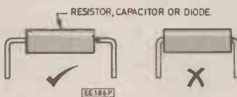
Fig. 3. The rights and wrongs of component lead forming.
