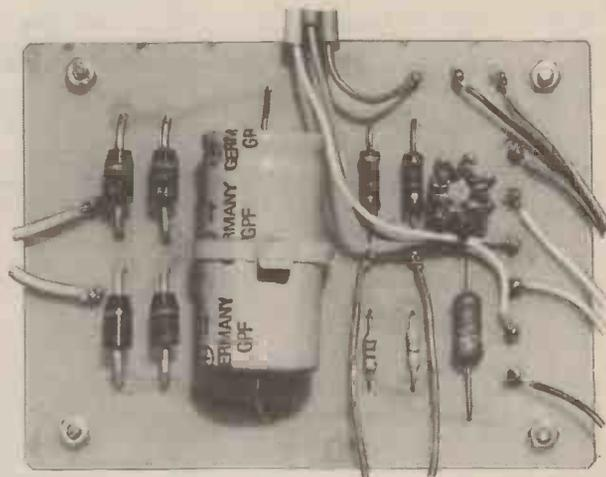
size. The tie-wrap passes around the capacitor and through holes in the p.c.b. on each side. Also, the transistor TR1 was fitted with a push-on T0-18 heatsink which will aid dissipation when the transistor is conducting.
