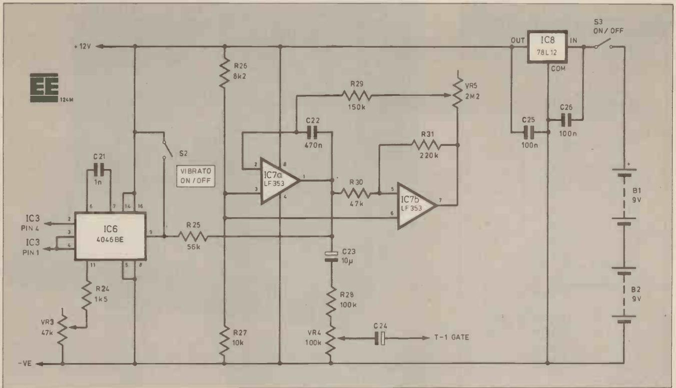
Fig. 3. Oscillator circuit diagram.
