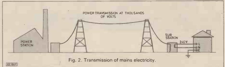
Fig. 2. Transmission of mains electricity.
