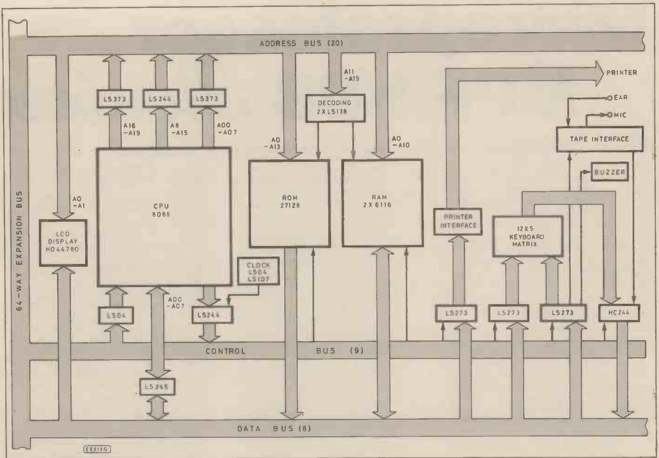
Fig. 1. Simplified block schematic of the MPF-I/88 hardware.
