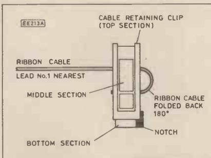
Fig. 7. IDC socket assembly.
