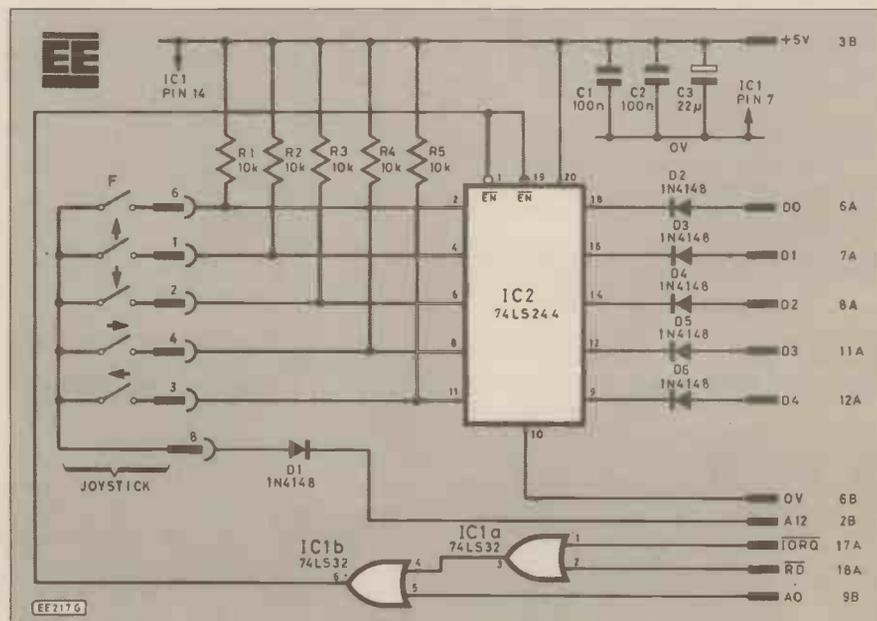
Fig. 2. Complete circuit diagram for the Joystick Interface.
