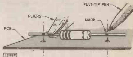
Fig. 5. Marking a component to fit its p.c.b. position.
