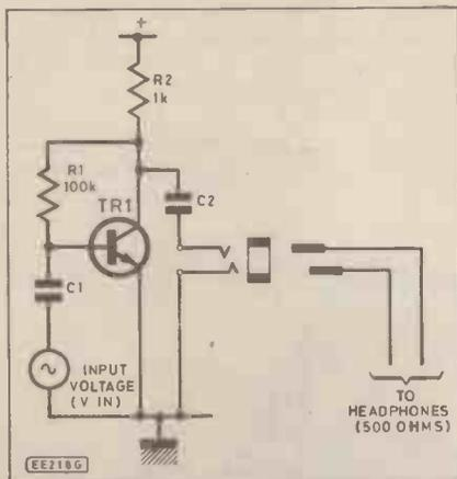
Fig. 1. Typical circuit for connection to an external load resistance.
