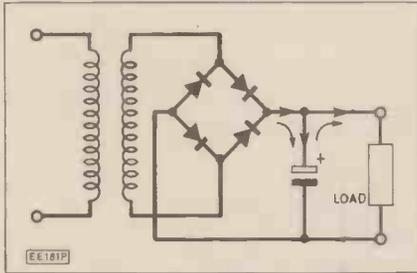
Fig. 9. The capacitor is supplied with energy.
