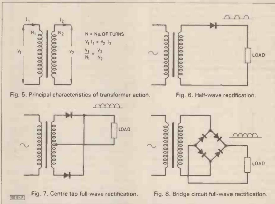
Fig. 5. Principal characteristics of transformer action.
