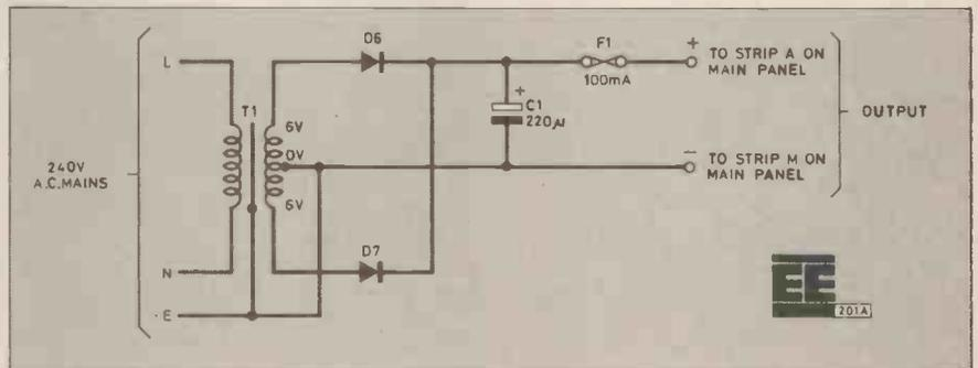
Fig. 2. Optional circuit for mains-powered operation.
