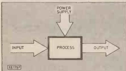
Fig. 1. Components of a basic system.
