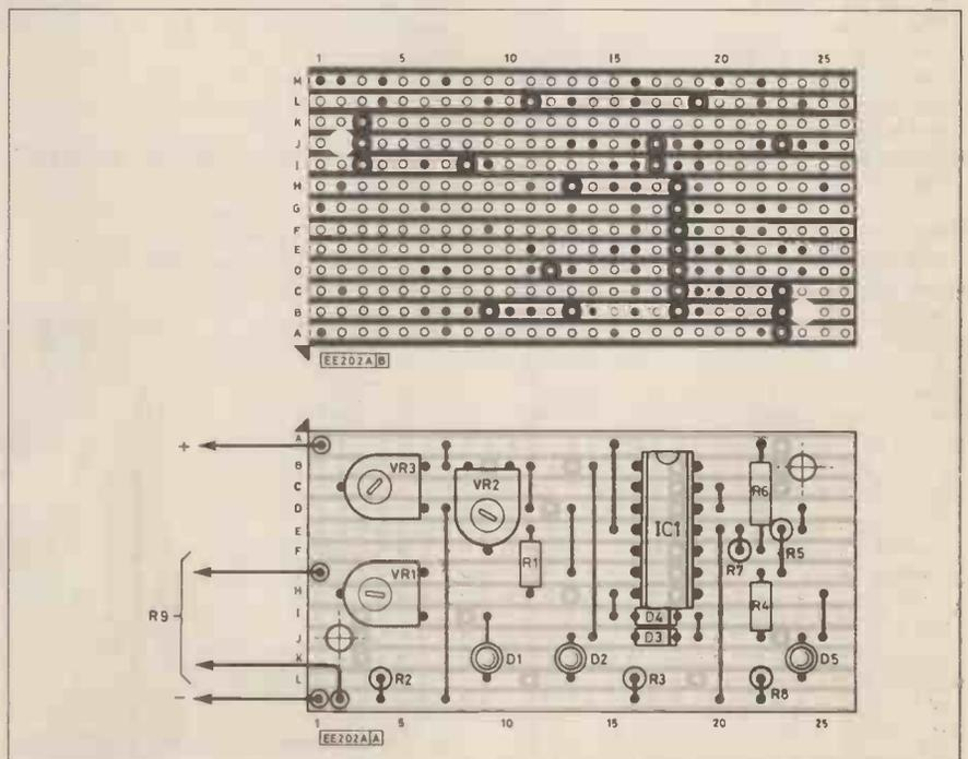
Fig. 3. Component layout and stripboard drilling details.
