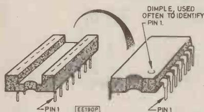
Fig. 2. Orientation of d.i.l. (dual in-line) i.c.s and their sockets. The end of the device which has the "nibble", or the "dimple", or both, is designated pin 1.
