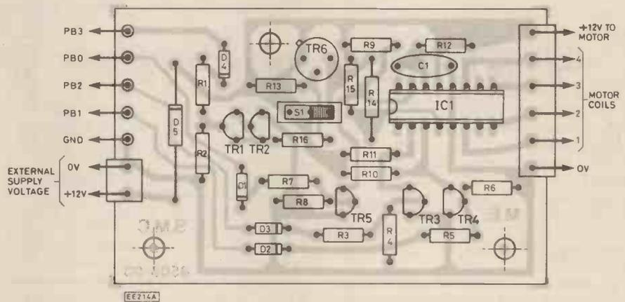
Fig. 6. Component layout for the Stepper Motor Interface.
