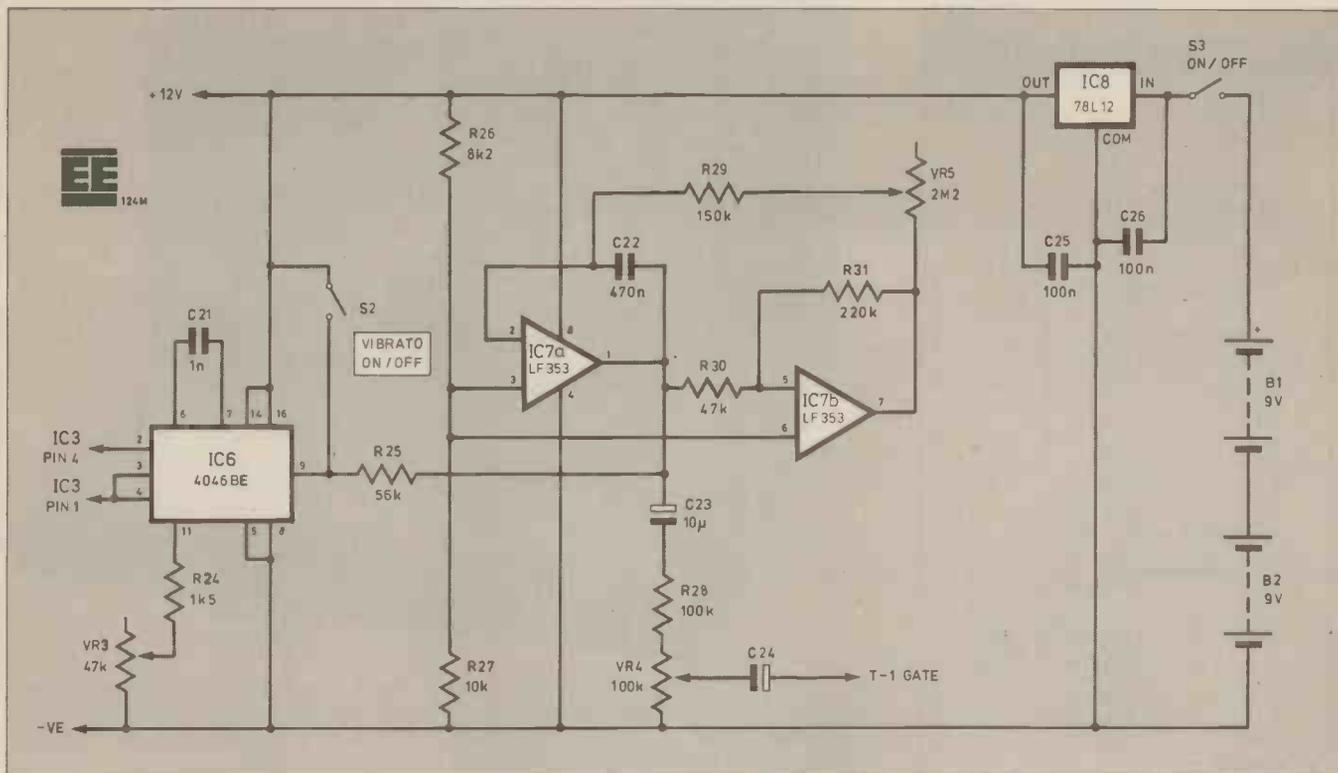
Fig. 3. Oscillator circuit diagram.
