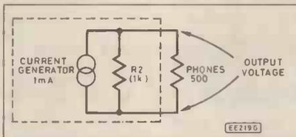
Fig. 2. Equivalent circuit in "current generator" form for the problem.
