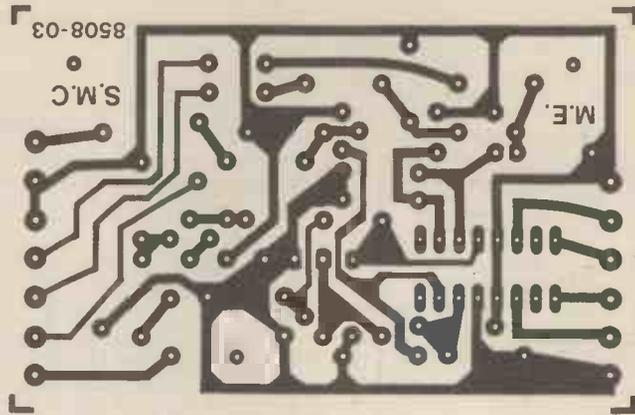
Fig. 5. P.c.b. design for the Stepper Motor Interface.
