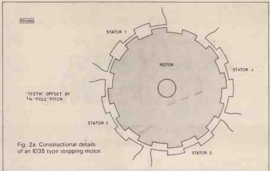
Fig. 2a. Constructional details of an ID35 type stepping motor.
