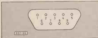
Fig. 3. Pin details for D-type connector.
