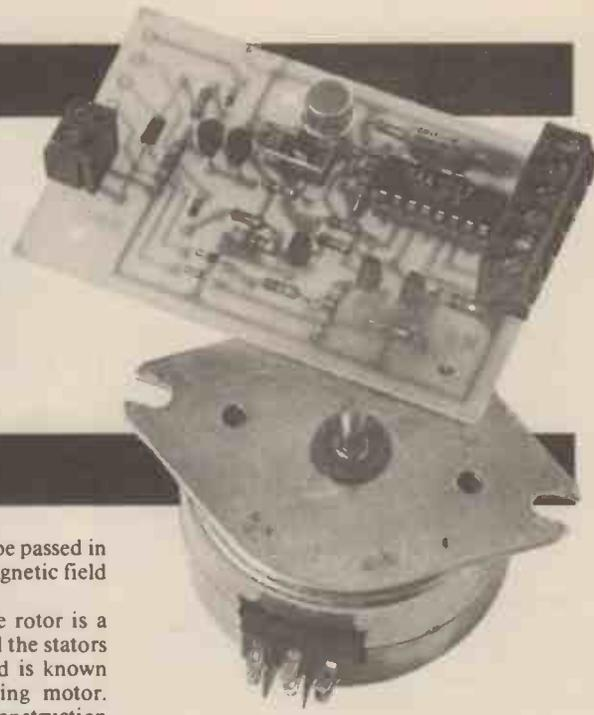
**S**TEPPING motors provide a very simple means of producing precise controlled movement from digital input signals. For this reason their use has become more and more common in all kinds of computer controlled mechanisms.
