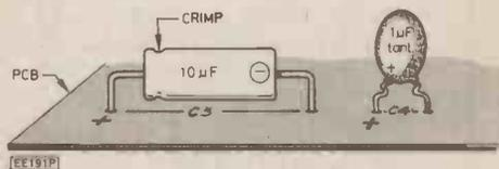
Fig. 6. Identifying the polarity of a typical electrolytic capacitor (left), and a typical tantalum (bead type) capacitor (right).
