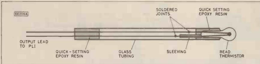
Fig. 7. Suggested arrangement for fixing the bead thermistor in a glass tube, to ensure good insulation.
