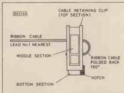
Fig. 7. IDC socket assembly.
