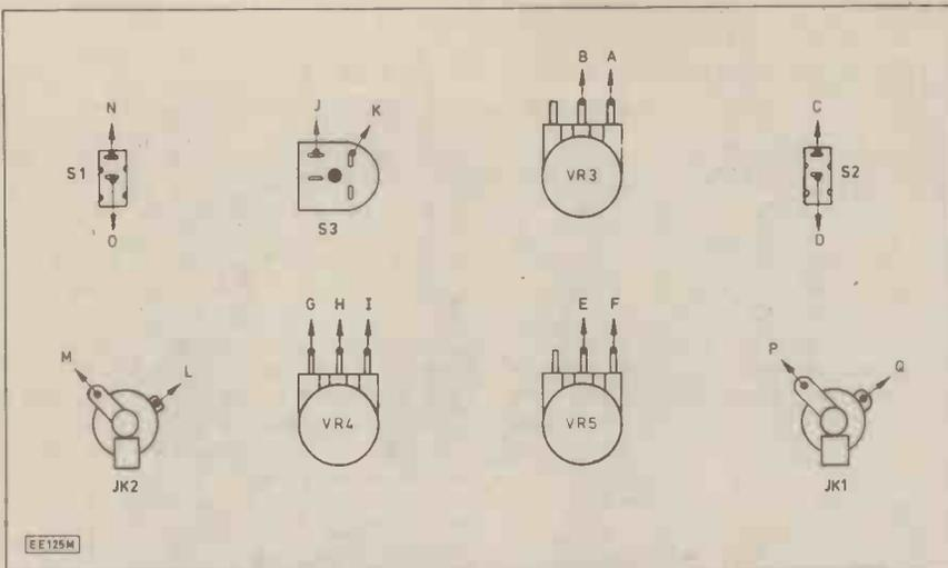
Fig. 5. Front panel wiring.
