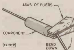
Fig. 4. When bending component leads, place a pair of pliers between the component body and the point on the lead to be bent.
