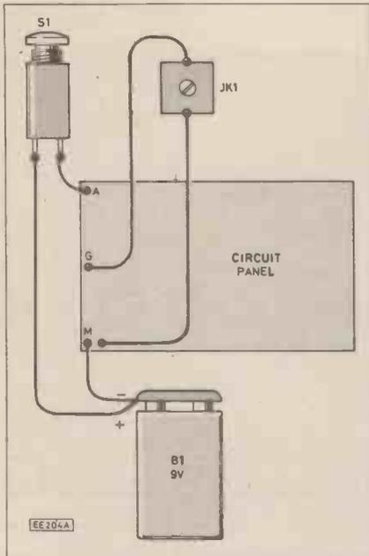
Fig. 4. Connections for battery operation.
