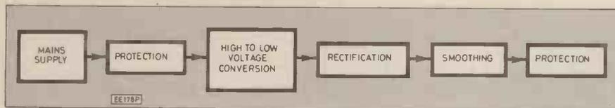
Fig. 4. Components of basic low voltage supply.
