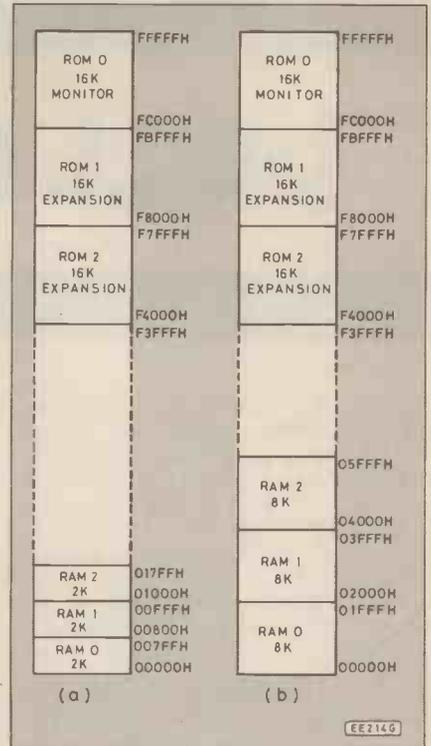
Fig. 2. MPF-I/88 Memory Map: (a) using standard 2k RAM chips, and (b) 8k chips.
