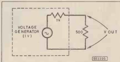
Fig. 3. A "voltage generator" circuit, which is an equally good conceptual arrangement of the actual circuit in Fig. 1.
