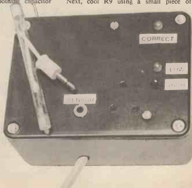
The enclosed unit with the temperature-sensing thermistor visible at the end of the glass rod.
