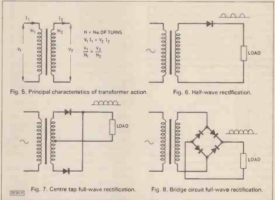
Fig. 5. Principal characteristics of transformer action.
