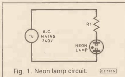
Fig. 1. Neon lamp circuit.
