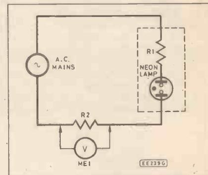
Fig. 3. Circuit for determining the approximate value of the ballast resistor.
