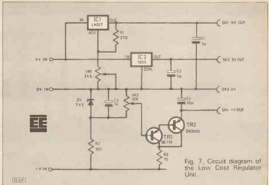
Fig. 7. Circuit diagram of the Low Cost Regulator Unit.
