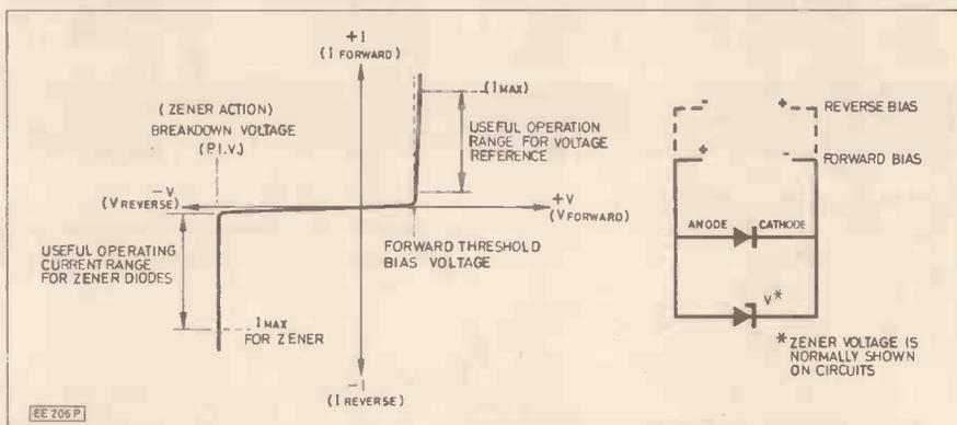
Fig. 2. Circuit symbols and diode characteristics.
