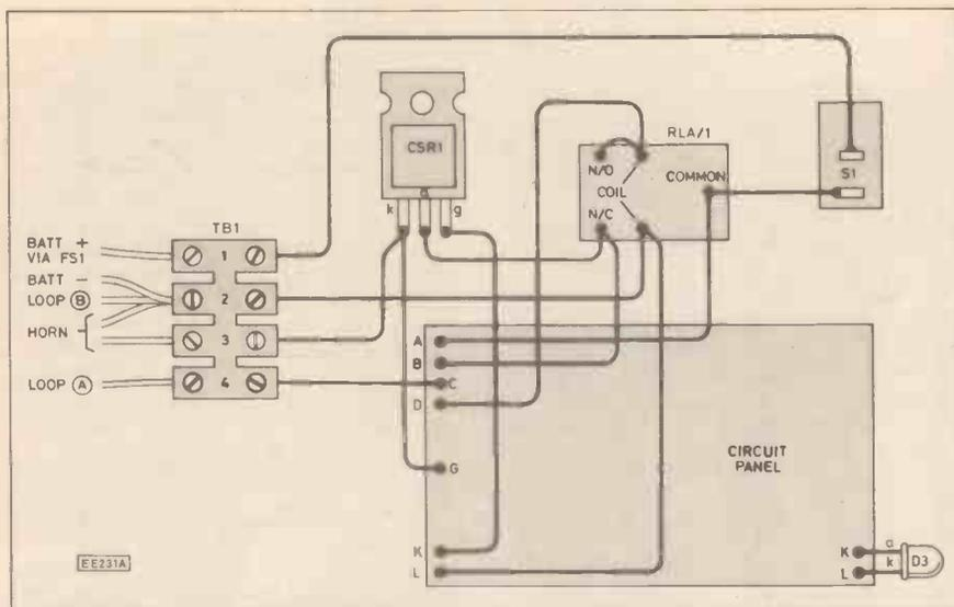
Fig. 3. Interwiring details for case mounted components. Note that the l.e.d. (D3) should be fixed using a plastic mounting clip.
