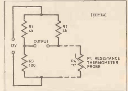
Fig. 1.3. Circuit diagram for a quarter bridge arrangement.
