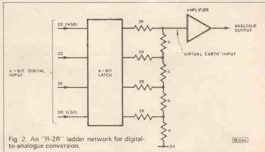
Fig. 2. An "R-2R" ladder network for digital-to-analogue conversion.
