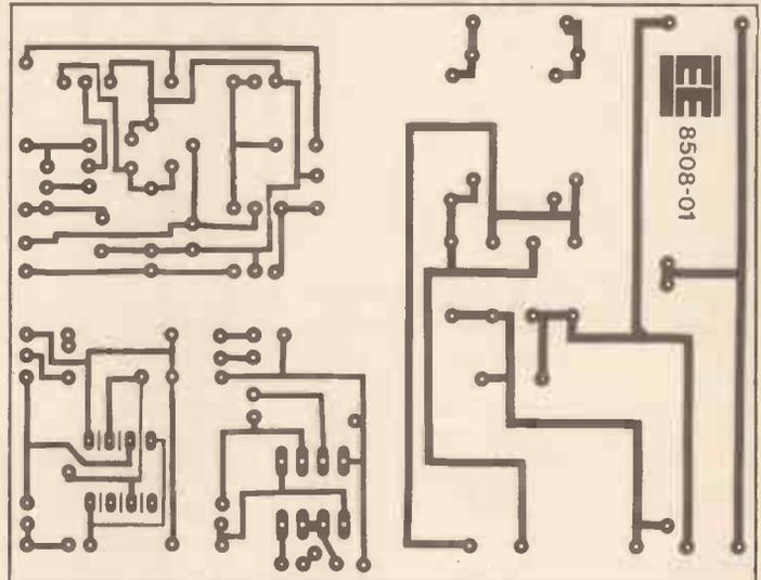
Fig. 8. P.c.b. design for four separate projects.
