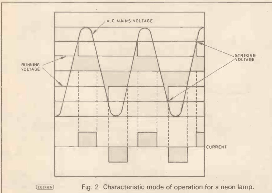
Fig. 2. Characteristic mode of operation for a neon lamp.
