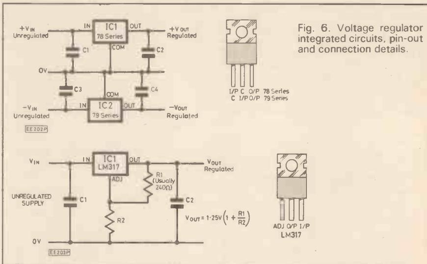
Fig. 6. Voltage regulator integrated circuits, pin-out and connection details.
