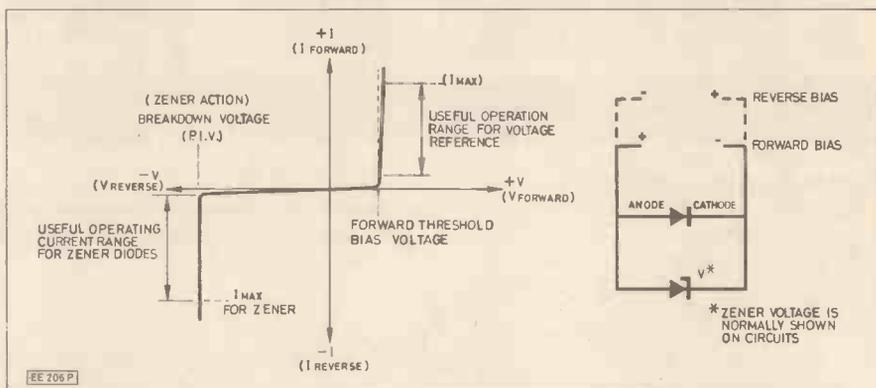
Fig. 2. Circuit symbols and diode characteristics.
