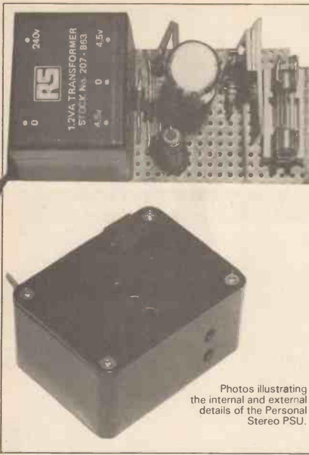
Photos illustrating the internal and external details of the Personal Stereo PSU.
