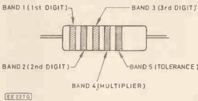
work out the value using the four band system, and then multiply this by ten to compensate for the ignored band.
