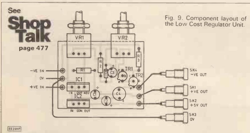
Fig. 9. Component layout of the Low Cost Regulator Unit.
