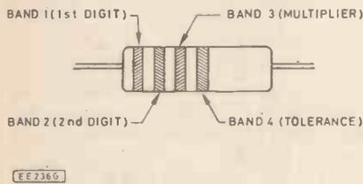
**Fig. 1. Four and five band resistor colour codes. Do not assume that a resistor having a similar code to the one you require will have a similar value. If the "multiplier" is wrong the value will be wrong by a factor of at least ten.**
