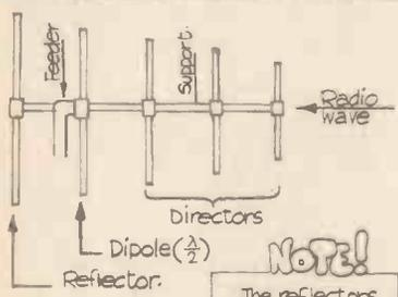
Transmission and reception are improved when 'director' and reflectors are added to the dipole. For transmitting aerials they have the effect of concentrating the radiation in one direction. For receiving aerials they have the effect of concentrating the strength of the received signal.
