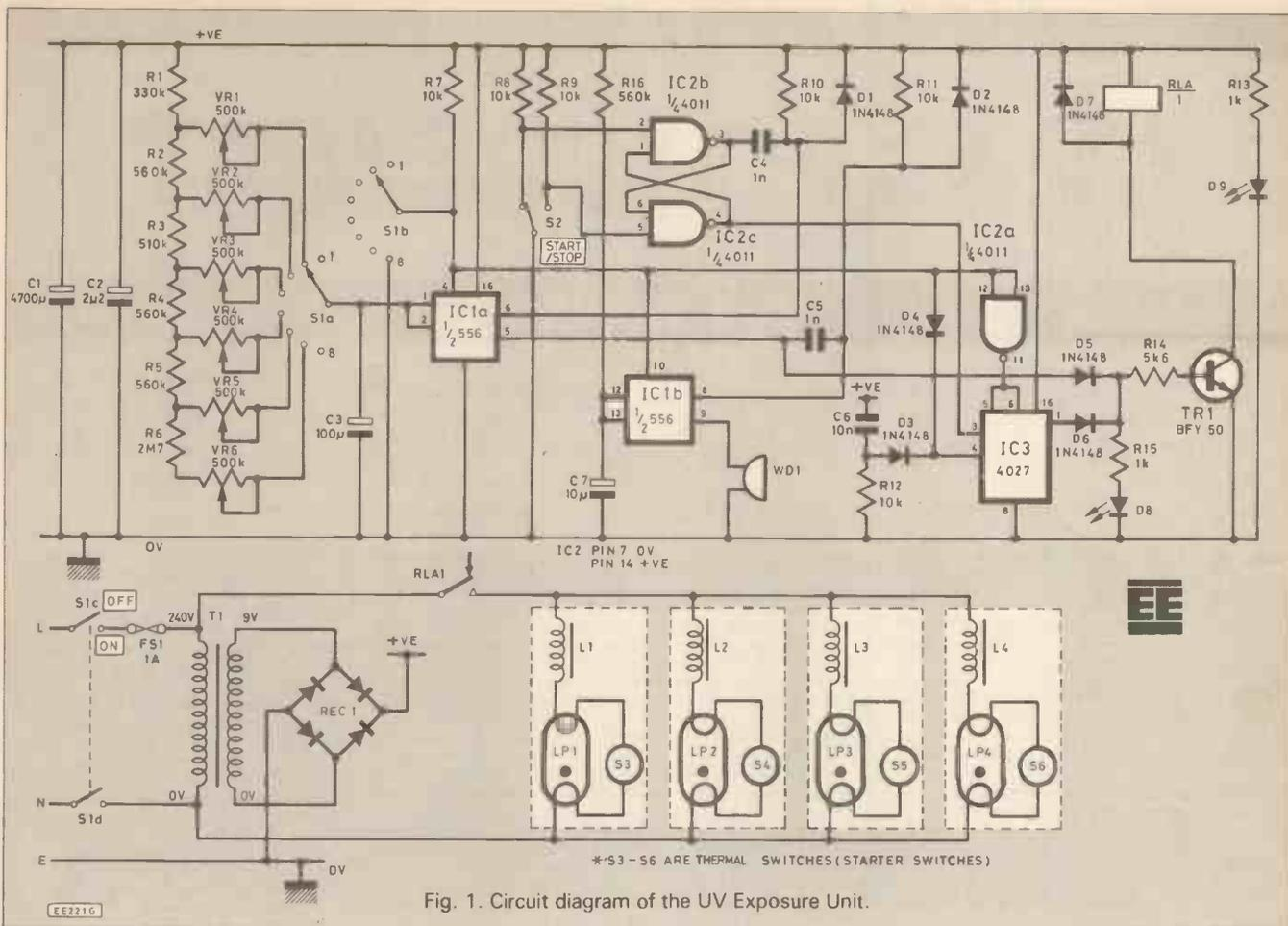
Fig. 1. Circuit diagram of the UV Exposure Unit.
