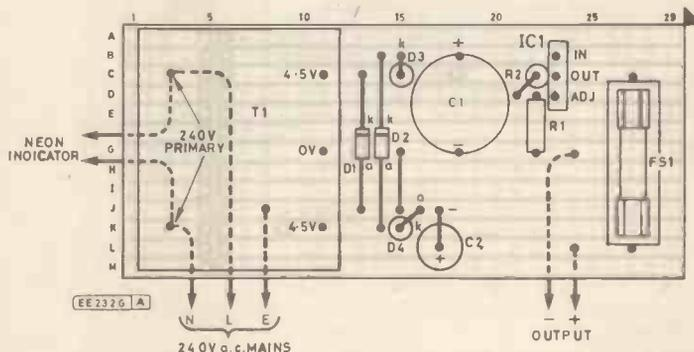
Fig. 3. Component layout of the Personal Stereo PSU.
