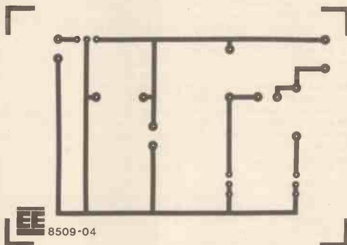
Fig. 1.10. Full size printed circuit board master for the Semiconductor Temperature Sensor. This board is available from the *EE PCB Service*, order code: 8509-04.
