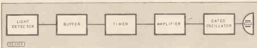
Fig. 1. Block diagram of the Fridge Alarm.
