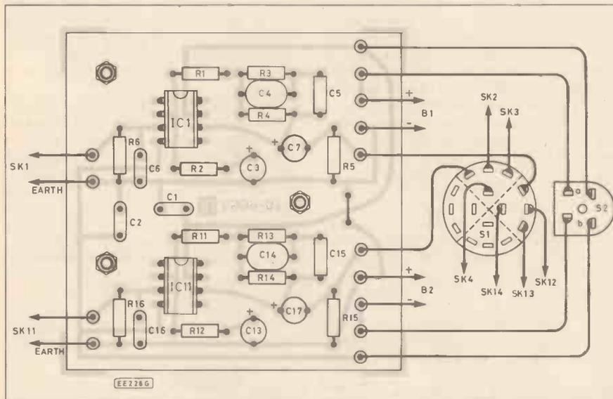
Fig. 4. Layout and wiring of the unit
