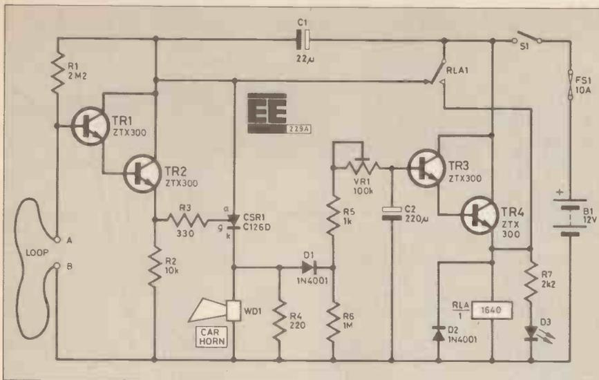
Fig. 1. Complete circuit diagram for the Caravan Alarm.
