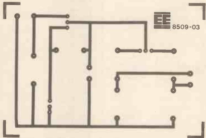
Fig. 1.7. Full size printed circuit board master for the Resistance Thermometer. This board is available from the *EE PCB Service*, order code: 8509-03.
