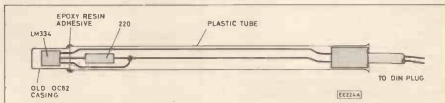
Fig. 1.11. Suggested probe assembly for the LM334.
