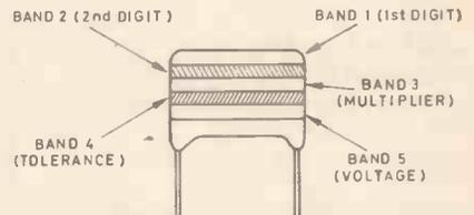
**Fig. 2. C280 capacitor colour coding. This first three bands give the value (in pF) using the same system as for the four band resistor coding.**
