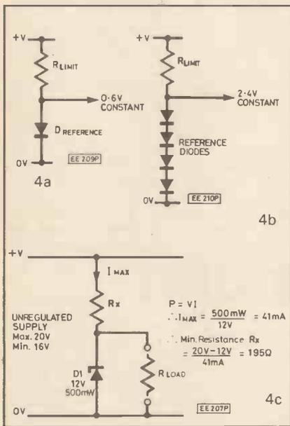
Fig. 4. Diode voltage references.
