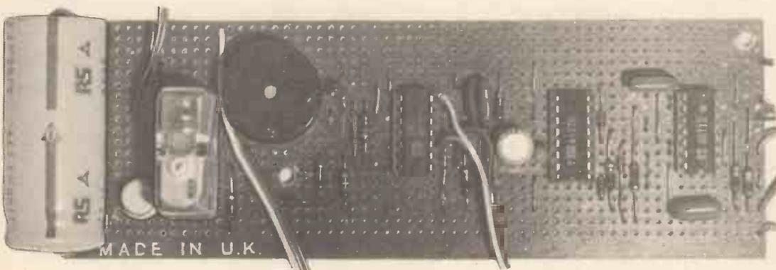
Main stripboard layout showing the position of C1, the p.c.b. mounted relay and AWD1.
