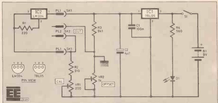
Fig. 1.8. Circuit diagram for the Semiconductor Temperature Sensor using the LM334.
