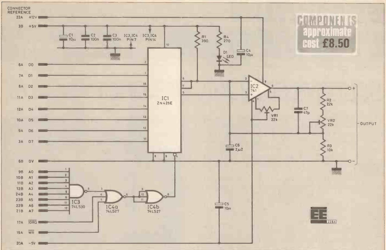
Fig. 3. Complete circuit diagram for the converter, using address 255 decimal.
