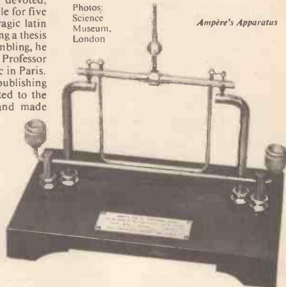
later on 18 September he presented to the academy the results of his experiments which showed that when electric current is passed through two parallel wires in the same direction they are attracted, and when the current flows in opposite directions they repulse.
