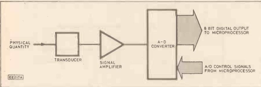
Fig. 1.2. Microprocessor interfacing using an A to D converter.
