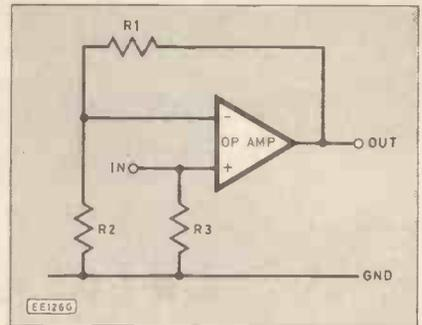
Fig. 2. Op.amp non-inverting mode configuration
