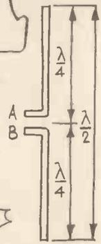
For maximum radiated and received energy, the aerial has to be a optimum length, equal to half the wave length of the signal.
