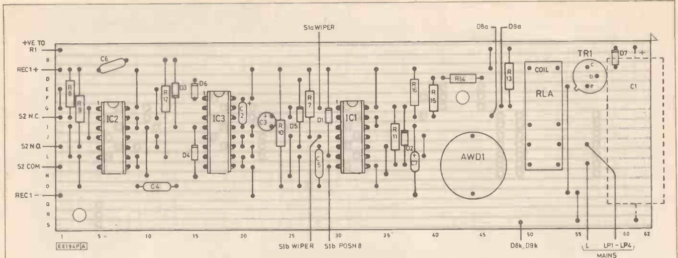
Fig. 2. Main stripboard layout and track details.
