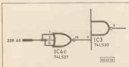
Fig. 4. Example of circuitry for decoding for port address 191 decimal.
