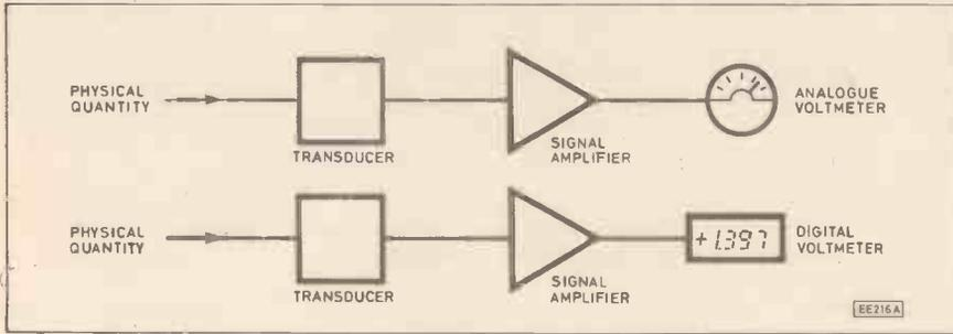
Fig. 1.1. Block diagrams for analogue and digital readouts.
