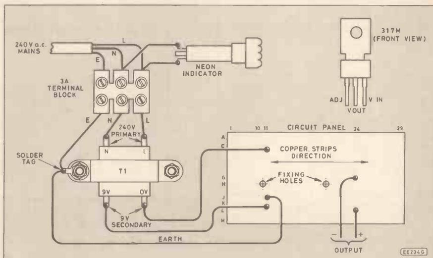
Fig. 4. Alternative transformer wiring details for the Personal Stereo PSU. The same stripboard is used.
