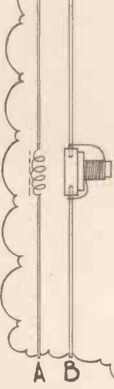
To match an aerial to a I.F. wave length particularly in a portable situation becomes impractical. Shorter aerials can be used by increasing the electrical length of the aerial by loading with a coil.
