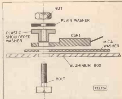
Fig. 4. Method of fixing the thyristor (CSR1) on the case using the mounting kit.
