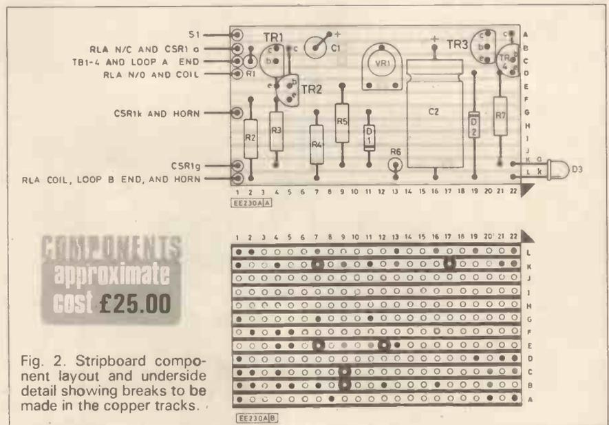
Fig. 2. Stripboard component layout and underside detail showing breaks to be made in the copper tracks.
