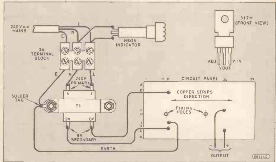
Fig. 4. Alternative transformer wiring details for the Personal Stereo PSU. The same stripboard is used.
