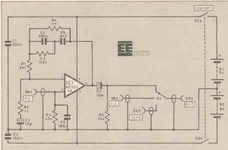
Fig. 3. Circuit for one channel of the RIAA Preamp Input Selector
