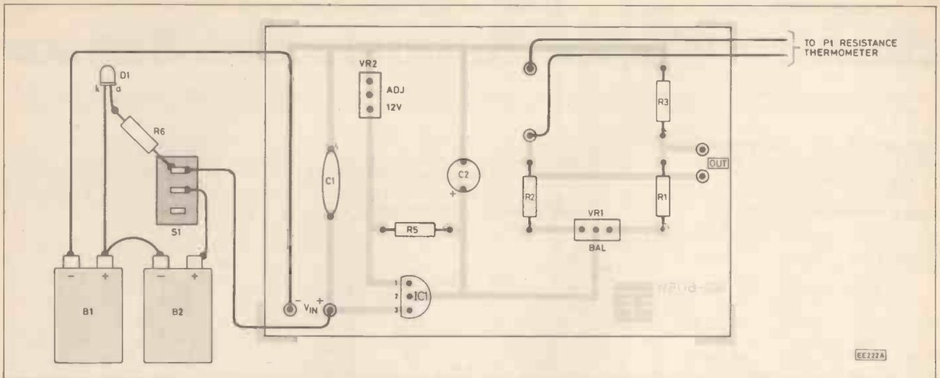
Fig. 1.6. Component layout and interwiring for the Resistance Thermometer.
