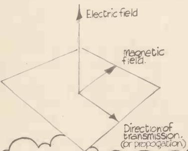
A vertical aerial creates a VERTICAL electric field and the radiation is said to be vertically polarised.
