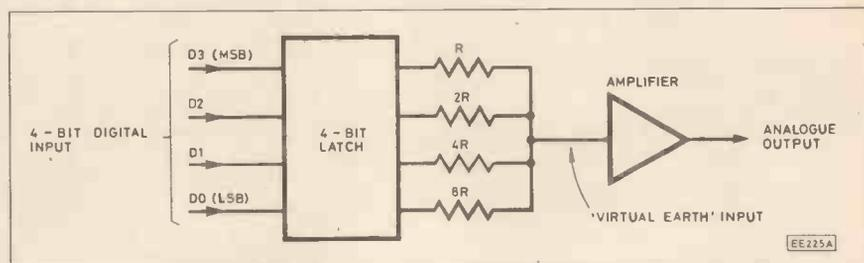
Fig. 1. Binary-weighted resistor network for D-to-A conversion.
