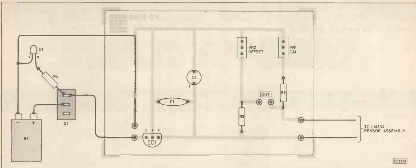
Fig. 1.9. Component layout and interwiring for the Semiconductor Temperature Sensor.
