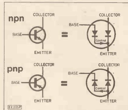
Fig. 3. Transistor action.
