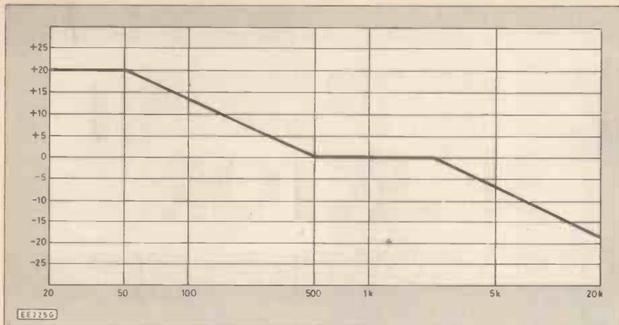
cut right through the master disc. Obviously the problem could be overcome simply by reducing the amplitude of the whole signal, but this would give an unacceptable reduction in the signal to noise ratio of around 20dB. By only reducing the amplitude of low frequency signals the signal to noise ratio only deteriorates at these frequencies. While even this loss of performance is undesirable, it does not prevent excellent results from being obtained in practice.
