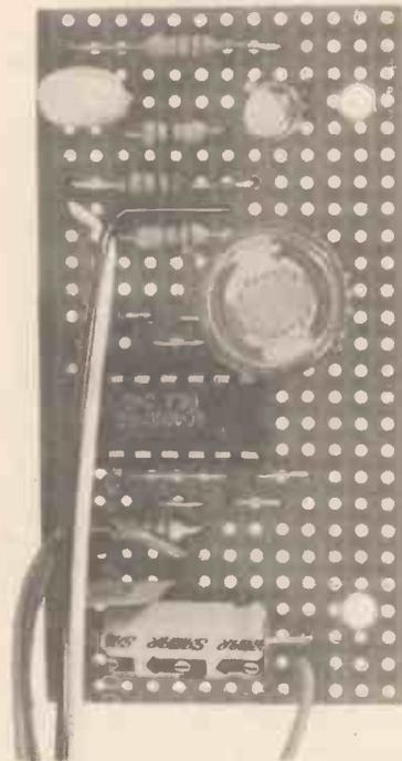
Fig. 3. Veroboard layout and wiring for the Fridge Alarm.
