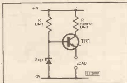
Fig. 5. Simple transistor regulator.
