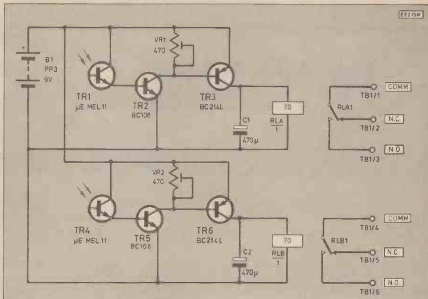
Fig. 2. Circuit diagram for a two-channel Oport.
