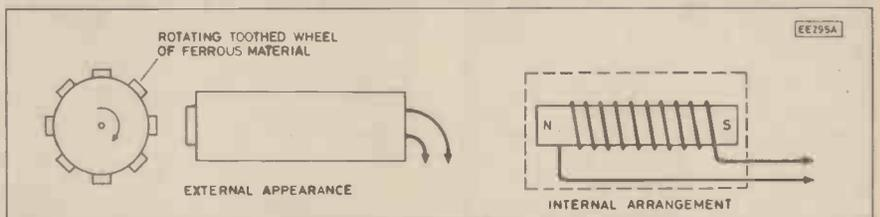
Fig. 5.2. Magnetic pick-up used for speed sensing.
