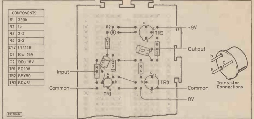
Fig. 4.17. Wiring diagram for the circuit of Fig. 4.16.
