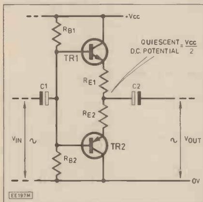
Fig. 4.10. Simplified complementary symmetrical output stage.
