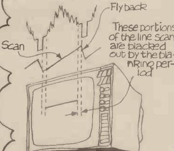
The **EFFECTIVE** period of the line duration. The blanking period is about twice as long as the sync pulse duration. This means, of course, that the actual picture visible on the screen is determined by the time interval separating the line blanking periods.
