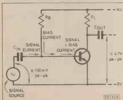
A base current swing of  $\pm 50\mu A$  (i.e.  $100\mu A$  pk-pk) will result in a collector-emitter voltage swing (developed across the load) of approximately 4.7V pk-pk.
