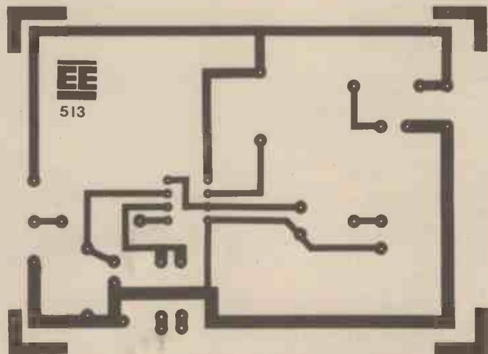
Fig. 5.7. Top, the component overlay for the frequency measurement/tachometer unit and, above, the p.c.b.—available from the EE PCB Service.
