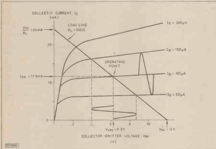
Fig. 4.6. Use of output characteristics and load line to predict the performance of a common emitter amplifier.
