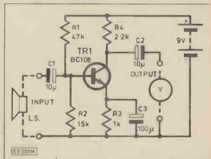
Fig. 4.14. Circuit used in Assignment 4.1.
