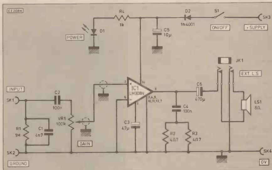
Fig. 4.3. Circuit diagram of the Audio Signal Tracer.
