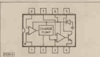
Fig. 5.1. Internal circuitry of the 2917 tachometer i.c.
