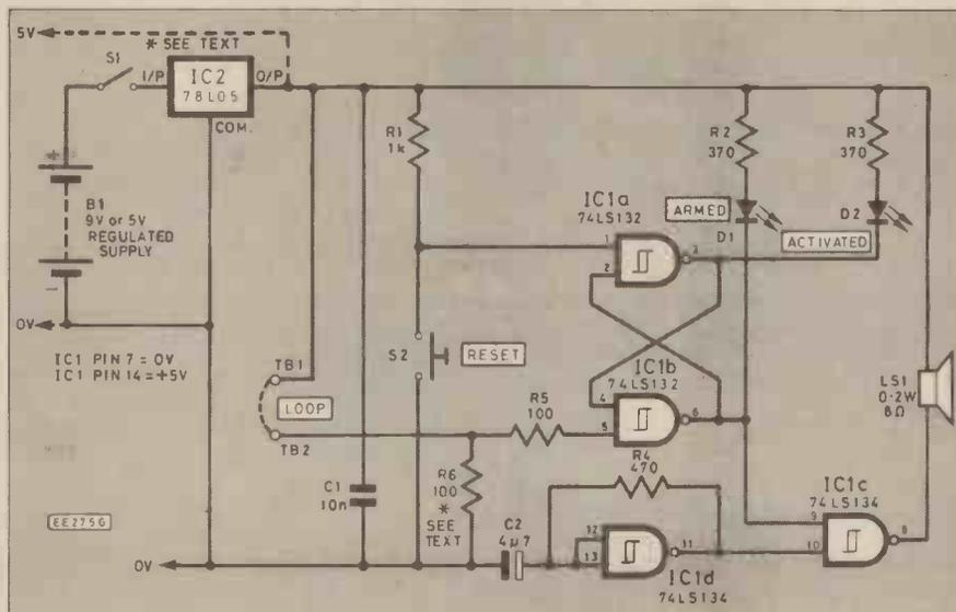
Fig. 8. Complete circuit diagram of the One-Chip Alarm.
