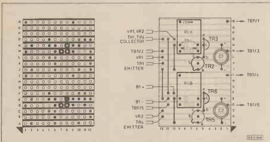
Fig. 4. Stripboard layout—soldering points, track breaks, and component overlay.
