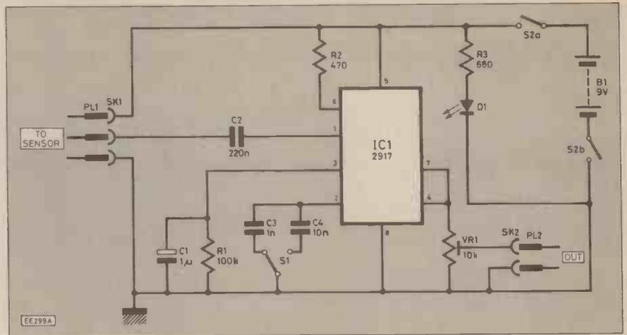
Fig. 5.6. Circuit diagram for the frequency measurement/tachometer unit.
