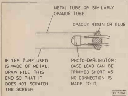
Fig. 3. Suggested method for mounting TR1 and TR4 in tubes.
