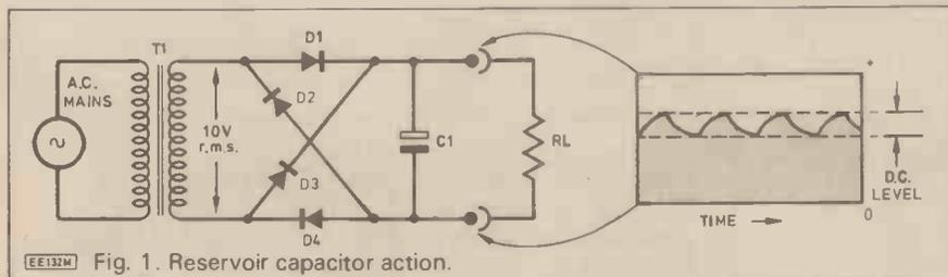
Fig. 1. Reservoir capacitor action.
