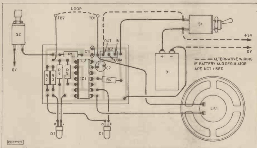
Fig. 9. P.c.b. design, component layout and wiring diagram of the One-Chip Alarm.
