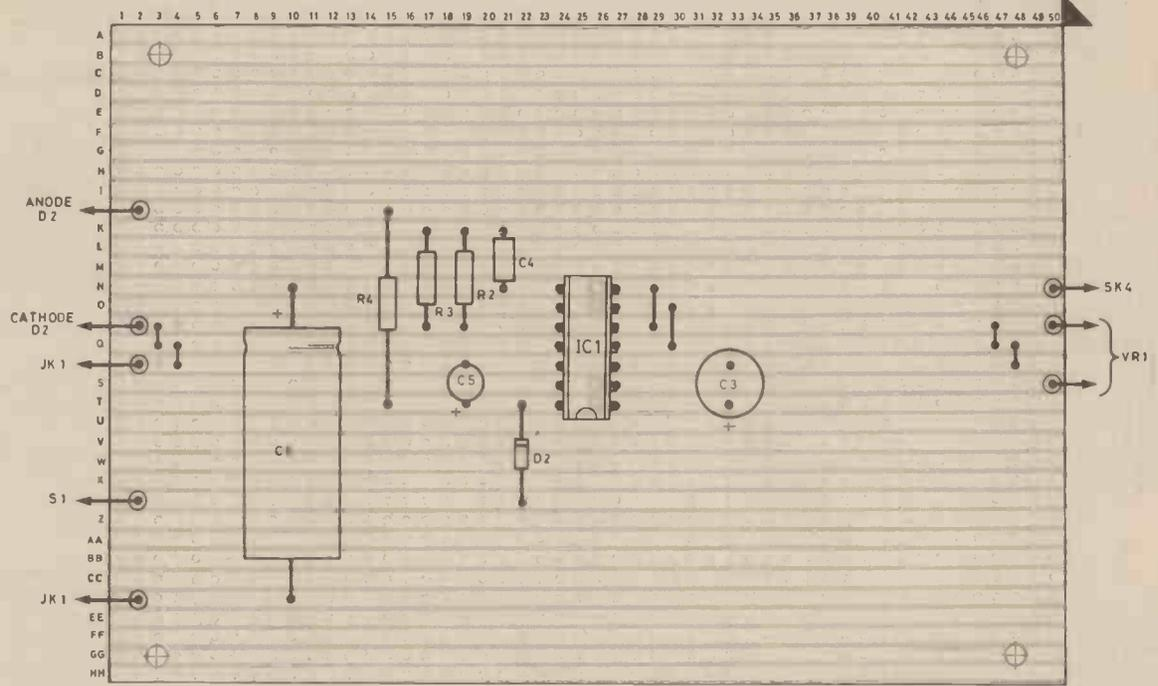
Fig. 4.4. Circuit board component layout of the Audio Signal Tracer.
