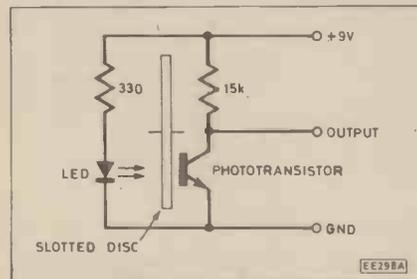
Fig. 5.5. Basic circuit for opto-switches.
