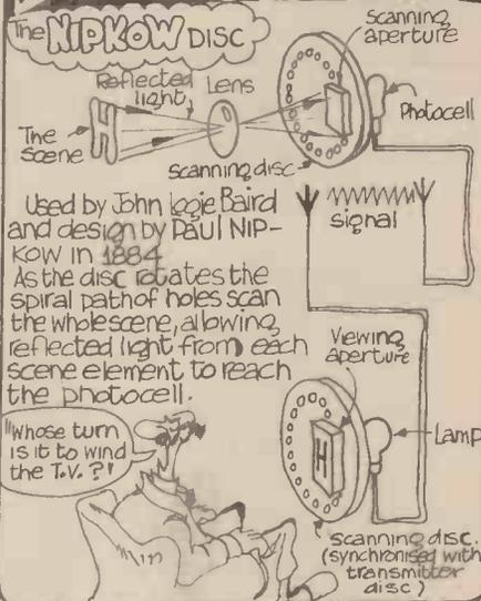
Used by John Logie Baird and design by Paul NIPKOW in 1884. As the disc rotates the spiral path of holes scan the whole scene, allowing reflected light from each scene element to reach the photocell.
