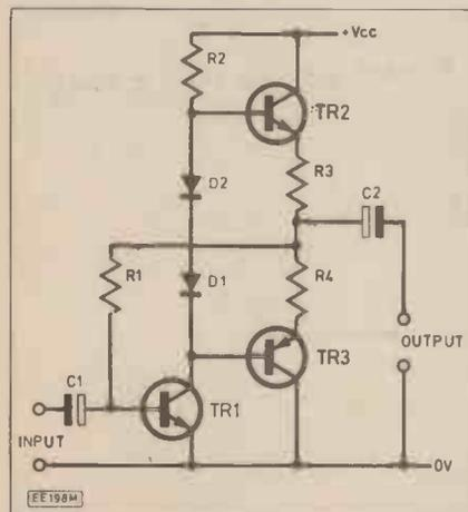
ward biased diodes, D1 and D2, provide a constant voltage drop (of approximately 1.2V) in order to bias the output pair, TR2 and TR3, to the threshold of conduction.
