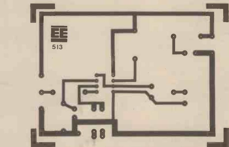
Fig. 5.7. Top, the component overlay for the frequency measurement/tachometer unit and, above, the p.c.b.—available from the EE PCB Service.
