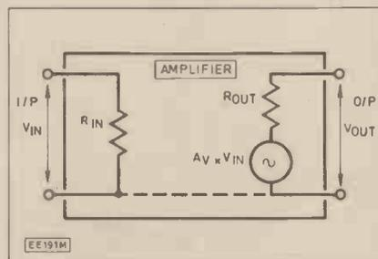
Fig. 4.4. Equivalent circuit of an amplifier.
