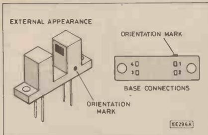
Fig. 5.3. Details of the slotted optical switch sensor.
