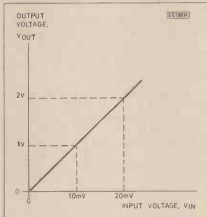
Fig. 4.1. Voltage transfer characteristic.
