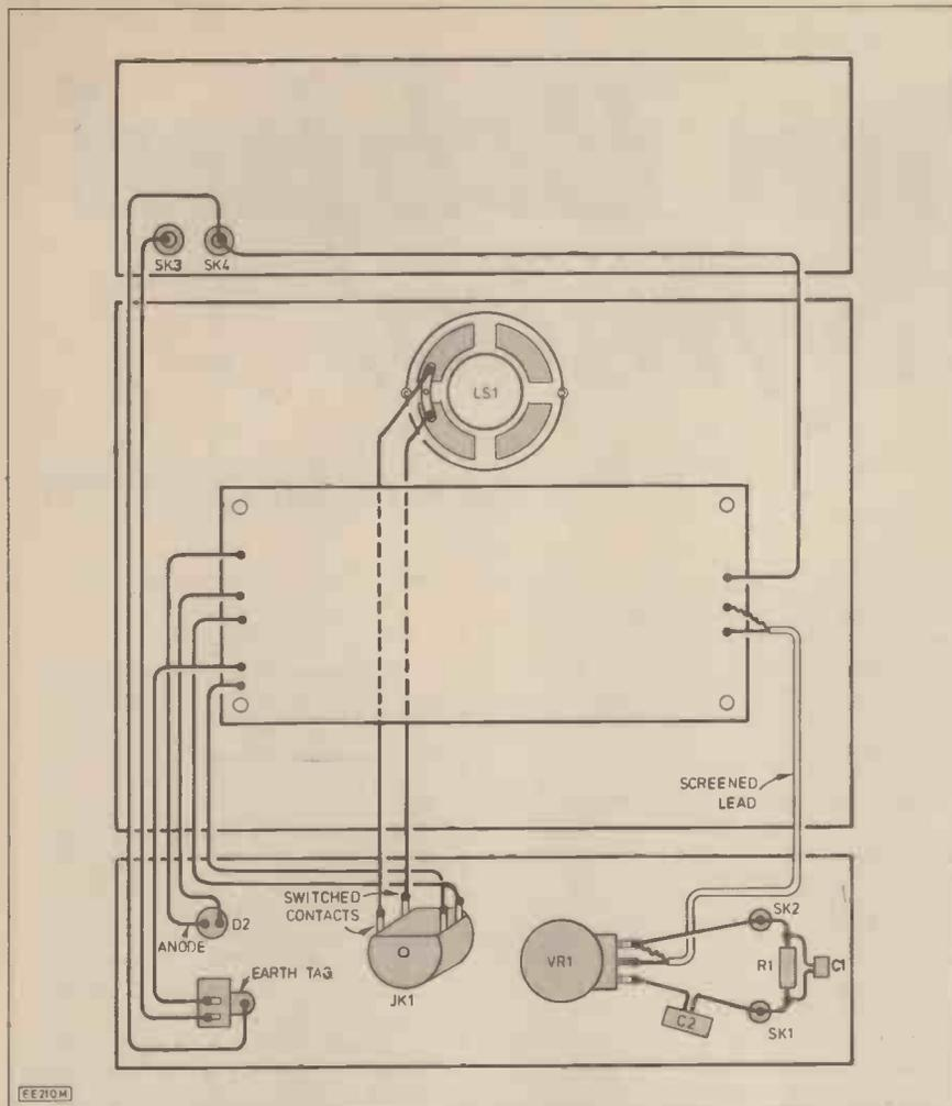
Fig. 4.5. Overall wiring diagram of the Audio Signal Tracer.
