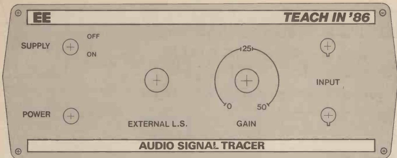
Fig. 4.2. Front panel design of the Audio Signal Tracer.
