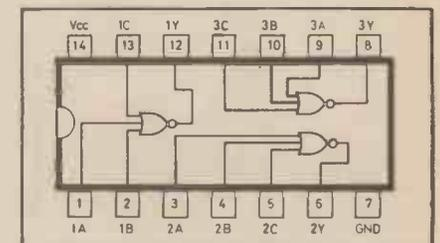
Fig. 7. Example of TTL (7427 Triple 3-input NOR).
