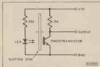
Fig. 5.5. Basic circuit for opto-switches.
