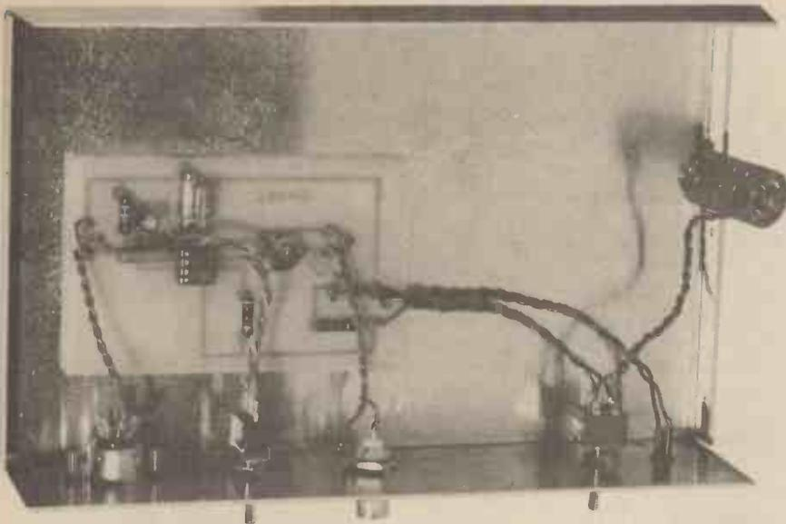
Internal details of the prototype frequency measurement unit: the +9V line was not taken to the DIN socket in the prototype, but is made available as a pad on the p.c.b. supplied from the *EE PCB Service*.
