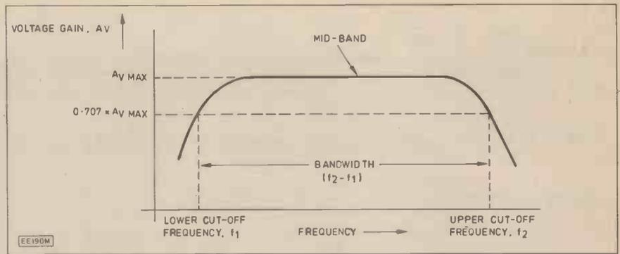
Fig. 4.3. Typical frequency response characteristic.
