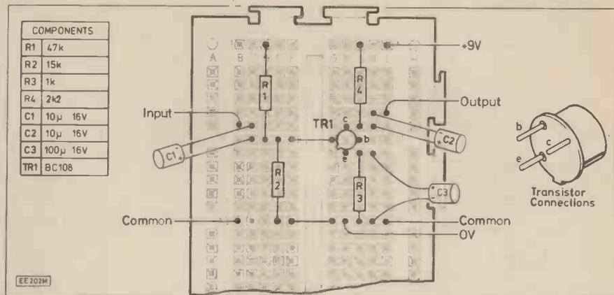
Fig. 4.15. Wiring diagram for the circuit of Fig. 4.14.
