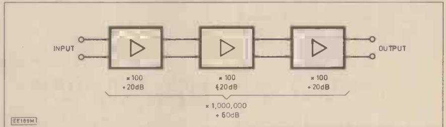
Fig. 4.2. Cascade arrangement of three amplifiers.
