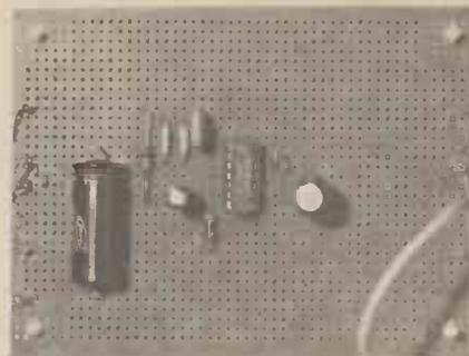
Photo 4. Veroboard layout of the Audio Signal Tracer.
