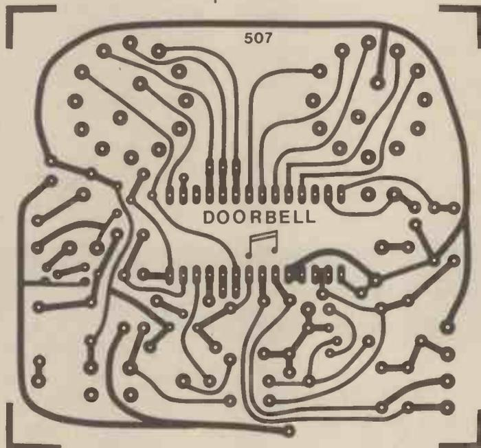
Fig. 2. Full size printed circuit master. This board is available from the *EE PCB Service*: code EE-507.
