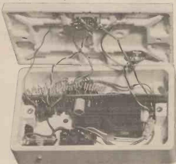
with a "tapping" between the 20th and 21st. This is not as laborious as it sounds! The full length of C2 leads should be used and sleeved to prevent short-circuits. When the circuit panel is in position, C2 may then be moved into a free space.
