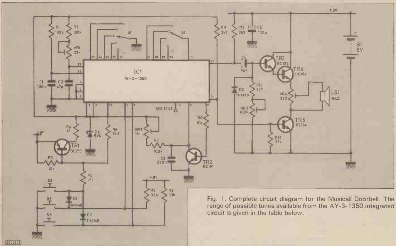
Fig. 1. Complete circuit diagram for the Musical Doorbell. The range of possible tunes available from the AY-3-1350 integrated circuit is given in the table below.
