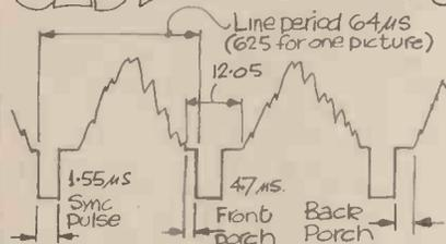
This system uses 625 lines to make-up a picture. Signal is shown above.
