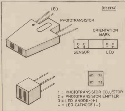
Fig. 5.4. The diffuse scan photo-reflective sensor: top, the large type is shown and, above, the miniature version.
