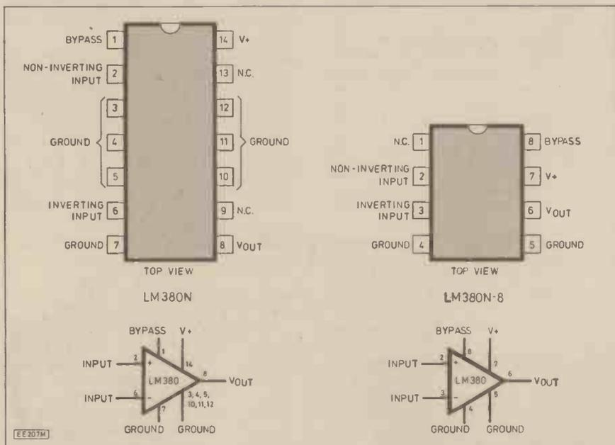
Fig. 4.1. LM380 pin connections.
