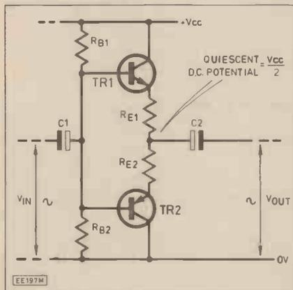
Fig. 4.10. Simplified complementary symmetrical output stage.
