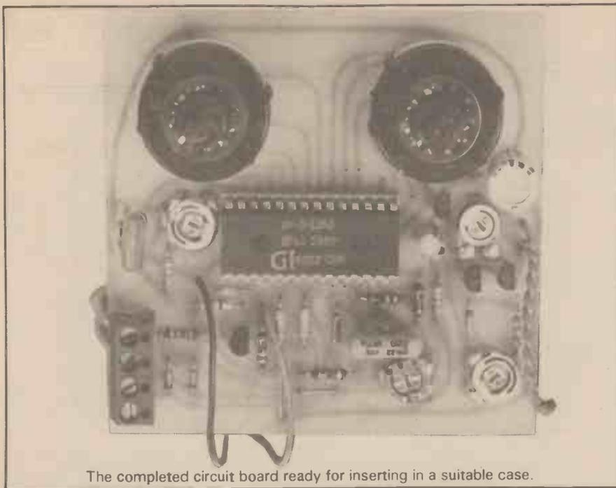
The completed circuit board ready for inserting in a suitable case.
