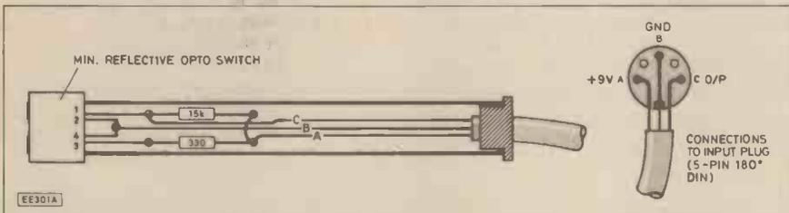
Fig. 5.8. The photo-reflective probe assembly—suggested method of construction.
