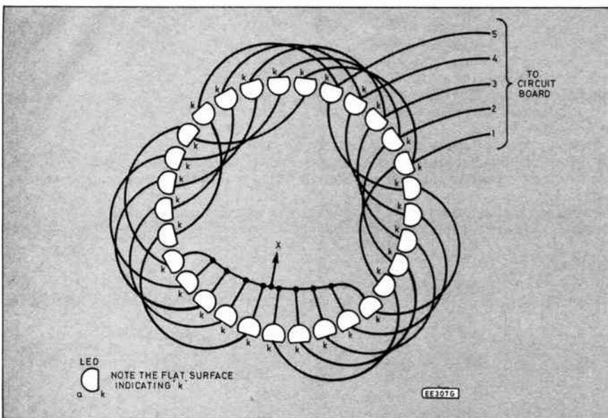
Fig. 4. Wiring to the display i.e.d.s D6 to D35. The polarity of the i.e.d.s can be ascertained by referring to the pinning diagram.
