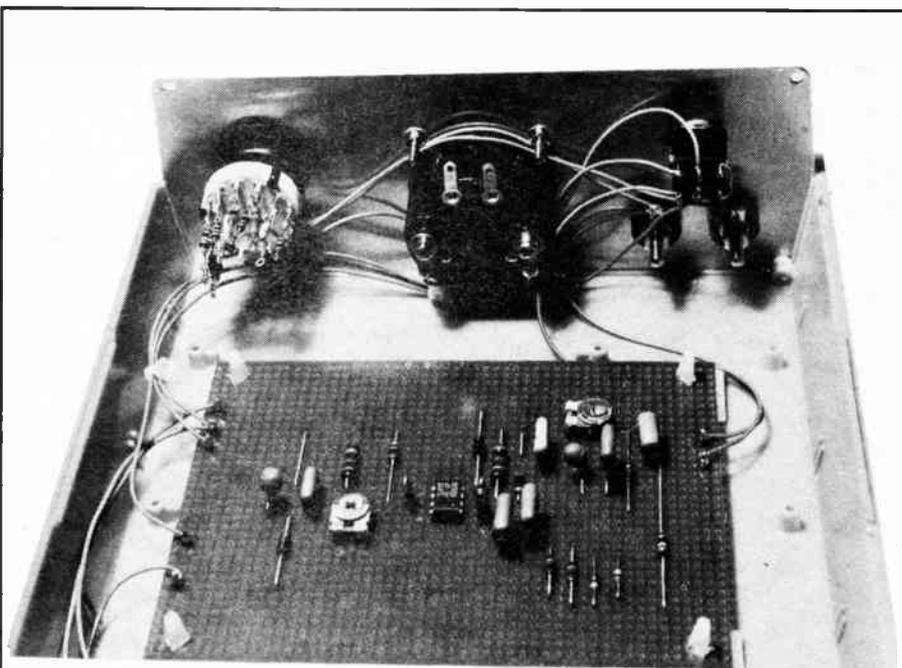
Wiring to the front panel range switch, meter, mode switch, input terminals and the solder pins on the circuit board.
