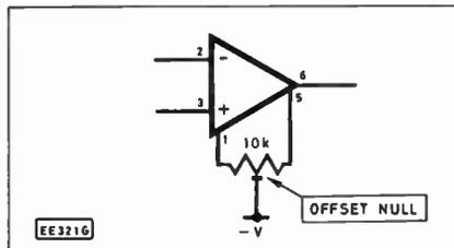
Fig. 7.13. Offset null provision for the 741.
