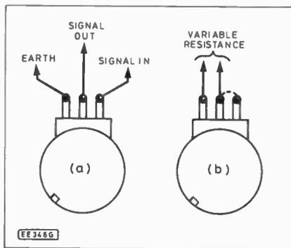
Fig. 3. Using a potentiometer as a volume control (a) and a variable resistance (b).
