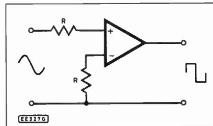
Fig. 7.19. Square wave converter.
