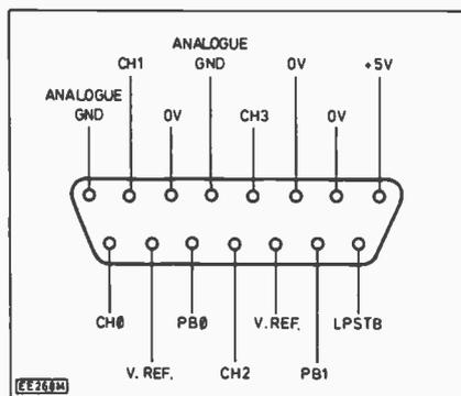
Fig. 2. Joystick connection to the analogue port.
