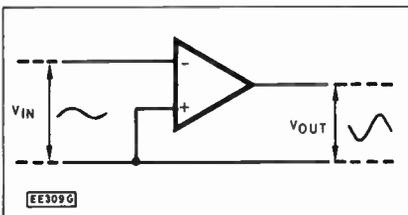
Fig. 7.2(a). Basic configuration for an inverting amplifier.
