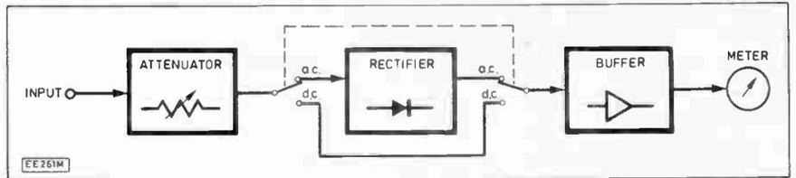
Fig. 2. Block diagram for the FET Voltmeter.
