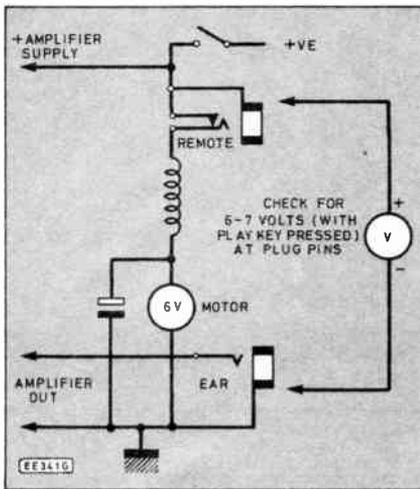
Fig. 2. Remote wiring connections on most recorders.
