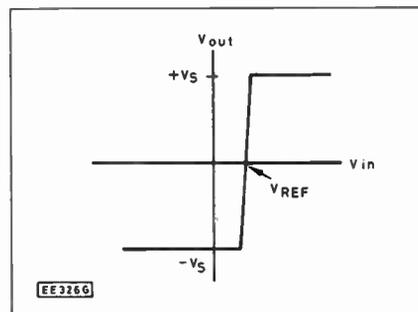
Fig. 7.18. Transfer characteristic of the arrangement shown in Fig. 7.17.
