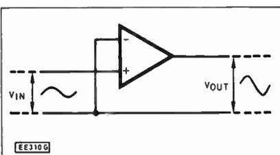
Fig. 7.2(b). Basic configuration for a non-inverting amplifier.
