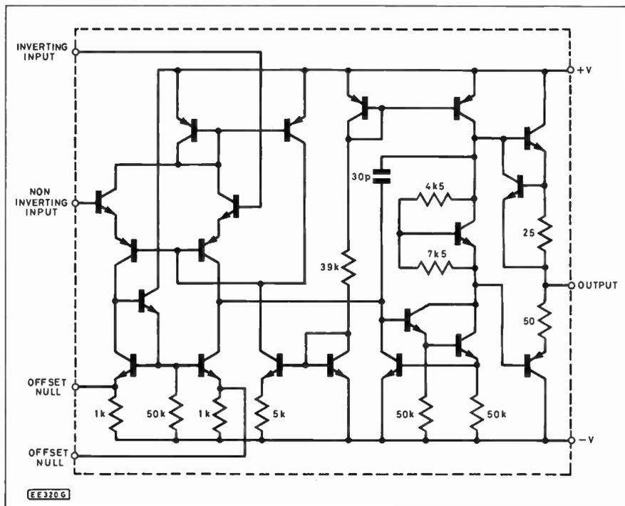
Fig. 7.12. Internal circuit of a 741.
