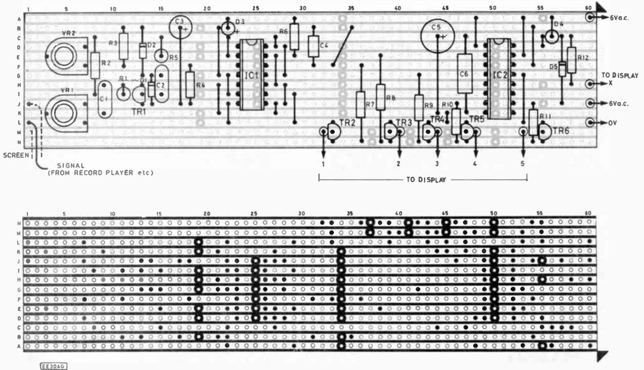
Fig. 3. Component layout, underside showing breaks (44 off) in the copper strips and interwiring details. Use screened cable for the input signal lead.
