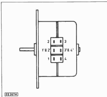
Fig. 3. Stepper motor connection details.
