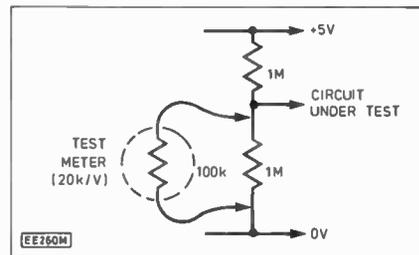
Fig. 1. Voltmeter impedance effects.
