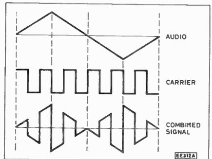
Fig. 4. The effect of combining the audio and carrier waves.
