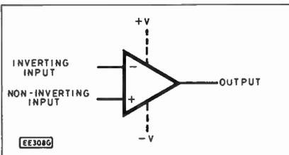
Fig. 7.1. Symbol used for an operational amplifier.
