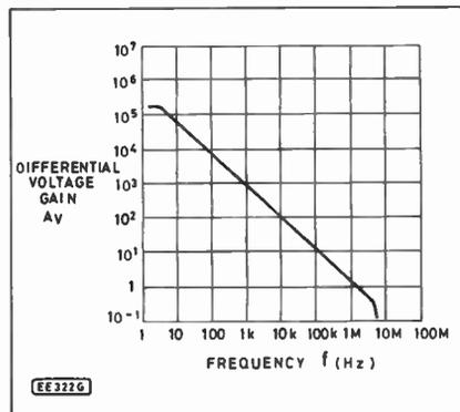
Fig. 7.14. Typical frequency response of a 741.
