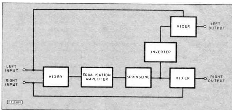
Fig. 1. Block diagram of the Stereo Reverb.
