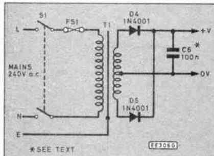
Fig. 2. Suggested mains power supply circuit. Capacitor C5 forms part of the power supply but is shown on the main circuit Fig. 1.
