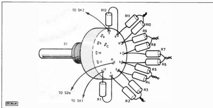
Fig. 7. Range selector switch S1 detailed assembly. The "free ends" of the resistors should be twisted together in pairs and soldered.
