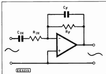
Fig. 7.15. Bandwidth limited amplifier.
