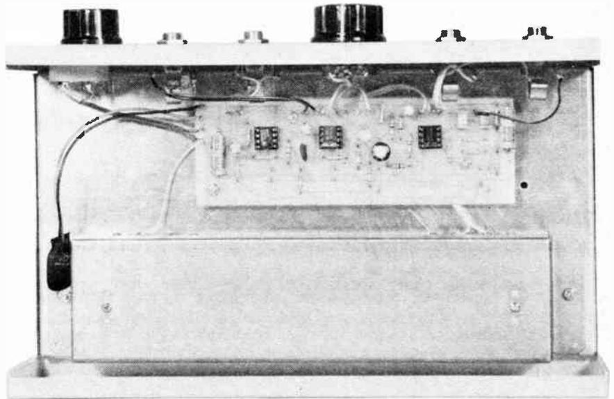
Completed Stereo Reverb showing positioning of printed circuit board, springline and wiring to front panel components.
