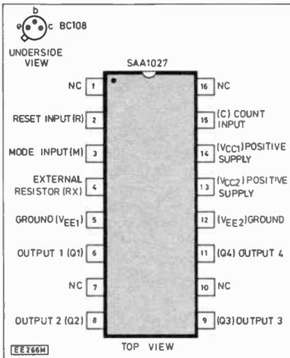
Fig. 2. Pinning details for the BC108 and SAA1027.
