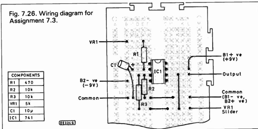
Fig. 7.26. Wiring diagram for Assignment 7.3.
