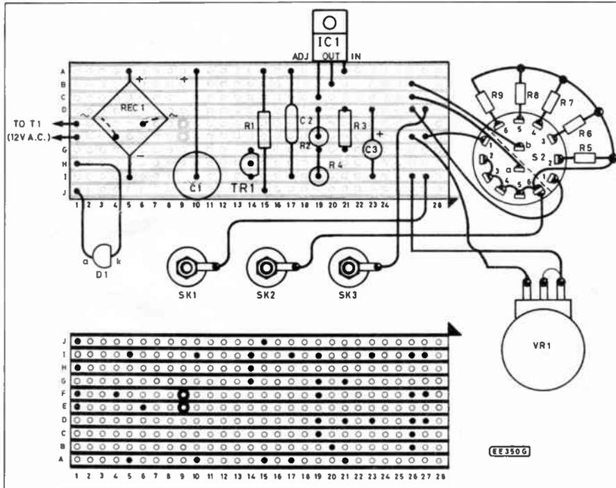
Fig. 4. Component layout, details of breaks in copper strips (2 off) and interwiring to the front panel mounted components. The wires from S2 to the stripboard should be kept as short as possible and reasonably thick.
