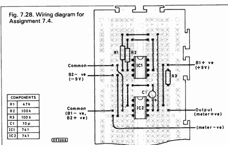
Fig. 7.28. Wiring diagram for Assignment 7.4.
