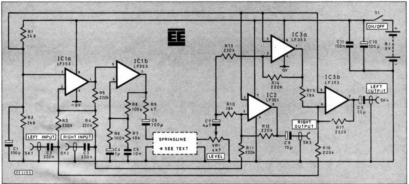
Fig. 2. Full circuit diagram of the Stereo Springline Reverberation Unit.
