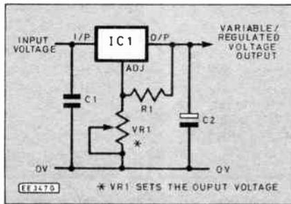
Fig. 1. Basic regulated voltage circuit.
