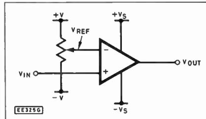
Fig. 7.17. An operational comparator.
