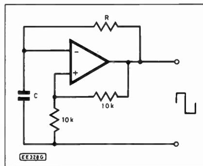
Fig. 7.20. Simple square wave oscillator.
