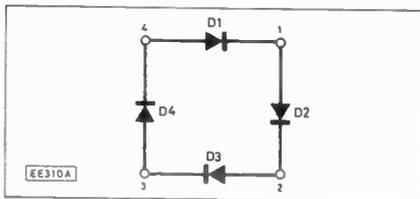
Fig. 2. The "ring" arrangement of the diodes in Fig. 1.
