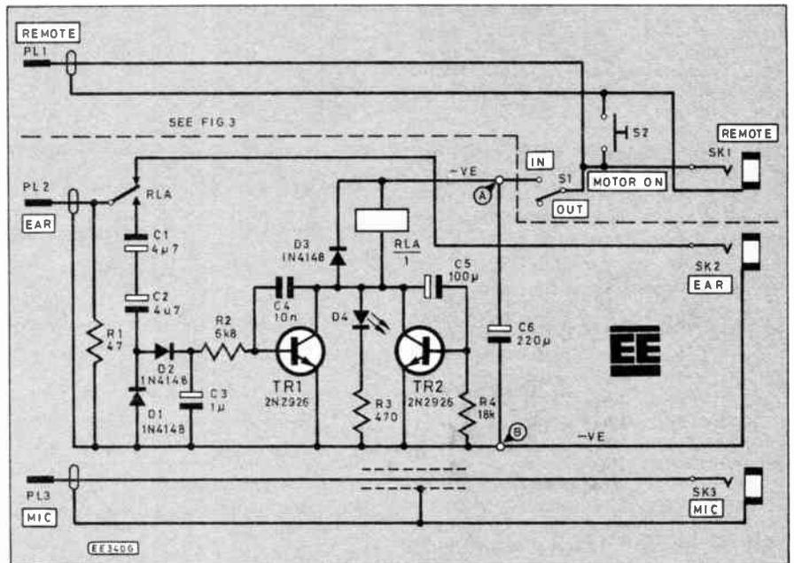
Fig. 1. Complete circuit diagram of the Freeloder when powered by the cassette recorder.
