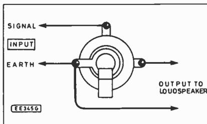
Fig. 2. The 3.5mm jack sockets normally have a break contact which can be used in this fashion. In many applications the switched output is not required, and the third tag is left unused.
