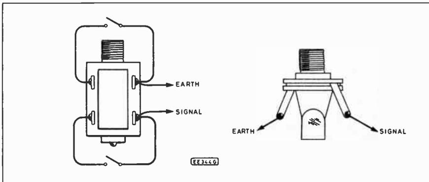
Fig. 1. These jack sockets differ in that one has d.p.s.t. contacts while the other has none. Both are suitable for most applications.
