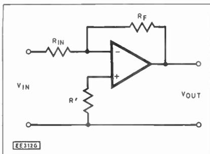
Fig. 7.4. A practical inverting amplifier.
