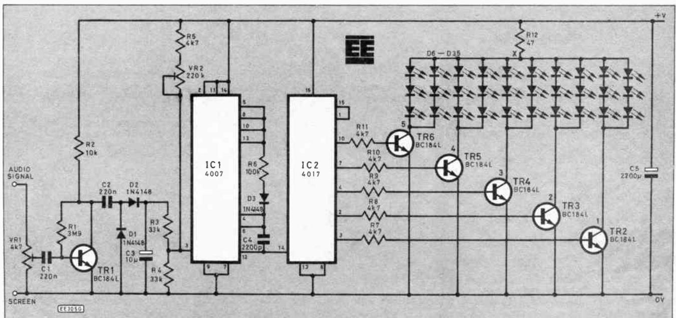
Each transistor is connected to two of these groups, wired in parallel with each other. Thus with the value of R12 shown, a total of about 40mA is used by the six i.e.d.s lit at any one time.
