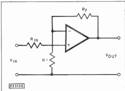
Fig. 7.5. A practical non-inverting amplifier.
