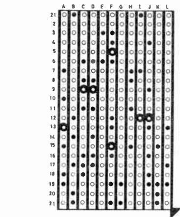
Fig. 4. Veroboard layout and wiring for the Freeloader. The board is mounted by SK1 and SK2.
