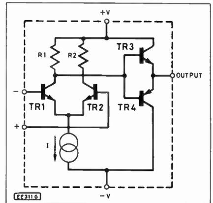
Fig. 7.3. Simplified internal circuitry of an operational amplifier.
