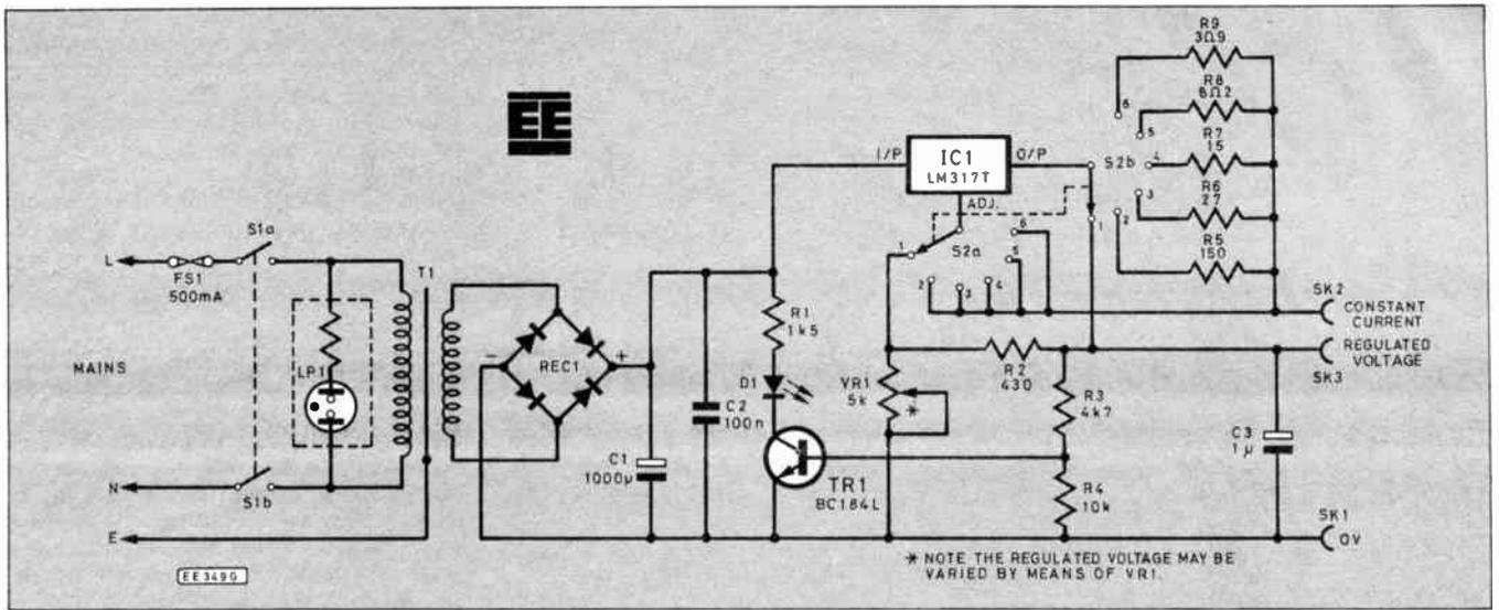
Fig. 3. Complete circuit diagram for the Versatile Power Supply Unit.
