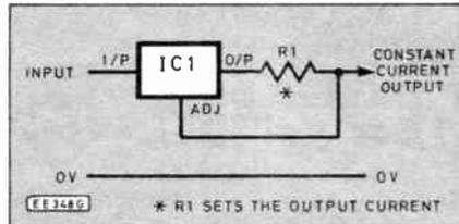
Fig. 2. Constant current regulation is determined by resistor R1.
