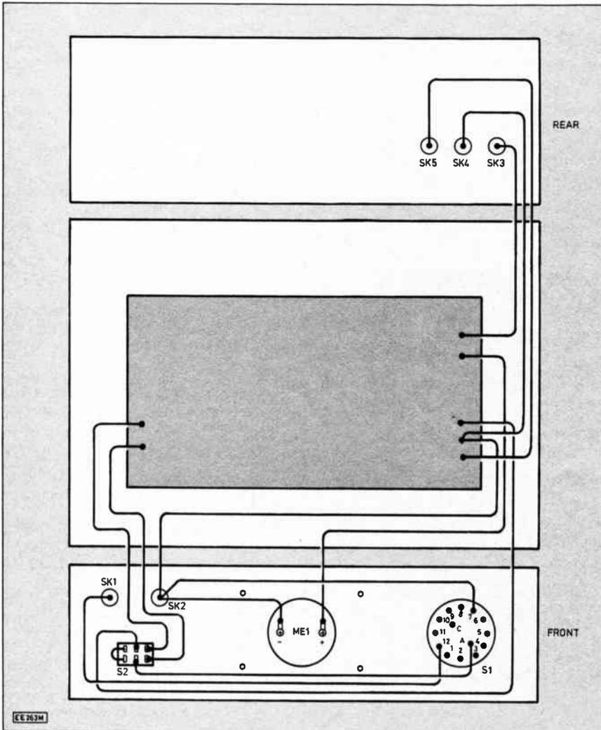
Fig. 6. Assembly and interwiring details.
