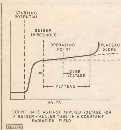
Fig. 4. Graph showing count rate against applied voltage.
