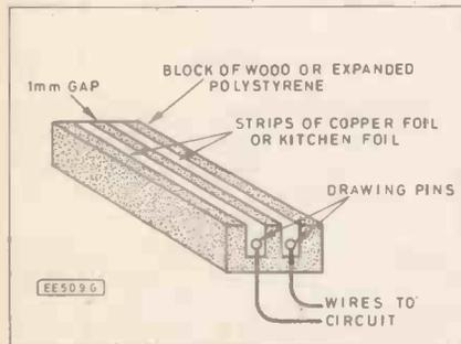
Fig. 2.6. Design for a rain detector probe.
