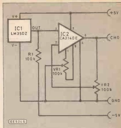
Fig. 6. Circuit diagram for improved accuracy at low temperature readings.
