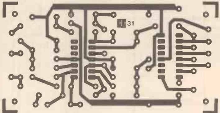
Fig. 3 Layout and wiring of the p.c.b.
