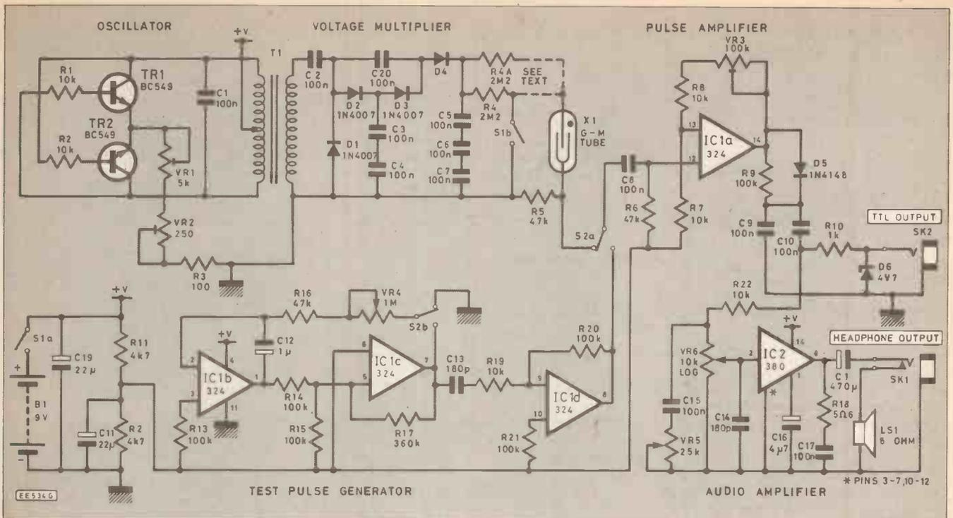
Fig. 5. Circuit diagram of the EE Geiger Counter.
