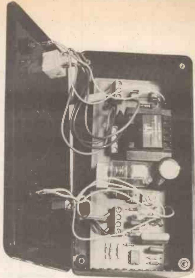
Front panel folded back to reveal the mounting of the printed circuit board and wiring to components on the rear of the front panel.
