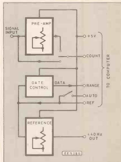
Fig. 1 Block diagram of the Micro Mini Tuner.
