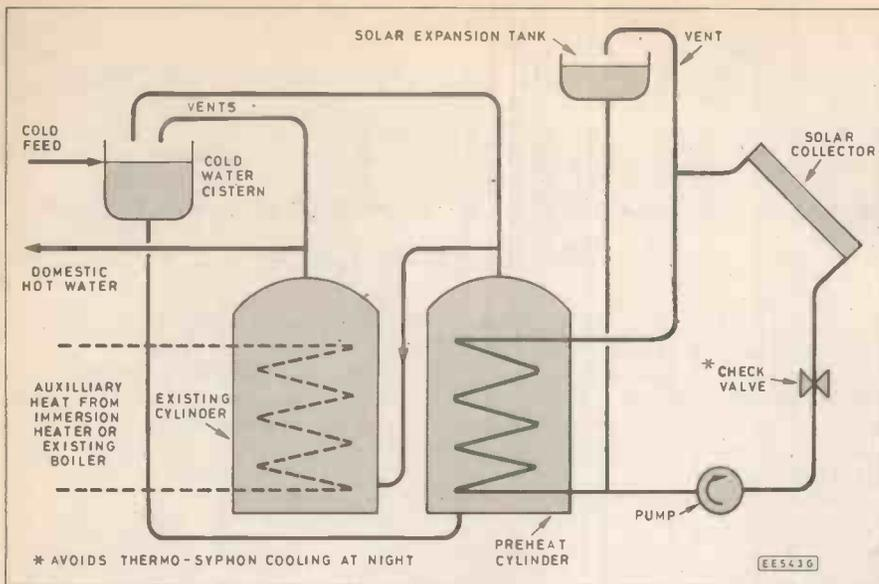
Fig. 5. Typical arrangement for a solar water heating system.
