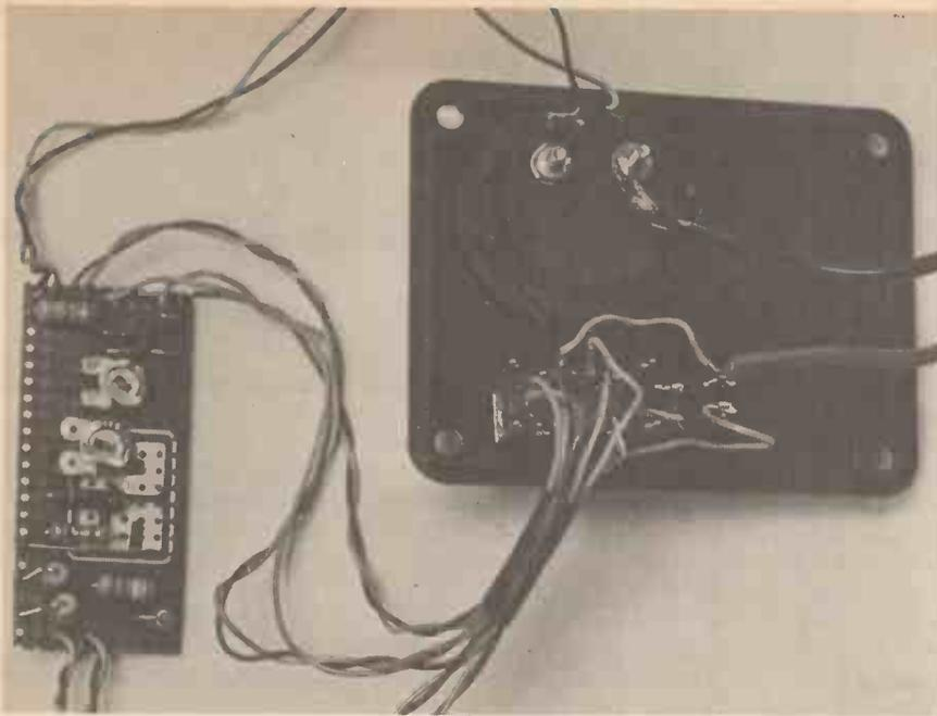
Completed Battery Tester showing interwiring to the stripboard, meter ME1 and the slide switch S1.
