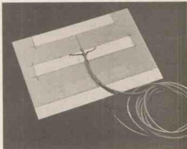
The completed aerial before being "sandwiched" with a piece of card.
