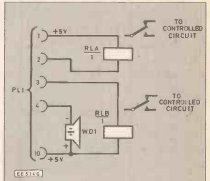
Fig. 4. Using the output interface to control a programmable darkroom timer.
