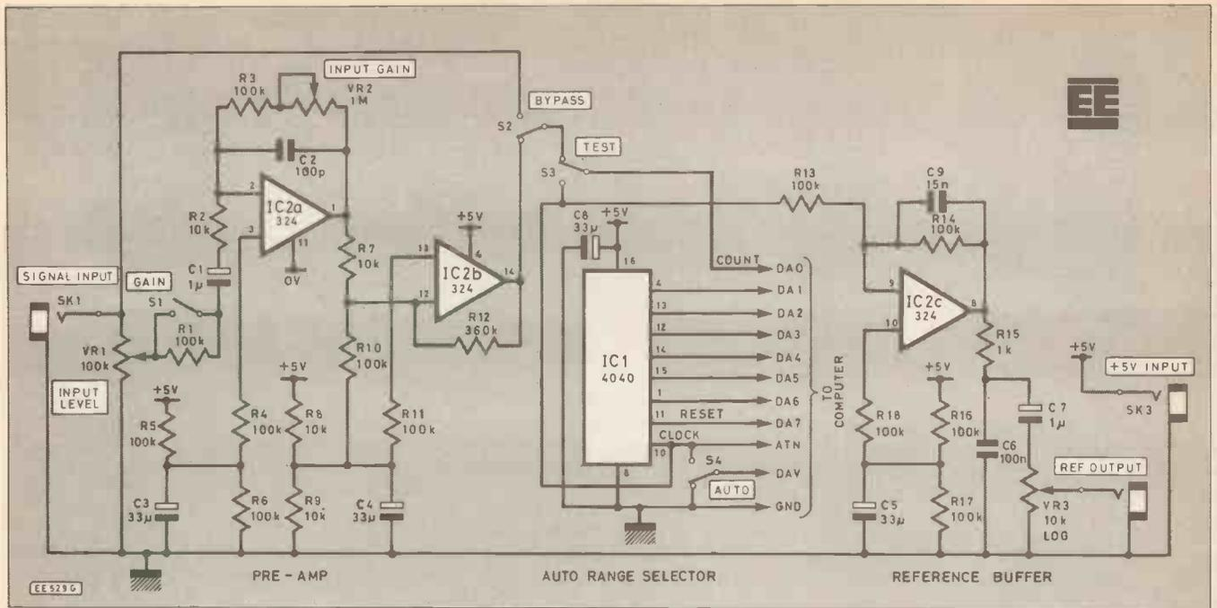
Fig. 2 Complete circuit of the Micro Mini Tuner.
