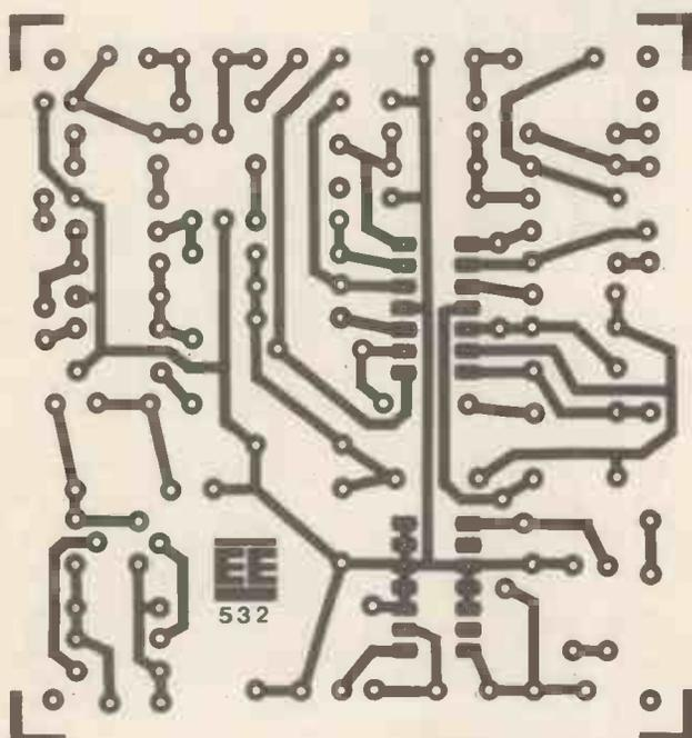
frequency range is determined by C12, and can be varied by VR4. The squarewave output at IC1c is coupled to C13. Since C13 has a low value it will only pass the output at the edges of the squarewave, and so a short duration pulse is generated. This is amplified to a respectable level by IC1d. With the G-M tube switched out by S2a, S2b completes the oscillator feedback circuit allowing it to generate.
