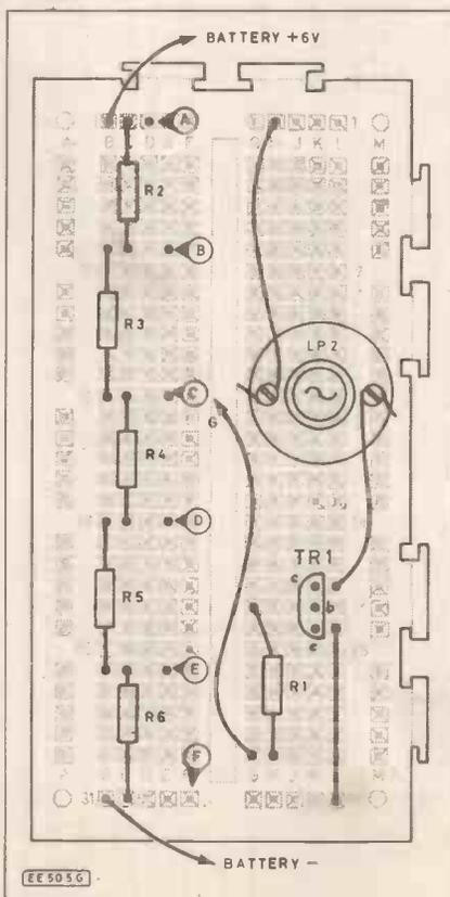
Fig. 2.2 (above). Circuit for demonstrating transistor action (Investigation 1) and working layout.
