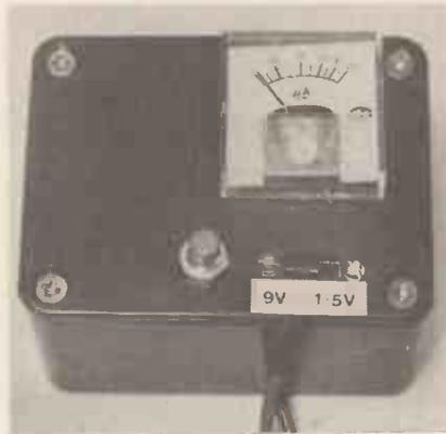
preserving readings below 1V approximately since any such cell would be "dead". Similarly, with 9V batteries, the section of scale below 6V is not needed. This maximises the useful part of the scale and leads to more accurate readings. A slide switch selects a basic load according to whether a 1.5V or a 9V battery is being tested and a push-button switch increases the load by a factor of five for larger types of battery.
