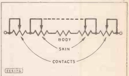
Fig. 3. Adding variable resistance to model effects of "contact resistance".
