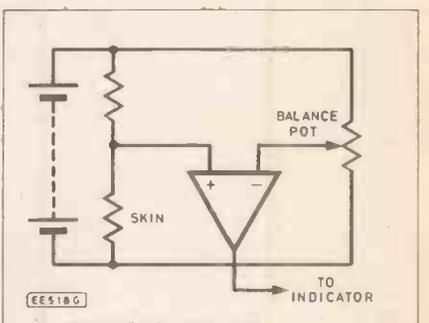
Fig. 4. Employing an op-amp in a bridge circuit to improve sensitivity.
