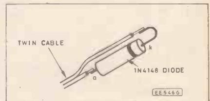
Fig. 4. Sensor construction.
