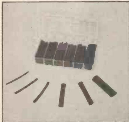
With mains equipment, prior to heat shrinking, it is good practice to push the sleeving over the wire and plastic covering before soldering the lead in place. It is then possible to slide the sleeving over the exposed solder joint and then slide it back during testing. Once the testing has been completed satisfactorily, the tubing can be shrunk over the join or terminal.
