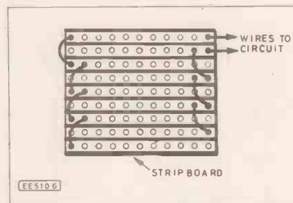
Fig. 2.7. Alternative stripboard design for a rain detector sensor.
