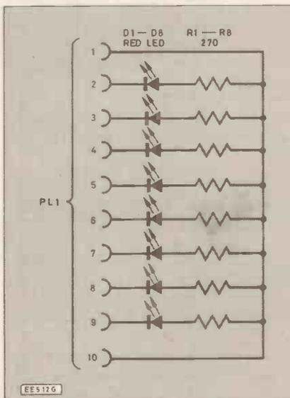
Fig. 2. Circuit for testing the Two-chip Output Interface.
