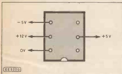
Fig. 4. Details of the power port connector.
