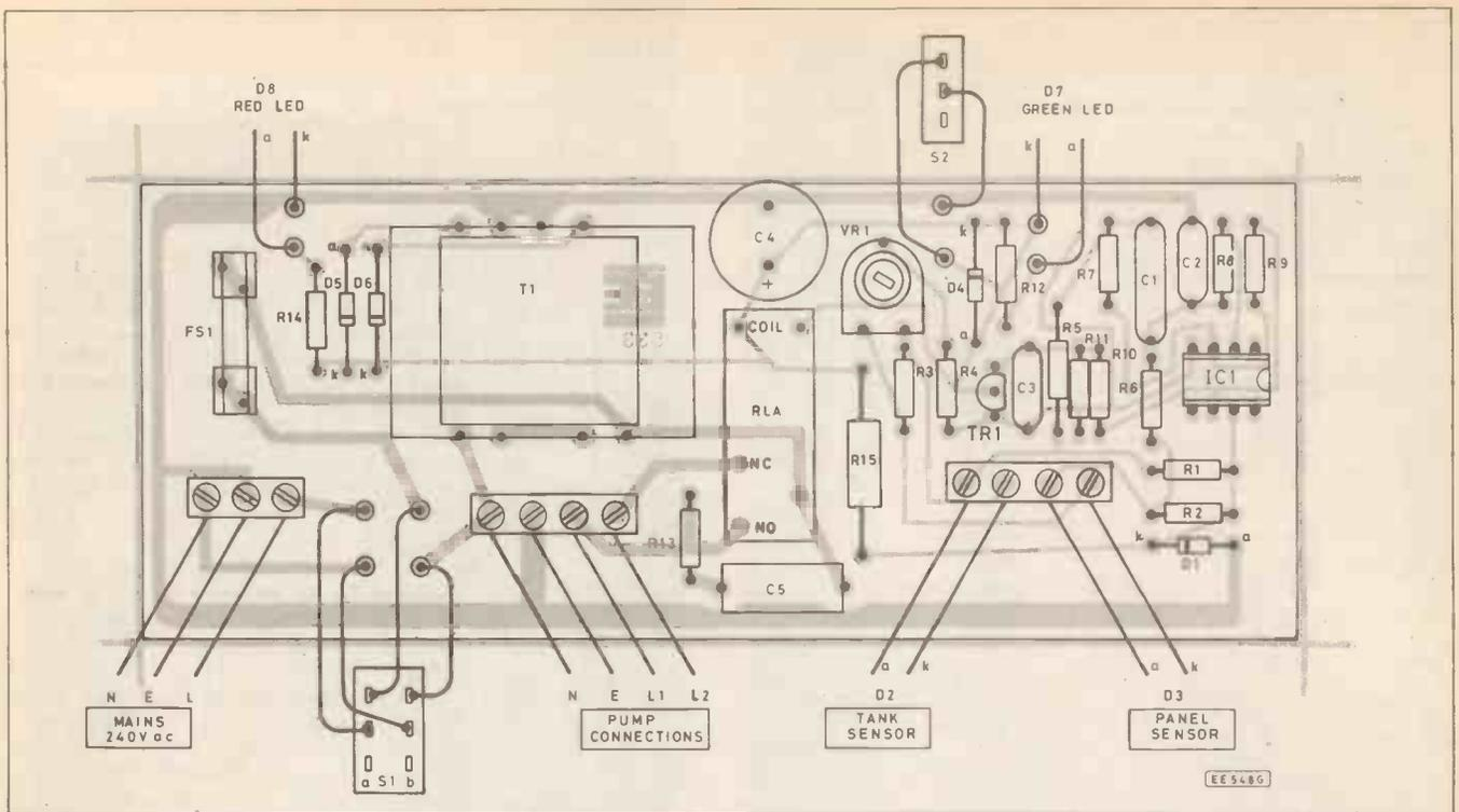
Fig. 3. Component layout, interwiring details and full size printed circuit board master pattern for the Solar Heating Controller.
