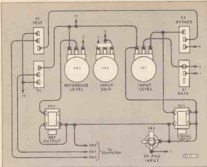
Fig. 4 Interwiring of the controls and connectors.
