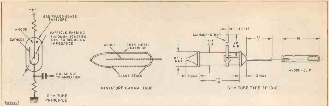
Fig. 3. The Geiger Muller tube principle and construction.
