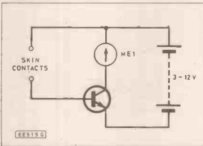
Fig. 1. A simple transistor amplifier circuit.
