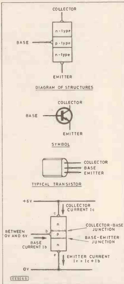
Fig. 2.1. The construction, circuit symbol and operation of junction transistor.
