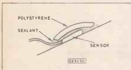
Fig. 6. Method of mounting the sensors.
