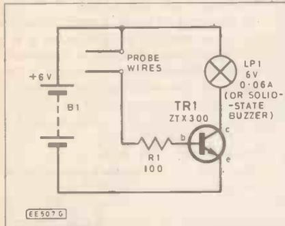
Fig. 2.4. Water detecting circuit (the breadboard layout is similar to that for Fig. 2.2).
