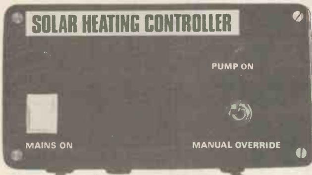
Check the operation of the controller by holding a soldering iron against the panel sensor. The relay should turn on after a few seconds. Leave the panel sensor to cool down for a few minutes and the relay should turn off. Disconnect the unit from the mains supply ready for installation.
