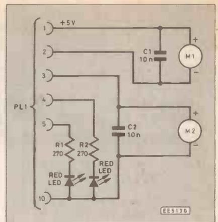
Fig. 3. Motor control for a buggy using the interface.
