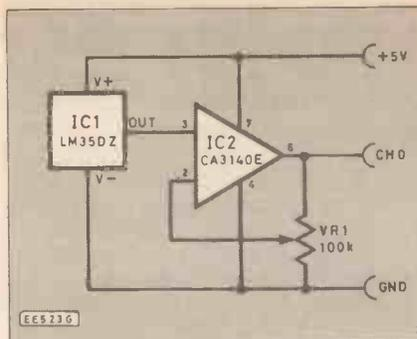
Fig. 5. Simple temperature to voltage converter circuit.
