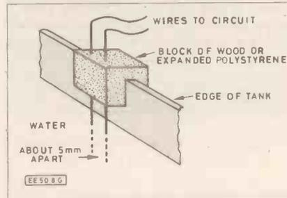
Fig. 2.5. Probe to detect water level in tank. Wires slide up or down to set operating level.
