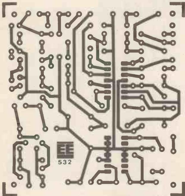
Fig. 6. P.c.b. layout and wiring. Note that C18 is carefully laid flat across the board towards C12.
