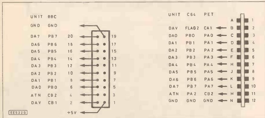
Fig. 5 Connection details for the PET, C64 and BBC computers.
