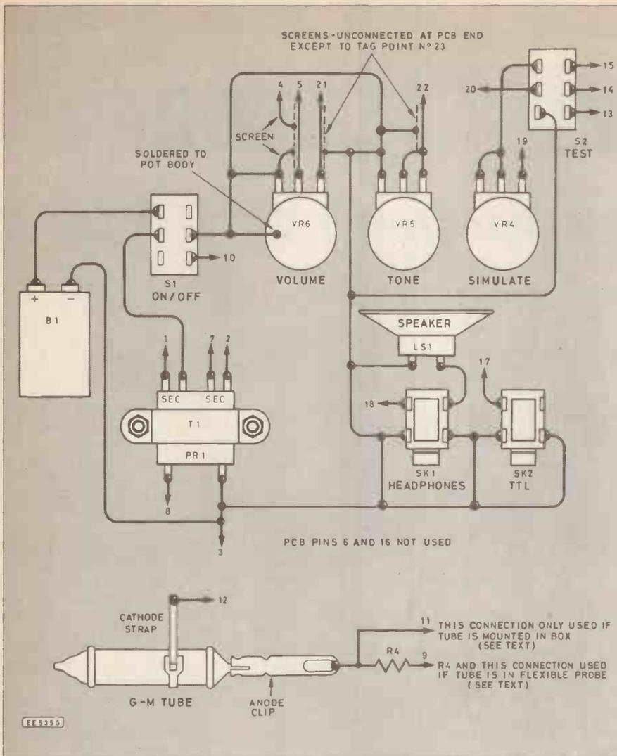
Fig. 7. Component interwiring and connections to the G-M tube.
