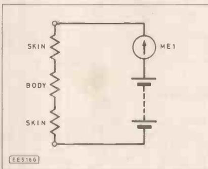
Fig. 2. Analogy of "skin resistance" using Fig. 1.
