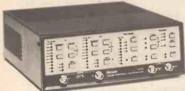
THE new Maplin ID-4850 Digital Memory Oscilloscope is designed to increase the power and versatility of both oscilloscopes and personal computers. The interface adds testing capabilities to any IBM PC or PC-compatible computer, enhancing the computer function as a workstation.
