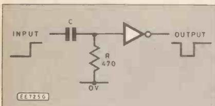
Fig. 3.1. Simple negative-going monostable pulse generator.
