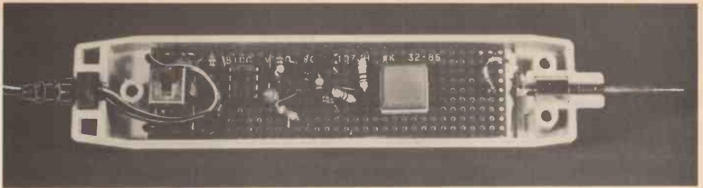
the standard size stripboard used in this series (24 strips of 37 holes); alternatively the remaining unused board from last month's project may be employed.
