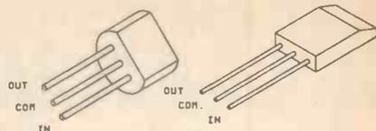
Fig. 4. Pinout details for low power voltage regulators such as the  $\mu$ A78L05.
