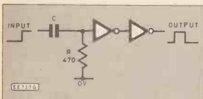
Fig. 3.3. Simple positive-going monostable pulse generator.
