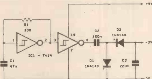
Fig. 4. Generating a negative supply for the tail resistor from the +5 supply.
