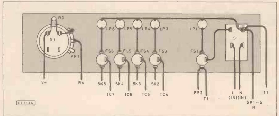
Fig. 3. Wiring of components mounted on the front panel.
