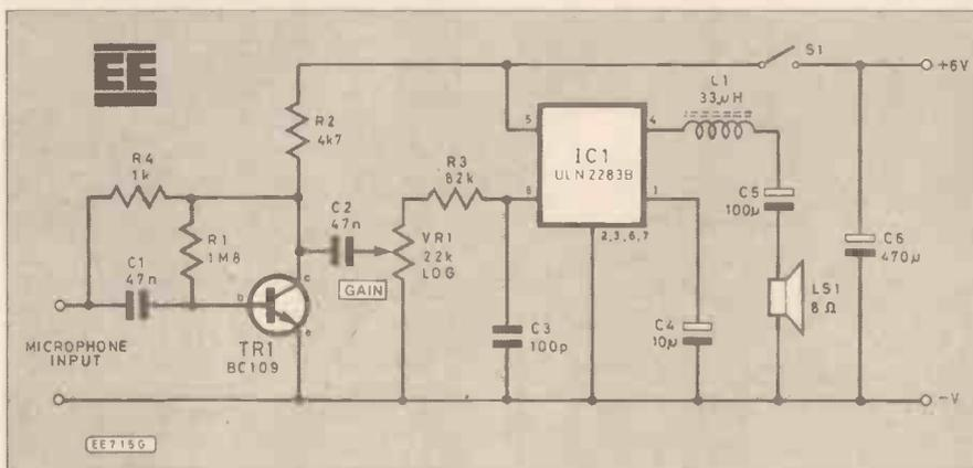
The power supply can be conveniently located anywhere along the route of the connecting cable, where it can be placed out of sight. A 6V lantern battery should be satisfactory for occasional use. In the prototype system the total quiescent current at 6V was about 16mA.
