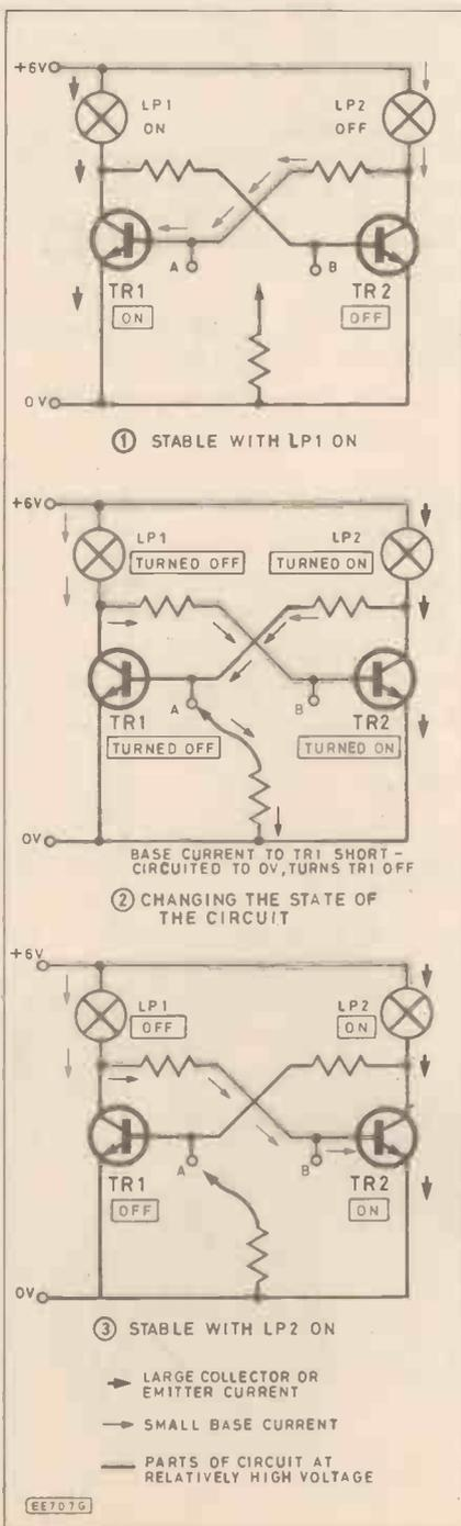
is enough to start a base current flowing through TR1. This turns TR1 "on". Immediately the potential of the collector of TR1 begins to fall. This falling potential pulls down the potential of both plates of C1 and the base of TR2. Base current to TR2 is cut off, and TR2 is turned "off". The circuit has now reached state B.
