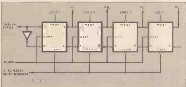
Fig. 3.14. Four stage shift register using JK bistables.
