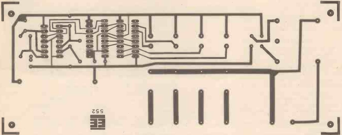
outputs selected to be live by the circuit. It is therefore important to ensure that the cable carrying the "live" power connection to the p.c.b. is capable of withstanding this load. The outputs from the relays to the fuseholders should be wired in flexible cable capable of carrying a current of 2A. All the remaining connections are required to carry relatively small currents and can therefore be made with relatively small flexible cables.
