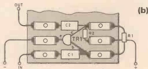
Fig. 6. Illustration of how a simple transistor amplifier stage (a) can be assembled using only three pairs of tags.
