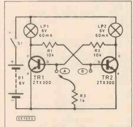
Fig. 7.1. Experimental circuit diagram for a bistable multivibrator.
