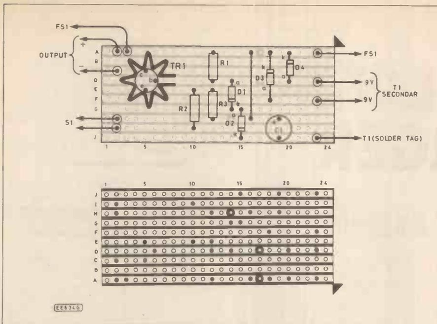
Fig. 2. Component layout and details of breaks to be made in the underside copper strips of the stripboard for the mains hand lamp charging system.
