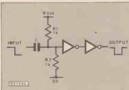
Fig. 3.5. Falling edge triggered negative-going pulse generator.
