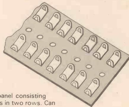
Fig. 5. Tag panel consisting of double tags in two rows. Can be a useful alternative to circuit boards for simple assemblies.
