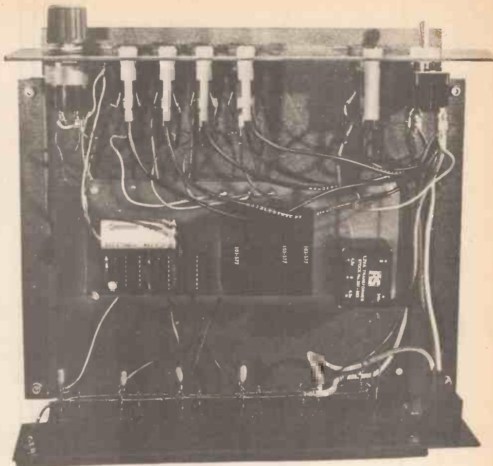
**SENT ON THE UNDERSIDE OF THE PRINTED CIRCUIT BOARD.** Great care should therefore be taken when investigating the underside of the p.c.b. whilst the unit is connected to mains power.
