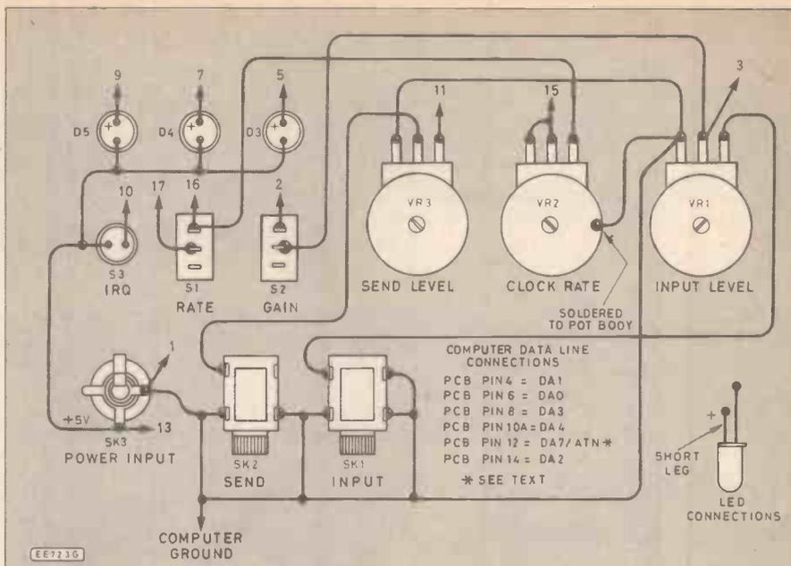
Fig. 4. Wiring of panel mounted components.
