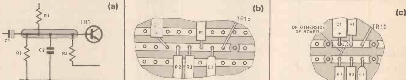
Fig. 2. When several connections have to be made to a single point as in circuit (a), the result on Vero can be elongated as in (b). A more compact and convenient group can be made if two adjacent strips are used. A link can be made by soldering a wire from one component across the two strips (c).
