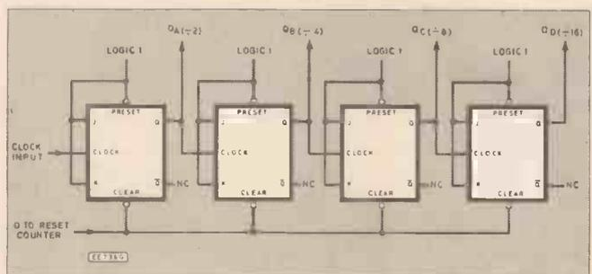
Fig. 3.12. Four stage binary counter using JK bistables.
