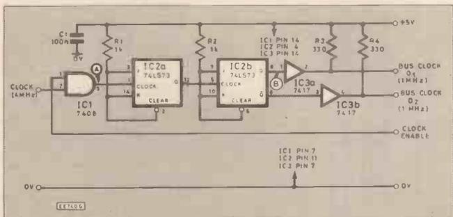
Fig. 3.16 (above). Dual phase microprocessor clock divider. Logic Pulser applied to A, Logic Probe (last month) applied to B.
