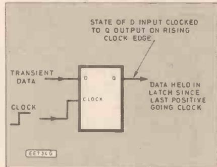
Fig. 3.10. D-type bistable as a data latch.
