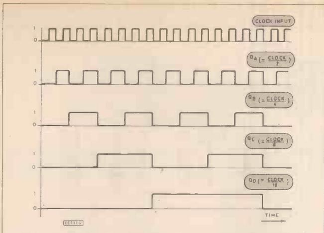
Fig. 3.13. Timing diagram for the circuit of Fig. 3.12.
