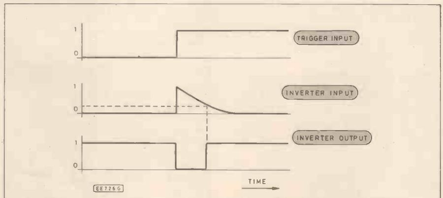
Fig. 3.2. Waveforms for the circuit of Fig. 3.1.
