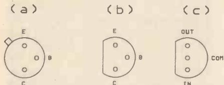
Fig. 2. Typical TO-18 (a) and TO-92 (b) transistor underside views. (c) is for a low power voltage regulator, and is a top view. Compare these with the 3-D views of Figs. 3 and 4.
