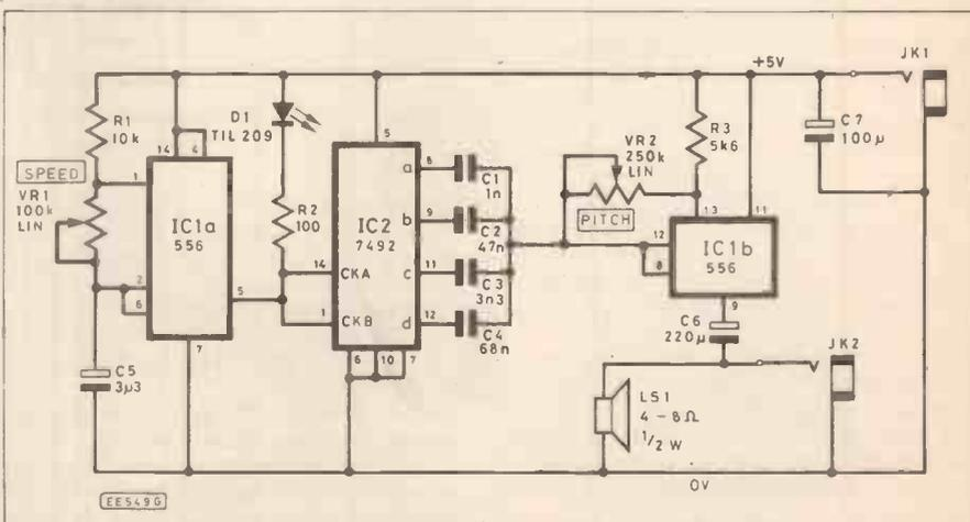
capacitors C1 to C4, with respect of the binary counting. This develops the generation of different notes, the "Pitch" potentiometer VR2 is used to change the frequency of these notes.
