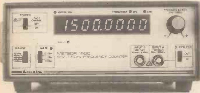
**T**HE latest addition to the Black Star range of Frequency Counters is the Meteor 1500, utilising the latest monolithic microwave integrated circuit technology to measure frequency up to 1.5GHz.
