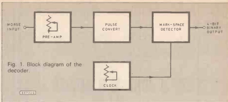
Fig. 1. Block diagram of the decoder.
