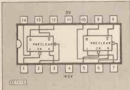
Fig. 3.17. Internal arrangement of the 7473 JK bistable.
