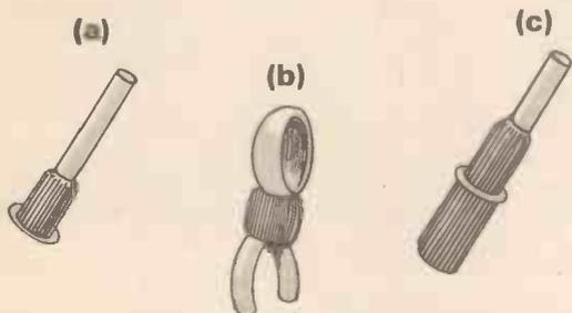
Fig. 4. Types of terminal post. (a) Single-sided. Inserted from the print side, the serrated boss holds the post firm in the hole while the bottom stud is soldered to the print. (b) Eyelet post inserted from component side. (c) Double-sided post.
