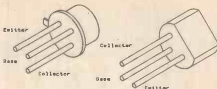
Fig. 3. 3-D equivalents of Fig. 2 (a) and (b).
