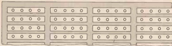
Fig. 1. VQ board consisting of matrix board divided into groups of four holes.
