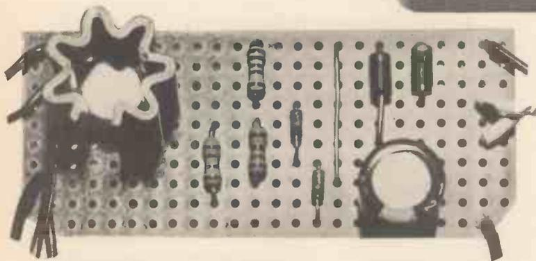
(above) Layout of components inside the plastic case of the prototype mains version. The micro-switch is mounted on the lid together with the spring connector bracket.
