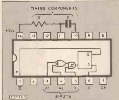
Fig. 3.6. Internal arrangement of 74121 monostable.
