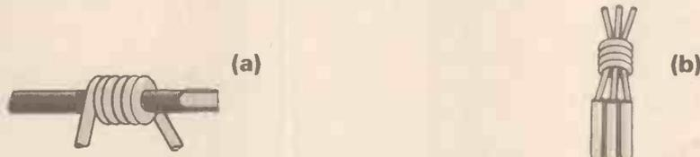
Fig. 3. Above-board connections can be made by making a wire spiral on a screwdriver shaft (a), slipping it over the free wires of the components and soldering (b).
