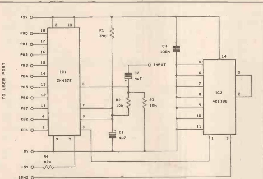
Fig. 2. An A/D converter circuit using a ZN427E.
