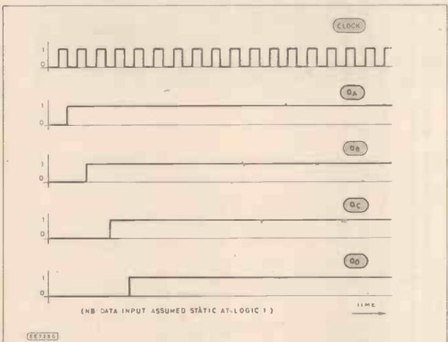
Fig. 3.15. Timing diagram for circuit Fig. 3.14. Data input assumed static at logic 1.
