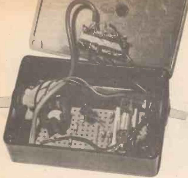
Layout of components inside the plastic case of the battery version.
