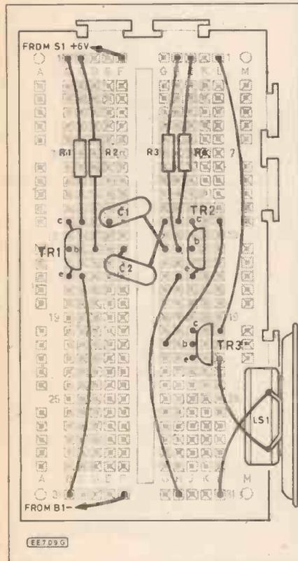
Fig. 7.5. Demonstration breadboard layout for the Simple Buzzer.
