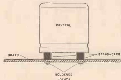
Fig. 1. Using stand-offs to reduce the risk of heat damage when mounting a crystal.
