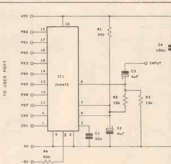
Fig. 1. The circuit of a simple A/D converter based on a ZN447E chip.
