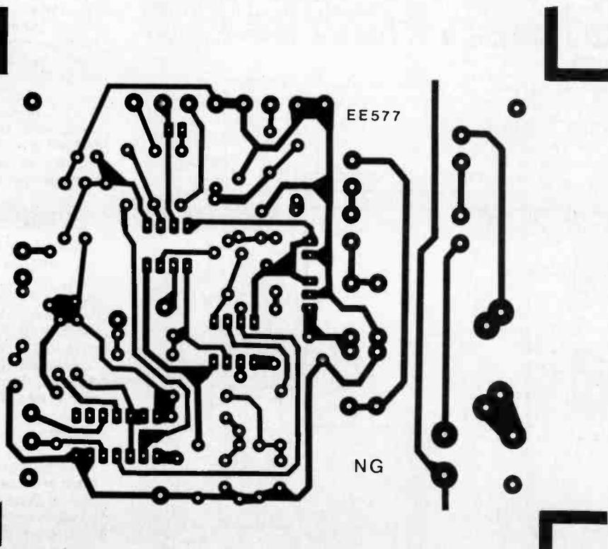
Fig. 2. Component layout and full size printed circuit foil master pattern for the Noise-Gate. Note that the wires terminated with single letters should be a single sleeved link, i.e. x to x, y to y etc, and be soldered on the underside.
