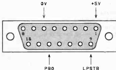
Fig. 3. Rear view of D-plug.
