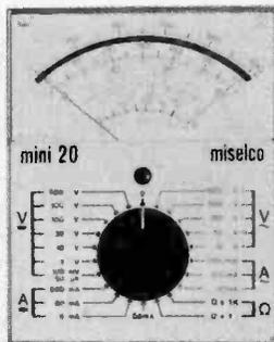
The general purpose Miselco Mini 20 from Alcon Instruments boasts an easy to read mirrored scale, single knob switching and sensitivities of 20k/V d.c. and 4k/V a.c.—Alcon Instruments ☎ 01-352 1897
