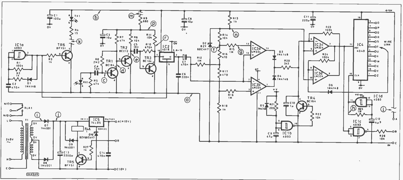
Fig. 2. Some typical measurement "test points" in a working circuit for an Active Infra Red Burglar Alarm (EE Mar '87). Points k, l, and m indicate where current measurements are made.
