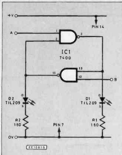
Fig. 15.6. A "flip-flop" circuit using NAND gates.
