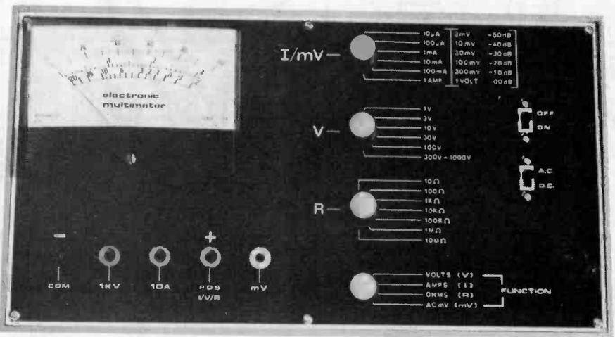
Front panel layout and lettering. The positioning of the p.c.b. and other components is shown below.
