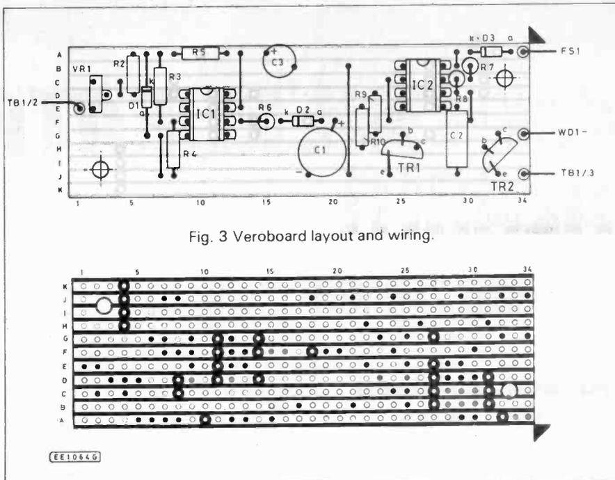
Fig. 3 Veroboard layout and wiring.
