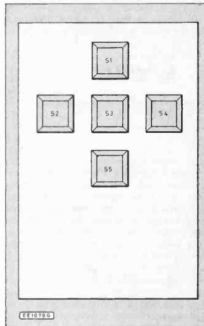
Fig. 4. Suggest keypad layout using low profile p.c.b. mounting switches.
