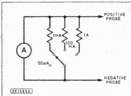
Fig. 5. Circuit diagram of multimeter Current ranges—1A; 100mA and 1mA.
