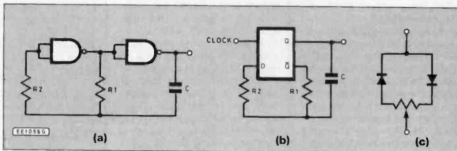
Fig. 1a. CMOS NAND gate oscillator. Fig. 1b. Oscillator built with a "D" type flip-flop. Fig. 1c. Substitute for R1 to obtain variable mark to space output.
