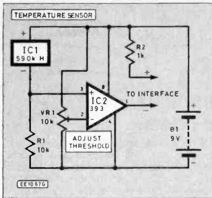
Fig. 1. Temperature sensor signal conditioning (NB: No series limiting resistor need be used within the interface).
