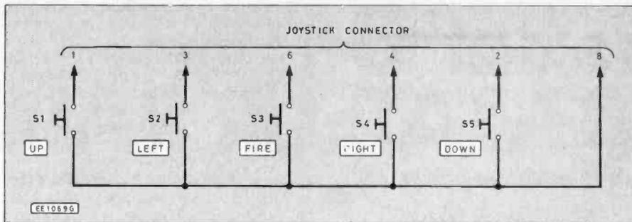
Fig. 3. Keypad circuitry (NB: See July EE for Spectrum Plus Two joystick connections).
