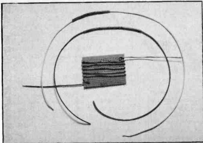
The 10A "shunt resistor" wound around some plain board. Also shown are the two resistor leads, R1 and R46.
