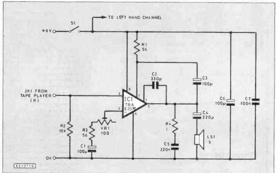
Fig. 1. Circuit of the right hand channel of the amplifier. In the left hand channel VR1 and R3 are replaced by R5. Capacitors C6 and C7 are common to both channels, all other components are duplicated.
