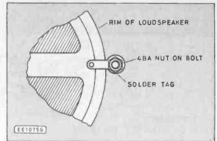
Fig. 5. Loudspeaker mounting.
