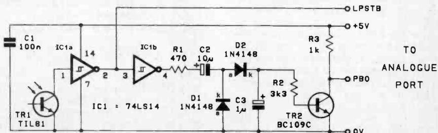
Fig. 2. The light pen circuit diagram.
