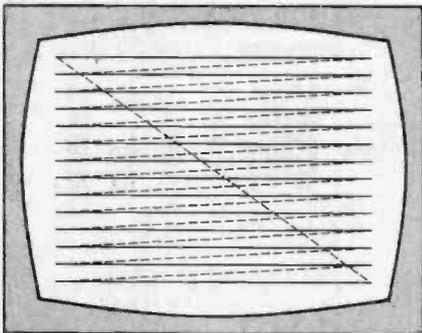
Fig. 1. Computer/television display is produced using this scanning system (dotted lines represent the flyback periods).
