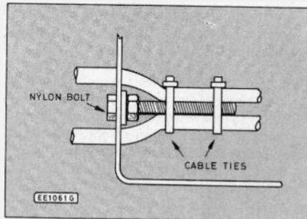
Fig. 4. Method of securing the mains leads.
