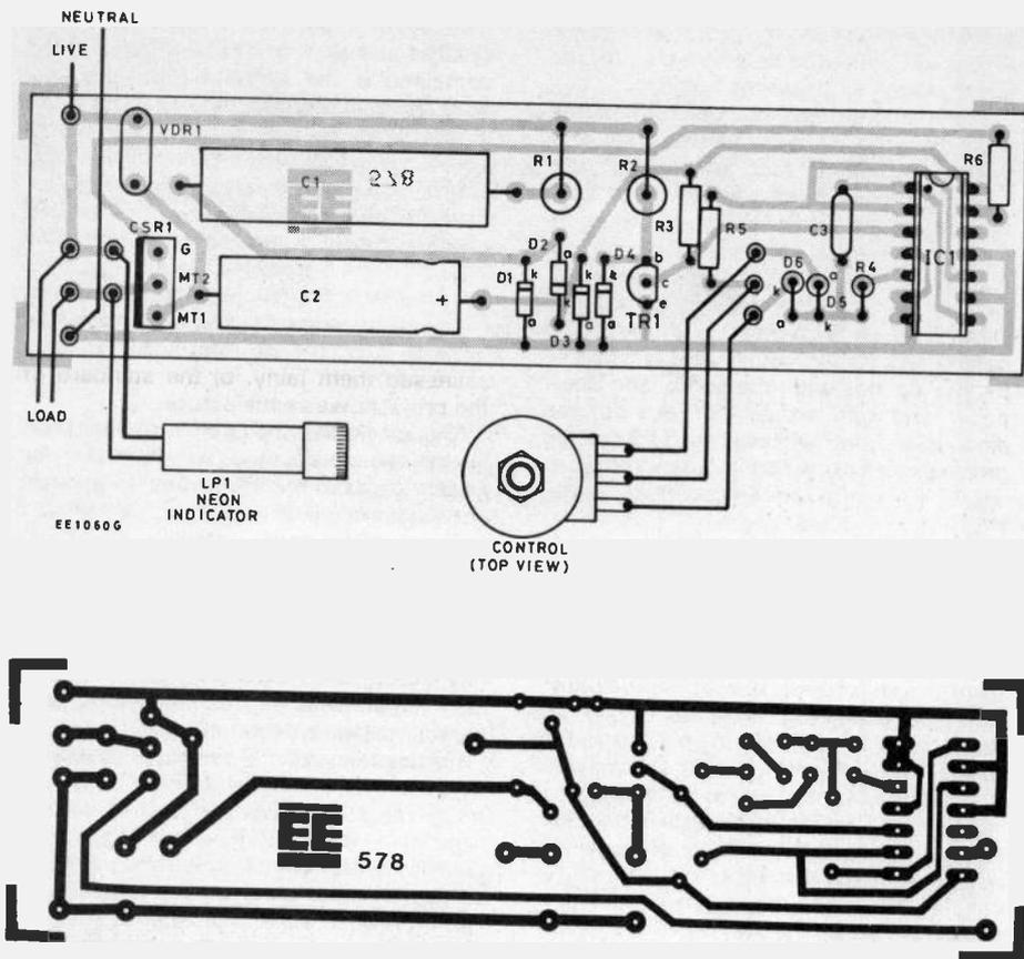
Fig. 3. Layout and wiring of the controller. The earth wires from the mains input and to the load should be connected together with a screw connector—see photo.
