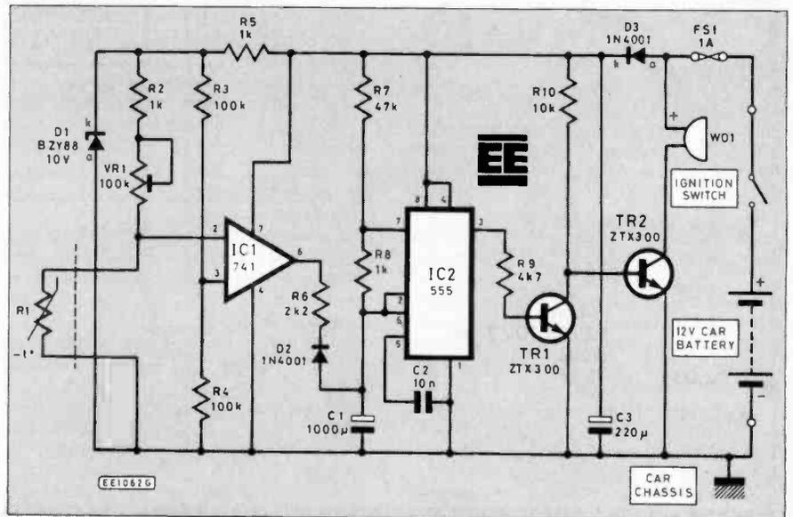
Fig. 1 Circuit diagram of the Car Overheating Alarm.
