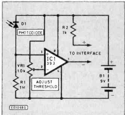
Fig. 2. Light level sensor signal conditioning (NB: No series limiting resistor need be used within the interface).
