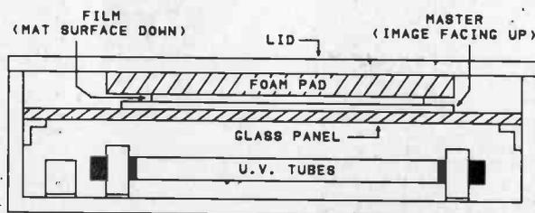
Fig. 1. The set up when using a lightbox to make the exposure.
