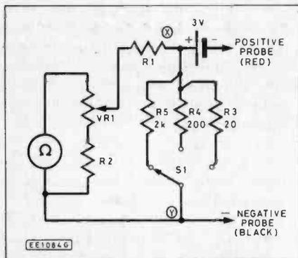
Fig. 4. Circuit diagram of multimeter Ohms ranges—20 ohms; 200 ohms and 2 kilohms (2k).
