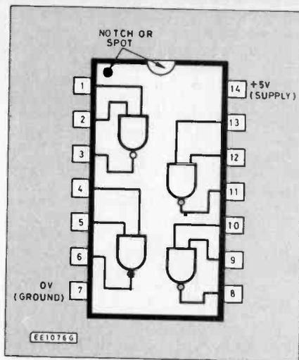
Fig. 15.1. The 7400 i.c. showing the pin connections for its four NAND gates.
