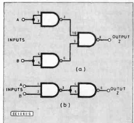
Fig. 15.5. Two more ways of connecting NAND gates.
