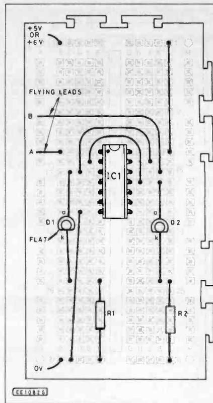
Fig. 15.7. Test-bed component layout for demonstrating the action of the "flip-flop" circuit.
