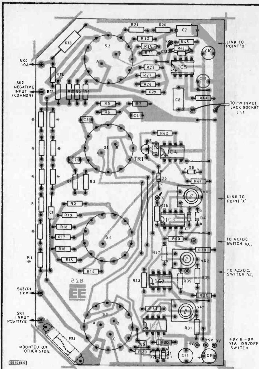
Fig. 2. Component layout on the printed circuit board. Note that the long link wires should be made with plastic insulated connecting wire, see photographs.
