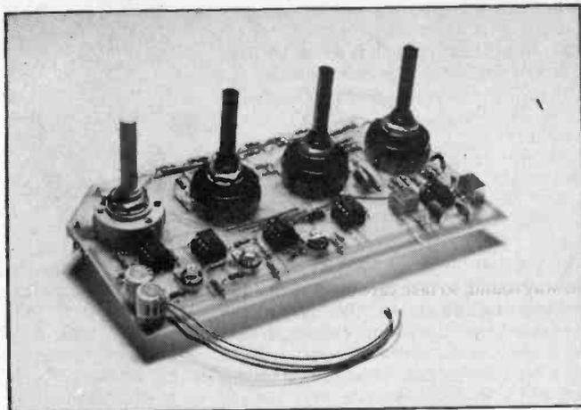
The completed printed circuit board ready for mounting on the rear of the front panel. The board is held in place by the potentiometer fixing nuts.
