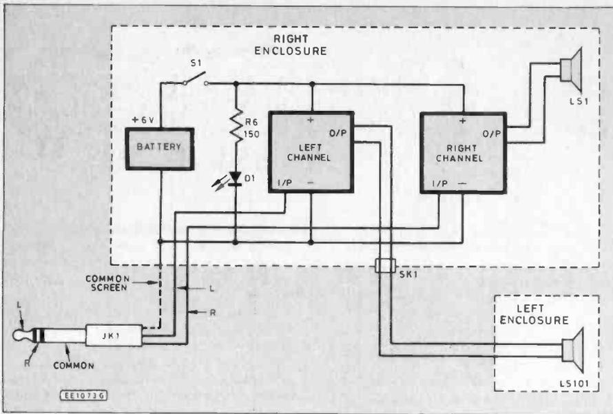
Fig. 3. Interconnection of the various parts of the amplifier system.
