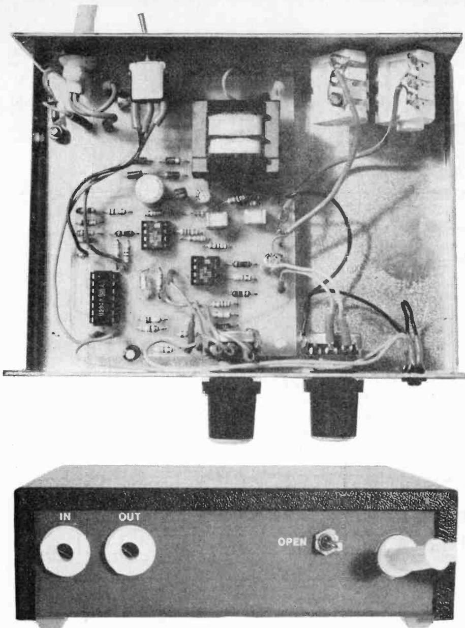
Fig. 3. Front and rear panel wiring and connections to the p.c.b. The internal wiring, board positioning and rear mounted components are shown in the photographs above.
