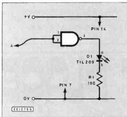
Fig. 15.4. Another way of using a 2-input NAND gate.
