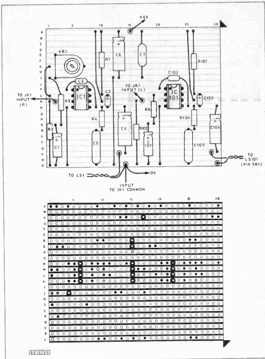
Fig. 2. Components layout and wiring.
