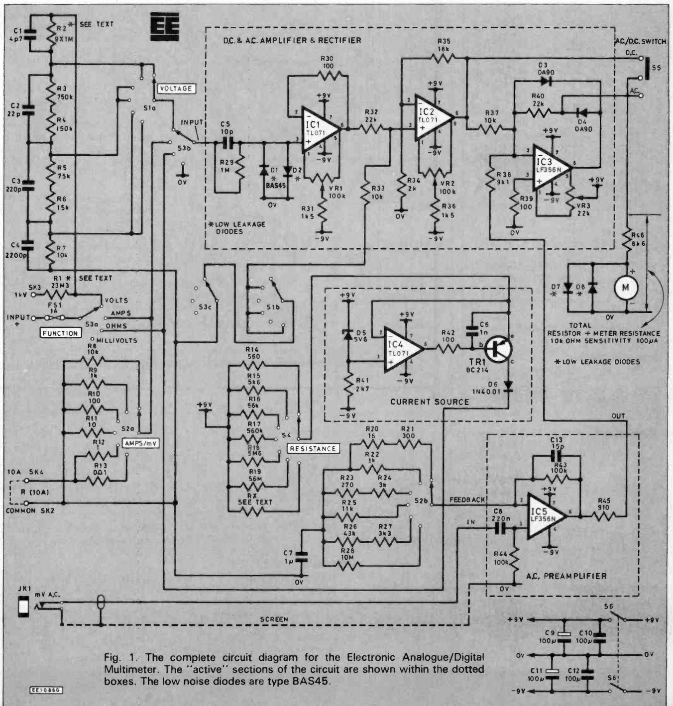
Fig. 1. The complete circuit diagram for the Electronic Analogue/Digital Multimeter. The "active" sections of the circuit are shown within the dotted boxes. The low noise diodes are type BAS45.
