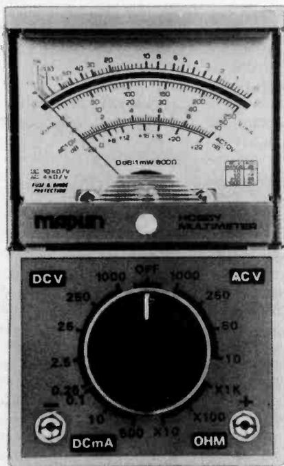
The Hobby Multimeter from Maplin has 10k/V d.c. and 4k/V a.c. sensitivities. The meter also features a clear, easy to read, mirrored scale for accurate reading.—Maplin Supplies ☎ 0702 552911
