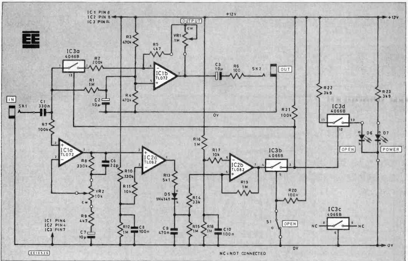
Fig. 1. Complete circuit diagram for the Noise-Gate. The 12V power supply section is shown below.
