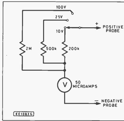
Fig. 3. Circuit diagram of multimeter Voltage ranges—10V; 25V and 100V.
