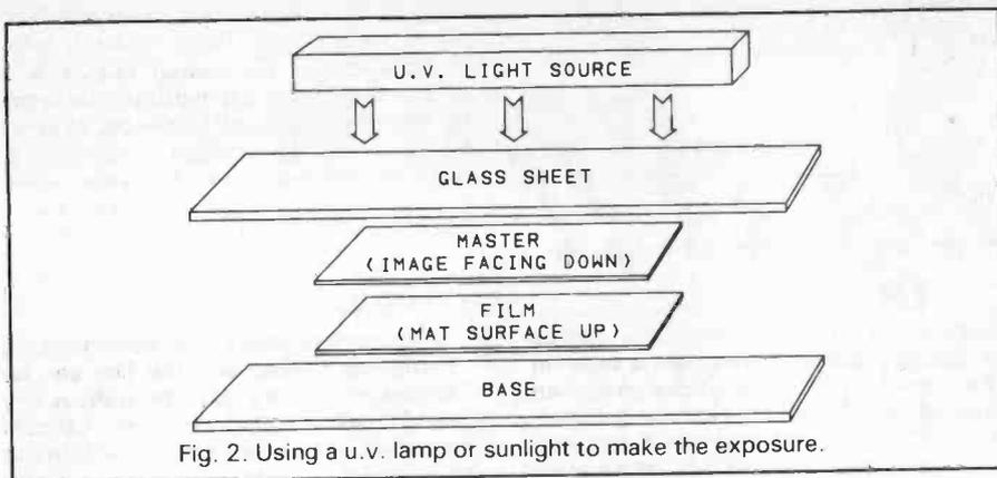
Fig. 2. Using a u.v. lamp or sunlight to make the exposure.
