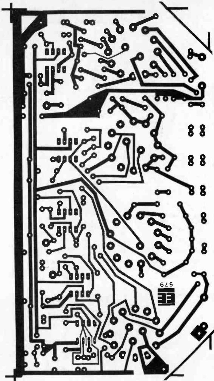
Fig. 3. Full size printed circuit board foil master pattern. This board is available from the EE PCB Service.
