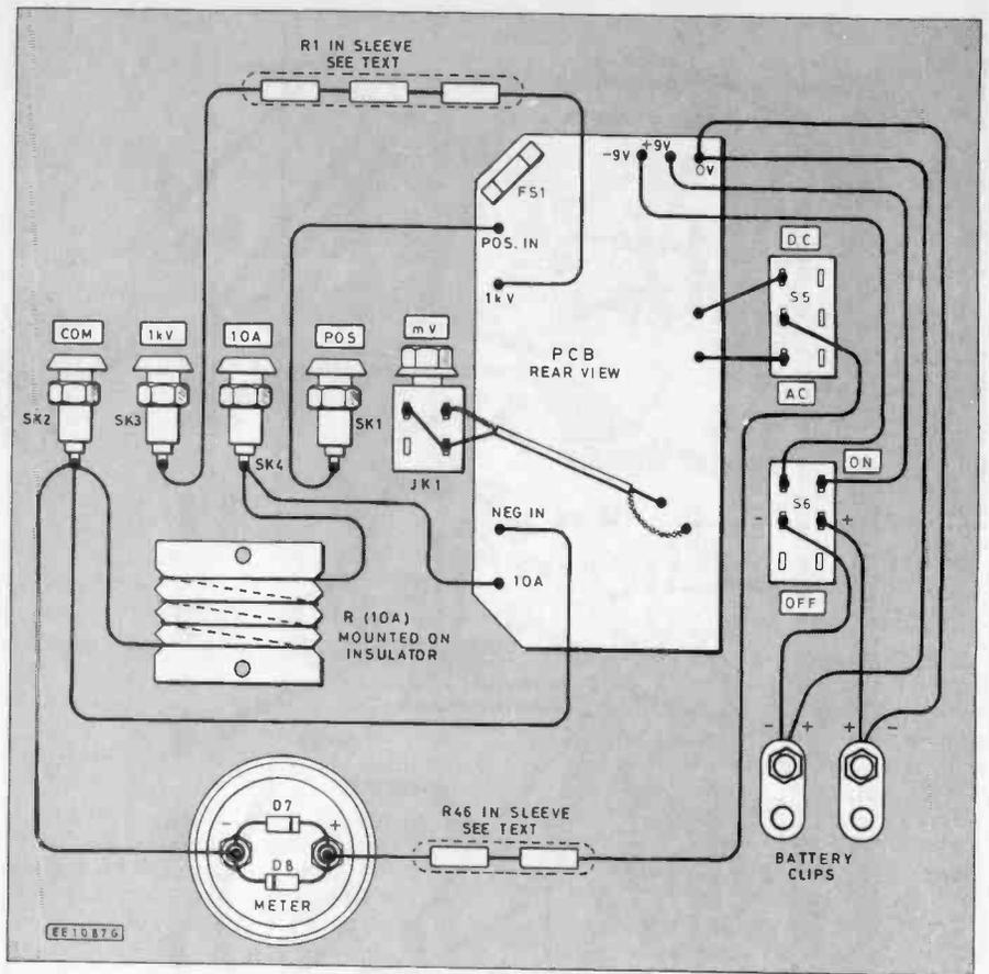
Fig. 4. Interwiring details for the off-board components. The circuit board and components are all mounted on the rear of the front panel. Note the resistors "encased" in plastic sleeving, see photo opposite page.
