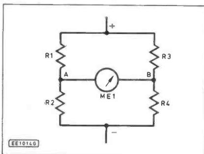
Fig. 1. Basic circuit for a Wheatstone bridge.
