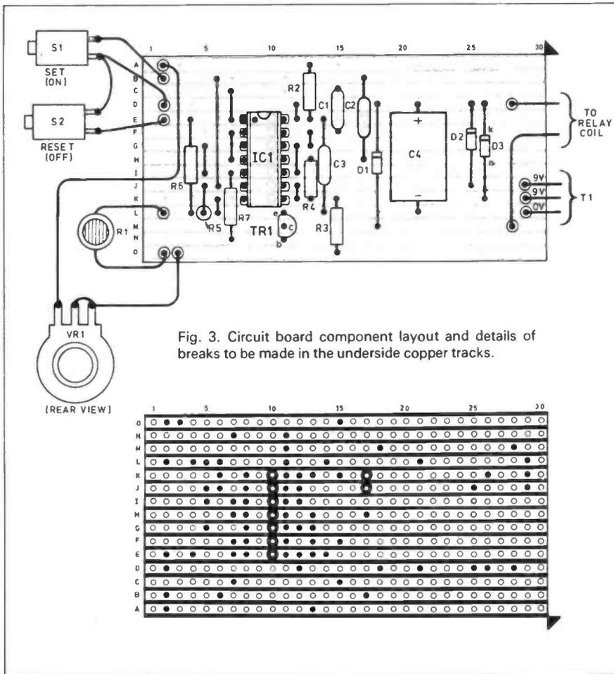
Fig. 3. Circuit board component layout and details of breaks to be made in the underside copper tracks.
