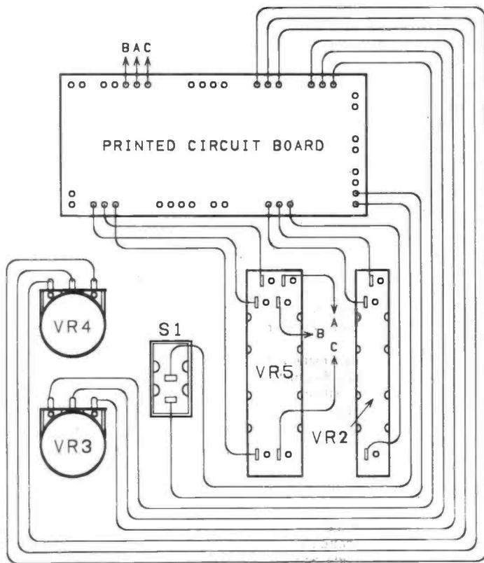
Fig. 4. Interwiring of the controls.
