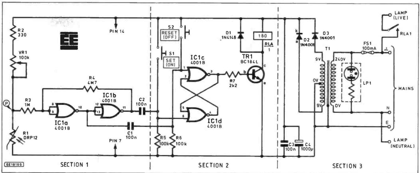
Fig. 2. Complete circuit diagram for the Automatic/Manual Porch Light. This circuit is broken down into three sections; Schmitt trigger, ‘flip-flop’ and power supply.
