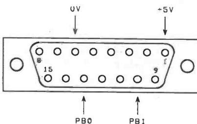
Fig. 1. Using the analogue port to provide two digital inputs.
