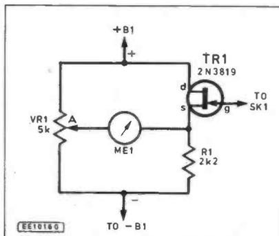
Fig. 3. Complete circuit diagram for the Simple Static Monitor.
