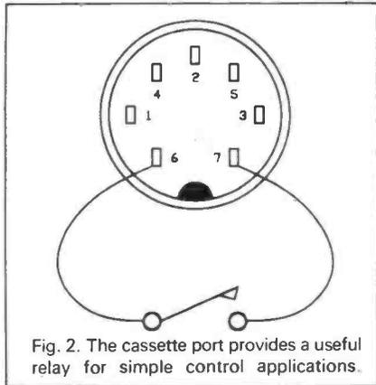
Fig. 2. The cassette port provides a useful relay for simple control applications.
