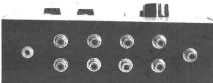
sockets were used for all the input and output sockets, apart from SK3 (the microphone socket) which is a 3.5 millimetre jack type. If necessary though, these can be changed to any types which fit in with your particular audio and video equipment. You might find it better to use BNC connectors for SK1 and SK2 for example.
