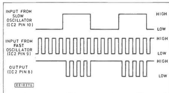
Fig. 16.6. Timing waveforms for the oscillators.
