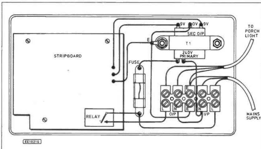
Fig. 4. Interwiring details for the high voltage (mains) section of the unit and wiring to the circuit board. The compact positioning of components inside the plastic case can be seen in the photograph below.
