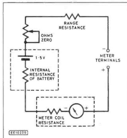
when the ohms-zero resistor is correctly set, all these resistances inside the meter must add up to 1.5k. ( $1.5V/1.5k = 1mA$ .) The whole of the battery's 1.5V is, under these conditions, absorbed by the inside resistances.
