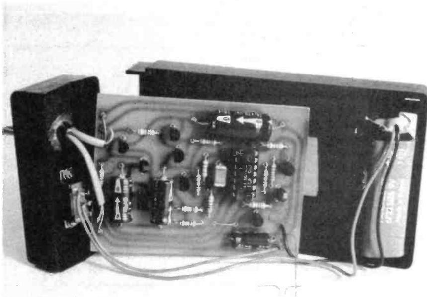
connected. The current drawn from the supply should be checked; after the initial surge as C5 charges this should fall to a mere 3mA or so. Five volts should appear across the 10μ capacitor C4, indicating correct operation of the regulator IC2. With respect to negative, an analogue meter should indicate about 2V to 2.5V at each probe connection, possibly with a slight visible flicker. If it does not, the appropriate outputs of IC1 (pins 10 and 11) can be checked as a first step.
