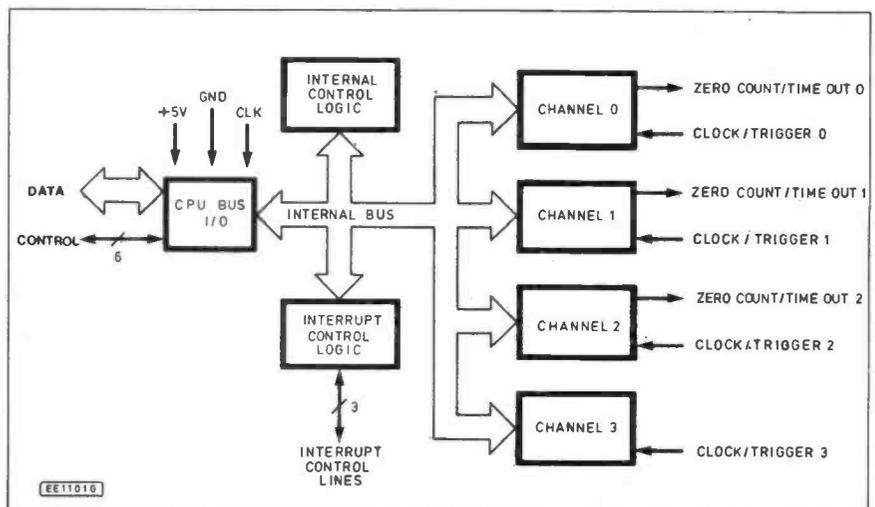
Fig. 1. The internal architecture for the Z80-CTC microprocessor.
