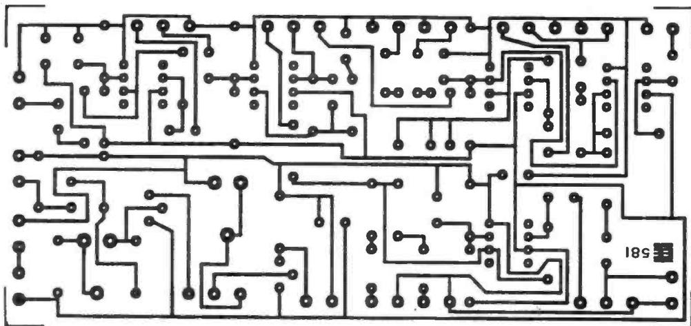
Fig. 3 Printed circuit board layout and wiring for the Video Controller. The \*s mark the earth connections.
