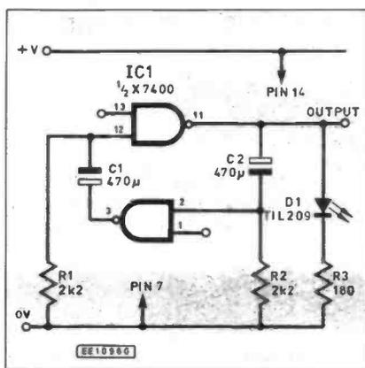
Fig. 6.1. Oscillator circuit using two NAND gates.
