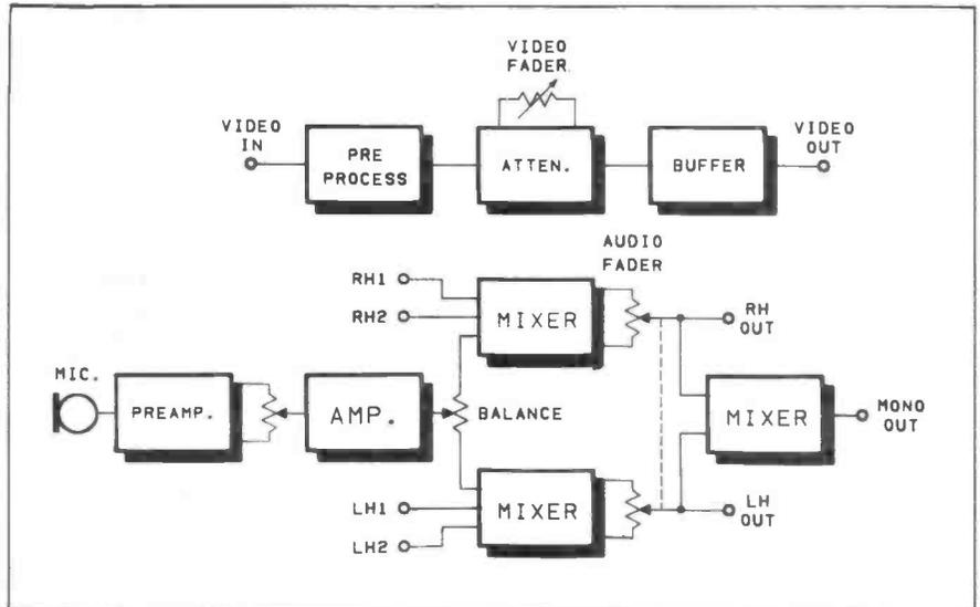
Fig. 1. Block diagram of the Video Controller.
