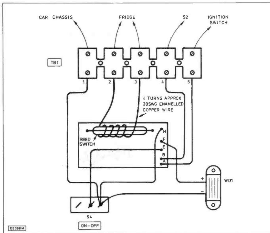
Fig. 3. Details of interwiring from the circuit board to the 5-way terminal block, rocker switch and the warning buzzer.
