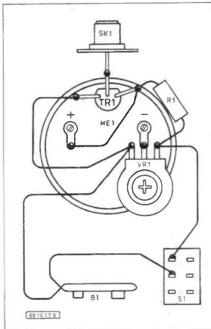
Fig. 4. Wiring details for the prototype model. The f.e.t. transistor is mounted directly on the coaxial socket.
