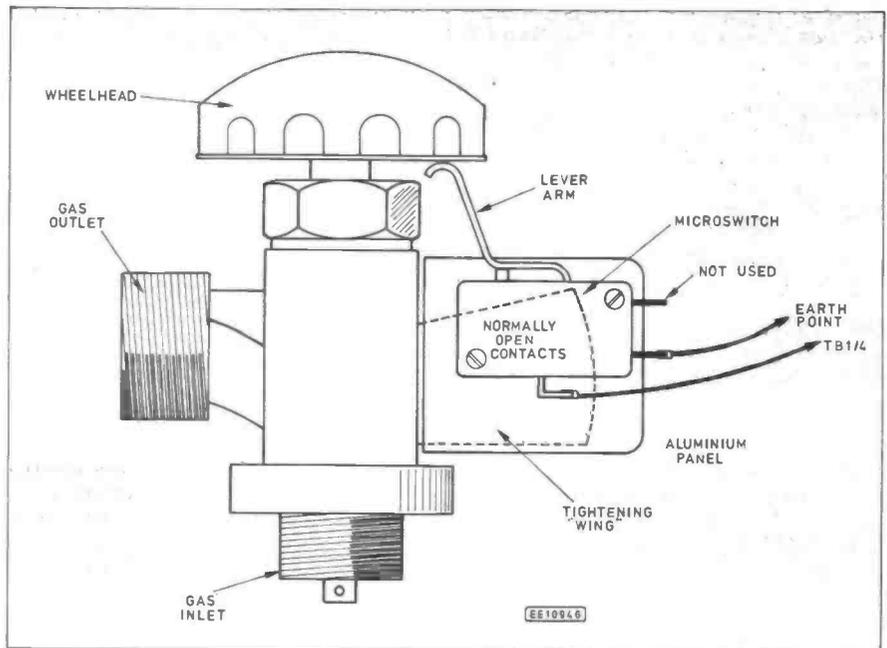
Fig. 4. Suggested method of mounting the microswitch below the gas supply "valve" control knob. The microswitch operating lever should be carefully bent so that adjustment of the gas knob operates the lever arm. *If there is any doubt about being able to make a safe job, the assistance of a qualified caravan gas fitter must be sought.*
