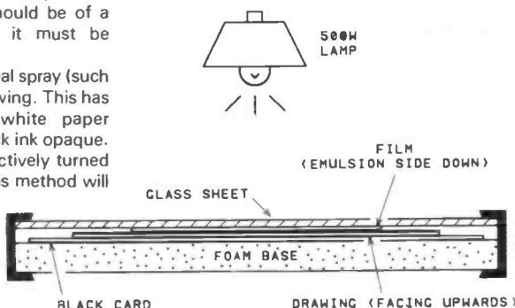
Fig. 1. Basic set up used by the CM100 kit.
