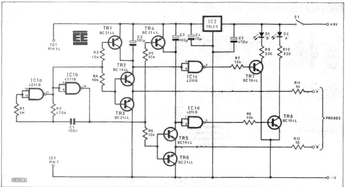
Fig. 1. Transtest circuit diagram
