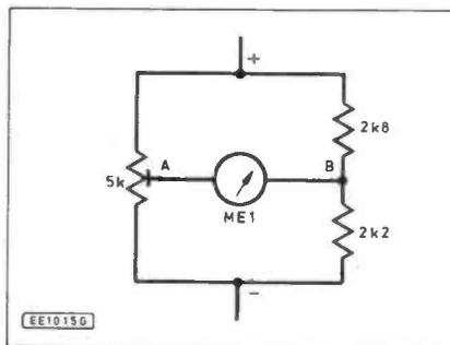
Fig. 2. Adding a potentiometer to "balance" the bridge circuit.
