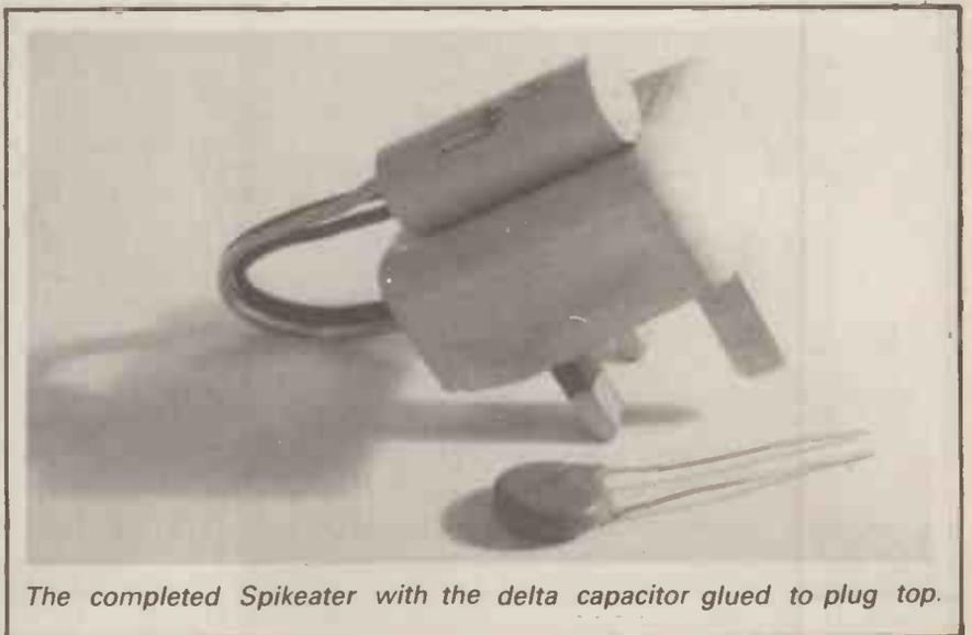
*The completed Spikeater with the delta capacitor glued to plug top.*
