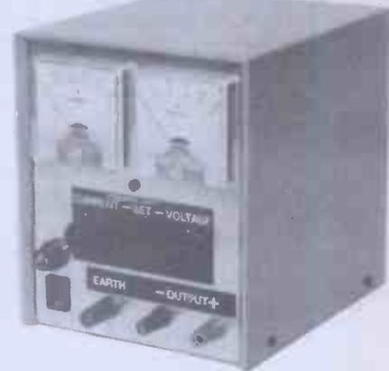
A superb design giving 0-25V and 0-2.5A. Twin panel meters indicate Voltage and Current. Voltage is variable from zero to 25V. Current-Limit control allows Constant Current charging of NICAD batteries, and protects circuits from overload. A Toroidal transformer MOSFET power output device, and Quad op-amp IC design give excellent performance.
