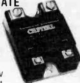
Zero voltage switching - no radio interference. 2.5KV input to output isolation. 4 KV terminals to heatsink isolation. 3V to 32V input voltage easily interlaced to TTL or CMOS logic. 24V to 240V rms load voltage. Inductive load switching. Built-in snubber network. 10A max. 4A with no heatsink at 40°C.
