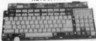
**Z8852 Keyboard:** Superb brand new keyboard 392 x 181 with LCD displaying 1 line of 10 characters and a further line with various symbols. 100 keys, inc. separate numeric keypad. Chips on board are 2 x 74HC05, 80C48. LCD + driver chips are easily removable from board. .... £15.00
