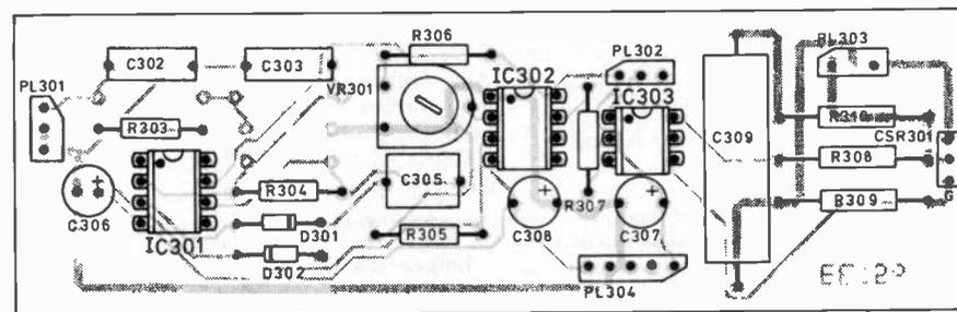
Fig. 6(c). "High" range filter/triac p.c.b. layout.
