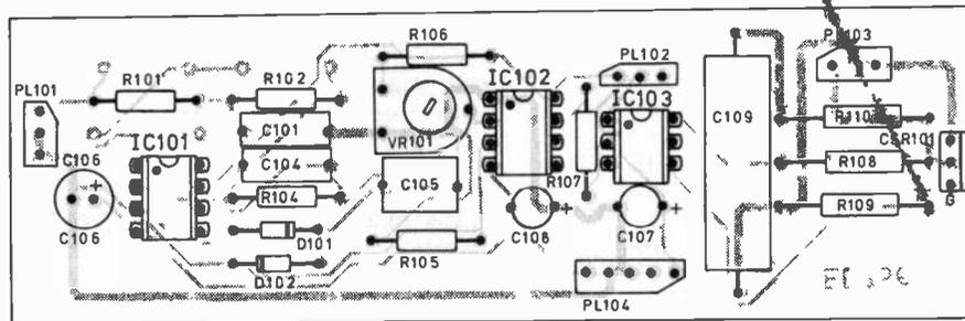
Fig. 6(a). "Low" range filter/triac p.c.b. layout.
