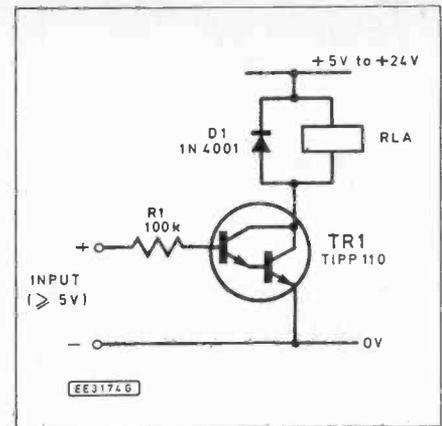
Fig. 8.3. Relay driver based on a plastic Darlington transistor.
