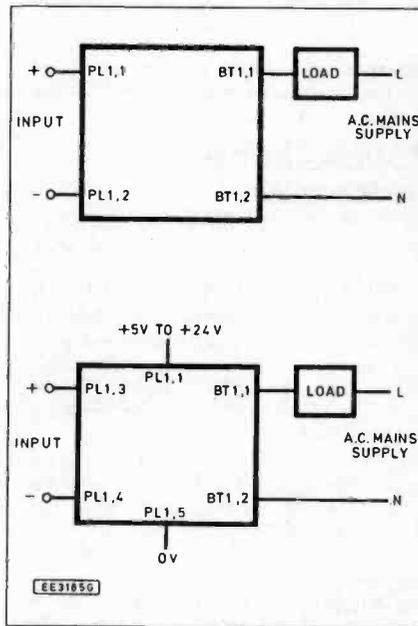
Fig. 8.14. Operating configurations for the Solid-State Switch Module (a) basic Solid-State Switch (R1 and TR1 not fitted) (b) sensitive Solid-State Switch (R1 and TR1 fitted).
