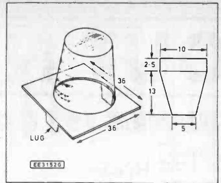
Fig. 7. Mounting the beacon light cover.
