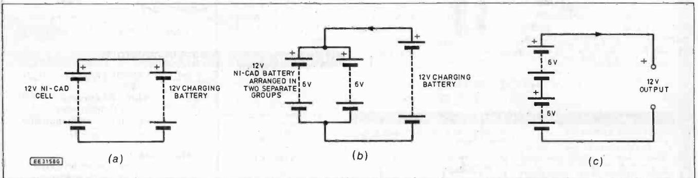
Fig. 1a. The charging battery cannot charge the NiCad cells because the two voltages are equal and opposite. No current therefore flows in the circuit.
