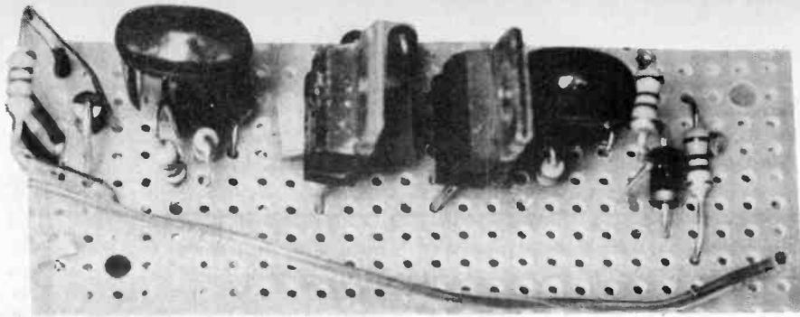
The completed circuit board. Small 20mm square aluminium heatsinks should be bolted to the two i.c. tabs – see photograph below.
