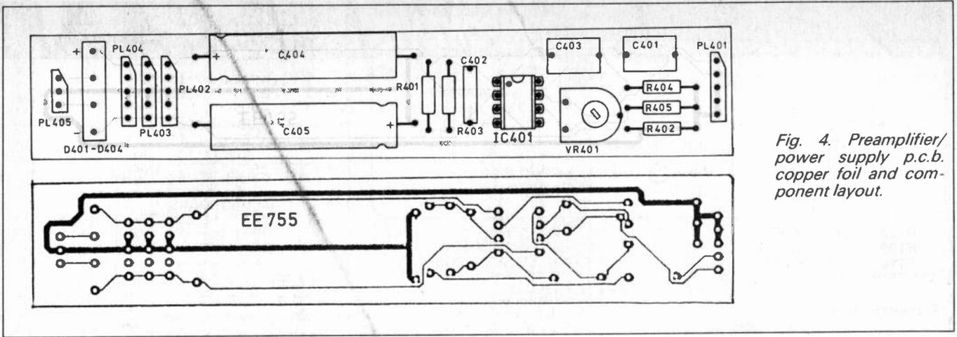
Fig. 4. Preamplifier/power supply p.c.b. copper foil and component layout.
