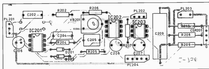
Fig. 6(b). "Mid" range filter/triac p.c.b. layout.
