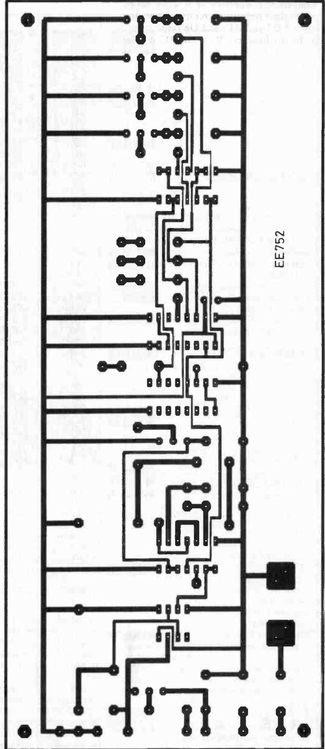
Fig. 3. Printed circuit board component layout and full size copper foil master pattern. A lead is also taken directly from one side of switch S2 to pin 7 of DIN socket SK1.
