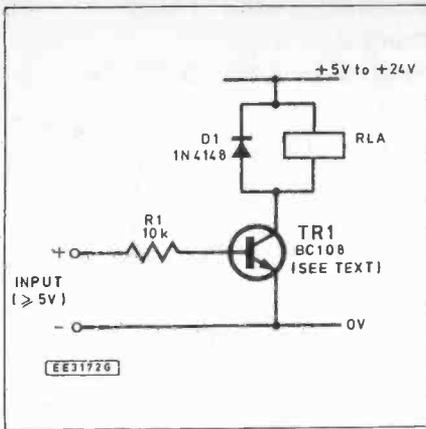
Fig. 8.1. A simple relay driver circuit.
