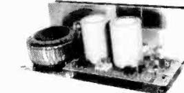
**OMP/MF200 Mos-Fet** Output power 200 watts R.M.S. into 4 ohms, Frequency Response 1Hz - 100KHz - 3dB, Damping Factor >300, Slew Rate 50V/uS, T.H.D. Typical 0.001%, Input Sensitivity 500mV, S.N.R. -130dB, Size 300 x 155 x 100mm.
