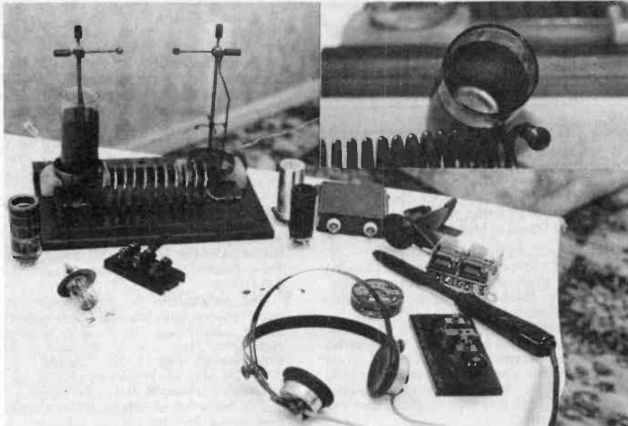
An early static electricity experiment is shown utilising a coil and two Leyden jars (one jar has been removed to show "static collector"). Inset reveals the lead coating, both inside and outside of the jar, which forms a capacitor. Other components shown are a switch (to earth the aerial when not in use); a microwave valve; coils and capacitors (the tiny dots behind the phones are latter-day capacitors); a Morse key; an early "Solon" soldering iron – and a tin of "Fluxite".
