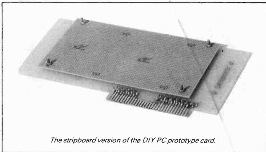
The stripboard version of the DIY PC prototype card.
