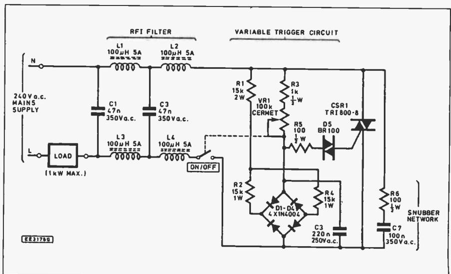
Fig. 8.7. Triac a.c. power controller for up to 1kW of tungsten filament lighting.
