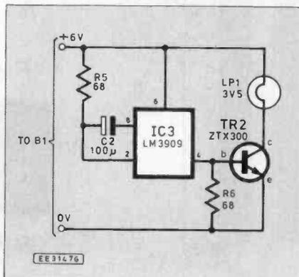
Fig. 2. Circuit for the flashing blue light beacon.
