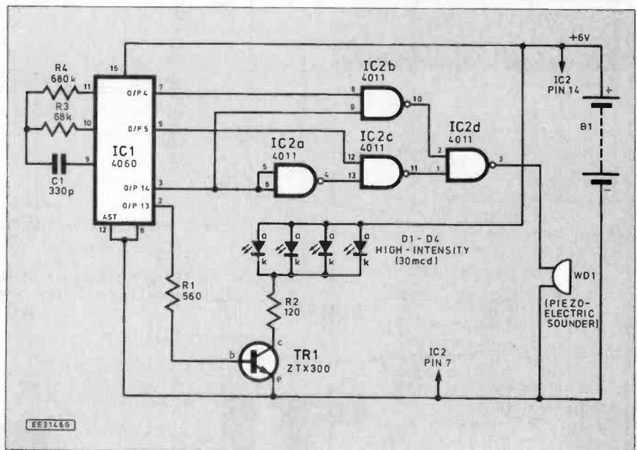
Fig. 1. Circuit diagram of the hazard flashers and siren section.
