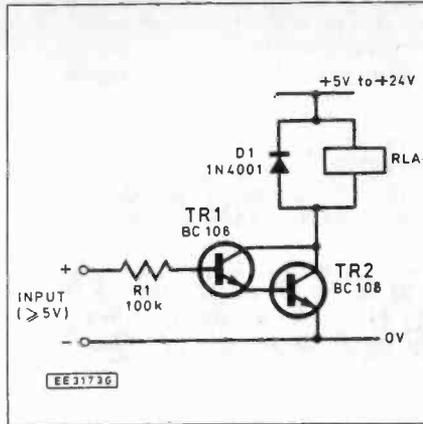
Fig. 8.2. Relay driver circuit based on a discrete Darlington arrangement.
