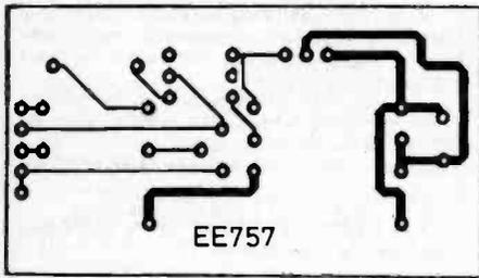
Fig. 8.13. P.C.B. track and component layout for the Solid-State Switch Module.
