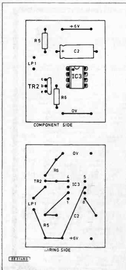
Fig. 6. Beacon circuit card construction.
