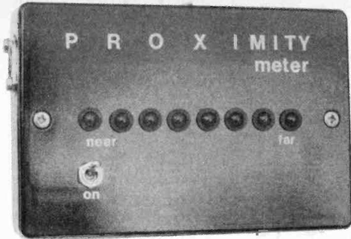
Front panel layout of the Display Unit.
