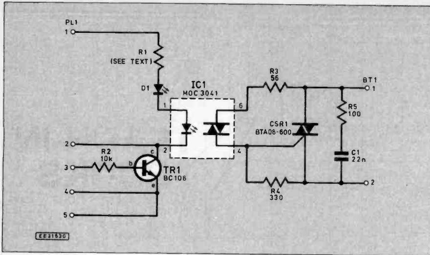
Fig. 8.12. Complete circuit diagram for the Solid-State Switch Module.
