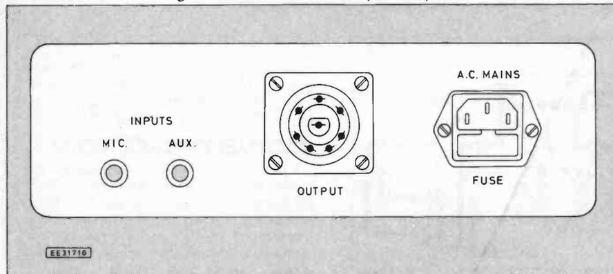
Fig. 8. Recommended rear panel layout.
