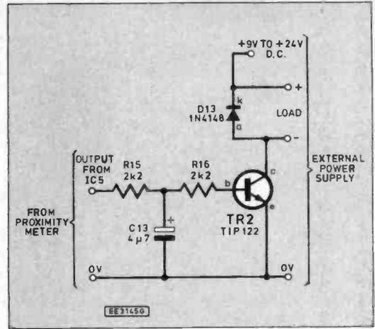
Fig. 6. External output driver circuit diagram.
