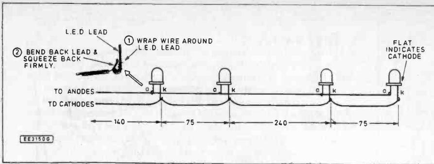
Fig. 5. Connection and wiring of the I.e.d.s.
