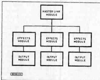
Fig. 1. Using Masterlink to synchronize any number of effects modules.
