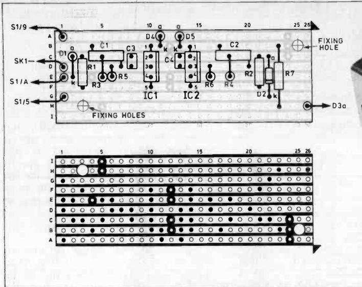
Fig. 3. Stripboard component layout and details of breaks required in the underside copper tracks.
