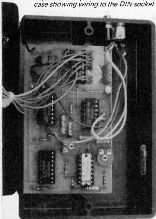
(right) The completed circuit board mounted in a small plastic case. The ultrasonic transducers are glued to one side panel and the screened lead is held in the recess by the lid.
