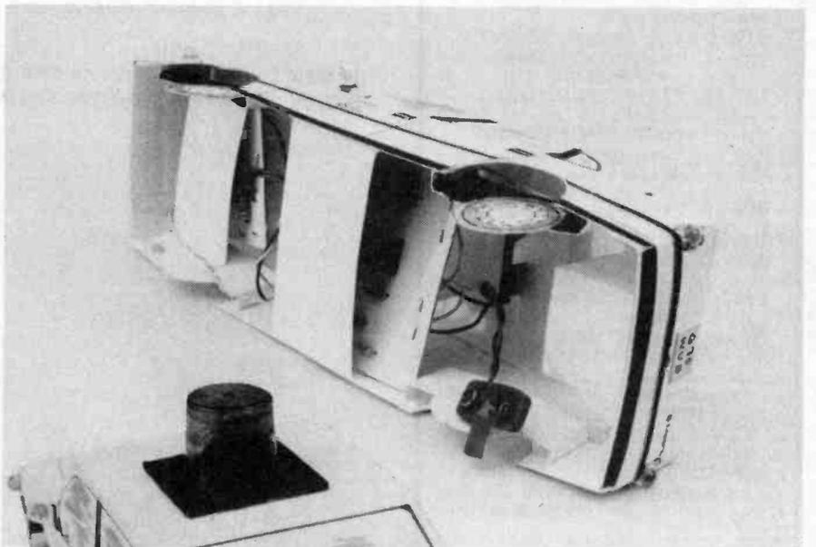
Internal structure of the Police Car showing the circuit cards and rear battery mounting.
