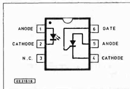
Fig. 8.10. Optically coupled thyristor.
