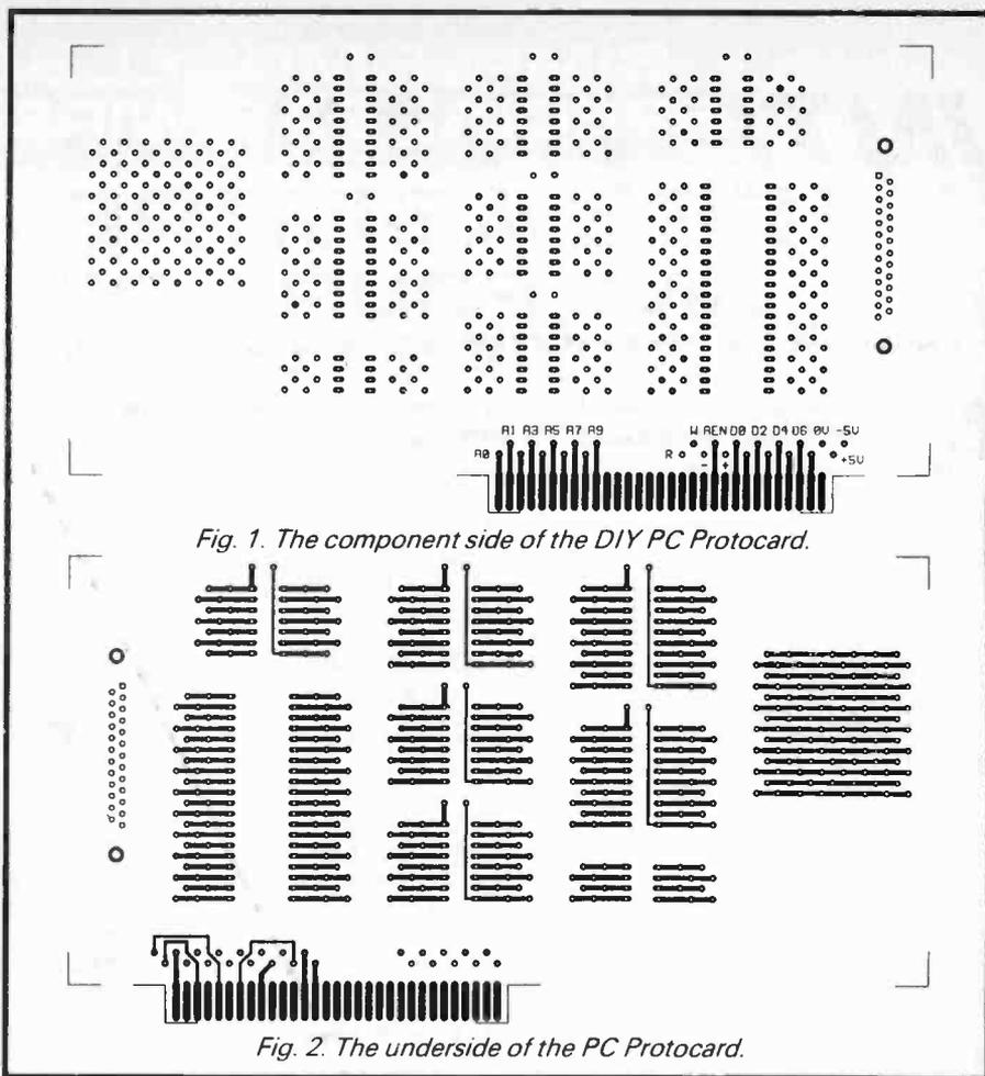
Fig. 1. The component side of the DIY PC Protocard.
