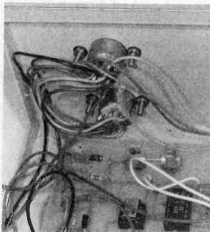
(above) Wiring to front panel components, completed board and (left) interwiring to the rear DIN sockets.
