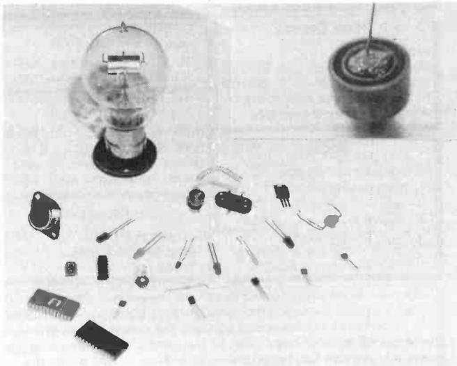
An early thermionic "bright-emitter" triode valve, circa 1907; a galena crystal and catswhisker (point-contact shown in inset); and a miscellany of more modern diodes, i.e.d.s and transistors; some integrated circuits and an EPROM.
