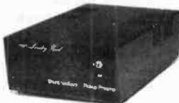
This new circuit by John Linsley Hood uses latest generation integrated circuits in the sonically preferred shunt feedback configuration to give an accurate and musical sound, with the ability to use moving magnet and moving coil cartridges.
