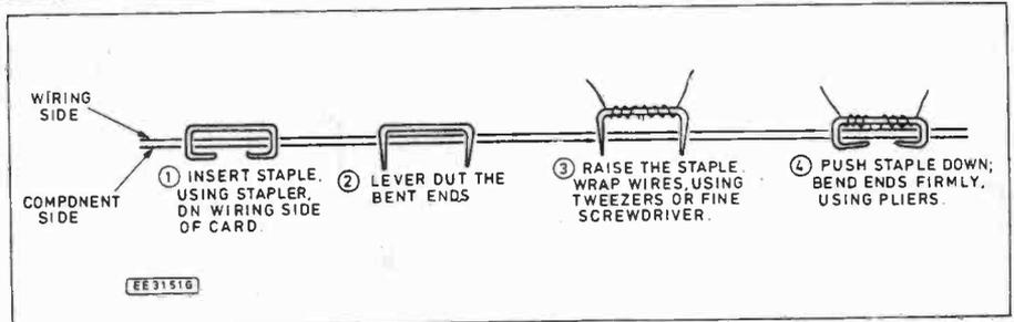
Fig. 4. Method of using staples to fix the flying lead connections.
