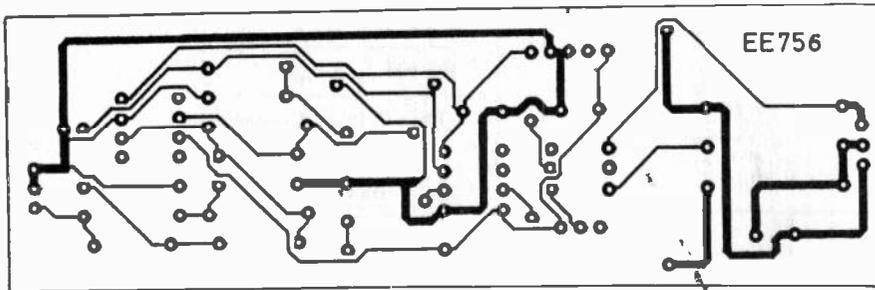
Fig. 5. Filter/triac p.c.b. copper foil layout.
