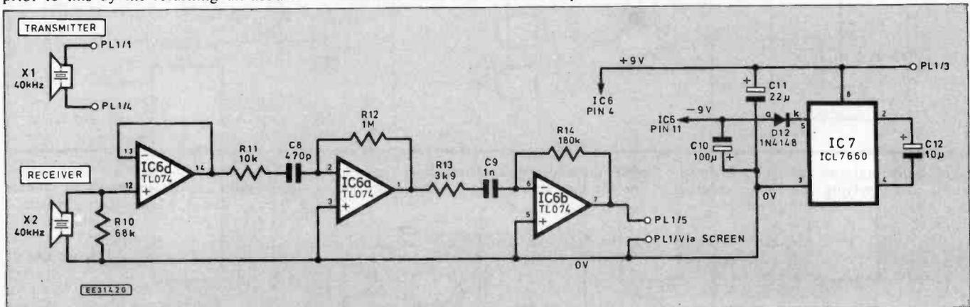
Fig. 3. Circuit diagram for the Sensor Unit.
