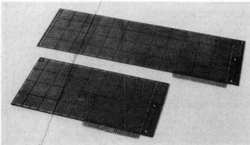
On the main part of the board there is no need for a complete matrix of holes. Some d.i.l. clusters connected to some pads are sufficient to accommodate TTL chips, a PLA chip, or whatever. A small area of pads and copper strips will accommodate transistor oscillators, amplifiers, etc. Provision for a 25-way D-connector for input/output lines is more than a little helpful.
