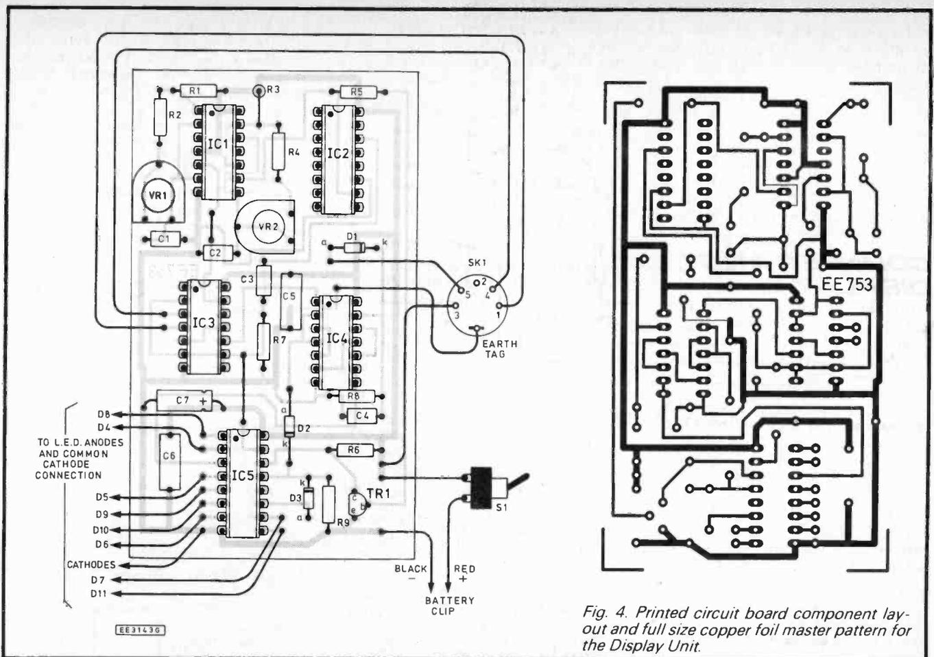
Fig. 4. Printed circuit board component layout and full size copper foil master pattern for the Display Unit.
