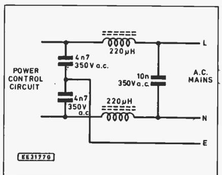
Fig. 8.6. Typical RFI filter.
