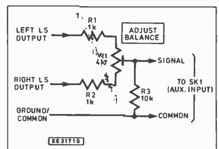
Fig. 10. Stereo loudspeaker signal combiner.
