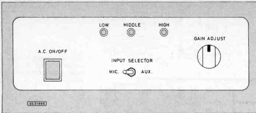
Fig. 7. Recommended front panel layout.
